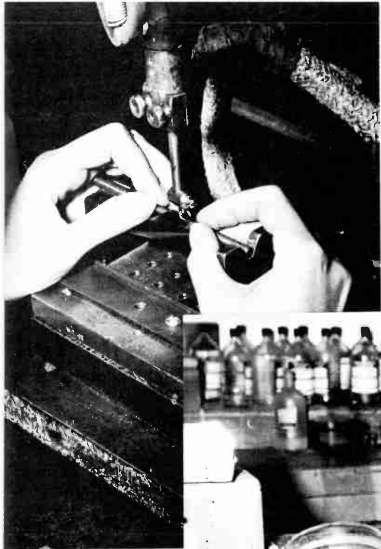
After forming on a tapered mandrel, nickel grid supports are then carefully welded
