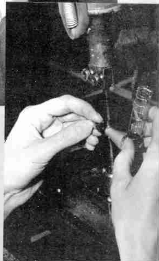
When the grid support has been welded to the grid, the grid lead is welded to the support and the result is a
