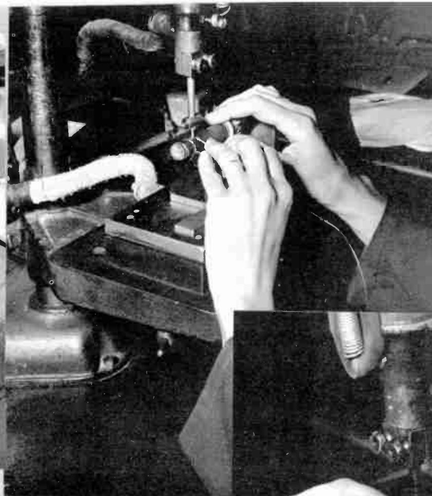
Platinum wire is wound around the grid skeleton in a spiral and welded to the strands of wire which form the grid.
