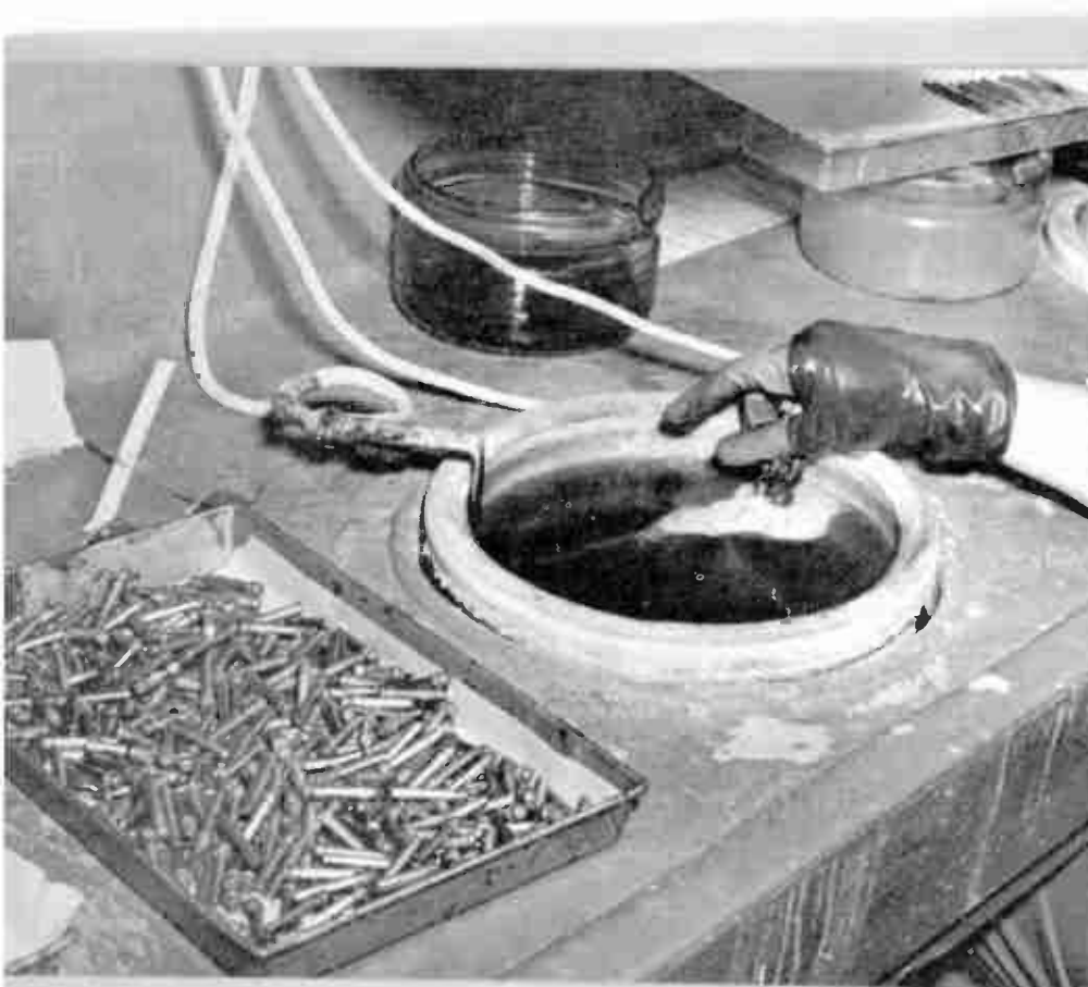
Grid leads are cleaned in an electrolytic solution in the Chemical department both before and after the beading is done. The operation shown here is more commonly known as "nitriting."
