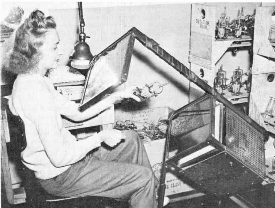
Strains just don't get by! Here Jo Russell demonstrates the use of a polariscopes in checking a tube assembly for glass strains
