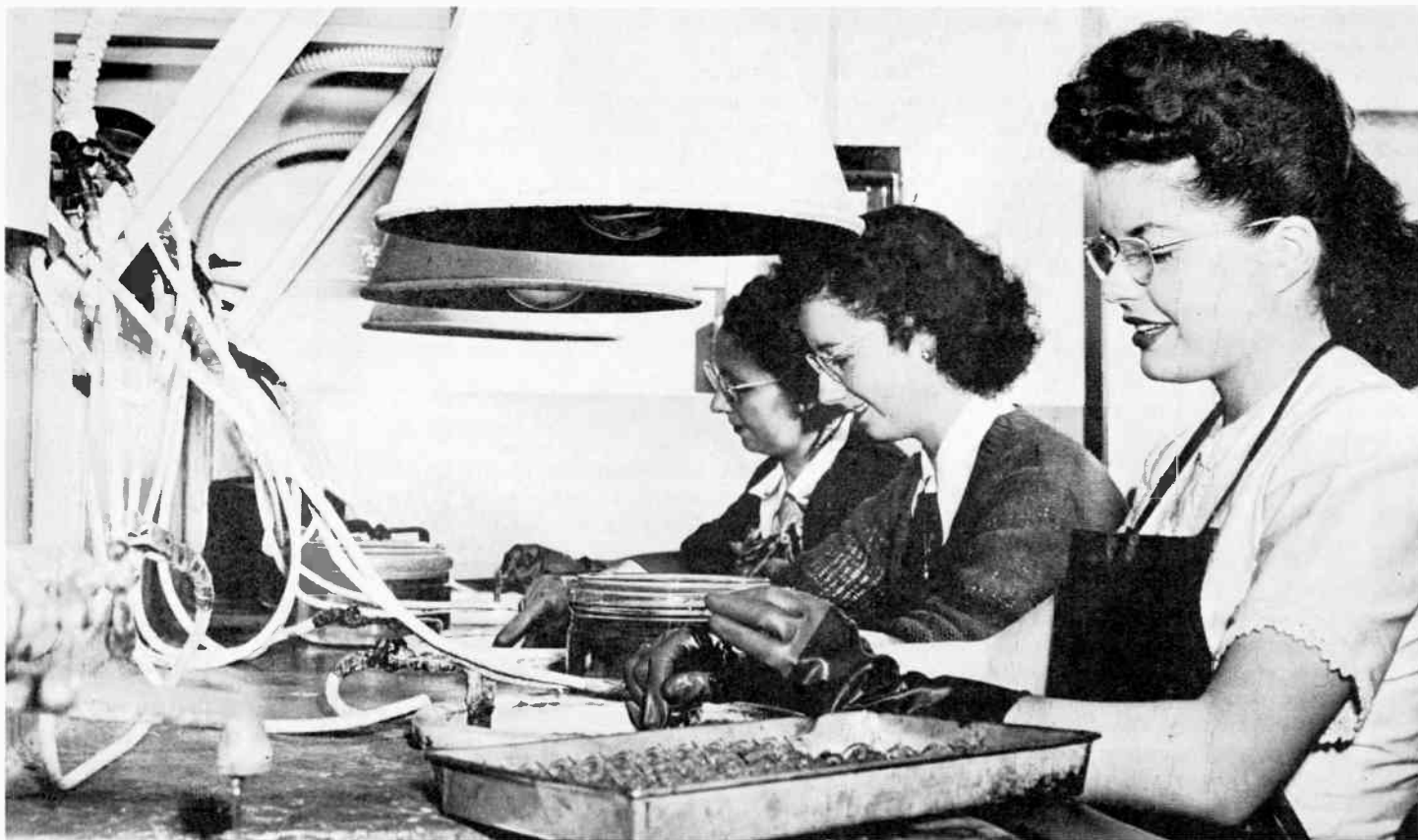
Gertrude Huggenberger, Marge Lage and Marge Hunt (foreground) perform the nitriting operation at one of the many rows of nitrite pots located in the Chemical department
