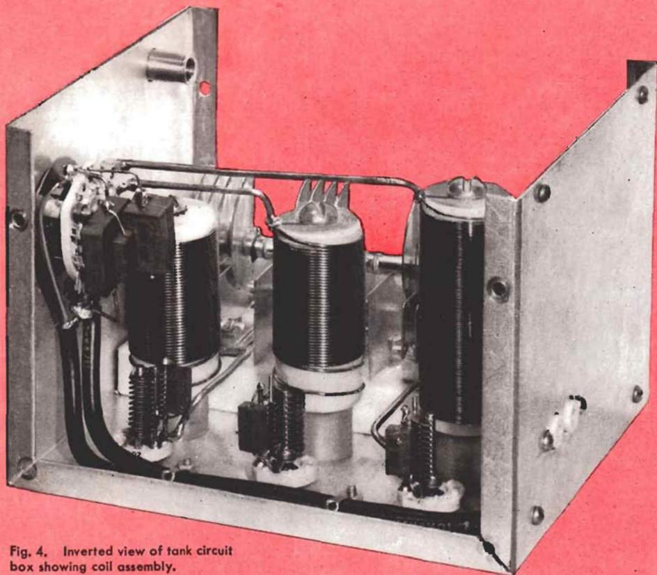
Fig. 4. Inverted view of tank circuit box showing coil assembly.
