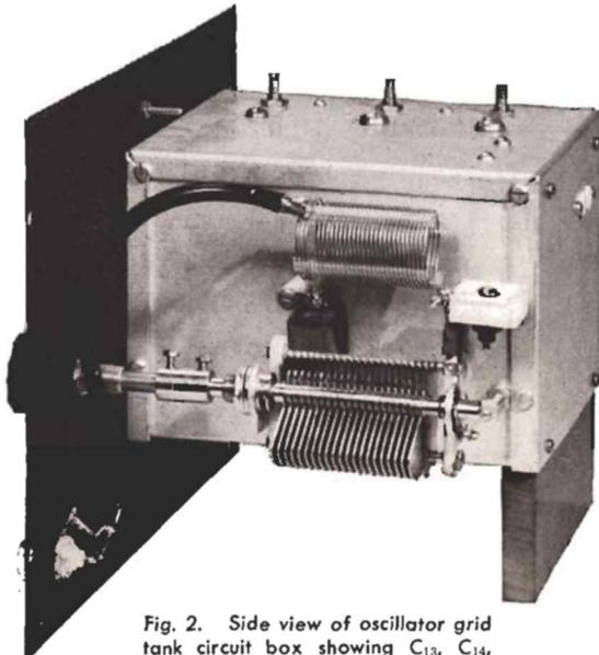
Fig. 2. Side view of oscillator grid tank circuit box showing  $C_{13}$ ,  $C_{14}$ ,  $C_{15}$ ,  $L_4$  attached to removable cover.
