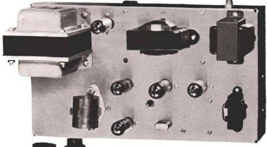
Fig. 4. Top view of the double sideband transmitter, showing the locations of major parts on chassis deck. Check to see that sufficient space is provided for components which differ in size and shape from those listed. The audio filter inductor  $(L_2)$  and the microphone transformer  $(T_3)$  should be oriented in the positions shown to prevent inductive hum pickup from the power transformer  $(T_1)$ .
