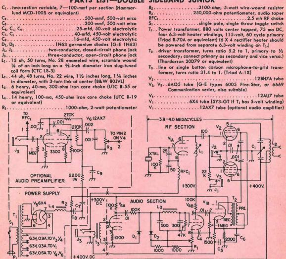
Fig. 2. Schematic diagram for the complete 20-watt double sideband transmitter. The high voltage power supply, shown within dotted lines, may be eliminated if a suitable supply already is available. The optional audio preamplifier appears in the upper left-hand corner. Capacitances given in whole numbers are mica, 500 volts working; those in decimals are disc ceramic, 500 volts working. Resistors are  $\frac{1}{2}$  watt unless otherwise specified.
