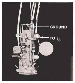
Fig. 6. Detail views of the audio preamplifier stage constructed on a turret type 9-pin miniature tube socket (Vector No. 8-N-97). Terminals to which external connections are made have been labeled.
