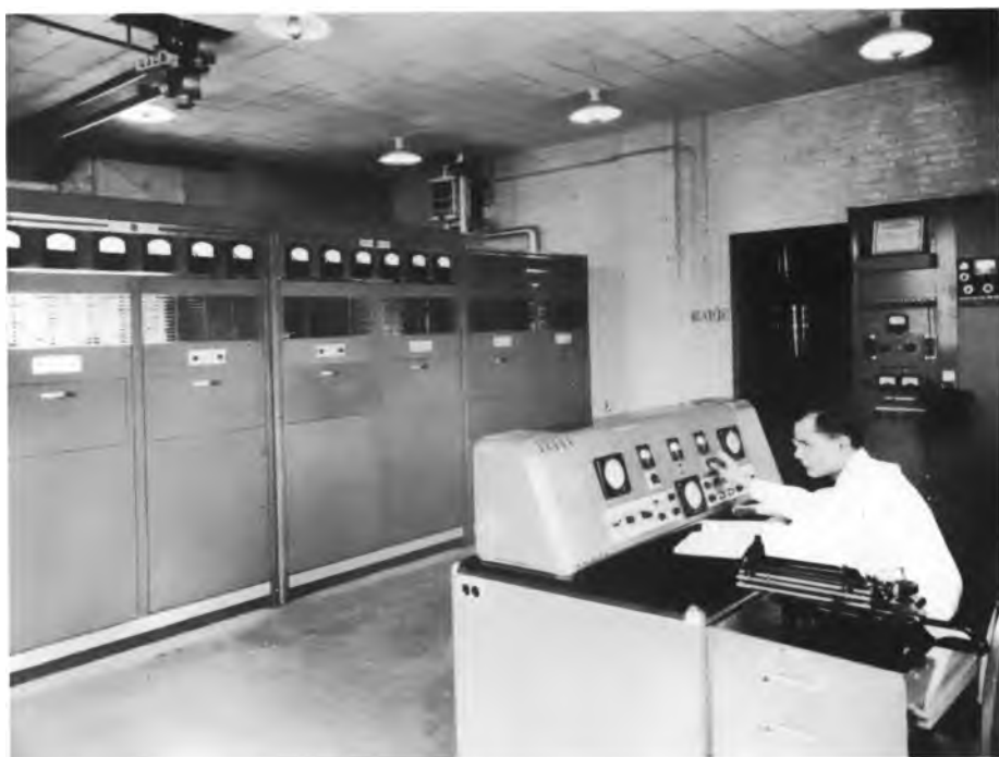
FIG. 1. 50-KW. G.E. FM TRANSMITTER SET UP FOR TESTS UNDER OPERATING CONDITIONS
