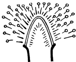
When a tungsten filament is heated by electricity in a vacuum, electrons boil out of it.
