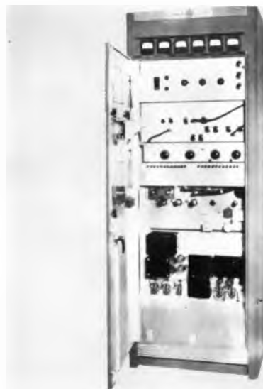
The S-T transmitter operates in the 260- to 350-mc range. It is compact, occupying less than five square feet of floor space.
