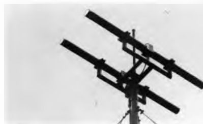
The S-T transmitting and receiving antenna.
