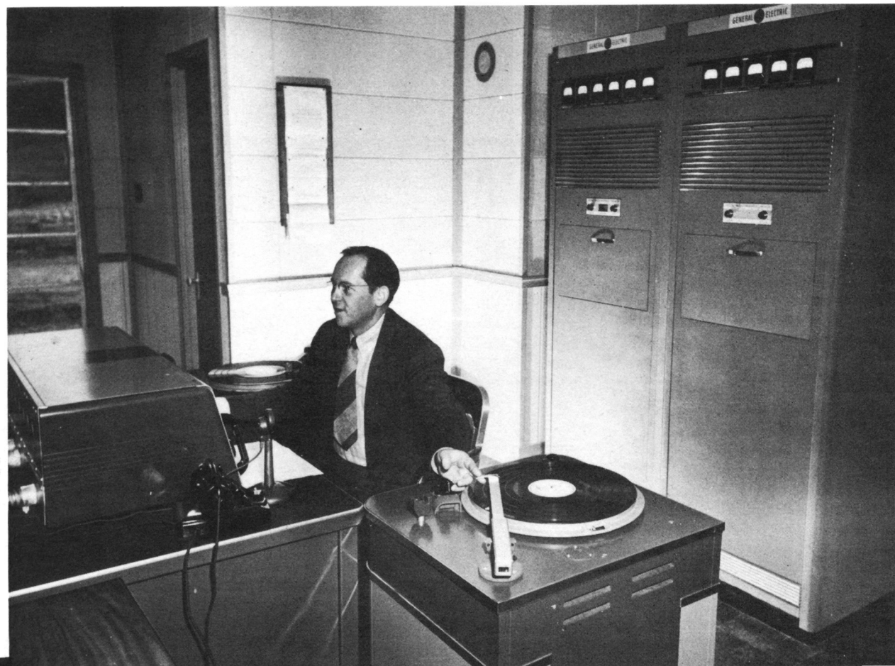
WELLE S. HOAG, W47A CHIEF ENGINEER, WATCHES FOR A SIGNAL FROM THE STUDIO. NOTE THE COMPACT "ARM'S LENGTH" ARRANGEMENT OF CONSOLE AND TURNTABLES
