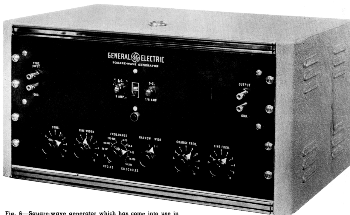
Fig. 6—Square-wave generator which has come into use in testing the waveform reproducing capabilities of an i-m system. Transient wavefront should be reproduced accurately when the full range of audibility is employed
