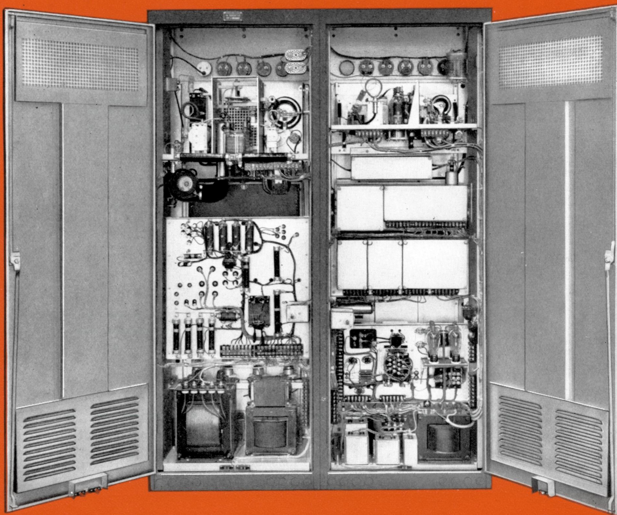
“Vertical chassis construction” makes every tube and soldered joint completely accessible. Removal of the simple shielding is a matter of seconds. There is no need of removing entire units from the transmitter for detailed inspection.
