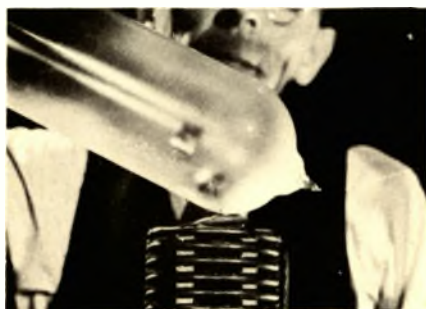
Exploding a pellet of sodium in a sodium-vapor lamp.
