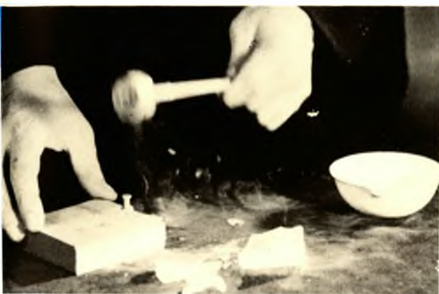
A "quicksilver hammer" made by liquid air.
