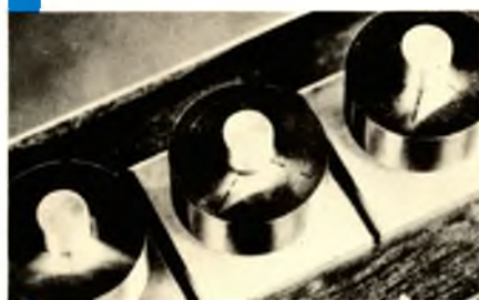
Gears without teeth which work by magnetic force.
