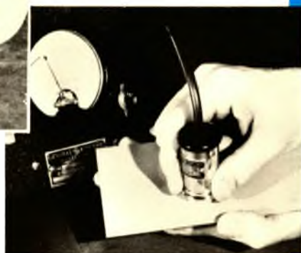
This device will measure the thickness of a coat of paint.
