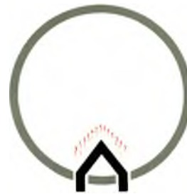
The heater heats the cathode
