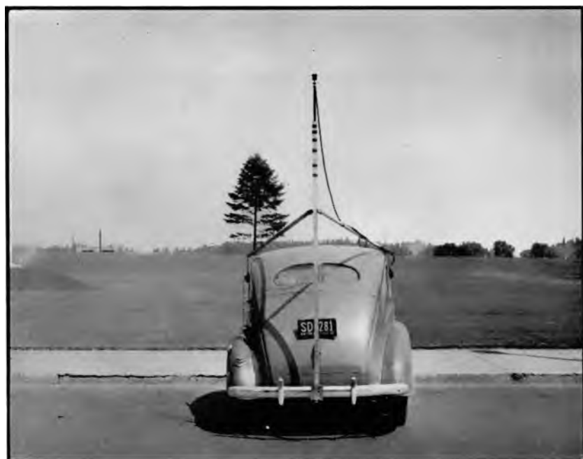
Fig. 2—Automobile equipped with horizontal dipole antenna for field-intensity surveys. This equipment was used in making actual surveys of frequency-modulation station W2XOY
