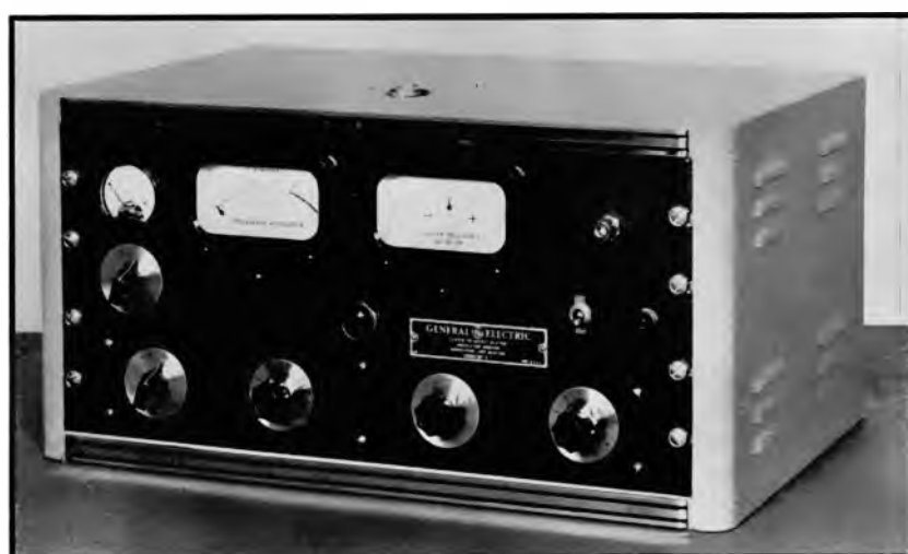
Fig. 1—Monitor for frequency-modulation radio station. This unit measures the center-frequency deviation with or without modulation as well as the percentage modulation. It contains a modulation limiter flasher, high fidelity audio frequency output, and temperature controlled piezoelectric crystal
