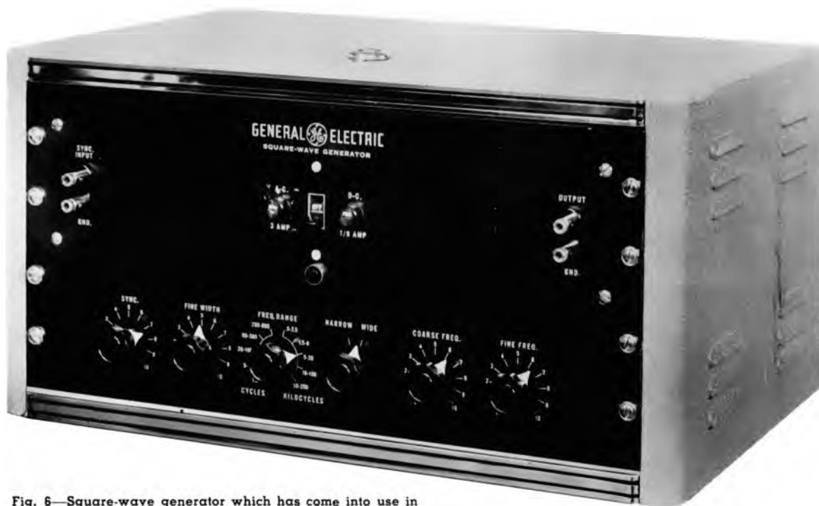
Fig. 6—Square-wave generator which has come into use in testing the waveform reproducing capabilities of an f-m system. Transient wavefront should be reproduced accurately when the full range of audibility is employed
