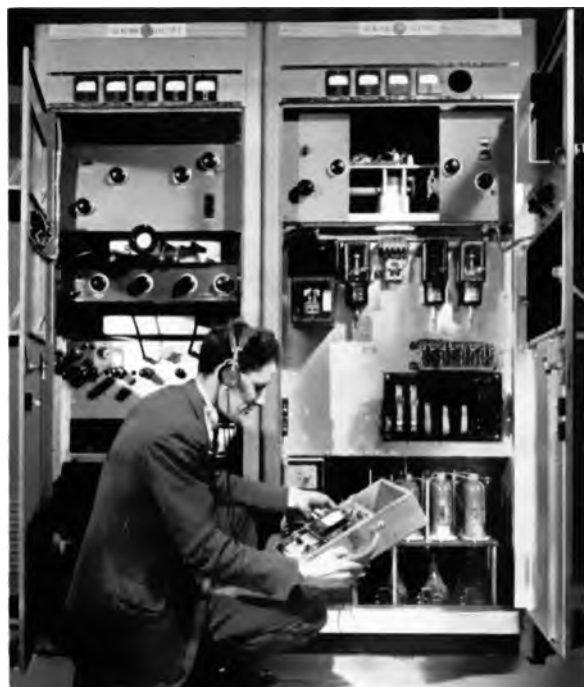
FIG. 8. G.E. 3-KW. FM TRANSMITTER UNDERGOING FINAL TEST RUN BEFORE SHIPMENT
