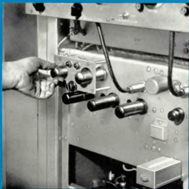
This is the hermetically sealed G-31 Thermocell crystal unit. It utilizes a new method of controlling crystal temperature, which far surpasses older methods in the frequency stability obtained. Although only one Thermocell is used in General Electric's simplified circuit, provision is made for switching to a spare during operation.
