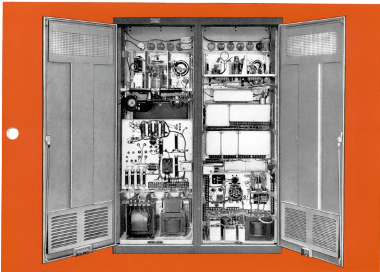
“Vertical chassis construction” makes every tube and soldered joint completely accessible. Removal of the simple shielding is a matter of seconds. There is no need of removing entire units from the transmitter for detailed inspection.
