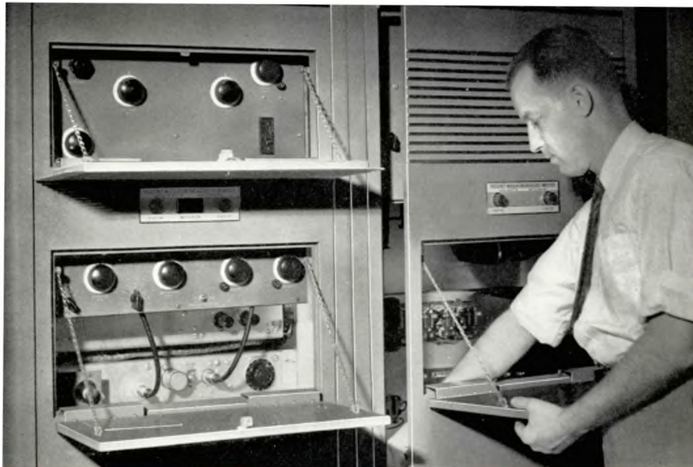
Handles for the front doors are purposely placed on the inside to make it difficult to put the transmitter inadvertently off the air. All tuning controls are within easy reach through the front door panels.
