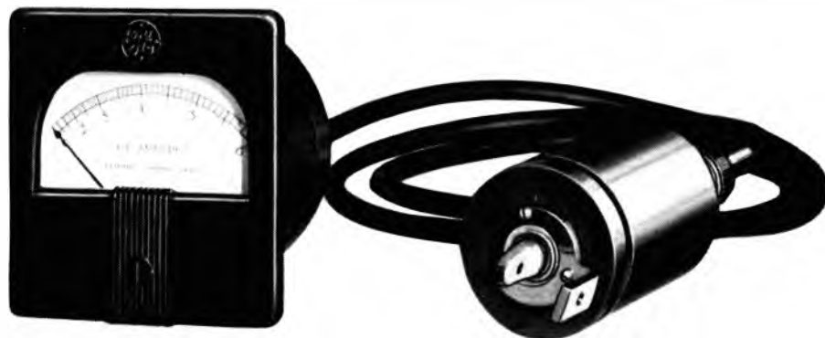
R-f Output Ammeter—a thermocouple-type instrument recently developed by General Electric for direct measurement of transmission-line current.
