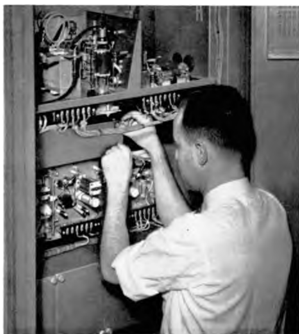
“Vertical chassis construction” makes every tube and soldered joint completely accessible. Removal of the simple shielding is a matter of seconds. There is no need of removing entire units from the transmitter for detailed inspection.
