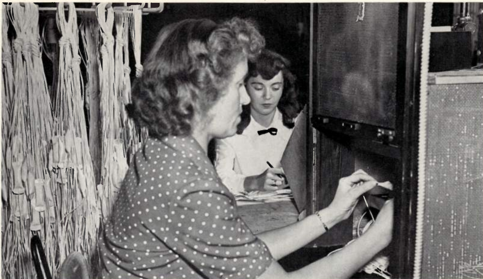
Using an electronic sealing machine, these Bridgeport Works employees seal up the outside coverings of thermostats. Eight of the nine thermostats in a G-E electric blanket are safety devices.
