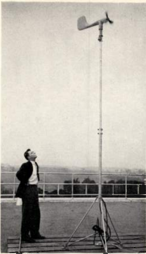
Ray Falconer inspects the aerovane, an instrument used in the Laboratory's famous weather research.
