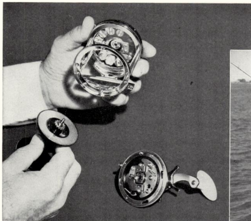
Alnico magnets in the reel (left hand) and a copper disk in the spool (right hand) are the working parts of the magnetically braked reel. The ends are made of G-E plastics.
