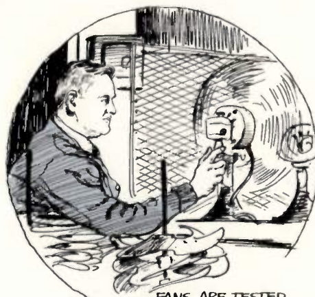
FANS ARE TESTED CAREFULLY FOR VIBRATION AND BALANCE BEFORE THEY LEAVE THE FACTORY
