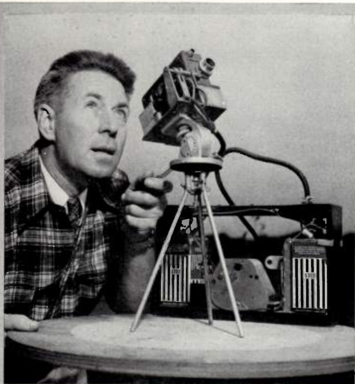
Dr. Vincent J. Schaefer of the Research Laboratory records the movements of clouds with this unusual camera system. A small hand movie camera is rigged to take a single movie frame every two seconds, so that 32 minutes of actual time turn up as one minute of movie screen time. The completed movies resemble an animated cartoon, as the clouds rise and fall, expand and contract at an increased tempo. Schaefer is one of the Laboratory's pioneers in the field of weather research.
