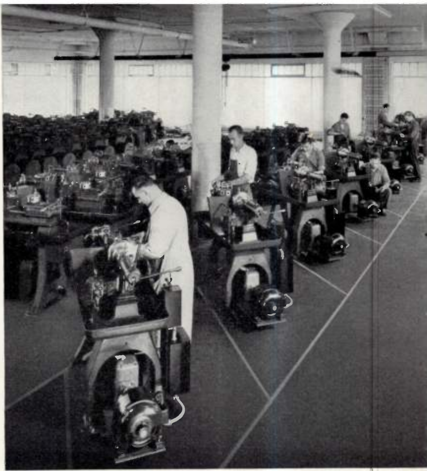
Separate electric motors on each machine eventually eliminated inefficient, ugly, and hazardous belt systems, and made way for a new era in factory design.
