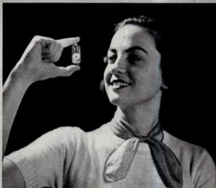
Winona Brown of the Electronics Department shows off a new tube developed by General Electric engineers for use in ultra-high-frequency television receivers. The tube is a tiny "magnetron," which is similar in principle to tubes used in radar and in quick-cooking electronic ovens. The television application marks the first consumer use of a magnetron, a tube type first devised by Research Laboratory scientists and used principally in industrial and military equipment.
