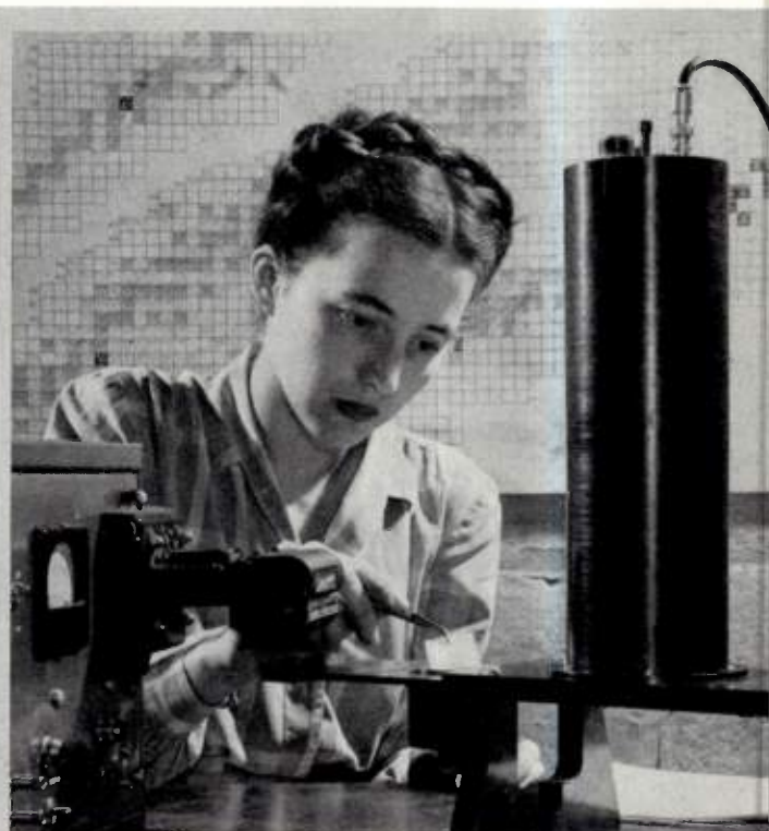
A white square of paper, containing a smear from an object suspected of being contaminated with radiation, is analyzed by a new General Electric radiation detector known as the "universal scintillation counter." The instrument is able to check the smear for the presence of alpha, beta, or gamma rays, the "big three" of nuclear radiation. Operating the instrument is Mrs. Ethelyn Langdon, an assistant in the General Engineering and Consulting Laboratory in Schenectady.
