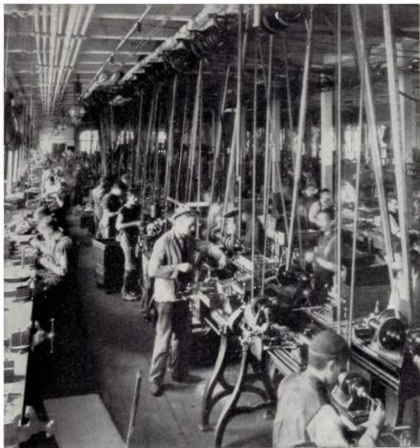
The drive power of steam engines used to be carried about plants on shafts and belts. At first, electric motors were used simply to drive these same systems.
