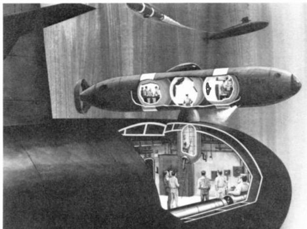
RESCUE VEHICLE: This small submarine vehicle is being developed by the Deep Submergence Systems Project to help give the Navy a 24-hour response time to any submarine distress call. Up to 24 survivors can be shuttled from sunken submarines per trip.
