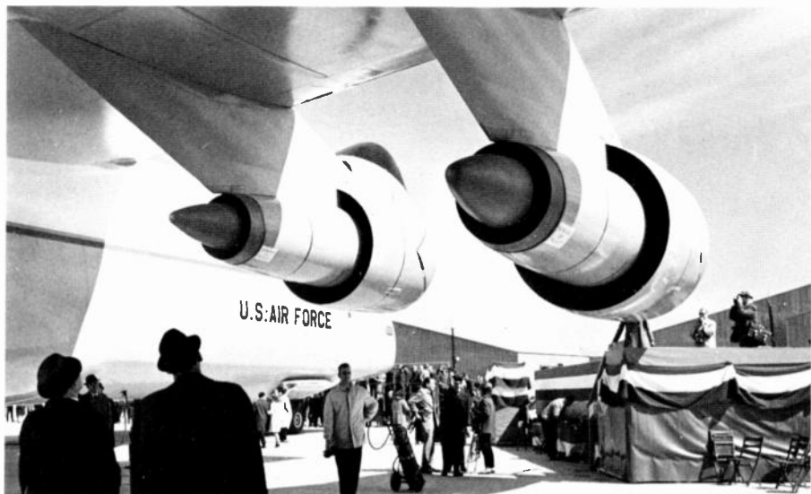
CLOSE-UP VIEW OF THE POWERFUL GE TF39 ENGINES ON THE C-5 GALAXY.
