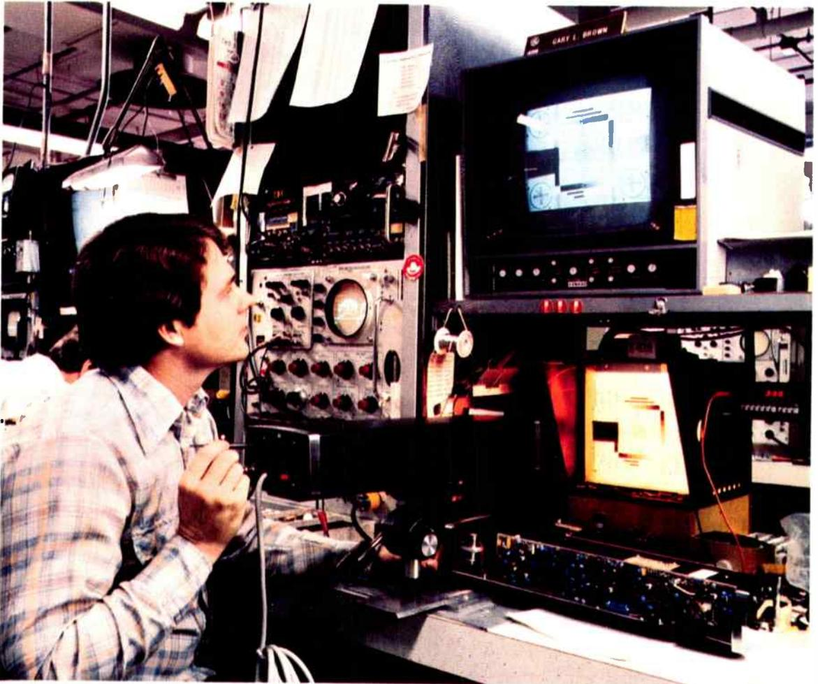
**NIGHT WATCH.** The Nite Gard<sup>®</sup> closed circuit TV camera being quality-tested above is so sensitive that starlight provides all the illumination it needs for security work.
