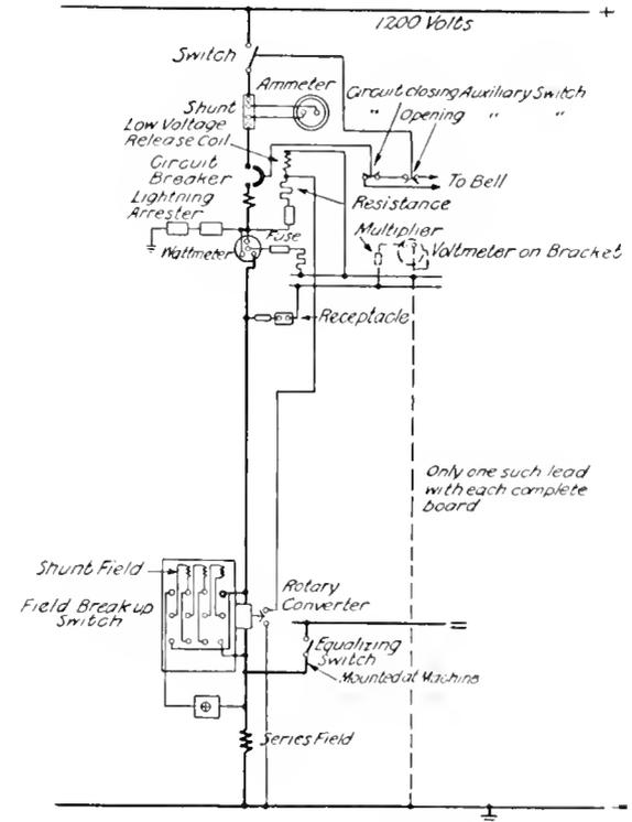
Fig. 4. Switchboard for 1200 Volt Railway Service, Rotary Converter Panel
