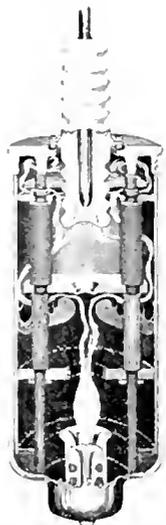
Fig. 2. Section of Switch Showing Baffle Plates
