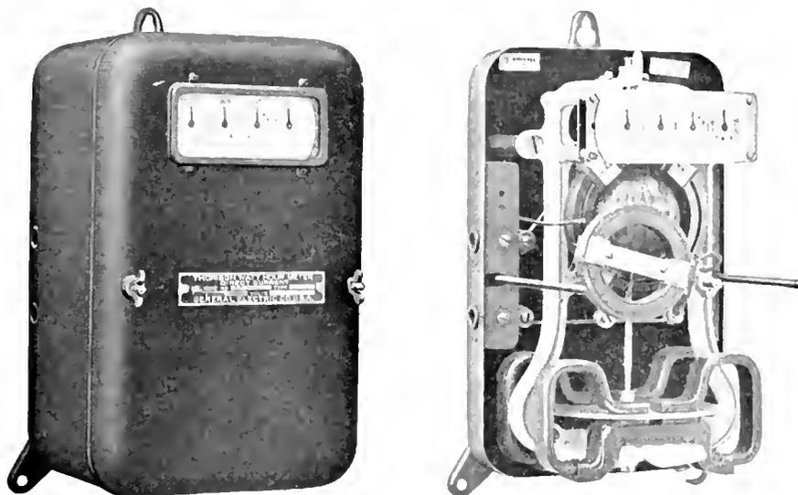
Direct Current Commutator Watt-hour Meter
