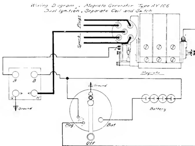
Fig. 5. Wiring Diagram for Dual Ignition, New Magneto
