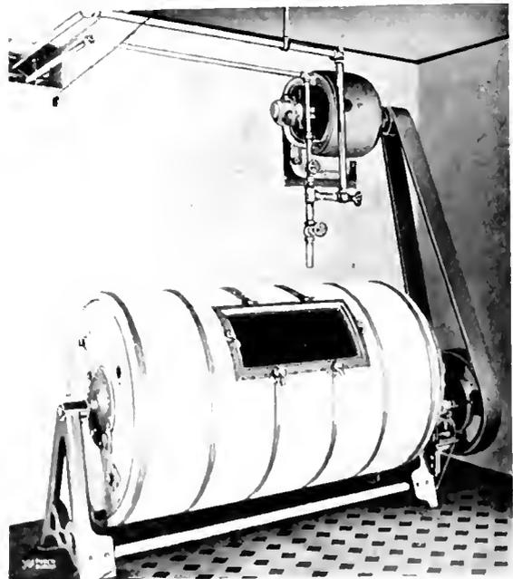
Fig. 8. Fargo Barrel Churn Operated by Belt-Connected Motor
