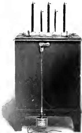
Fig. 5. Tube Tank Equipped with Shaking Magnet
