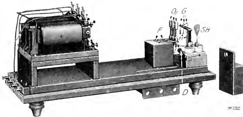
Fig. 3 Oscillograph Removed from Case, Showing Various Parts of Optical System and Galvanometer
