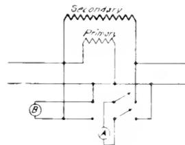
Fig. 66. Connections for Boost and Lower on Regulator
