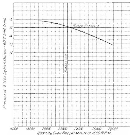
Fig. 7. Factory Test, showing Pressure Plotted Against Quantity of Air, 1650 R.P.M.
