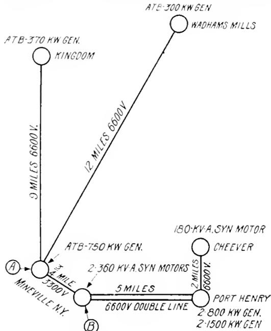
Fig. 5. Diagram showing relative location of Generators and Synchronous Motors
