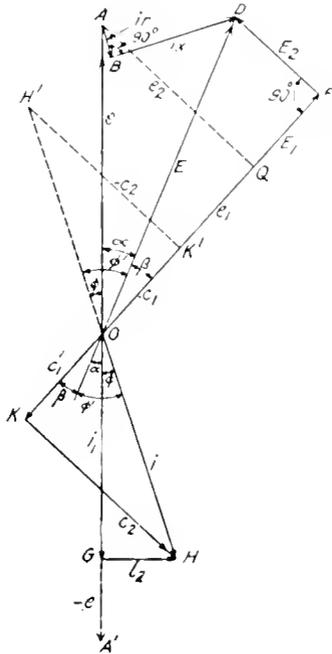
Fig. 6. Vector Diagram of Loaded Synchronous Motor
