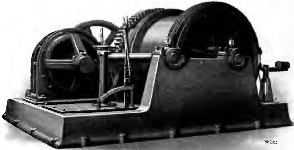
175 H.P. Induction Motor Driving 225 H.P. Band Friction Hoist, with Double Band Brakes, The Mexican Coal and Coke Company, Las Esperanzas, Coah, Mex.
