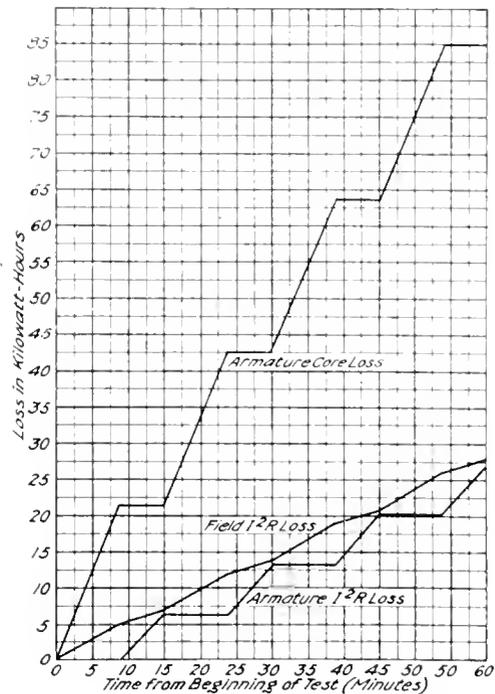
Fig 1. Calculated Loss Curves for Alternator (First Example)
