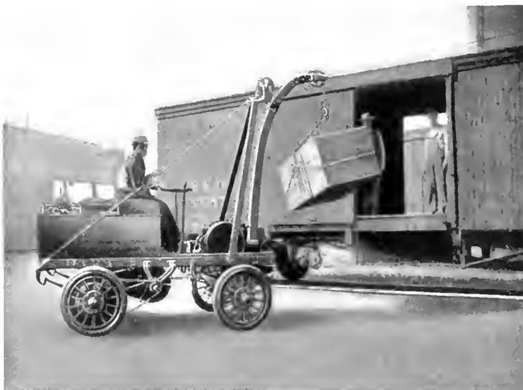
Battery Truck Crane Loading Freight Car
