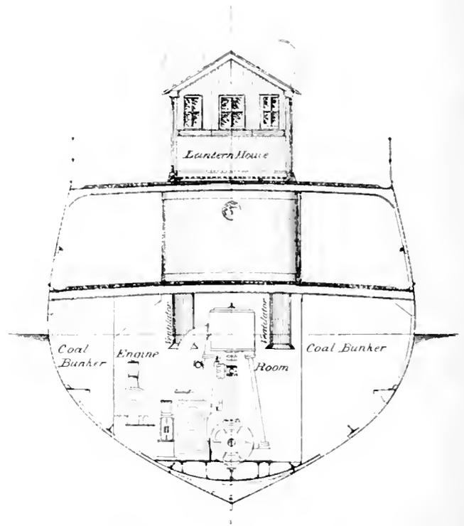
Fig. 4a Section Through Engine Room
