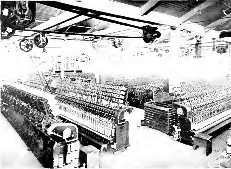
Fig 8 Roving and Twisting Frames
