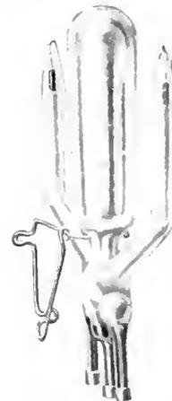
Fig. 9. Bracket for Holding Tubes While in Storage
