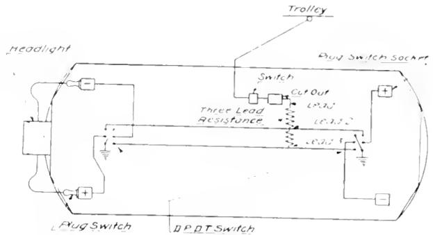
Fig. 13. Connections for Luminous Arc Headlight for Normal Operation, and for Operation with Reversed Polarity for Subdued Illumination.
