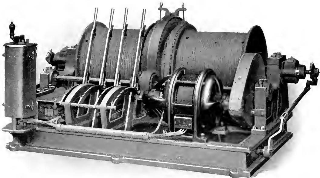
Double Friction Drum Electric Mining Hoist, with 3-Phase Induction Motor
