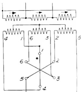
Fig. 72. Connections for Six-phase Boost and Lower
