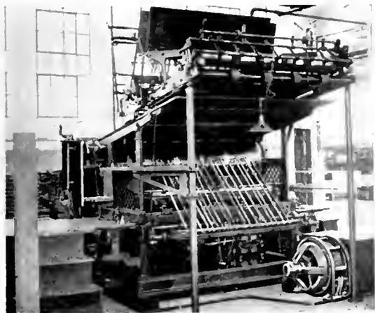
Fig. 2. No. 9 Hoe Press Driven by 7 1-2 H.P. Motor
