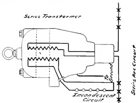
Fig. 1. Diagram of Connections of Series Lighting Transformer
