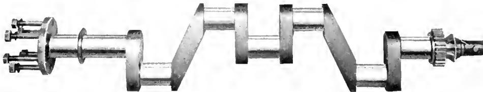
Fig. 2. Three-Bearing Crank Shaft
