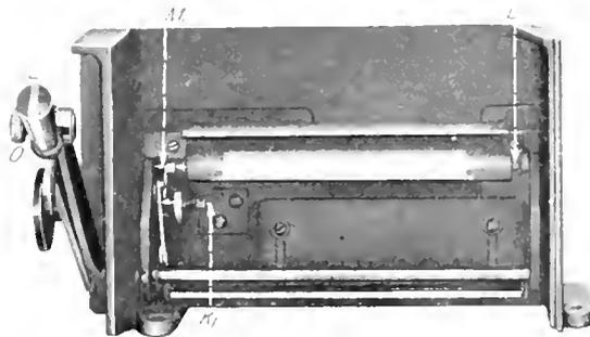
Fig. 6. Cylindrical Lenses, Cam and Cam Shaft
