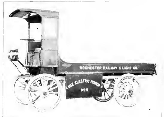
Figs. 4 and 5. 2000 Lb. Electrically Propelled Trucks
