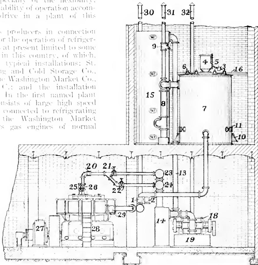
Fig. 1. Elevation, Showing Gas Producer Arrangement of Piping, and 150 Kw. Gas Engine Generating Set
