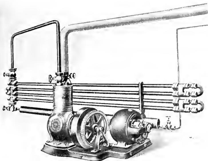
Fig. 9. Motor Direct Geared to Larsen Ice Machine
