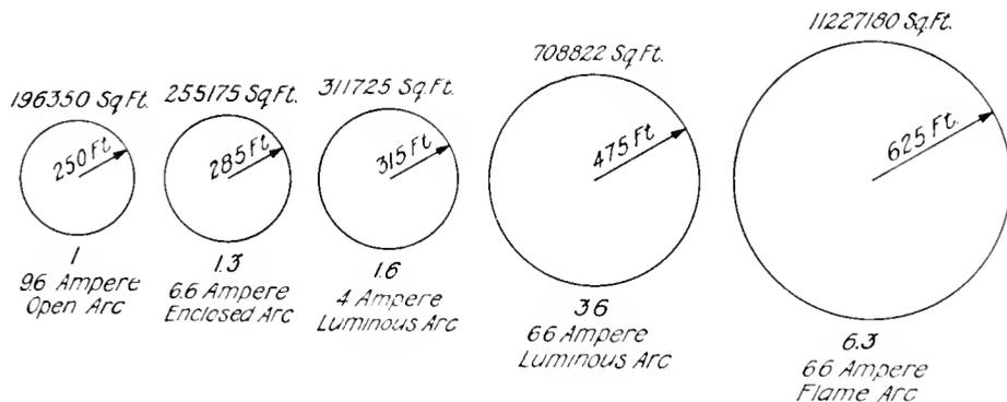
Fig. 8. Areas Lighted for Equal Minimum Illumination. Basis: Open Arc at 250 ft.
