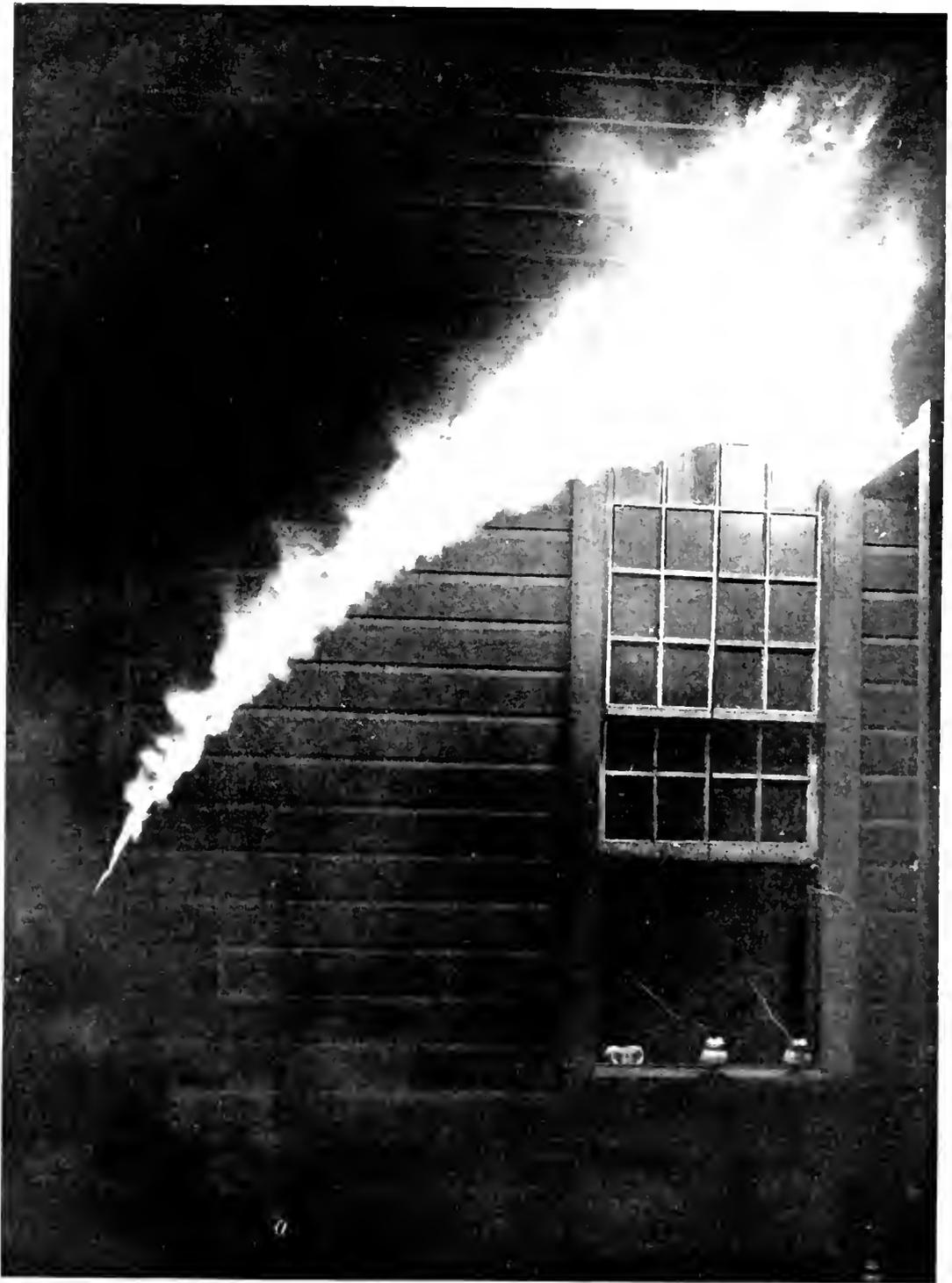
Arc Drawn by Air-Break Disconnecting Switch in Rupturing a Current
