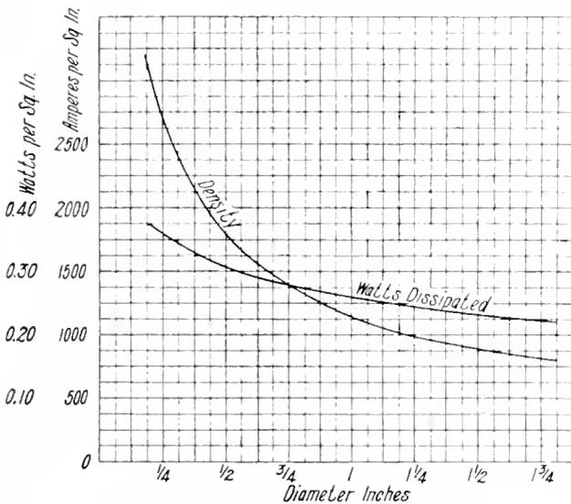
Fig. 1. Watt Dissipation and Corresponding Current Density at 30° C. Rise for Cylindrical Copper Conductors of Various Diameters
