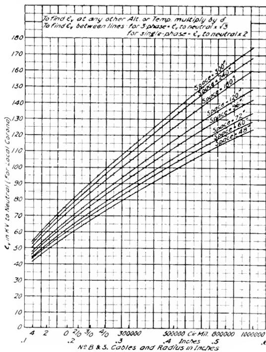
Fig. 16. Visual Critical Voltage to Neutral ( $m = .72$ )
