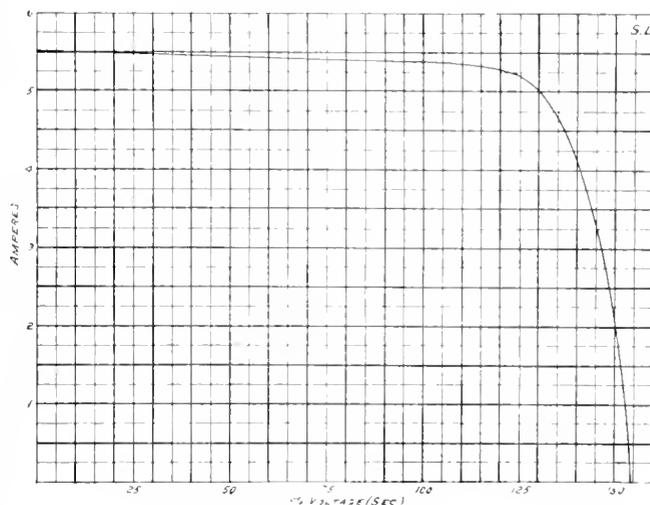
Fig. 2. Characteristic Regulation Curve, obtained from  $\frac{1}{2}$  kv-a. 5.5 Ampere Series Lighting Transformer
