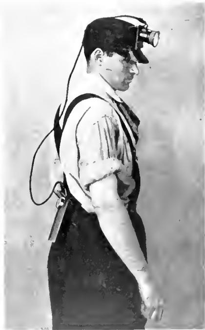
Miniature Tungsten Headlight Driving Current from Portable Storage Battery
