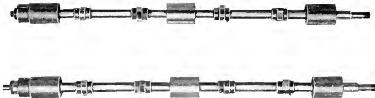
Fig. 3. Two Built Up Cam Shafts
