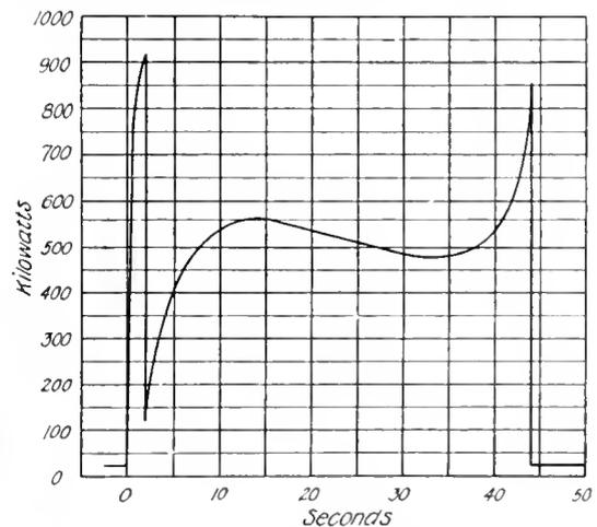
Fig. 1. Curve Showing Power Demand for One Hoisting Cycle
