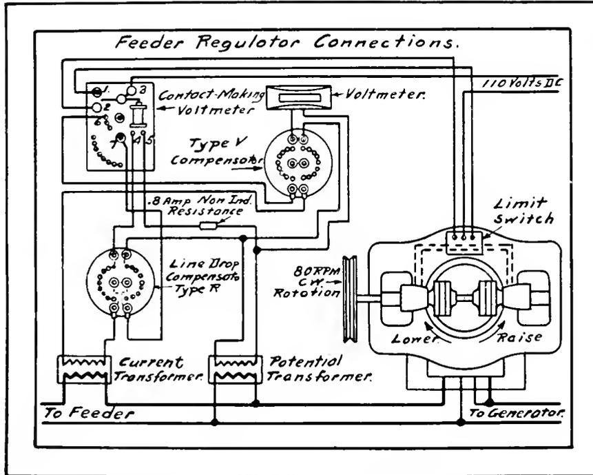
Fig. 74. Connections for BR Regulator
