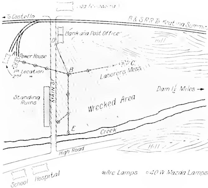
Fig. 1. Wrecked Area Showing Location of Power House
