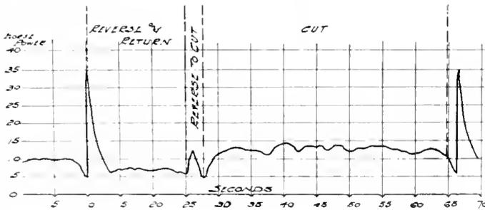
Fig. 5. Graphical Record of Bement Niles 120" Planer taking two cuts 1.2" by 151" with  $\frac{1}{8}$ " feed on Cast Iron, cutting speed 22 ft. per minute.
