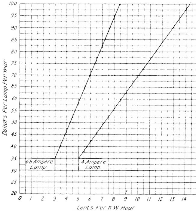
Cost per kilowatt-hour corresponding to various flat rates in dollars per lamp per year. Figures based on luminous lamps operated from series luminous rectifier system, with lamps in service from dusk until 12 p.m. daily
