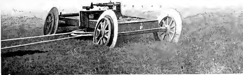
Fig. 13. Anchor Carriage for Electric Plow
