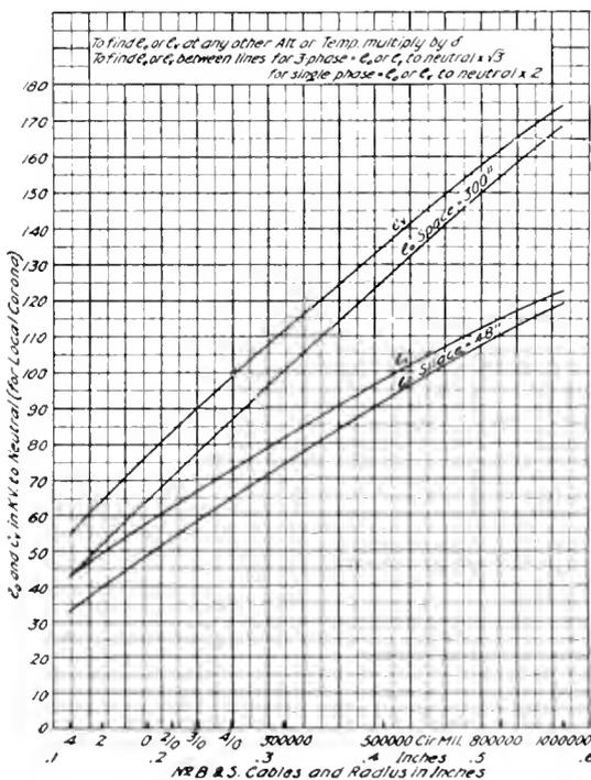
Fig. 18. Comparison of Disruptive and Visual Critical Voltages to Neutral
