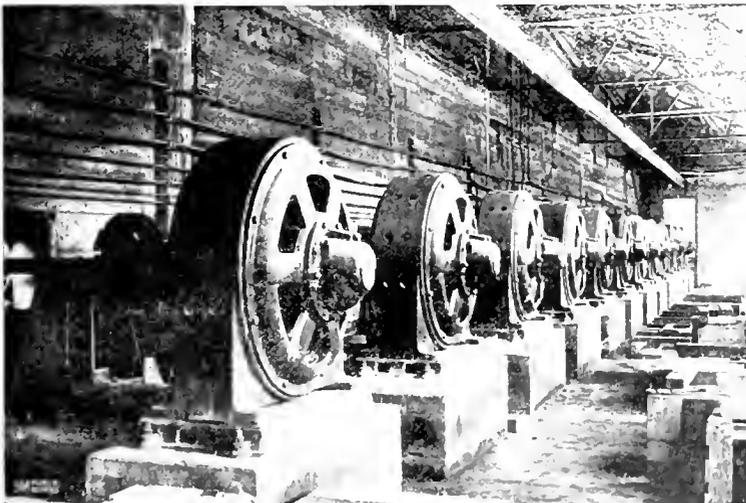
Twelve 18 h.p., 166 $\frac{2}{3}$  r.p.m. motors driving raw material tube mills in Universal Portland Cement Co., Plant No. 4. These motors are connected through flexible couplings to the countershafts of the mills. This arrangement necessitated only one gear reduction. The concrete wall separating the motors from the mills secures an unusually clean motor room
