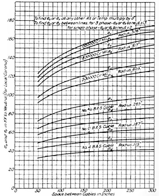
Fig. 14. Comparison of Disruptive and Visual Critical Voltages to Neutral ( $m = .72$ )
