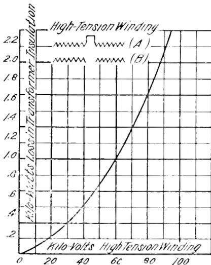
Fig. 3. Variation of Loss in Transformer Insulation due to Stress, WC-60 3750-60000/120000 138000 V 12000
