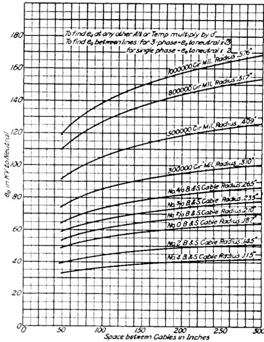
Fig. 11. Disruptive Critical Voltage to Neutral
