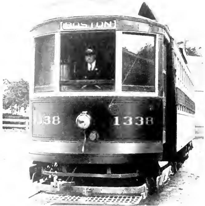
Fig. 7. Two-Ampere Headlight Permanently Attached to Front of Car
