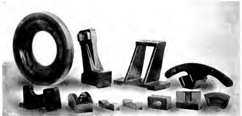
Patterns and Core Boxes for Commutator Turning Tools and Armature Flange, Made by Patternmaker Apprentices Six Months on Course. Training Room, Schenectady Works
