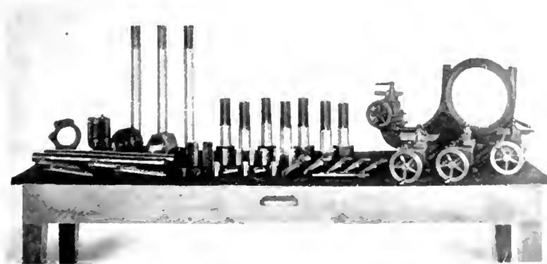
Axle Collar, Cable Guides, Bolts, Commutator Turning Tools, Worms, Milling Cutters, Counter Boxes, Motor Shaft. Made by Apprentices Three to Nine Months on Course. Training Room, Schenectady Works
