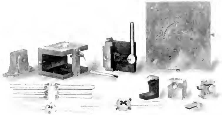
Drilling Jigs Designed and Made by First Year Apprentices. Die Holders Made by Four Months Apprentice. Training Room, Schenectady Works
