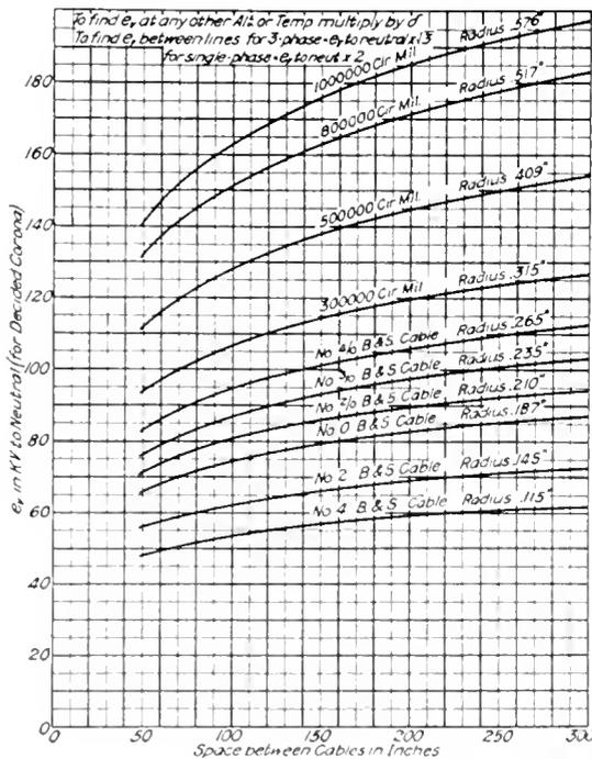
Fig. 13. Visual Critical Voltage to Neutral ( $m = .82$ )
