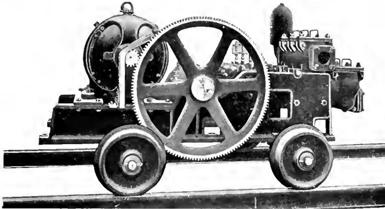
7 1/2 H.P. 925 R.P.M. CQ Motor Driving Portable Mine Pump
