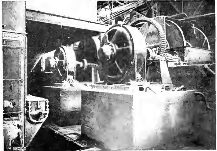
18 h.p., 166 $\frac{2}{3}$  r.p.m. motors driving ball mills in the raw material mill. Universal Portland Cement Co., Plant No. 4. There are nine of these mills, and very satisfactory results have been obtained by this type of slow speed drive, which eliminates one gear reduction
