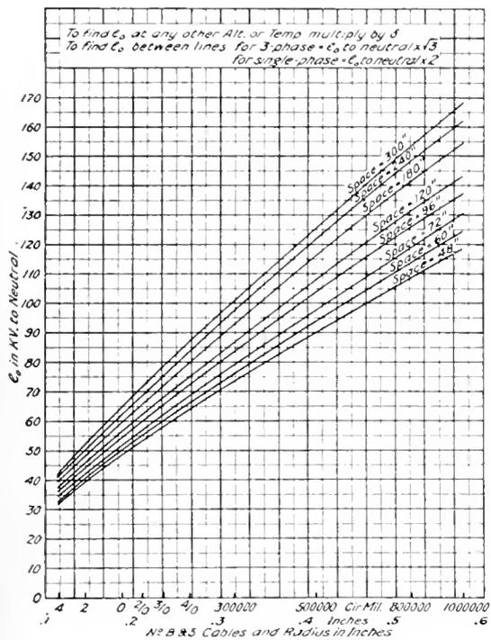
Fig. 15. Disruptive Critical Voltage to Neutral
