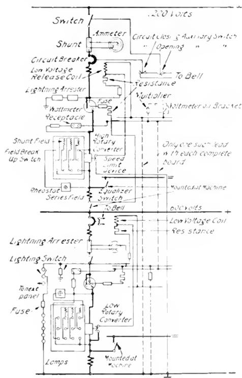
Fig. 9. Switchboard for 1200-600 Volt Railway Service. Generator Panel
