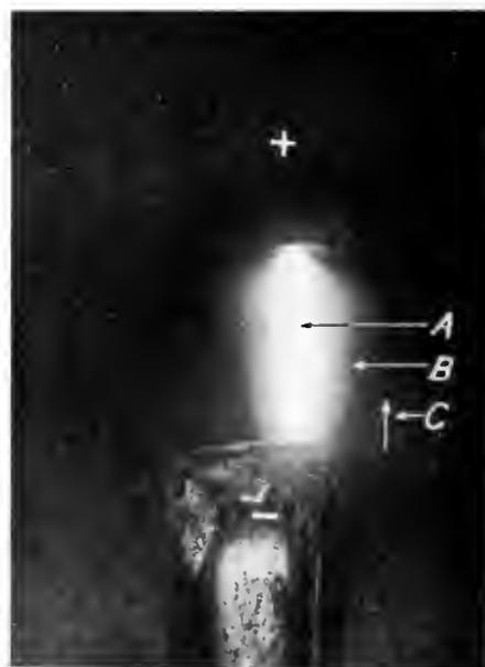
Fig. 2. Normal Arc of the Luminous Lamp
