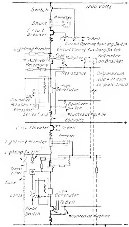
Fig. 8. Switchboard for 1200-600 Volt Railway Service, Generator Panel
