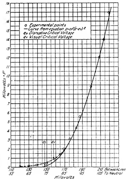
Fig. 9 Corona Loss for Large Conductor
