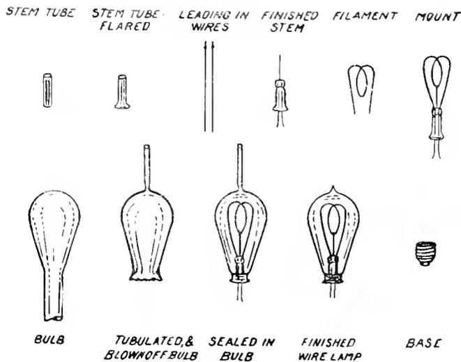
Parts of Lamp During Manufacture
