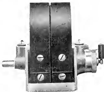
Fig. 7. Low Tension Alternating Current Magneto
