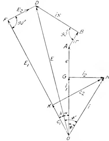
Fig. 2. Vector Diagram of Voltages in an Alternator
