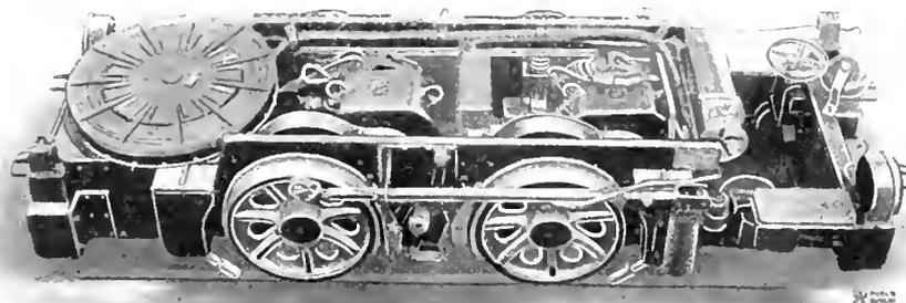
Internal Arrangement of Seven-Ton Gathering Locomotive Designed for Low Vein Work
