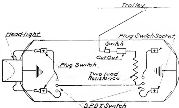
Fig. 12. Connections for Luminous Arc Headlight with Two-Lead Resistance and Incandescent Lamps for Dimming Purposes
