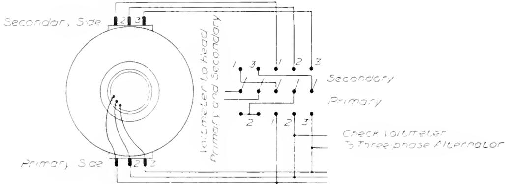
Fig. 69. Connections for Boost and Lower—Three-phase Regulator
