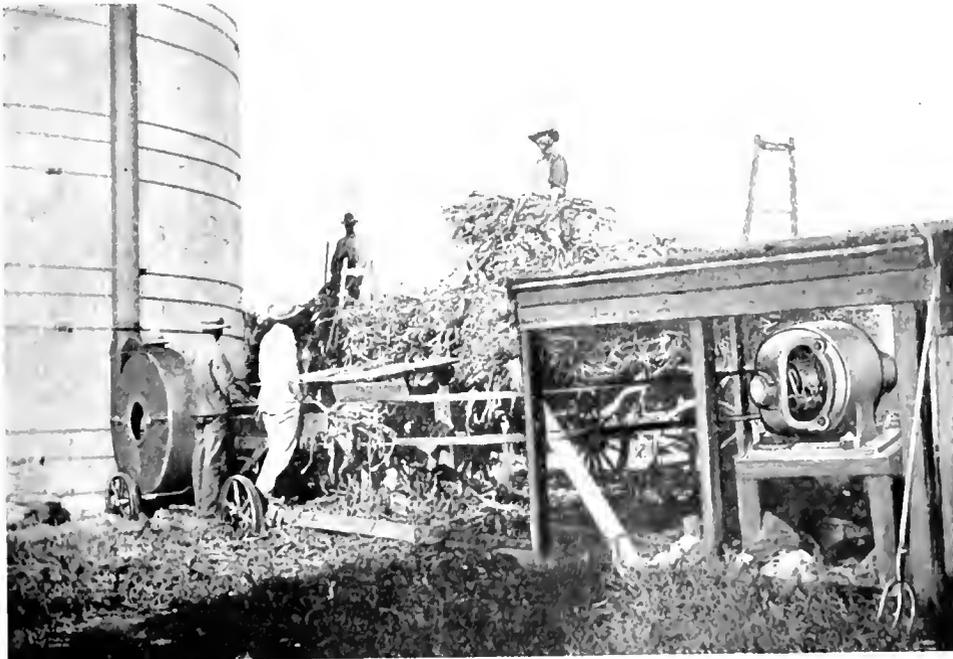
Fig. 2. Motor Driving No. 19 "Ohio" Self Feeding Blower Ensilage Cutter
