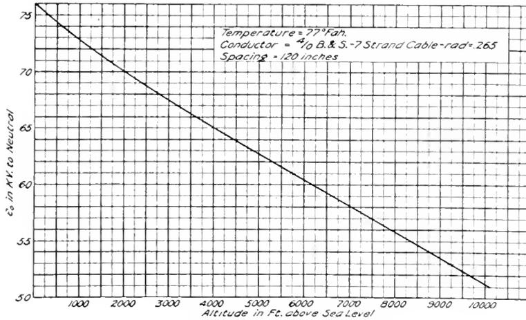
Fig. 19. Disruptive Voltage at Various Altitudes for 4 0 Cable
