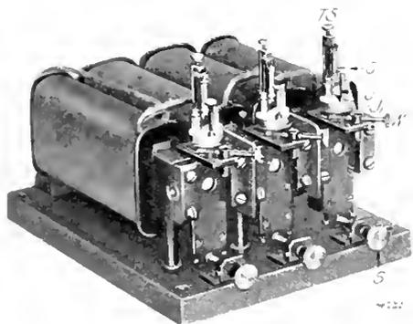
Fig. 5. Three Element Galvanometer
