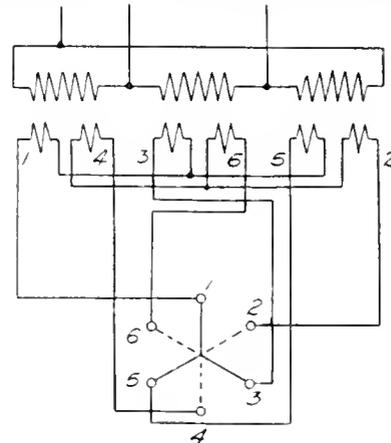
Fig. 71. Method of Connecting for Six-phase Voltage
