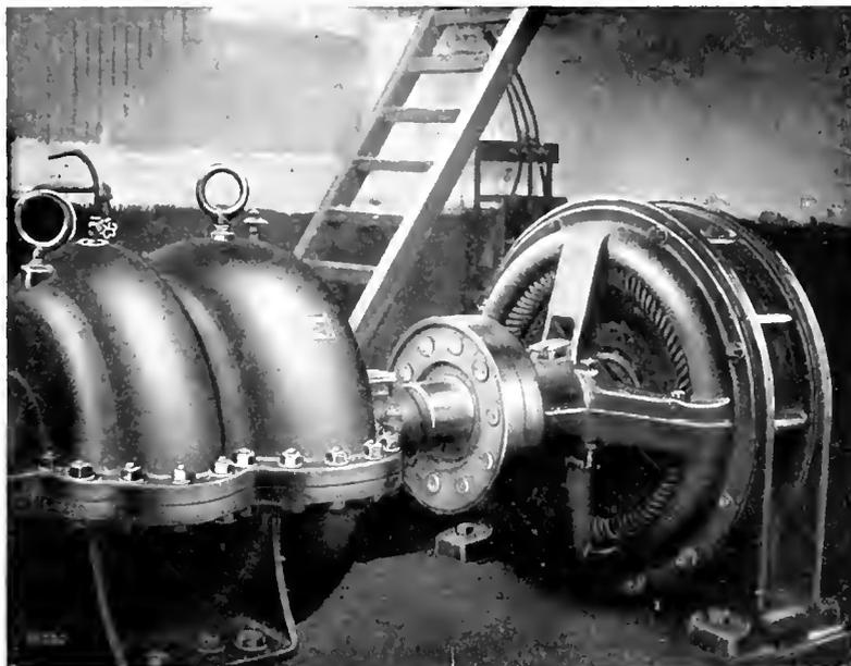
Type 1 Form K 150 H.P. Induction Motor Driving Centrifugal Pump
