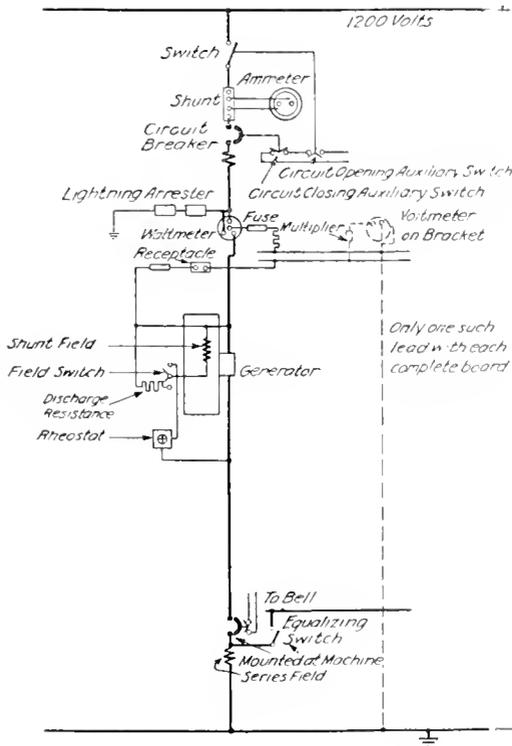
Fig. 3. Switchboard for 1200 Volt Railway Service, Generator Panel
