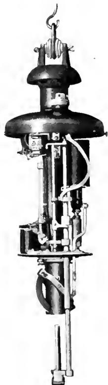
Fig. 1. Early Type of Luminous Arc Lamp
