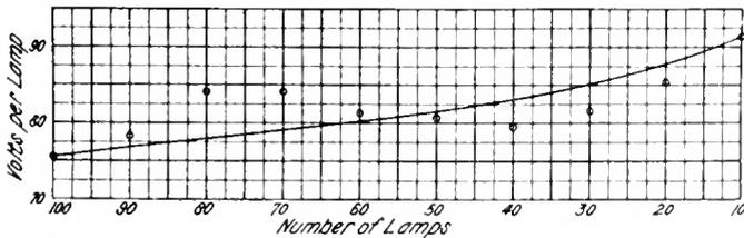
Fig. 7. Increase in Voltage Across Lamp with Decrease in Number of Lamps; 100 Lamp Transformers
