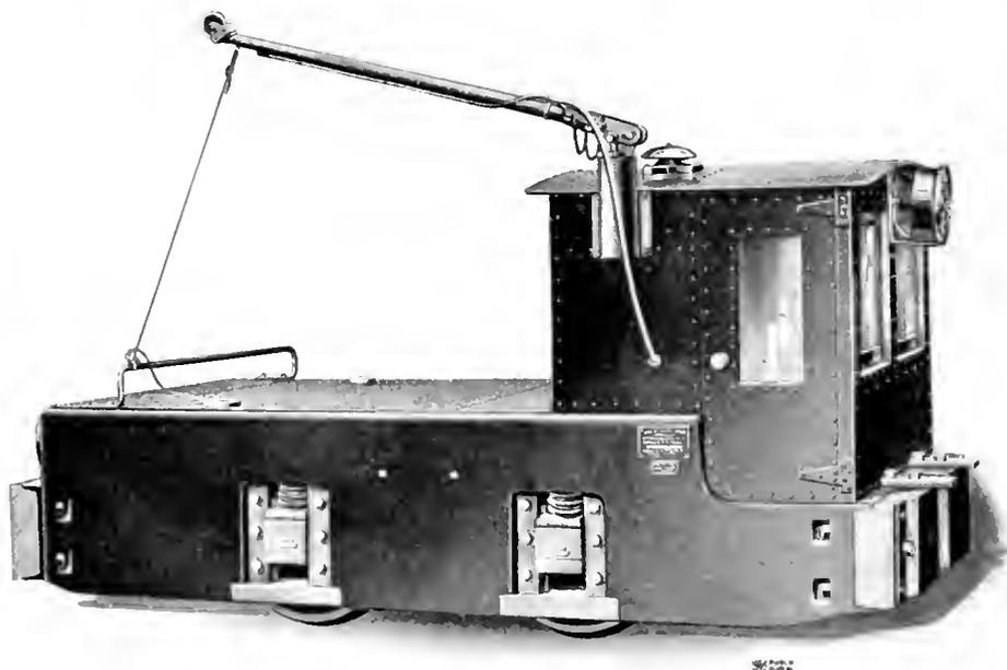
Mine Locomotive Equipped with Cab
