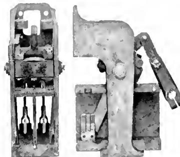
Fig. 1. Early Type of Oil-Break Circuit Breaker Consisting of a Knife Blade Switch Immersed in a Can of Insulating Oil
