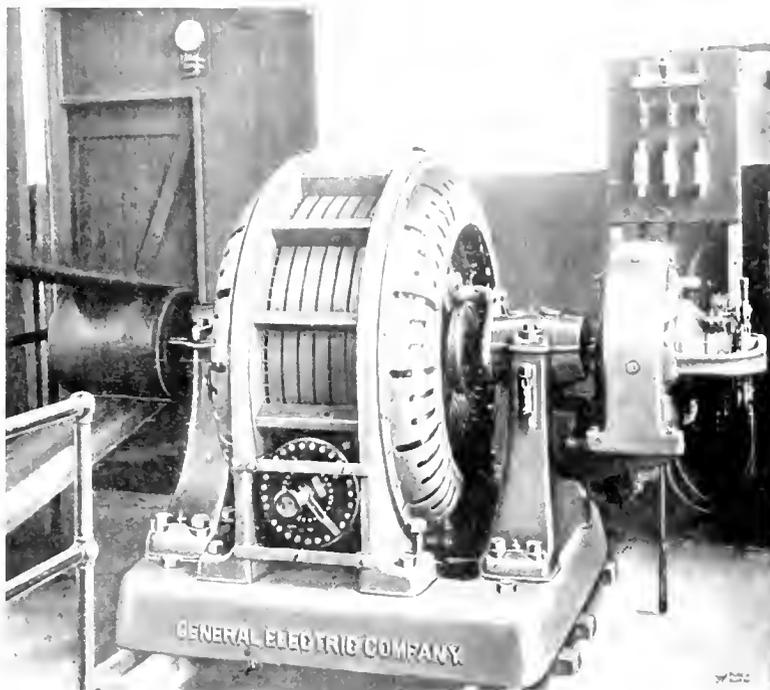
Fig. 4. 300 kv-a., 230 volt, 720 r.p.m. Synchronous Motor driving Air Compressor Chalmers Motor Company, Detroit, Mich.
