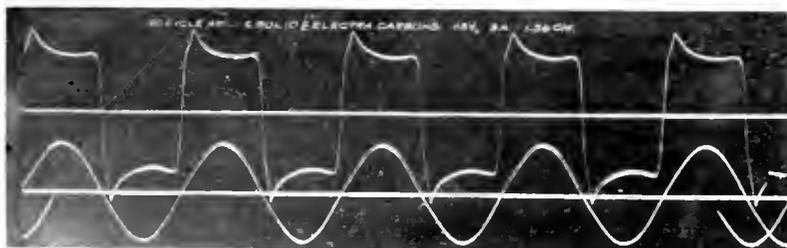
Fig. 10. Upper Curve, Current; Lower Curve, Voltage
