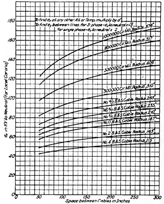
Fig. 12. Visual Critical Voltage to Neutral ( $m = .72$ )
