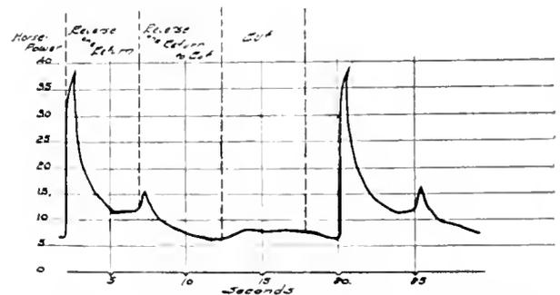
Fig 4 Graphical Record of Detrick & Harvey Open Side Planer taking one cut  $\frac{1}{8}$ " by 36" with  $\frac{1}{16}$ " feed on Steel, cutting speed 35 ft. per minute. Maximum Power = 39 h.p. Average Power = 10.9 h.p. Mean Power = 12.4 h.p.
