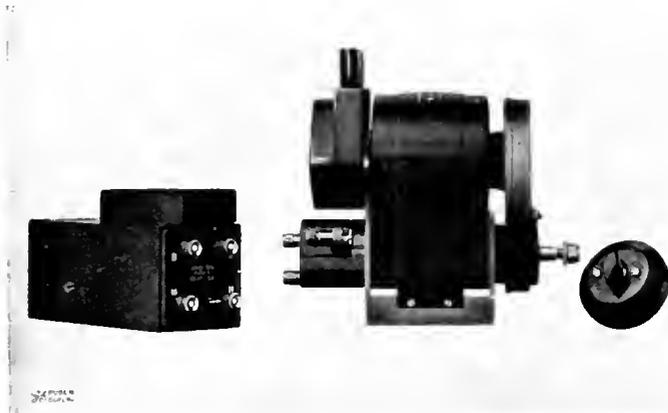
Fig. 1. First High Tension Magneto Developed by General Electric Company
