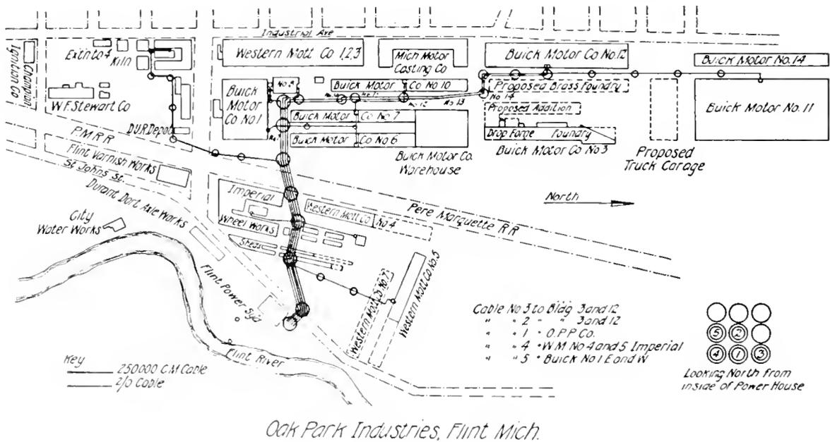
Fig. 1. Arrangement of Buildings and Underground Conduit System
