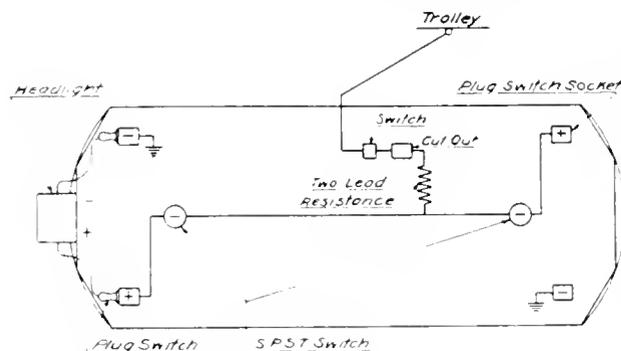
Fig. 10. Connections of Luminous Arc Headlight with Two-Lead Resistance for Street Railway Service
