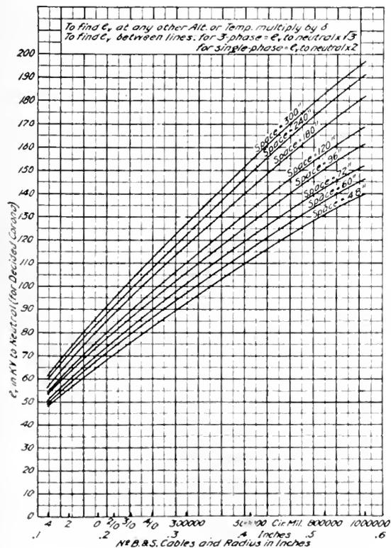
Fig. 17. Visual Critical Voltage to Neutral ( $m = .82$ )
