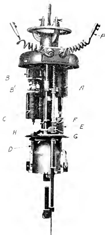
Fig. 8. Later Type of Luminous Arc Lamp
