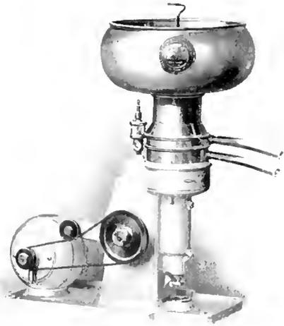
Fig. 6. Motor-Operated DeLaval No. 4 Separator
