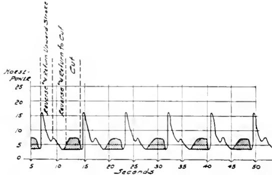
Fig. 3. Graphical Record of 48" Vertical Newton Slotter taking one cut  $\frac{1}{8}$ " by  $\frac{1}{16}$ " feed on Cast Iron, cutting 21.4 ft. per minute. Diagram is made from two curves superimposed. Maximum Power equals 16 h.p. Average Power equals 6.7 h.p. Shaded Portion shows useful work done in removing metal
