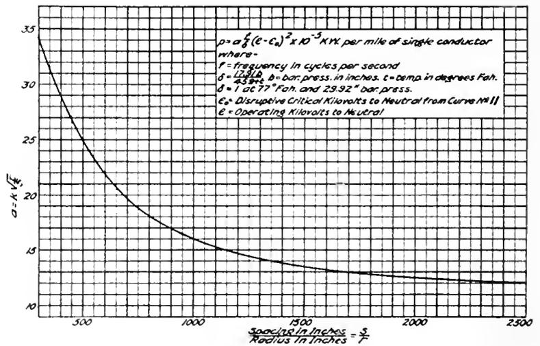
Fig. 20. Curve for Calculating Corona Loss
