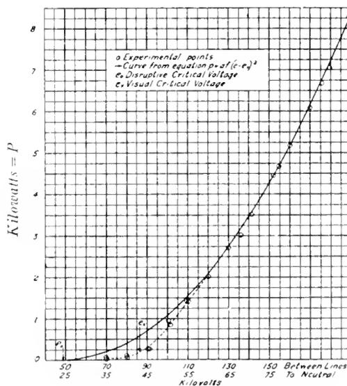
Fig. 10 Corona Loss for Small Conductor
