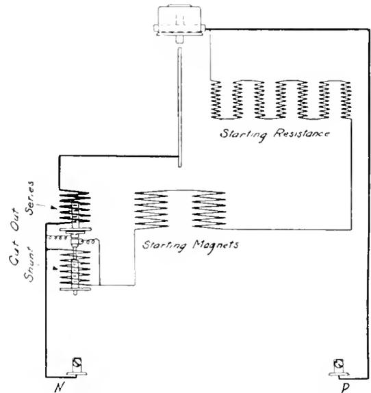
Fig. 24. Connections for Series Luminous Arc Lamp, Inverted Type
