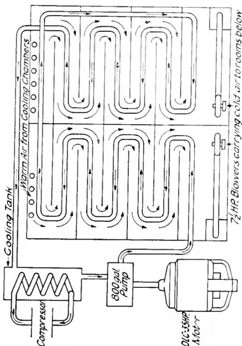
Fig. 6. General Arrangement of Pipin<sub>g</sub> for Circulating Brine
