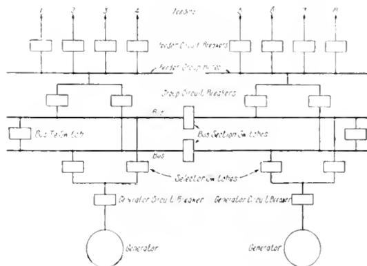
Fig. 5. Diagram Showing Possible Locations of Oil-Break Switches and Circuit Breakers in the Distributing System of the Modern Power Station
