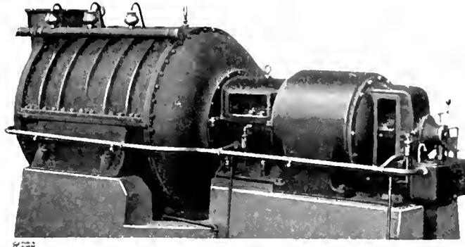
Motor Driven Multi-Stage Centrifugal Air Compressor
