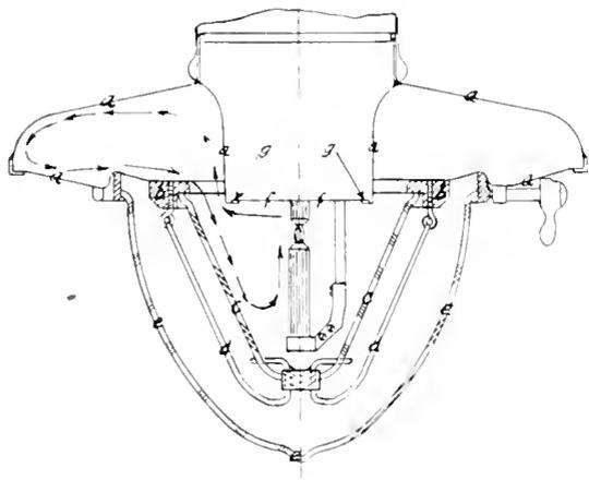
Fig. 1. Sectional View of Long Life Flame Arc Lamp, Showing Method of Ventilation
