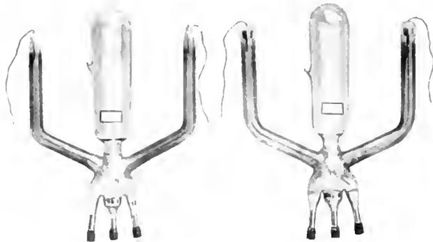
Fig. 6. Tube with Lava Bushing Anode on Left. Tube with Iron Over Graphite Anode on Right
