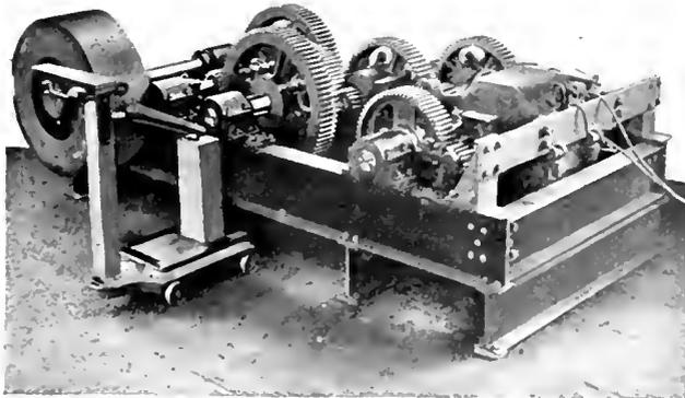
Fig. 4. Gear Breaking Machine
