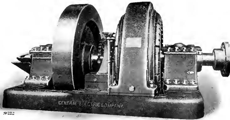
Fig. 7. 500 H.P., 214 R.P.M. Induction Motor with 30,000 Lb. Cast Iron Flywheel. Flywheel Effect, Including Rotor, 470,000 Lb. at One Foot Radius
