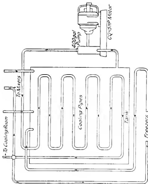
for circulating the brine. The 800 gallon pump takes the brine from the cooling tank and forces it through the coils in the large chill room on the second floor, while the 400 gallon pump supplies brine to the mixers, freezers and the third floor chill room. Fig. 8 shows the method of driving the brine-cooled freezers, which are each provided with a clutch on the main shaft for individual control, the whole group being driven by a 20 h.p. motor.
