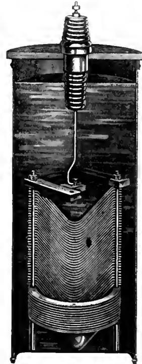
Fig. 4. Aluminum Cell Lightning Arrester
