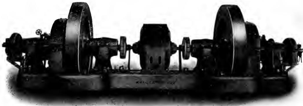
Double Flywheel Motor-Generator Set Consisting of Two 170 Kw. Shunt Wound Generators Driven by a 450 H.P. 2080 Volt Induction Motor—Speed of Set 600 R.P.M.
