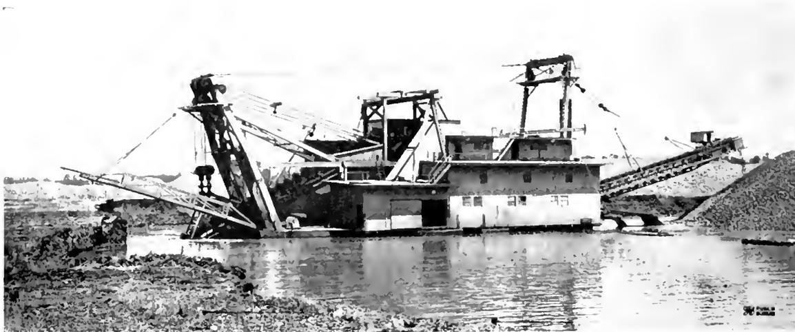
Gold Dredge—Capacity 7½ cu. ft.—Electrical Equipment: Three 125 Kw. 60 Cycle 4000 460 Volt Three-Phase Transformers, One 7½ Kw. 4000 -115 230 Volt Transformers, Switchboard and the Following 440 Volt Induction Motors: Bucket 200 H.P., Winch 25 H.P., Screen 35 H.P., Stacker 25 H.P., 10 In. High Pressure Pump 75 H.P., 10 In. Low Pressure Pump 35 H.P. and 4 In. Priming Pump 10 H.P.
