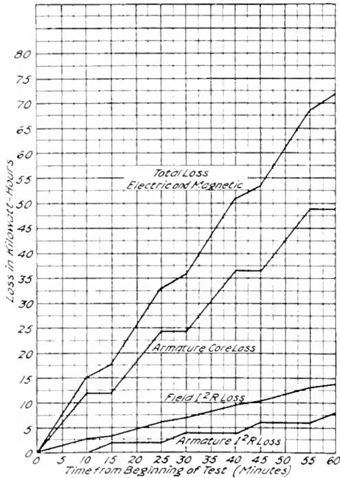
Fig. 2. Calculated Loss Curves Alternator (Second Example)
