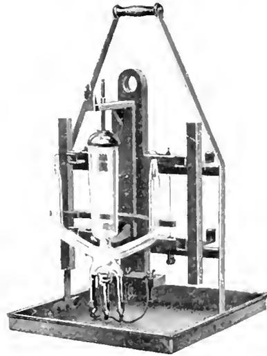
Fig. 8. Rack and Drip Pan for Handling Tubes
