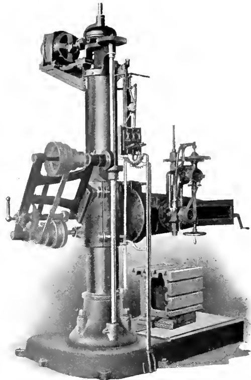
Fig. 4. Induction Motor driving 4 1-2 ft. Universal Radial Drill
