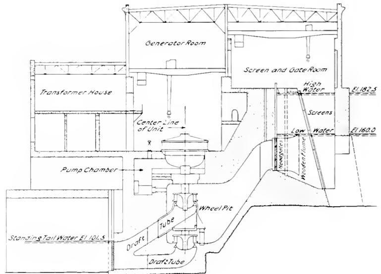
Fig. 3. Cross-section Through Turbine Room and Gate Room
