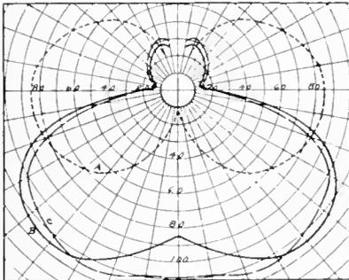
Fig. 13. Characteristic Distribution of Reflectors Shown in Fig. 12
