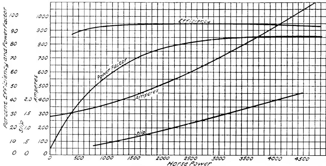
Fig. 6. Characteristic Curves of Induction Motors
