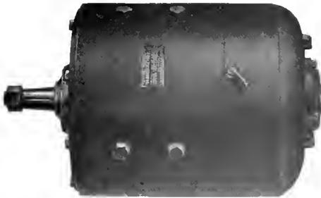
Fig. 15. Motor for Industrial Car
