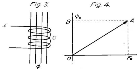
Fig. 4, and equal to  $W = \frac{F\phi}{2}$  just as the stored mechanical energy in Fig. 2 equalled  $W = \frac{F l}{2}$ .
