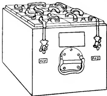
Fig. 2. Lead Battery for Electric Vehicle in Tray
