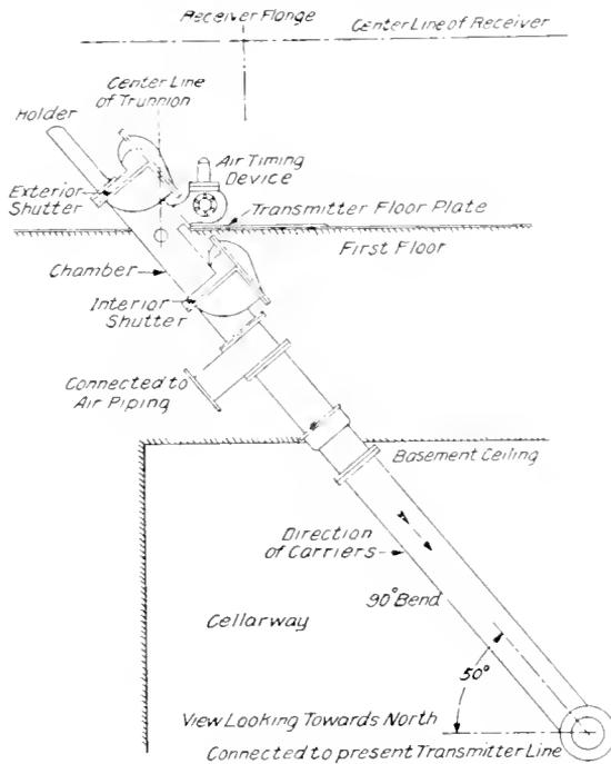
Fig. 1. Transmitter Used in Philadelphia Pneumatic Tube Mail Delivery System
