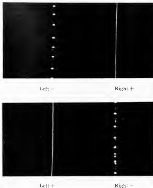
Fig. 4. Corona on Parallel Wires
