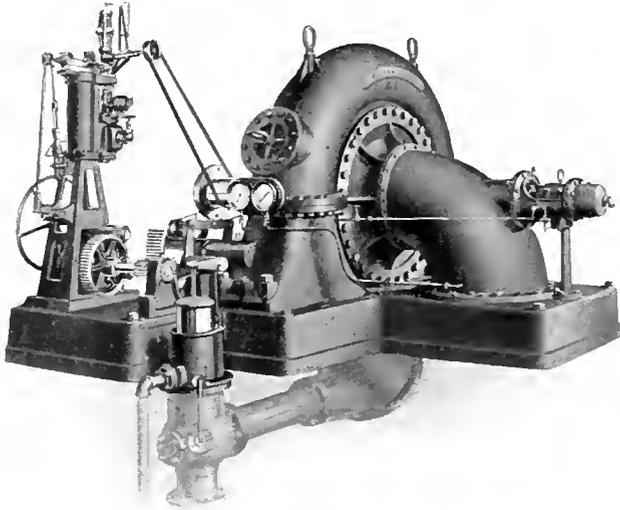
One of three units each of 800 H.P. at 600 R.P.M. under 250 feet head.
