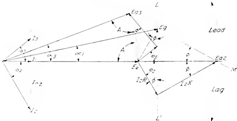
Fig. 8. Vector Diagram Showing Effect of Wattless Current on Generator Voltage if a Given Amount of Energy is Delivered at Constant Speed
