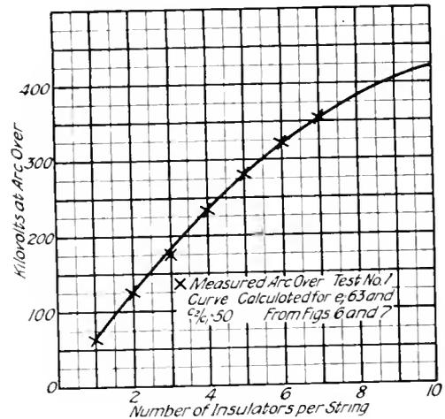
Fig. 8. Comparison of Calculated Curves and Test Curves
