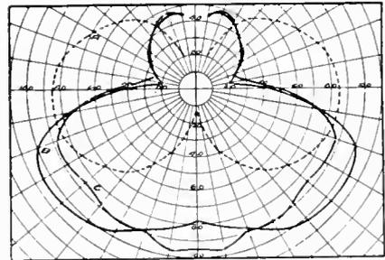
Fig. 15. Characteristic Distribution of Reflectors Shown in Fig. 14
