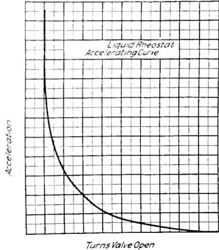
Fig. 5. Liquid Rheostat Accelerating Curve
