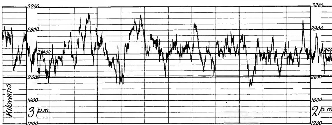
Fig. 1. Load Curve from Large Mine Power House
