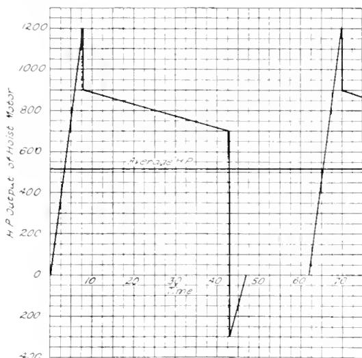
Fig. 2. Load Curve of Mine Hoist
