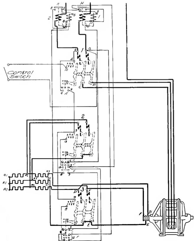
Fig. 3. Wiring Diagram of Three-point Automatic Control Panels for Slip Ring Induction Motor
