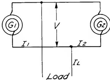
Fig. 3. Two Generators in Parallel
