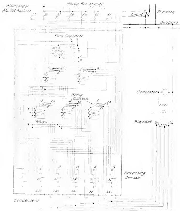
Fig. 3. Connections for Large Slow Speed Generators
