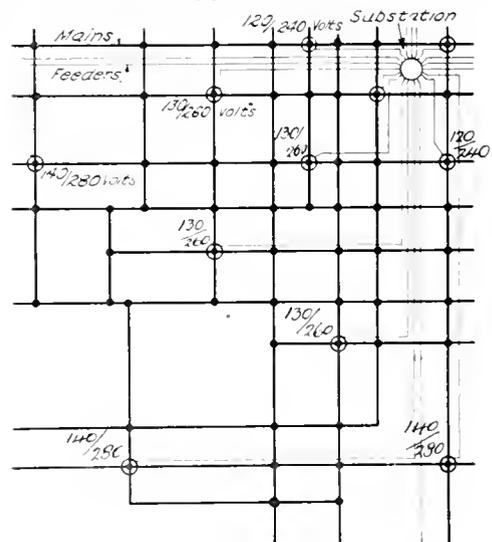
Fig. 1. Edison 3-wire System of Distribution
