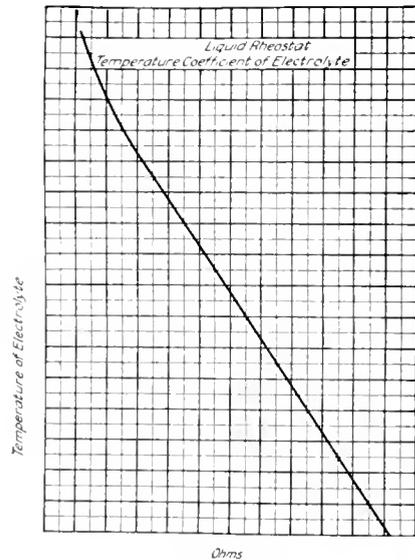
Fig. 6. Temperature Coefficient of Electrolyte in Liquid Rheostat
