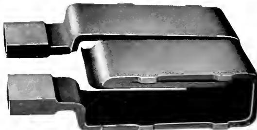
Fig. 8. Series Coil of Pure Copper, Cast in One Piece by the Use of Boron Suboxide
