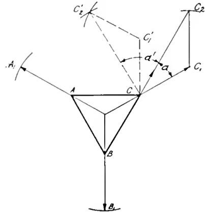
Fig. 2. One Single-phase Regulator on 3-phase System.
