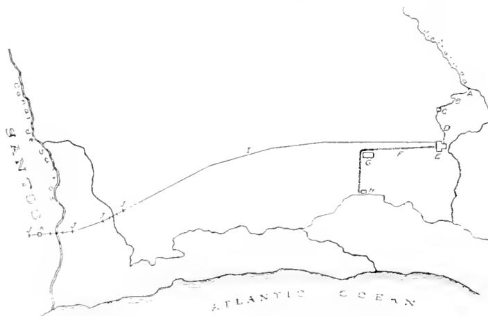
Fig. 1. Map of Cia Docas de Santos Hydro-electric System. A, intake; B, flume, C, forebay; D, pen stocks; E, power house; F, narrow gauge railway; G, general store; H, point of debarkation; I, transmission line; J, dead ends; K, substation.
