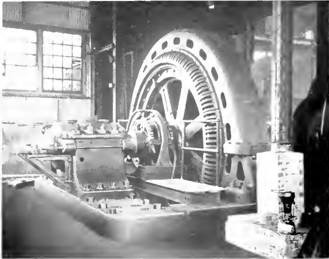
Fig. 9. 1000 H.P. Induction Motor Driving 20 in. Bar Mill
