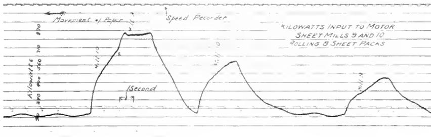
Fig. 15. Wattmeter Record of Power Supplied to Two Mills
