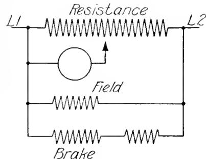
Fig. 2. Connection Diagram for Ammunition Hoist Motor
