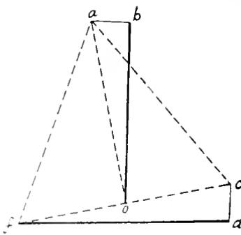
Fig. 21. Reactance Drop in T Connected Transformers, 3-Phase Primary. Perfect interlacing and equal per cent. reactance in main and teaser.
