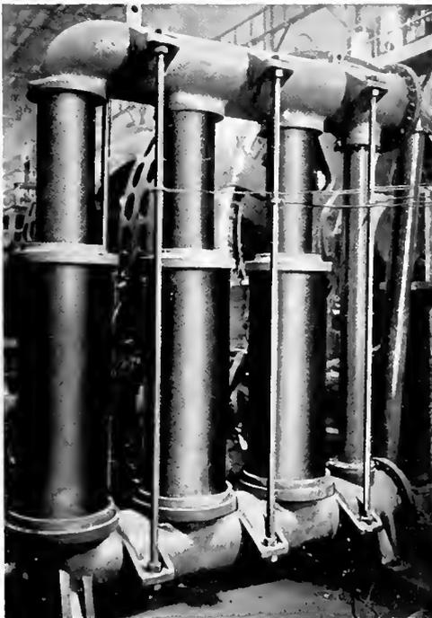
Fig. 3. Water-cooled Resistance for One Induction Motor
