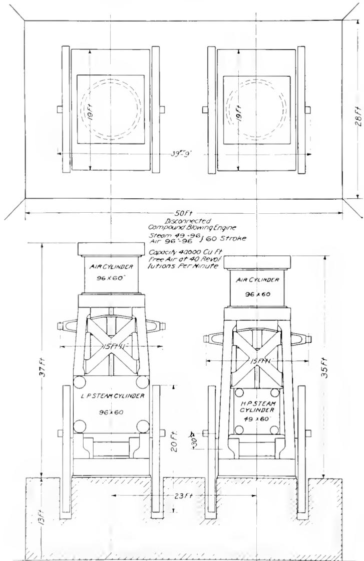
Disconnected Compound Steam Engine Driven Blower
