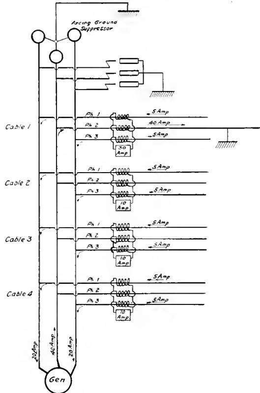
Fig. 6. The General Connections of the Localizer of Faulty Feeders and the Arcing Ground Suppressor
