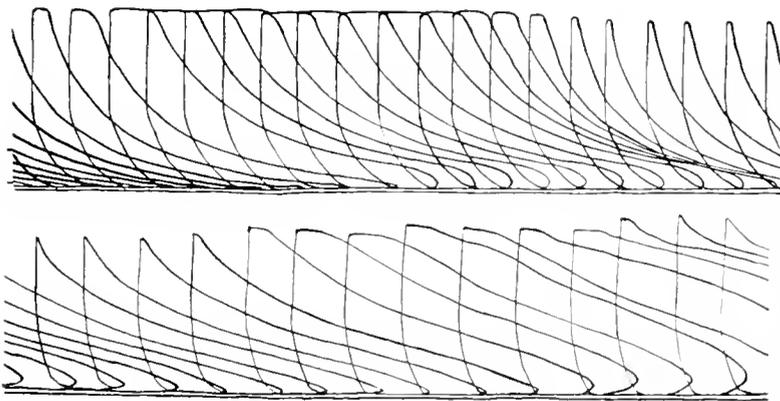
Figs. 4 (upper) and 5 (lower). Steam Engine Indicator Diagrams
