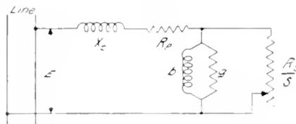
Fig. 6. Series-Parallel Circuit, approximately equivalent to induction motor operating at slip *s*. Circuit *B*
