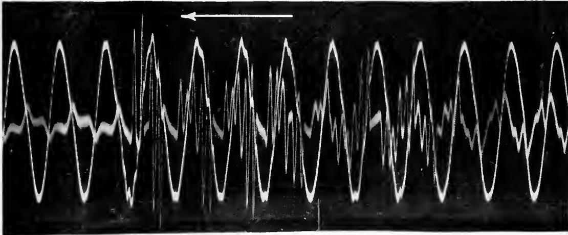
Fig. 10. 28 miles of single-phase 100,000 volt line with two 3333 kv-a. transformers at end) switched off by high-tension switches. Waves of low-tension current and potential
