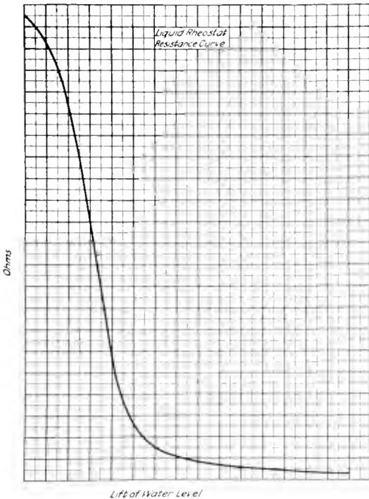
Fig. 4. Liquid Rheostat Resistance Curve
