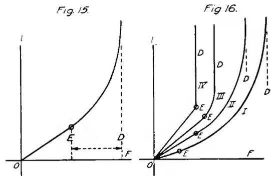
teresis loss begins, and the disruptive limit D, where the deformation curve becomes vertical and mechanical destruction occurs.
