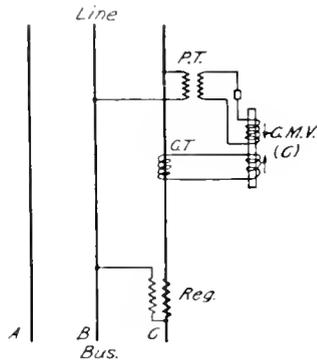
Fig. 1. One Single-phase Regulator on 3-phase System
