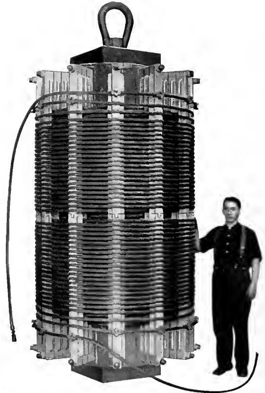
Fig. 6. 720 Kv-a. Busbar Reactance Built for the Commonwealth Edison Co., Chicago
