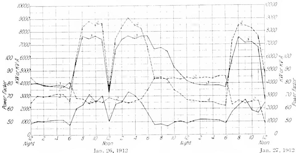
No. 1. Wattless kv-a. from synchronous condensers under automatic control.
