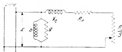
Fig. 7. Modified Circuit for Induction Motor, commonly used in the graphical solution of induction motor problems. Circuit *C*
