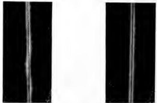
Fig. 3. Corona on Polished Parallel Wires without Stroboscope
