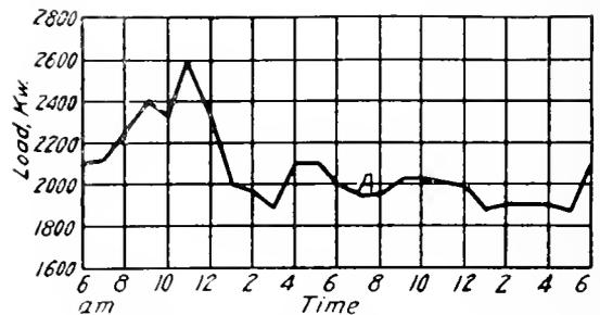
Fig. 1. Load Curve of 3000 Barrel Plant. Hourly Indicating Wattmeter Readings
