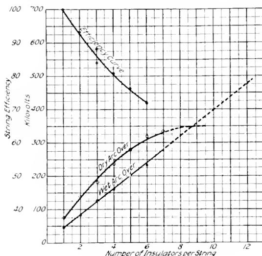
Fig. 2. Test Characteristic Curves of Suspension Insulators
