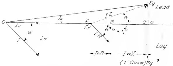
Fig. 7 Vector Diagram of a Transmission Line Illustrating the Relation Between Generator and Receiving Voltage for Different Loads and Power-factors
