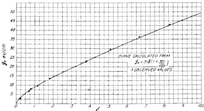
Fig. 12. Effect of Air Density on Visual Corona
