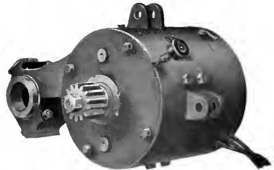
Fig. 13. Motor for Snow Sweeper, Converted Automobile Type
