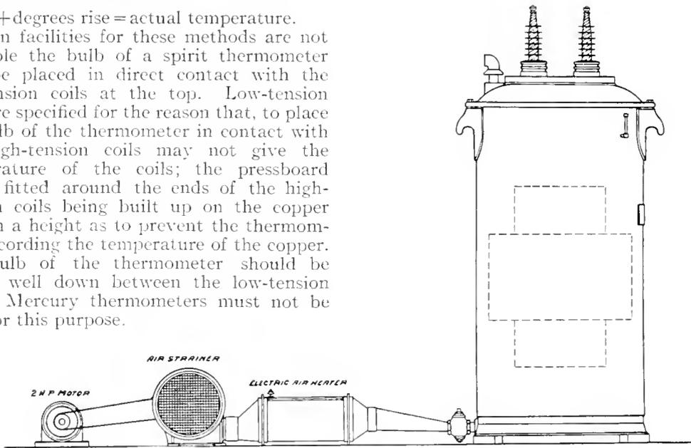
Fig. 3. Hot Air Drying Outfit for Drying Transformers
