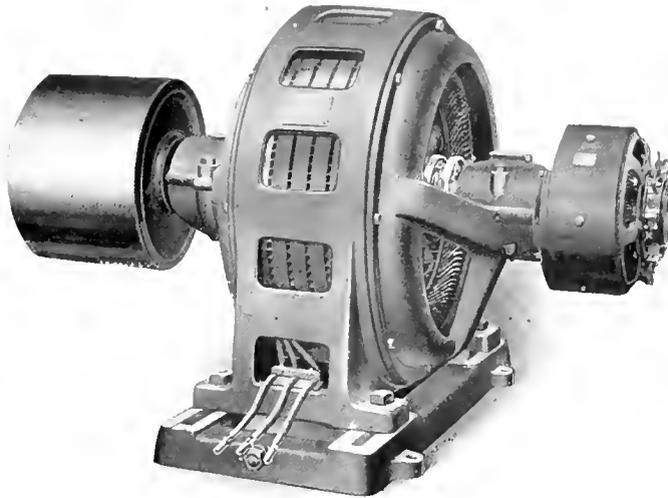
Fig. 4. Belt-driven Generator with Direct-connected Exciter
