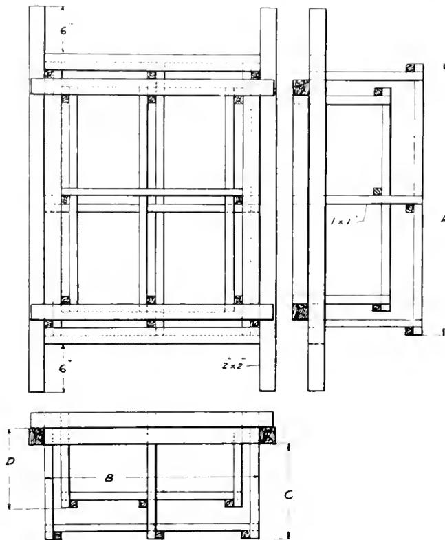
Fig. 5. Frame for Oil Strainer
