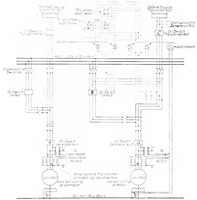
**Fig. 2. Diagram of Connections. Dotted Lines show Circuits of Special Testing Instruments**
