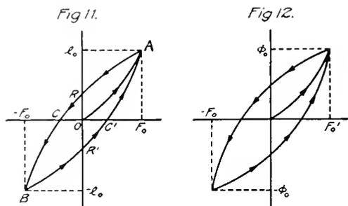
is, between tension and compression, a cycle of deformation results, as shown in Fig. 11. Such a cycle ARCBR'C'A is called a "hysteresis cycle," or "hysteresis loop." Its area measures the energy consumed in the material during the cyclic change of force, as *molecular mechanical friction*, as has been shown before; OR and OR' are the residual or remanent deformations, OC and OC' the coercitive forces required to overcome these deformations.
