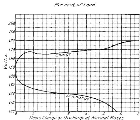
Fig. 6. Edison Cell. Normal Charge and Discharge Curves
