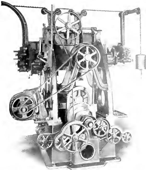
Fig. 5. Induction Motor driving Bullard 42 inch Boring Mill
