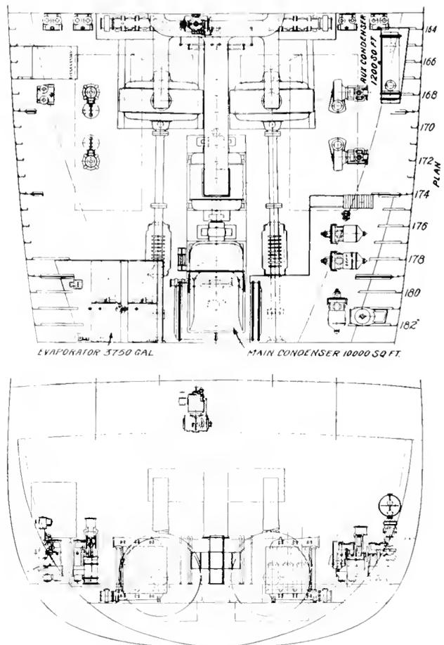
Fig. 1. Arrangement of Electrical Propelling Machinery shown in Plan and Elevation
