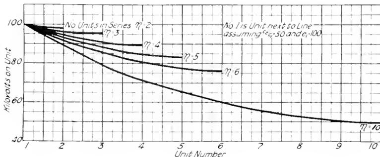
Fig. 6. Calculated Voltage Across Different Insulators in a String of *n* Units
