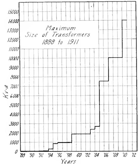
Fig. 6. Maximum Size of Transformers
