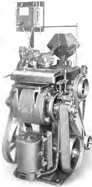
Fig. 7. Direct Current Motor Driving Manville Automatic Screw-slottting Machine
