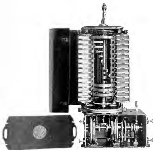
Fig. 13. Drum Controller for 300 H.P. Hoist Motor, Showing Mounting of Mechanical Acceleration and Retardation Limit Device
