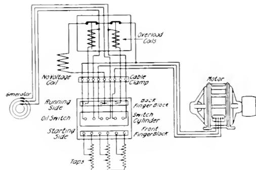
Fig. 2. Wiring Connection for Compensator Shown in Fig. 1
