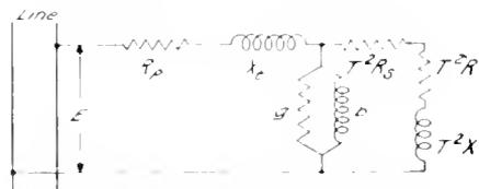
Fig. 3. Series-Parallel Circuit, approximately equivalent to Fig. 1. Circuit  $B_t$
