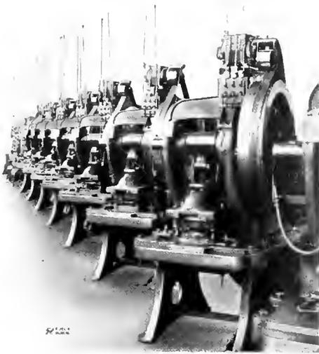
Fig. 9. Ferracut Punch Presses Individually Driven by Induction Motors
