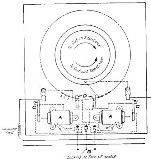
Fig. 6. Connection Diagram for Solenoid-operated Rheostat
