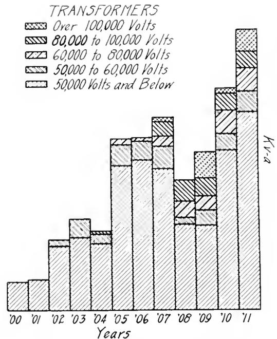
Fig. 1. Transformer Production, Classified by Voltages
