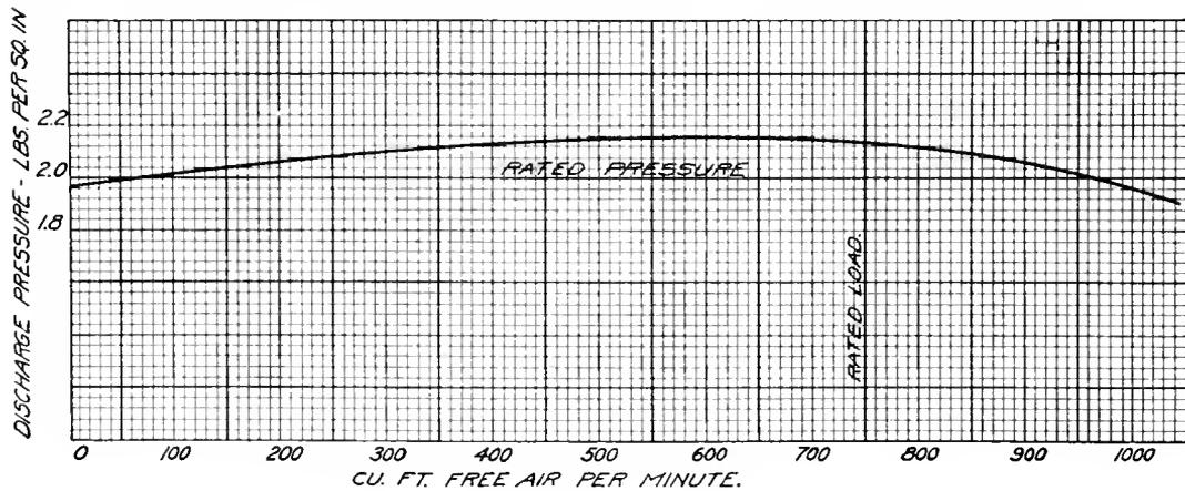
Fig. 25. Characteristic Curve of Single Stage Compressor
