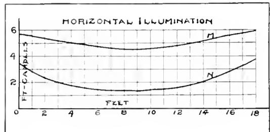
Fig. 3. Illumination Curves. N, Old Installation; M, 400 Watt Mazda Installation
