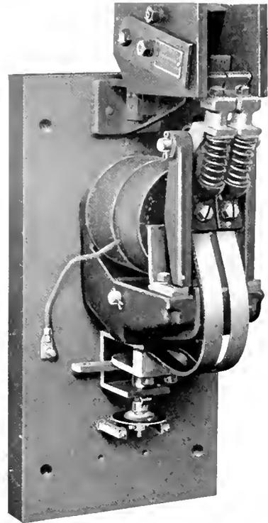
Fig. 3. Direct Current Contactor
