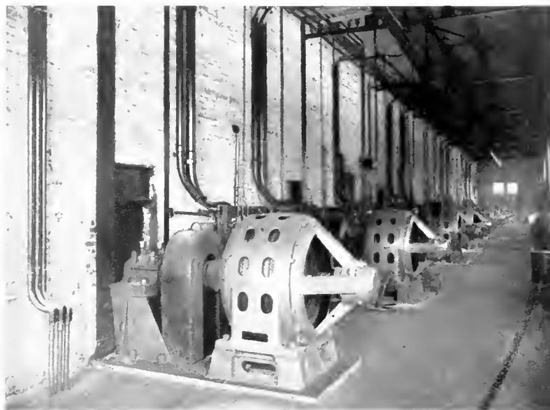
Fig. 2. 250 H.P. Squirrel-Cage Motors Driving Hammer Mills
