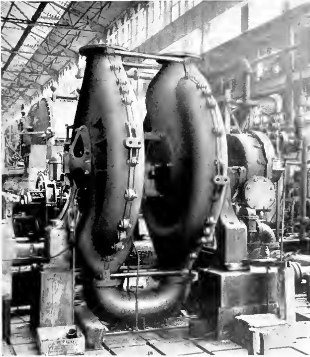
Fig. 26. Centrifugal Compressor Driven by 80 H.P. Curtis Turbine
