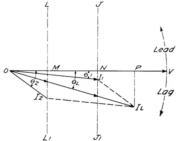
Fig. 4. Vector Diagram of Two Generators in Parallel
