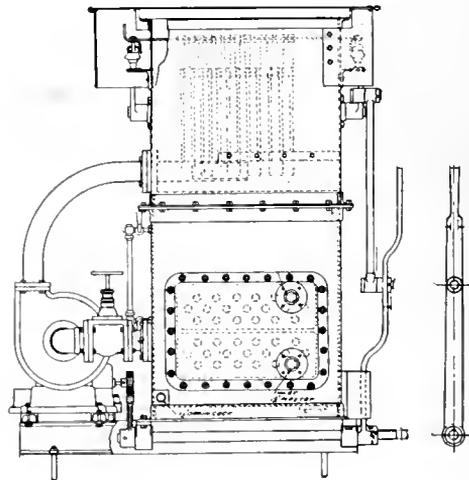
Fig. 3. Internal Construction of Liquid Rheostat
