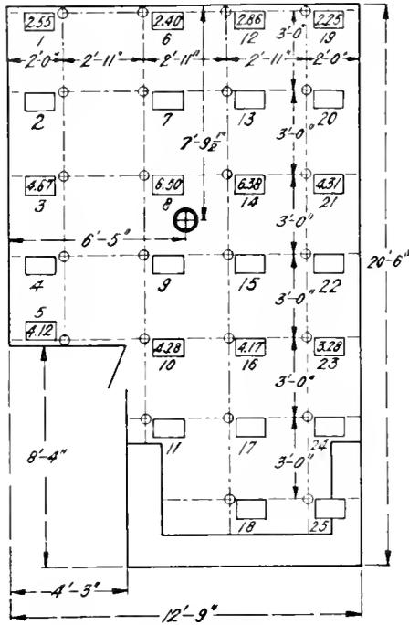
Fig. 6. Layout and Intensities for Indirect Illumination
