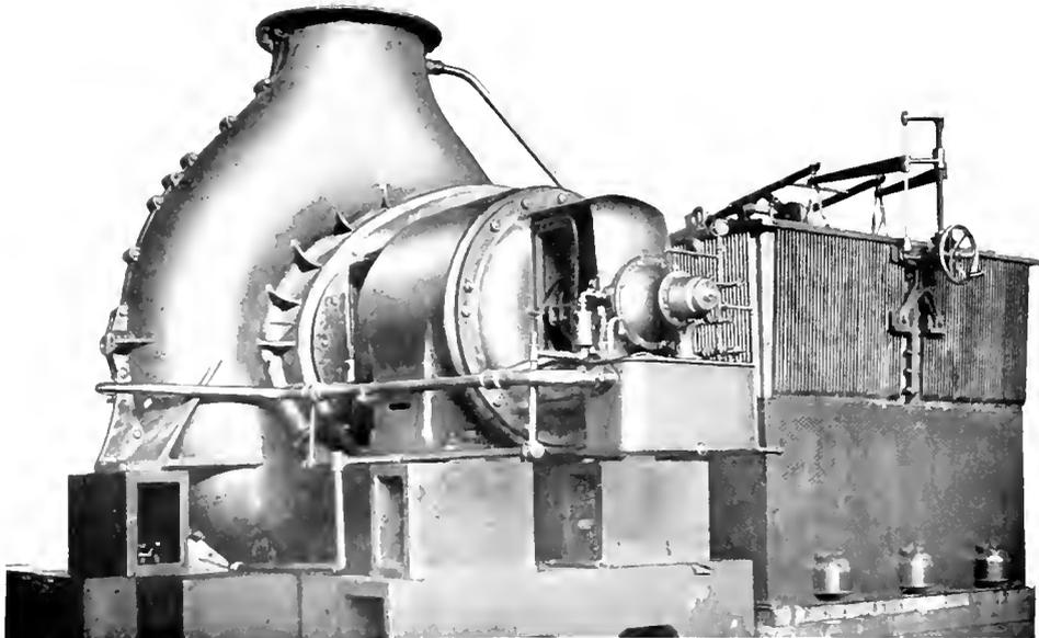
Fig. 27. Compressor Driven by 375 H.P. Curtis Turbine
