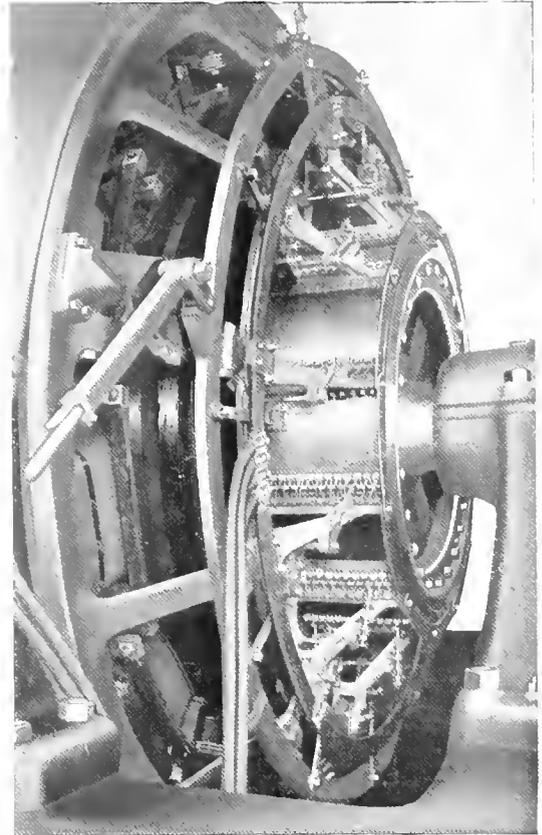
Fig. 8. Brush Raising Mechanism for Synchronous Converter
