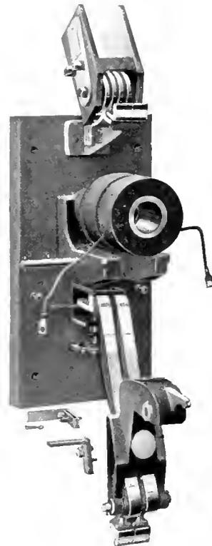
Fig. 2. Method of Removing Operating Coil of Contactor
