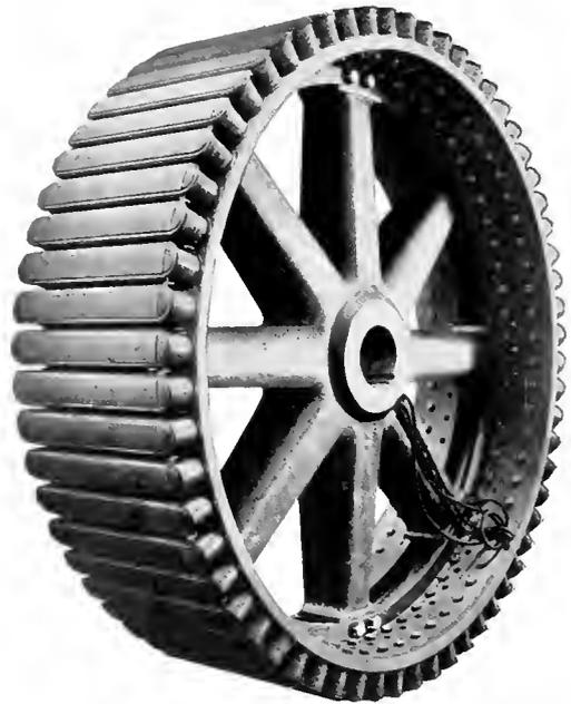
Fig. 2. Revolving Field of 4000 kw., 116 r.p.m. three-phase generator, showing design generally used for moderate and slow speed generators; all castings are made to be free from shrinkage strains
