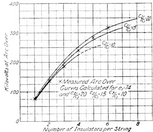
Fig. 9. Comparison of Calculated Curves and Test Curves
