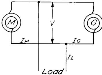
Fig. 5. An Alternator and Motor in Parallel
