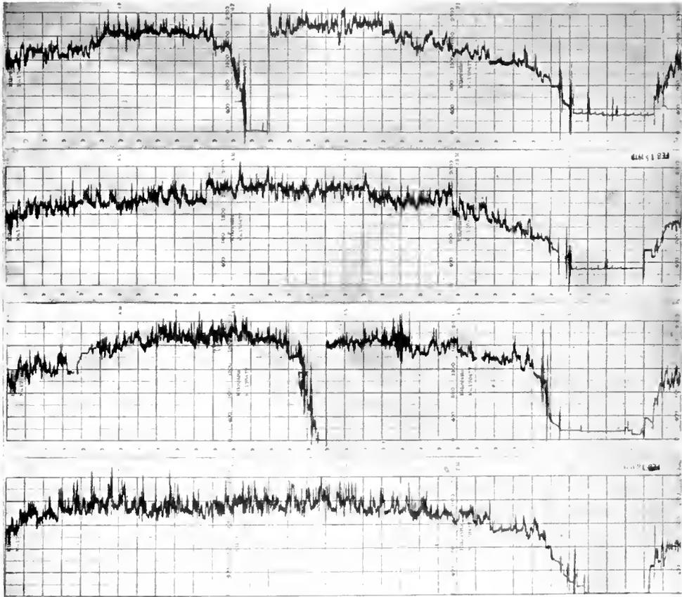
Fig. 13. Typical Load Curve (Feb. 15, 1911) Port Henry Power Station
