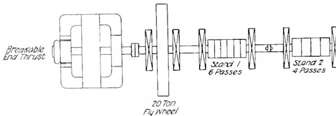
Fig. 10. Plan of 20 in. Bar Mill
