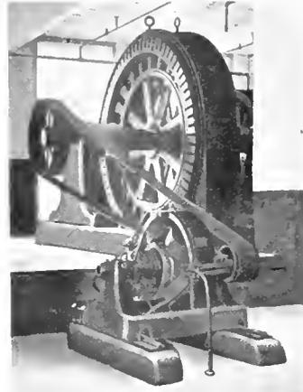
Fig. 1. 1250 Kw. Alternator, Wiscassett Mill
