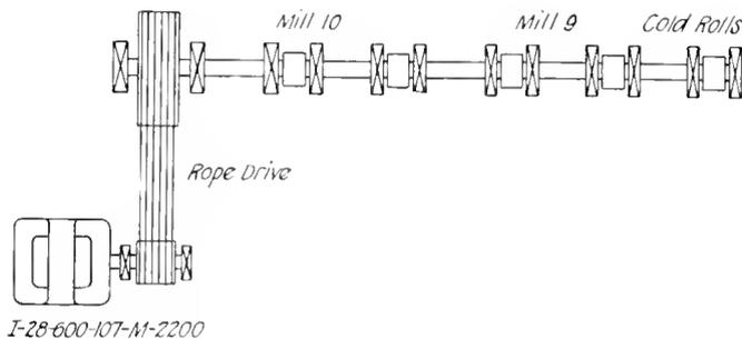
Fig. 12. Plan of 30 in. Four-Stand Sheet Mill
