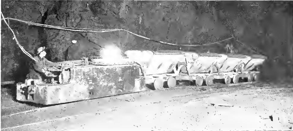
Fig. 11. 10 Ton Electric Mine Locomotive
