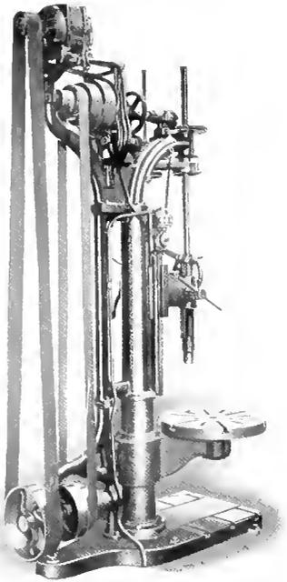
Fig. 3. Induction Motor driving Prentice 24 inch Drill
