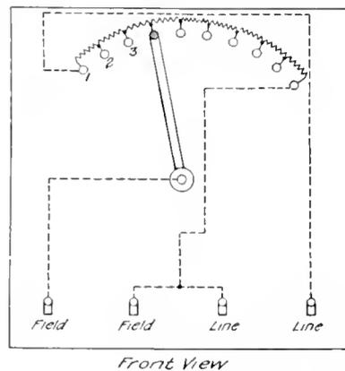
Fig. 10. Connections of Series Shunt Rheostat for Direct Current Generator
