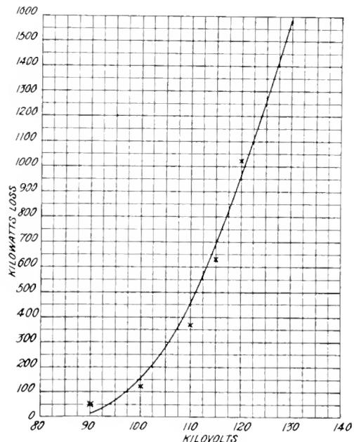
Fig. 1. Comparison of Calculated and Measured Losses
