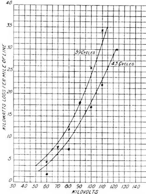
Fig. 2. Comparison of Calculated and Measured Losses
