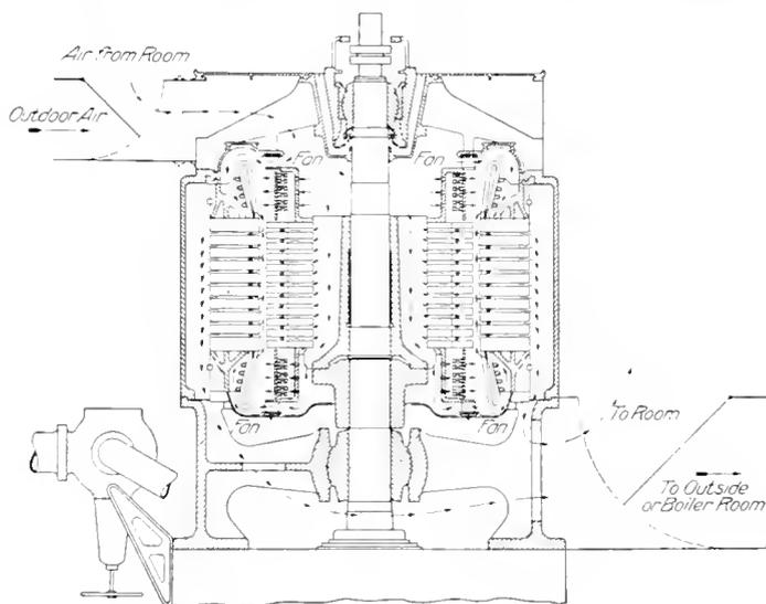
Fig. 1. Ventilation of Vertical Steam Turbine Alternator
