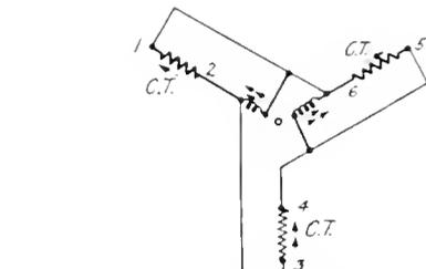
Fig. 6. Two Single-phase Regulators on 3-phase System, using one current transformer on middle leg instead of two as in Fig. 5
