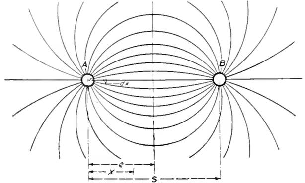
Fig. 9. Visual Critical Voltage Gradient—Two Parallel Wires
