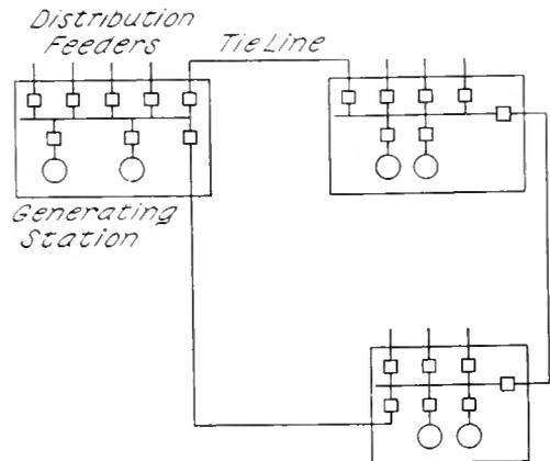
Fig. 2. Simple System, with Tie-Lines Between Generating Stations
