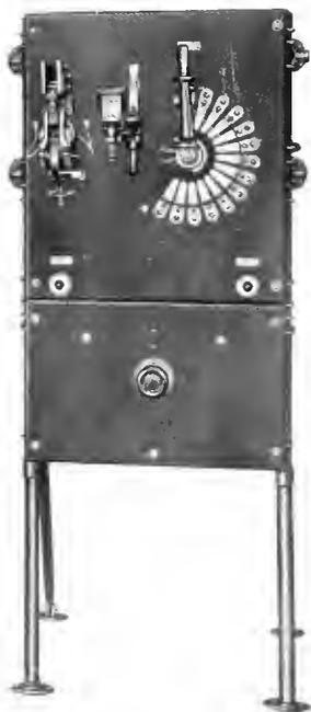
Fig. 1. Hand-operated Dial Controller used with direct current single motor semi-automatic printing press equipments. Push button jog; push button stop; no-voltage release; overload release; dynamic brake; slow speed; armature and shunt field regulation are provided.
