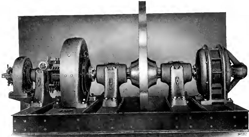
Fig. 7. 90 Kw., 500 Volt Generator Direct Connected to 75 H.P. 440 Volt Induction Motor, Kendall Gold Mines
