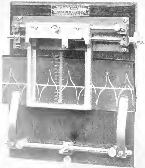
Fig. 1. Micrometer for Measuring Oscillograph Records
