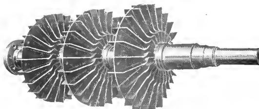
Fig. 17. Rotating Element of Three-Stage Blast Furnace Compressor
