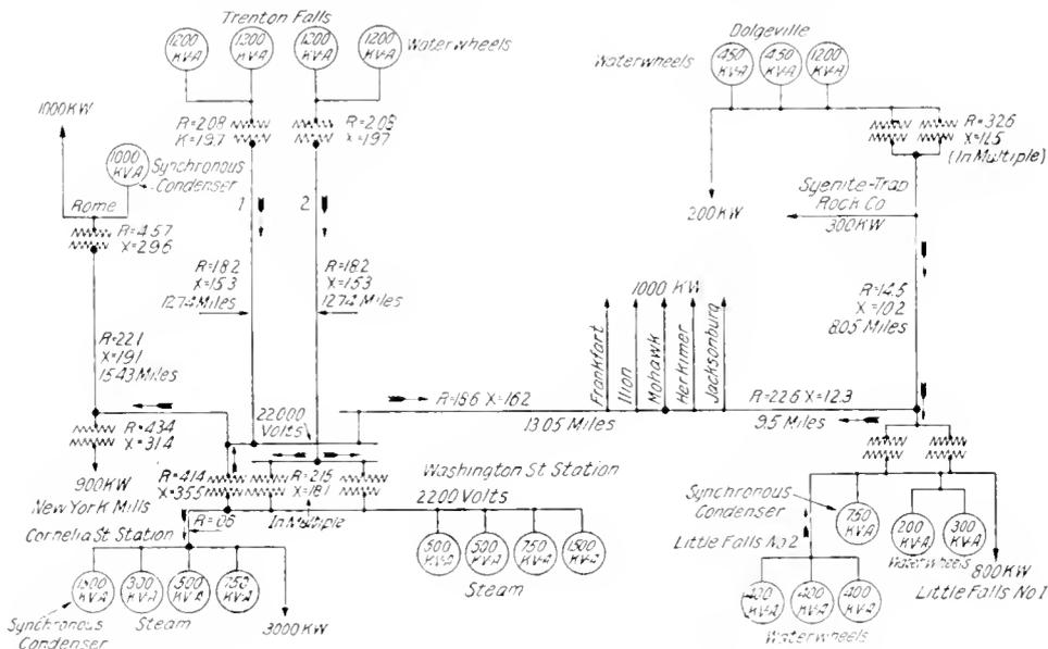
Fig. 22. One-line \* Diagram Showing the Generators, Synchronous Condensers, Transmission Lines, etc., of the System of the Utica Gas & Electric Company
