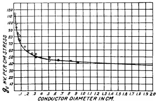
Fig. 10. Visual Critical Voltage Gradient, Two Parallel Wires
