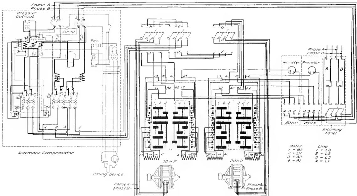
To start 50HP Motor from automatic compensator throw switch A into E position and switch C into H position
