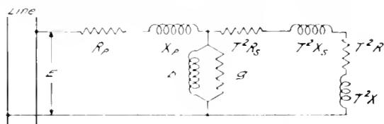
Fig. 2. Series-Parallel Circuit, the equivalent of Fig. 1. Circuit  $A_t$
