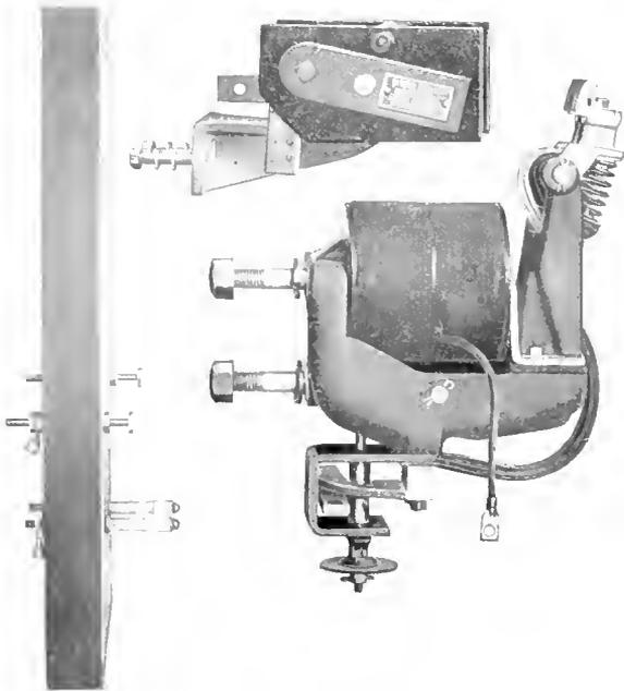
Fig. 1. Parts of Direct Current Contactor
