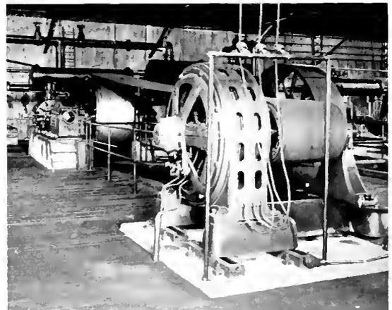
Fig. 4. Air Compressors Driven by 500 H.P. Induction Motor
