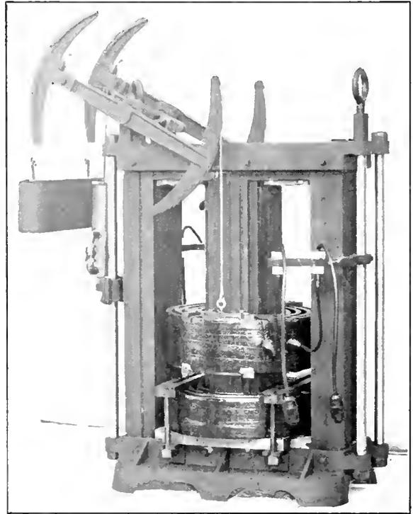
Fig. 3. Constant Current Transformer for Series Lighting
