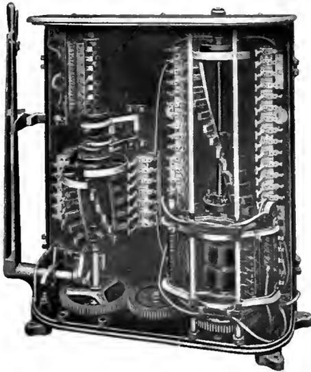
Fig. 4. Internal View of Controller for Starting, Regulating and Reversing Cogging Mill Motor
