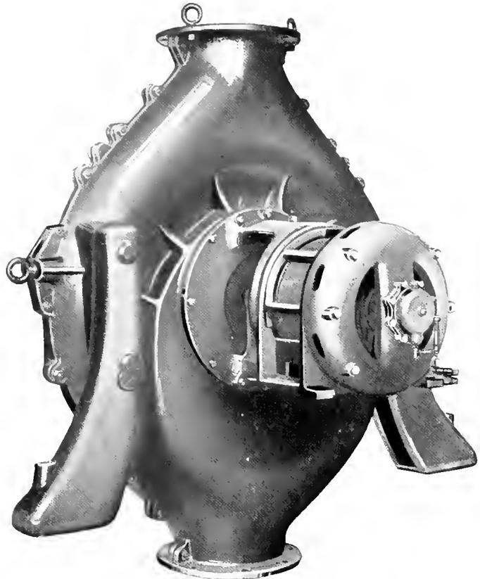
Fig. 12. Centrifugal Compressor Driven by 50 H.P. Induction Motor
