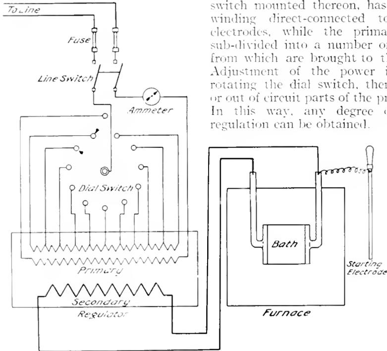
Fig. 4. Diagram of Electric Circuits
