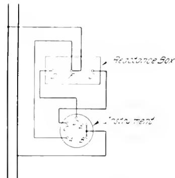
Fig. 7. Connections for Checking Location of Needle
