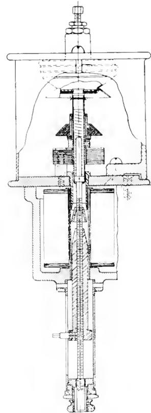
Fig. 4. Sectional View of Definite Time Limit Overload Relay
