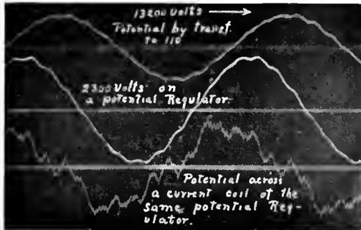
Fig. 9. Potential across a series coil of a potential regulator of the induction type operating at 2300 volts line potential (lower curve). Prominent harmonics are: the 13th from the teeth of the generator and still higher harmonics from the reactions of the teeth of motors. The upper and middle curves are potentials of the 13200-volt and 2300-volt circuits. The potential waves show only the 13th harmonic superposed on the fundamental wave at 60 cycles
