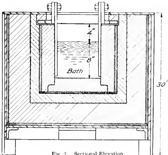
Fig. 2. Sectional Elevation of Furnace
