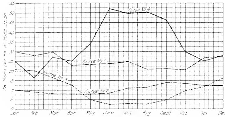
Fig. 7. Curves Showing Comparative Current Consumption of Four of the Principal Types of Farm Loads. Curve 1, Lighting, Irrigation, and General Farming. Curve 2, Lighting. Curve 3, Huskers, Shredders and Feed Grinders. Curve 4, Pumping and Refrigeration
