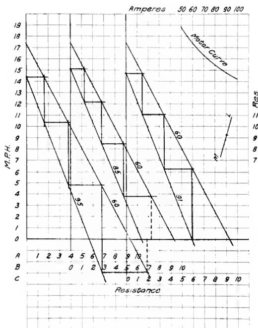
Fig. 3. Diagram showing the method of adjusting the current limit to satisfy assumed conditions
