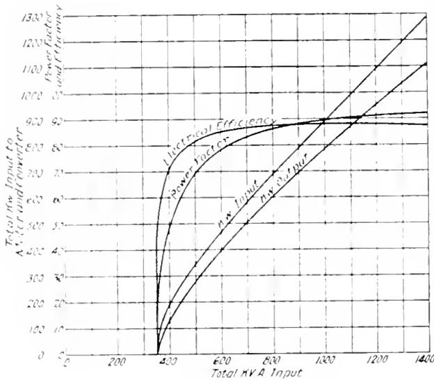
Fig. 5. Characteristic Curves of Split Phase Locomotive
