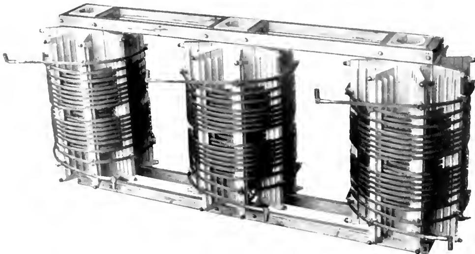
Bank of 6 per cent reactances for Three-Phase 50-Cycle, 15,000 Kv-a., 11,000-Volt, Turbo-Generator, Showing Method of Mounting and Bracing
