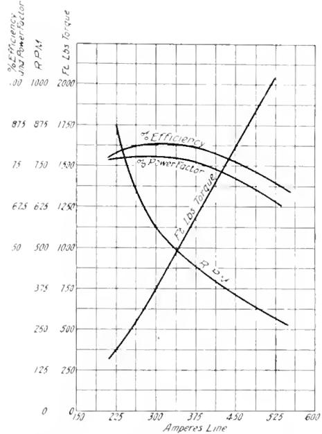
Fig. 6. Repulsion Characteristics (first connection at starting)
