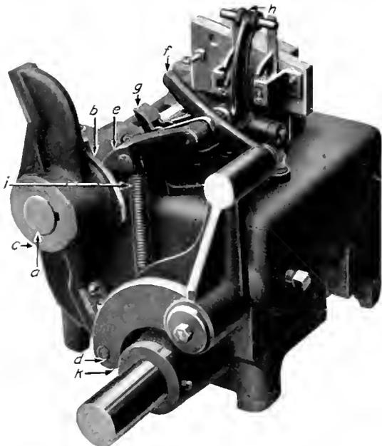
Fig. 1. Locking mechanism for motor-operated oil switch—
