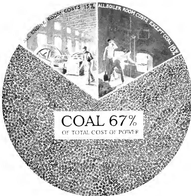
Fig. 16. Diagram Showing the Proportionate Division of the Operating Cost of a Steam Plant
