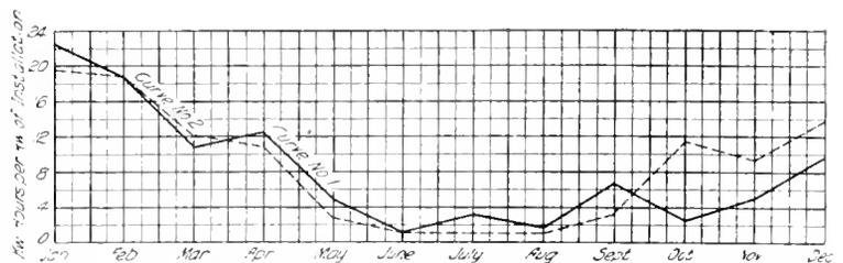
Fig. 12. Curves showing that Huskers and Shredders and Feed Grinders tend to make a Winter Load. Lighting will increase the load to some extent. Curve 1, Huskers and Shredders, and Feed Grinders (68.2 Kw) Curve 2, Huskers and Shredders, Feed Grinders and Lights. (125 Kw. Power) (8.5 Kw. Lighting)
