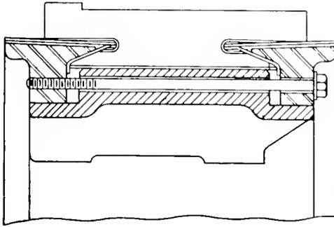
Fig. 2. Section of Body-bound Commutator
