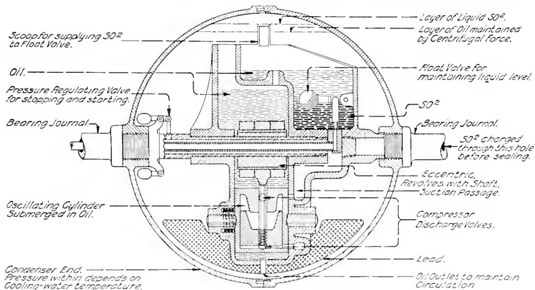
Fig. 14. Sectional View of the Compressor or Spherical End of the "Dumb-bell" Shown in Fig. 13
