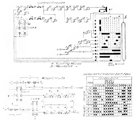
Fig. 17. Simplified Connections with C 74 Controller 1200 Volt Trolley
