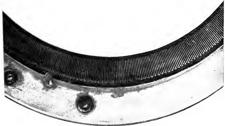
Fig. 7. Standard Winding for 100,000 Cycle Alternator, with 600 Slots
