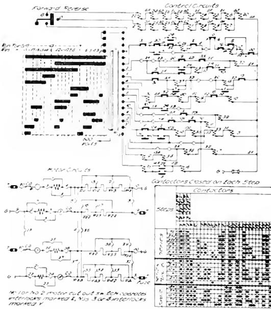
Fig. 21. Simplified Connections with C 83 Controller, 600 Volt Trolley
