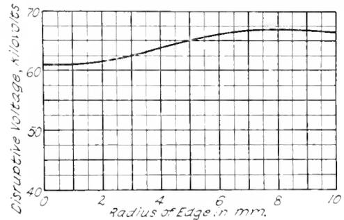
Fig. 5. Curve of Radius of Edge vs. Disruptive Voltage. Sample is of 0.03 cm. Varnished Cloth 10 Layers. 25 mm. Radius of Flat Face of Terminal
