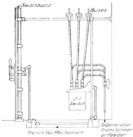
Fig. 1. A Common Arrangement of Oil-Switch on Frame-work back of Switchboard
