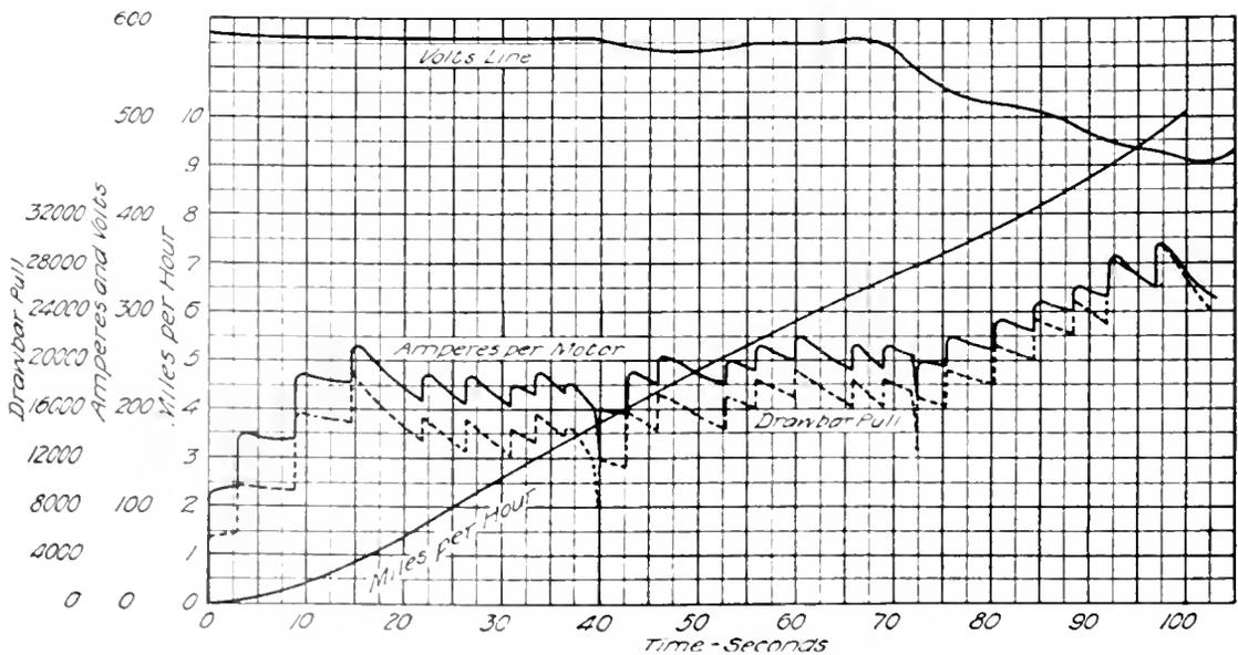
Fig. 18. Acceleration Curves— Locomotive and Twenty-six Freight Cars
