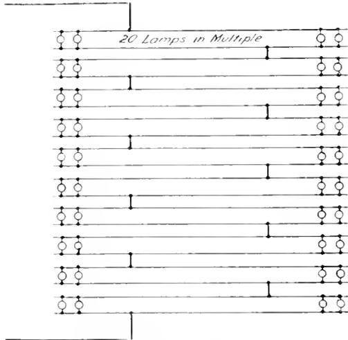
Fig. 7. Multiple-Series Wiring for Sign Lamps, Using 10 Volt Lamps
