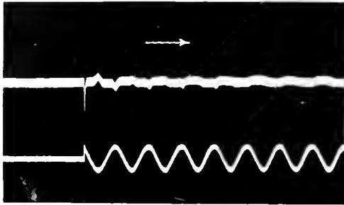
Fig. 23. Oscillogram of the electrostatic charge in an aluminum arrester practically independent of the current needed to reform the film. Note the initial current during the first half-cycle in the upper record. The lower record giving the e.m.f. across the cell starts at nearly its maximum value. This initial value of potential produces the extra current to charge the capacity of the cell
