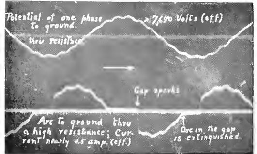
Fig. 31. Arc to ground through a high resistance on a 13,200-volt circuit (lower record). Delta potential of the circuit (upper record)
