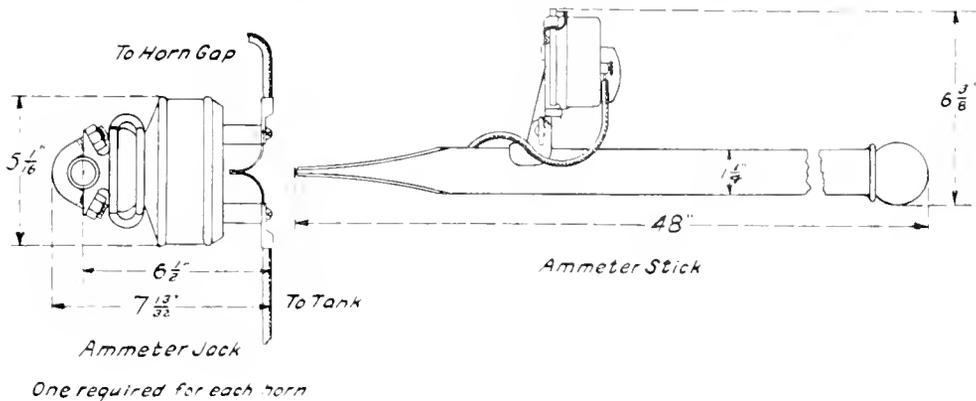
Fig. 20. Charging Current Indicator, 1000-7250 Volts
