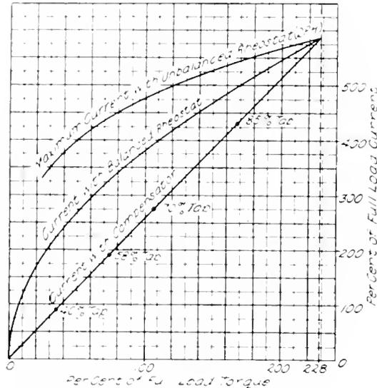
Fig. 5. Per cent Full Load Current for Various Values in per cent of Full Load Torque Observed on 20 h p., 440 Volt Motor when Started with Balanced Rheostat, Unbalanced Rheostat and Compensator
