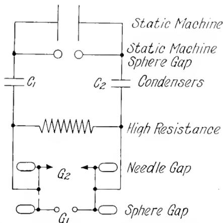
Fig. 1. Diagram of Initial Connections Employed. The Values Listed in Table I Resulted from This Set-up
