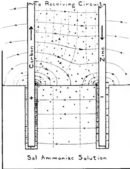
Fig. 4. Energy Stream Near an Electric Battery
