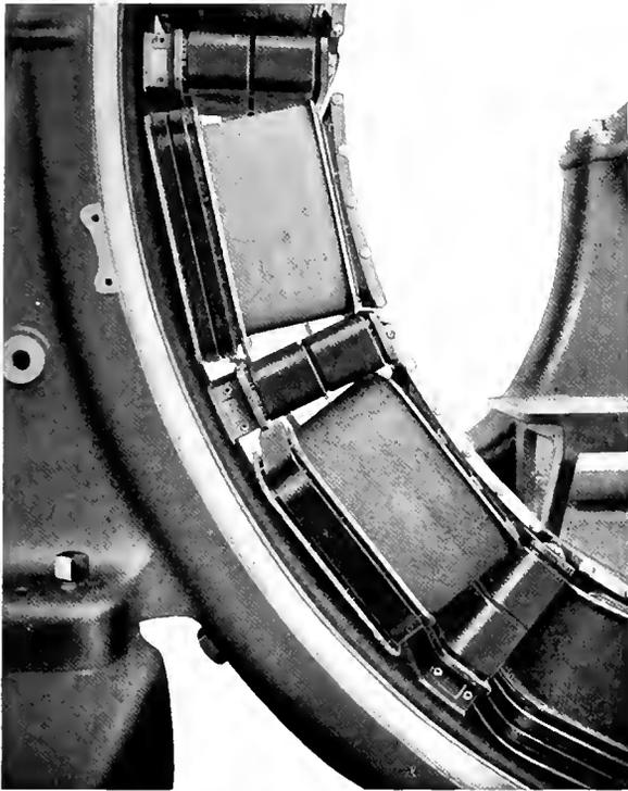
Fig. 7. Nearer View of Shunt Winding, Series Compounding Turn, and Commutating Poles of Converter Shown in Fig. 6
