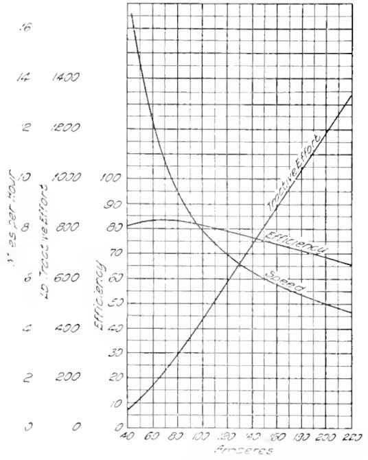
Fig. 2. Characteristic Curve of GE-1027 Motor on 85 Volts. Gear Reduction 6.2 to 1, Wheel Diameter 30 In.
