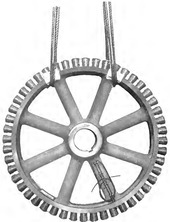
Fig. 31. Lifting Revolving Field (Right Way)
