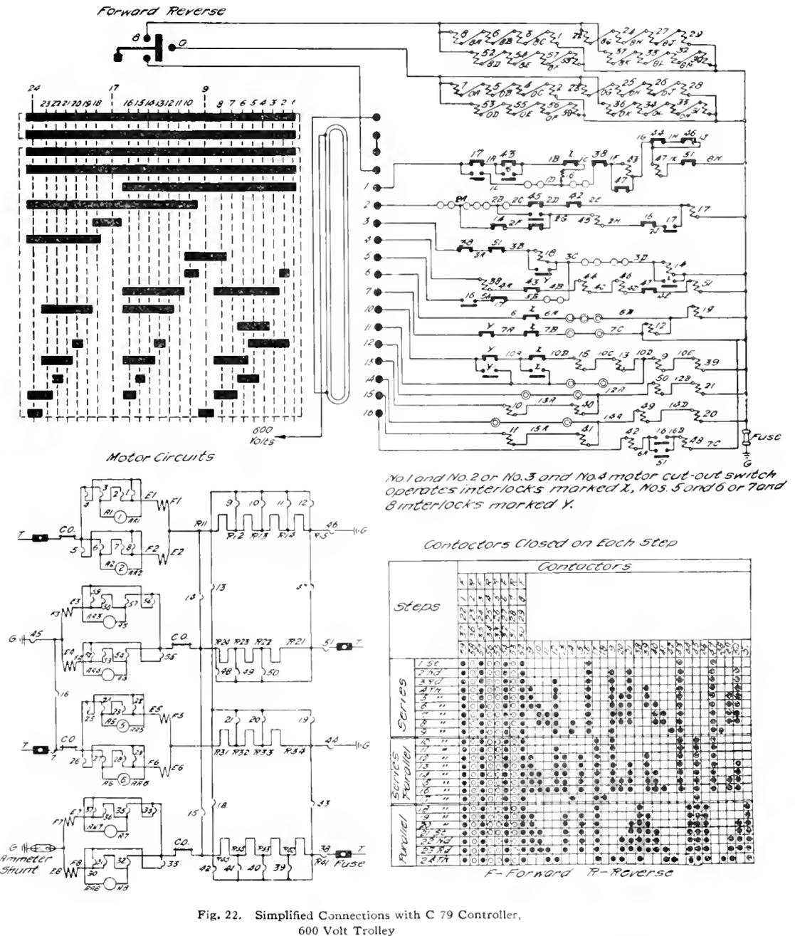
Fig. 22. Simplified Connections with C 79 Controller, 600 Volt Trolley
