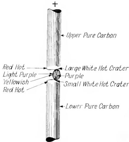
Fig. 6. Direct Current Enclosed Arc
