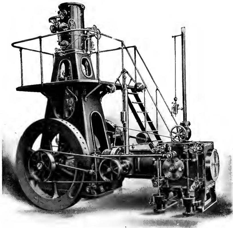
Fig. 9. A Vertical, Double-Acting, Open-Type Ammonia Compressor
