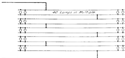
Fig. 8. Multiple-Series Wiring, Using 20-Volt Lamps
