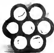
Fig. 15. Another Form of Impregnated Carbon Electrode. The dark section is carbon, the light section light-giving material.
