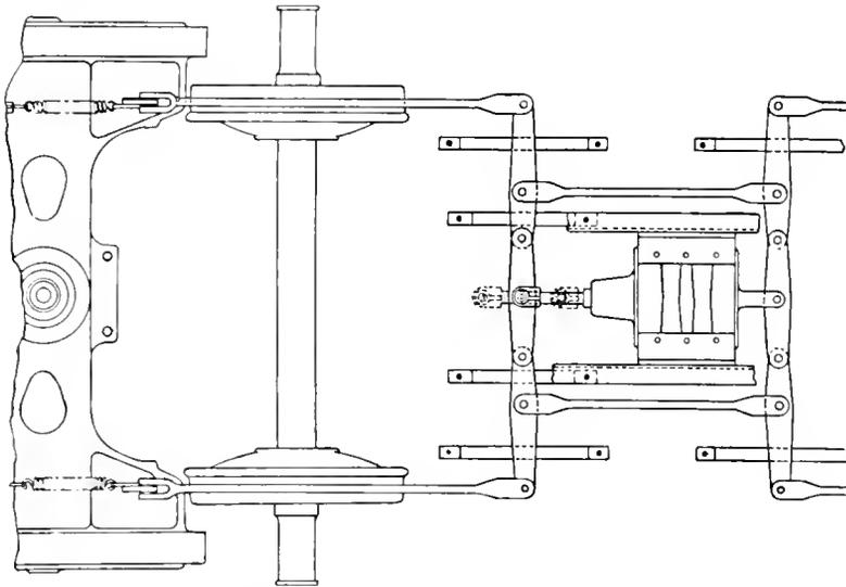
Fig. 9. Arrangement of Brake Levers, 25-Ton Locomotive
