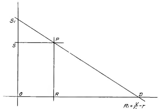
Fig. 1. A simple diagram showing the relation between the Current, Speed, and External Resistance for a Series Motor
