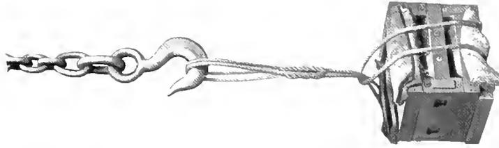
Fig. 18. Double Cable Sling
