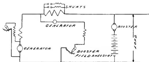
Fig. 21. Connections for Counter E.M.F. Booster
