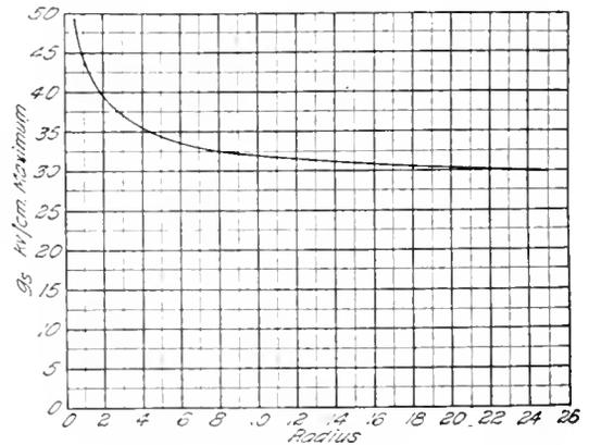
Fig. 7. Surface Gradient for Spheres of Different Size
