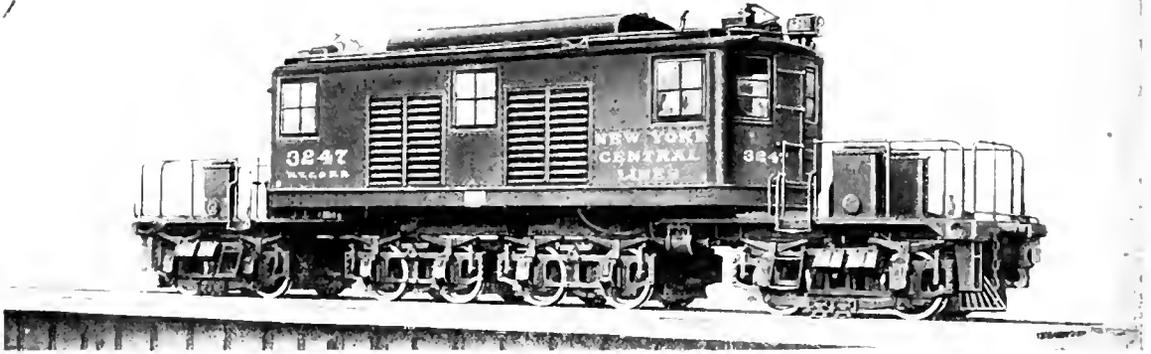
Fig. 1. Direct Current 600-Volt Electric Locomotive in the Service of the N.Y.C. & H.R.R.R.Co. Weight 100 Tons. Equipped with 8 Bipolar Gearless Driving Motors, Each Axle Being a Driving Axle. Capacity of Each Motor 325 Amperes (one-hour); or 250 Amperes (continuous) at 600 Volts. Capacity of Locomotive 13,500 lb. Tractive Effort at 54 Miles per Hour (one-hour rating); or 9500 lb. Tractive Effort at 60 Miles per Hour (continuous)
