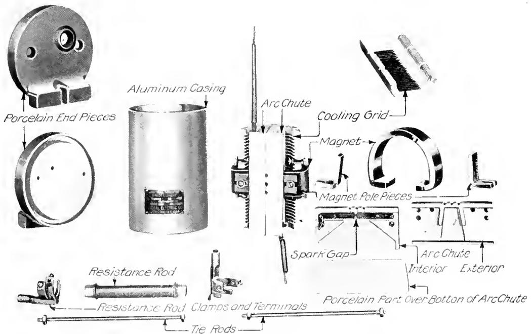
Fig. 3. Exploded View of the Magnetic Blowout Arrester shown in Fig. 2
