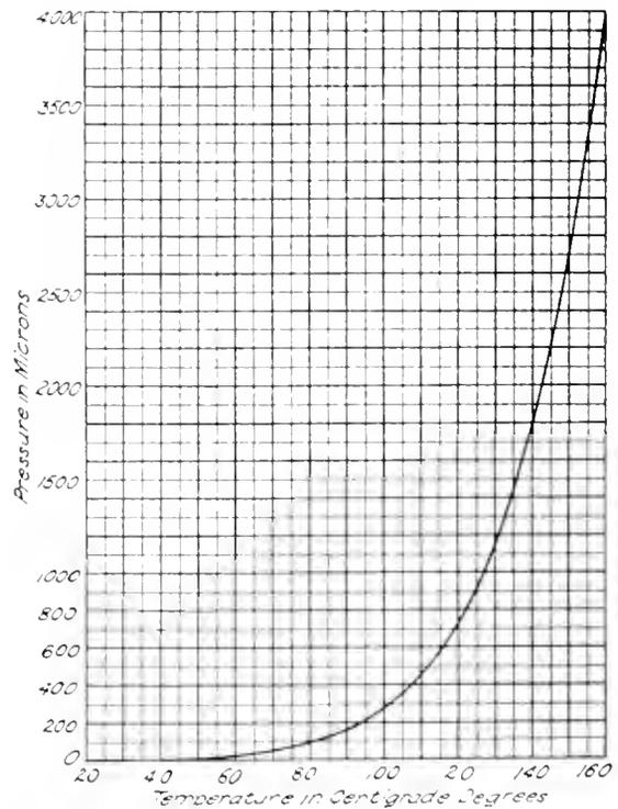
Fig. 6. Mercury Vapor Pressure
