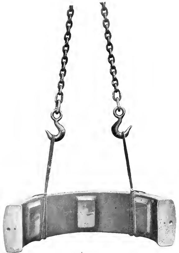
Fig. 23. Right Way of Making a Hitch
