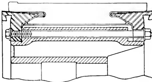
Fig. 1. Section of Arch-bound Type Commutator
