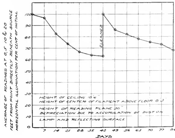
Fig. 1. Curve of Acquired Depreciation. Lamps Only Burned at the Test Periods to Prevent Inherent Depreciation
