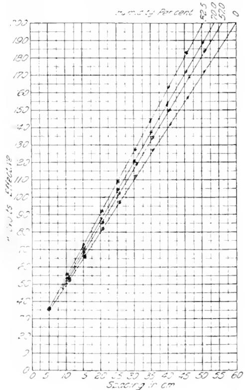
Fig. 1. Needle-Gap Curves for Different Relative Humidity
