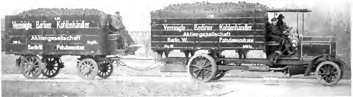
Fig. 5. A Daimler Mercedes Gasolene Truck with Trailer as Used by a Berlin Coal Company
