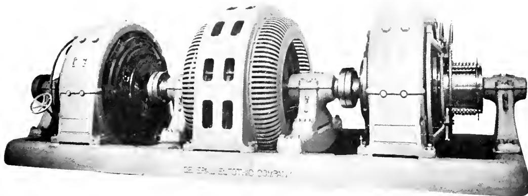
Fig. 2. 2400 Volt Motor-Generator Set
