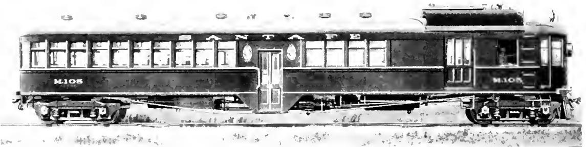
Fig. 2. Combination Passenger and Baggage Gas-Electric Motor Car Operating on the Atchafalaya, Topeka and Santa Fe Railway. This car is 68 ft. in length and has center entrance
