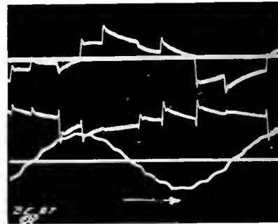
Fig. 34. Potential across a stack of aluminum cells while being charged through a gap of medium length (upper record).
