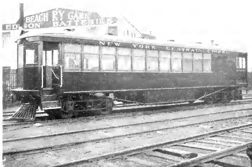
Fig 7. Storage Battery Car Operating on New York Central Lines
