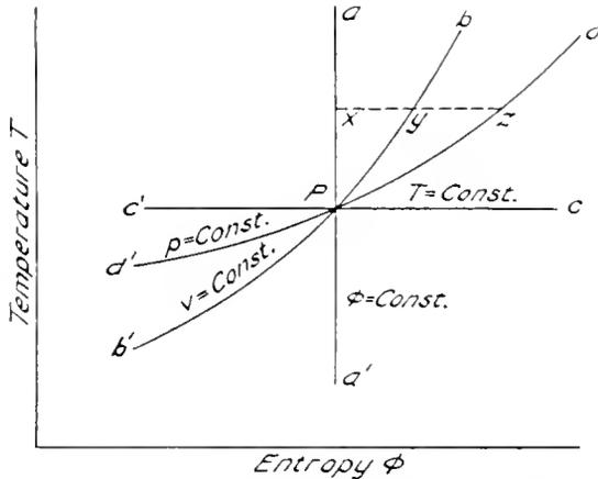
Fig. 5. Thermodynamic Changes in a Perfect Gas Represented in Terms of its Entropy and Temperature
