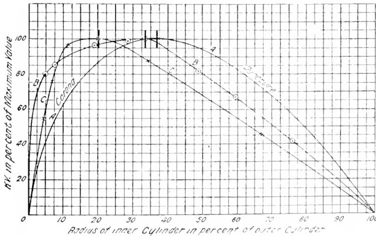
Fig. 1. Curves Illustrating the Effect of Shape of Edges of Outer Cylinder on the Ideal Critical Ratio of Cylinder Diameters
