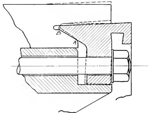
Fig. 3. Section of Commutator Showing Distortion Caused by Excessive Tightening of Clamping Bolts
