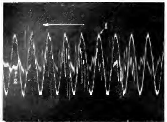
Fig. 14. Switching Line off Transformer by High-Tension Switch. Waves of Low-Tension Voltage and Current
