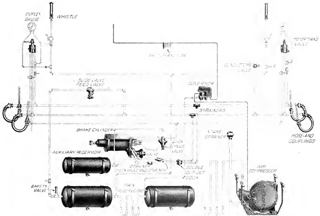
Fig. 4. Combined Straight and Automatic Air Brake Equipment for Motor Car
