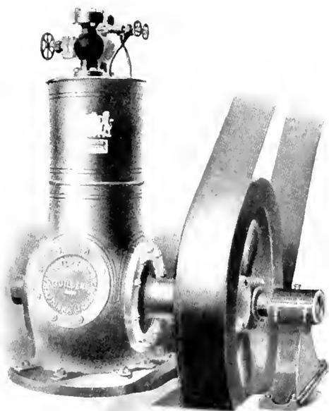
Fig. 10. A Vertical, Enclosed-Type Ammonia Compressor
