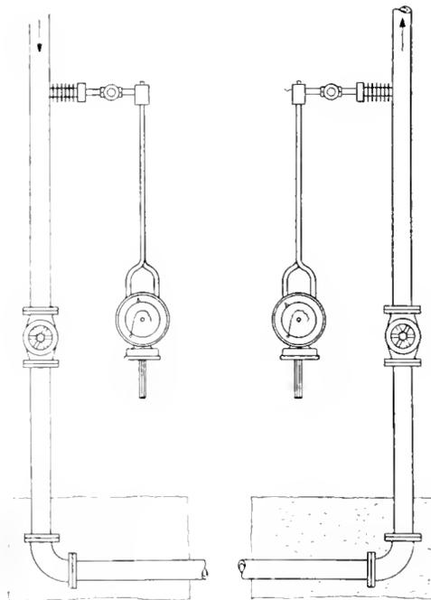
Fig. 3. The Indicating and Recording Flow Meter Measuring Underground Transmission of Steam for Heating and Power Purposes. By the use of two meters Flow Loss can be determined and any leakage discovered
