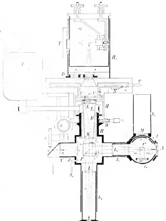
Fig. 5(b). Section of Beckstein Photometer
