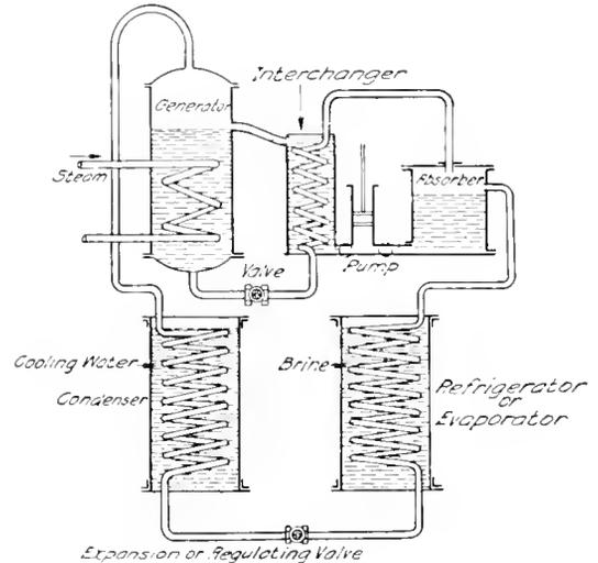
Fig. 2. Diagram of an Absorption-Type Refrigerating System
