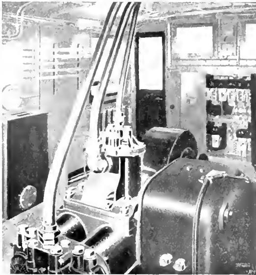
Fig. 11. Air Compressor and Contactors
