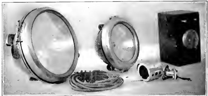
Fig. 2. A  $4\frac{1}{2}$ -Inch and 7-Inch Electric Headlight, and the Necessary Equipment to Operate Either
