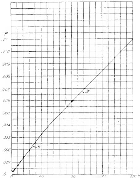
Fig. 3. Reactivity Curve of the Average of 12 Samples of 2.5 Per Cent Silicon Steel
