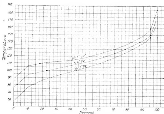
Fig. 2. Curves of Fractional Distillation of Gasolene the Values of Which as a Fuel Are Proportional to Their Hydrometer Readings
