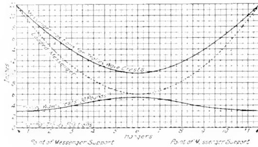
Fig. 6. Trolley Wave Crest Curve for One Span and Corresponding Position of Messenger
