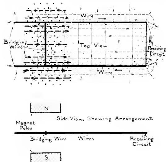
Fig. 5. Energy Stream Near a Dynamo
