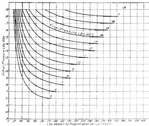
Fig. 7. Curves Showing Pounds of Water in Regenerator per Pound of Steam Generated, when Working Between Various Initial and Final Pressures
