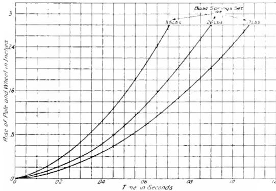
Fig. 3. Representative Time-Rise Curve Resulting From Inertia of a Standard Pole and Wheel Raised by Trolley Base Equipped with Compression Springs
