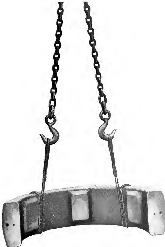
Fig. 22. Wrong Way of Making a Hitch
