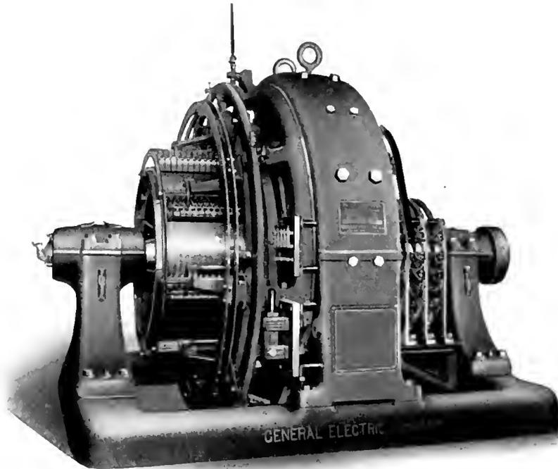
Fig. 10. Commutating Pole Railway Converter, Showing Brush Raising Device Which Must be Used When Machine is Started From A-C. End
