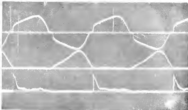
Fig. 15. Upper Curve, Voltage Between Anodes; Middle Curve, Current in One Arc; Lower Curve, Inverse Current
