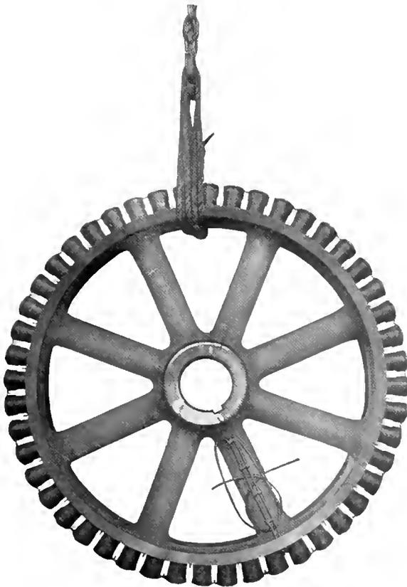
Fig. 30. Lifting Revolving Field (Wrong Way)
