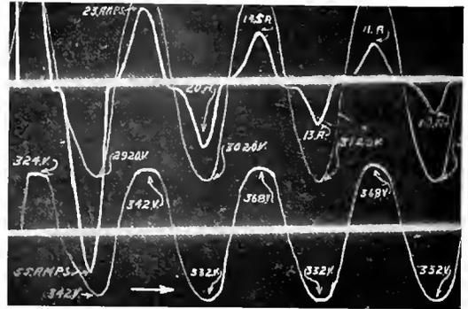
Fig. 22. Charging current and e.m.f. of an aluminum arrester in which the film is only partially formed (see text)
