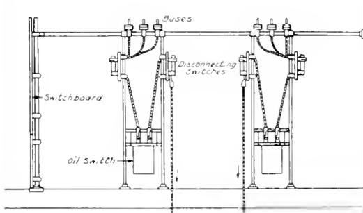
Fig. 6. Arrangement of Switching Apparatus with several sets of Busses
