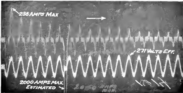
Fig. 28. Oscillographic records of the action of defective aluminum films in a foreign made arrester. An arc occurred between the aluminum plates but was extinguished in the same half cycle (Further description in the text)
