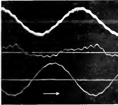
Fig. 17. Charging current in a healthy aluminum arrester with no gap in series (middle curve). The upper and lower curves are voltages on the same circuit. The 13th harmonic is prominent
