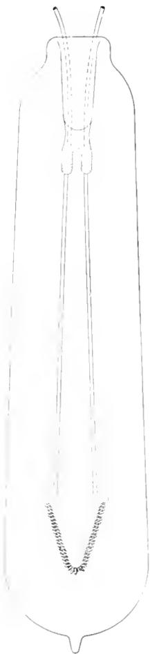
Fig. 1. High Efficiency Nitrogen-Filled Lamp for Low-Voltage Circuit
