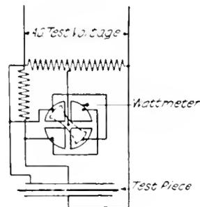
Fig 9 Connections for Electrostatic Wattmeter
