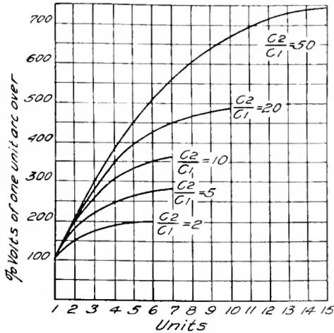
Fig. 11. Arc-over Voltage for Various Numbers of Disc Units for Various Values of  $\frac{C_2}{C_1}$
