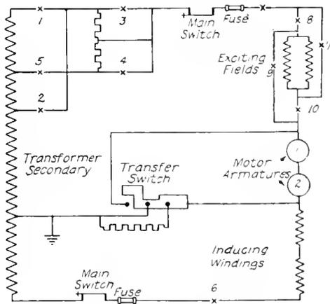
Fig. 1. Diagram of Connections of Single-Phase Traction Motor
