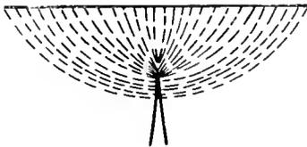
Fig. 5. Concentration of Electrostatic Field at Small Surface
