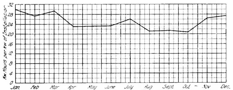
Fig. 4. Current Consumption of Truck Gardeners and General Farmers. 157 Installations. Total Installation 237 Kw., 137 Kw. in Motors, 100 Kw. in Lights. 72,085 Kw-Hours used during the Year
