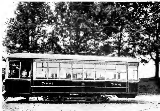
Near Side One-Man Car, International Railway Co., Buffalo, Equipped with Two 32/38 H P. Ventilafed Motors (GE-200)
