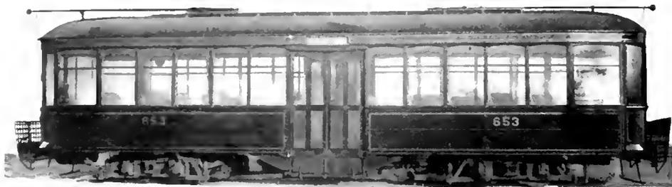
Center Entrance Car, Washington Railways & Electric Company, Equipped with Four 32/38 H.P. Ventilated Motors (GE-200)
