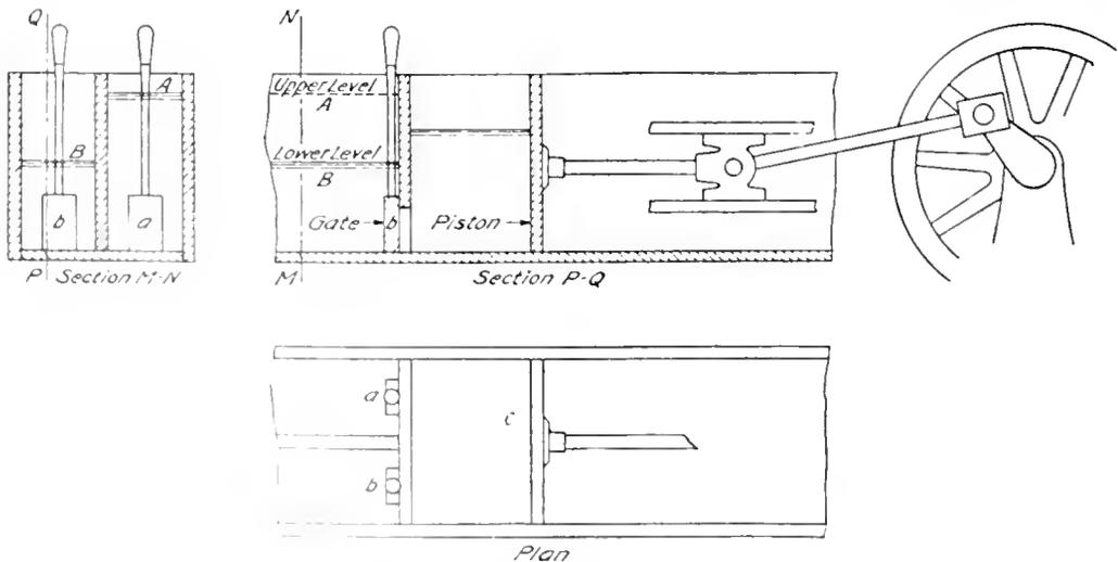
Fig. 2. A Hydraulic Analog to Carnot Cycle
