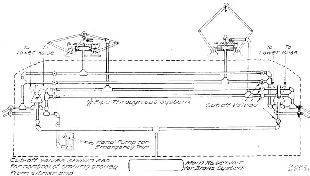
Cut-off valves shown set for control of trailing trolley from either end
