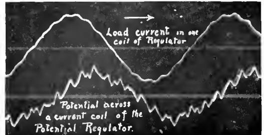
Fig. 10. Potential across a series coil of a potential regulator, the same as used in Fig. 9. The motors were disconnected so that some of the very high harmonics shown in Fig. 9 have disappeared. The 13th and some other higher harmonics are still present
