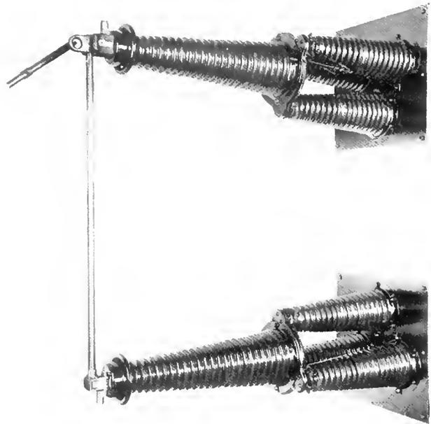
Fig. 5. Built-up Disconnecting Switch for Very High Voltages. All Corners of Current-Carrying Parts Rounded to Prevent Corona. Arc-over Voltage is 500,000 Volts
