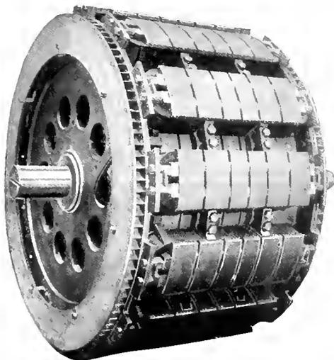
Fig. 5. Rotor of 10,000 Kw. 514 R.P.M. Waterwheel-Driven Generator. The Field Center is Made up of Rolled Steel Plates, Into Which the Pole-Pieces are Dovetailed
