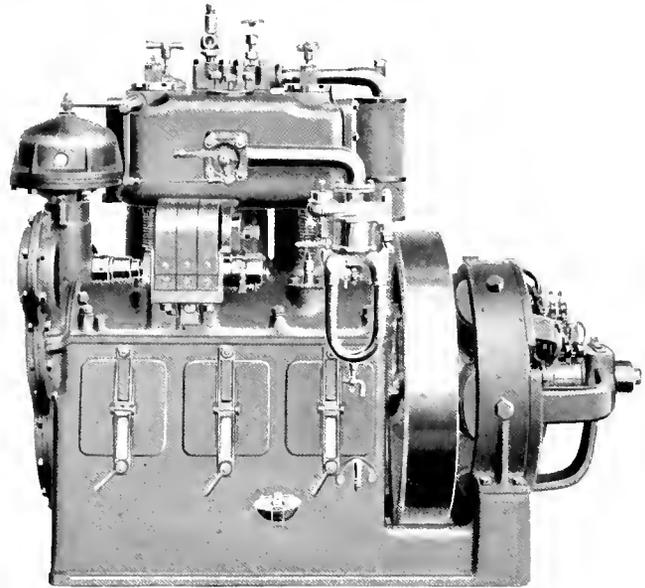
Fig. 10. Small Auxiliary Gasolene Engine and Generator for Furnishing Light, Etc.
