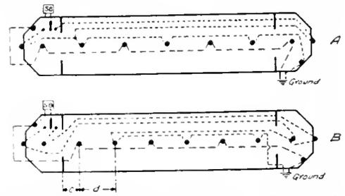
A- Car wired for burning both platform lamps and one marker on each platform, 5 lamps in car body.
