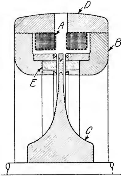
Fig. 2. Partial Section Through High-Frequency Alternator
