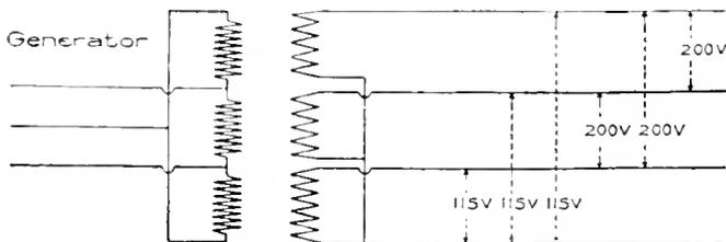
Fig. 3 Three Transformers for Four Wire Three-Phase Distribution
