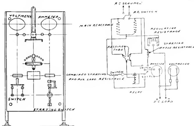
Fig. 18. Ignition Battery Panel Mercury Arc Rectifier
