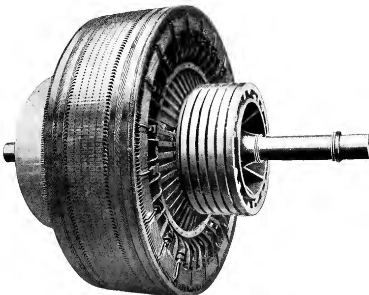
Fig. 1. Armature and Collector Rings of Six-Phase 3000 Kv-a. Railway Converter, Showing the U-Clamps for Equalizer Connections
