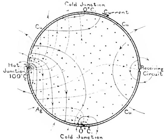
Fig. 3 Energy Flow Near a Thermo-Electric Circuit
