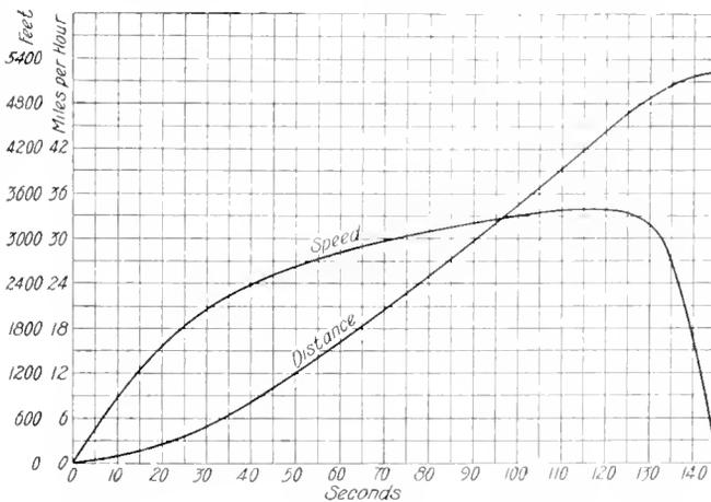
Fig. 5. Service Condition (speed and distance) During Acceleration
