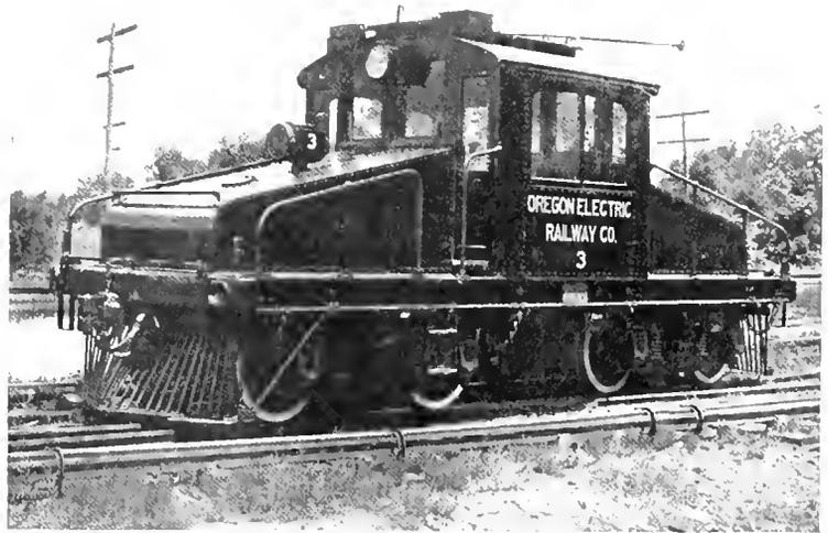
Fig. 2. 50-Ton Locomotive, Oregon Electric Railway Company
