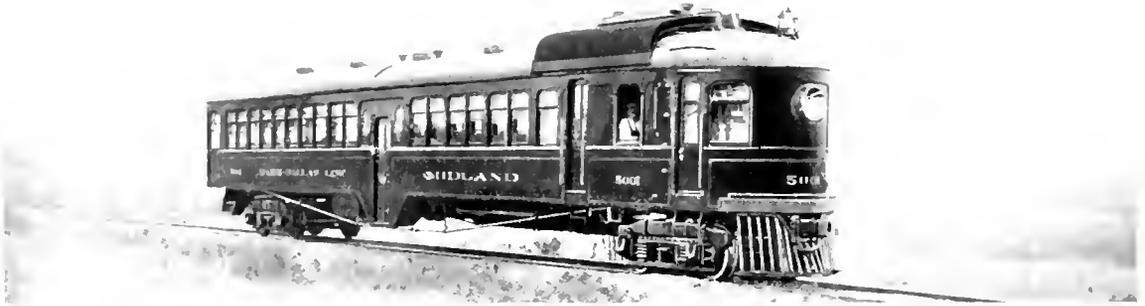
Fig. 1. Combination Passenger and Baggage Gas-Electric Motor Car on the Texas Midland Railroad. This car is 70 ft. long and is provided with both center and rear entrance
