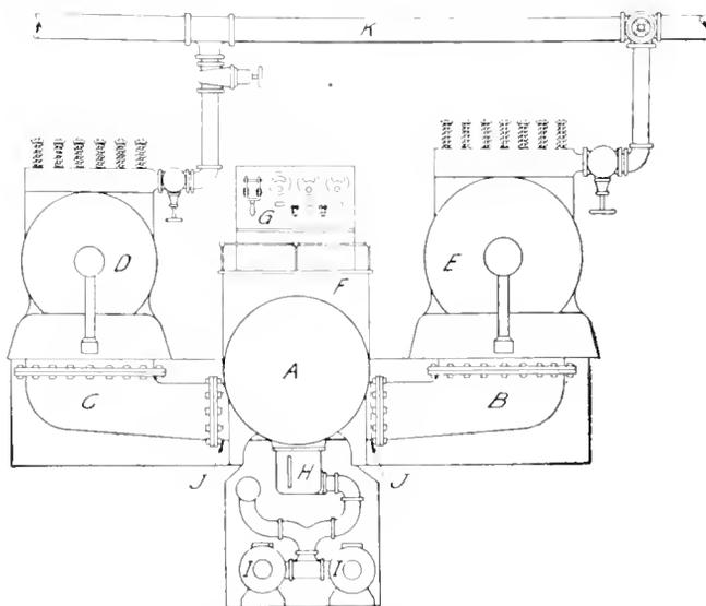
Fig. 4. General Arrangement of Turbines, Condensers, Switchboard, Piping, etc., as Followed in Water-Rate Tests
