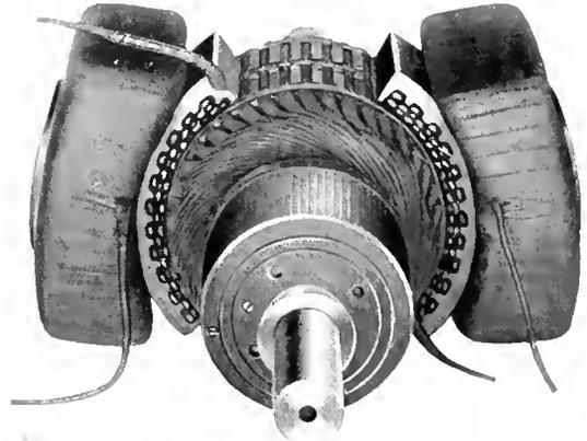
Fig. 1. D-C. Armature, A-C. Pole Face Winding and D-C. Field Coil of a 2000 Cycle Converter
