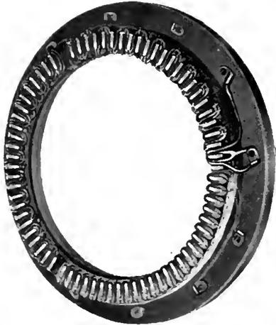
Fig. 9. Stationary Field and Armature of Single-Phase Telephone Relay
