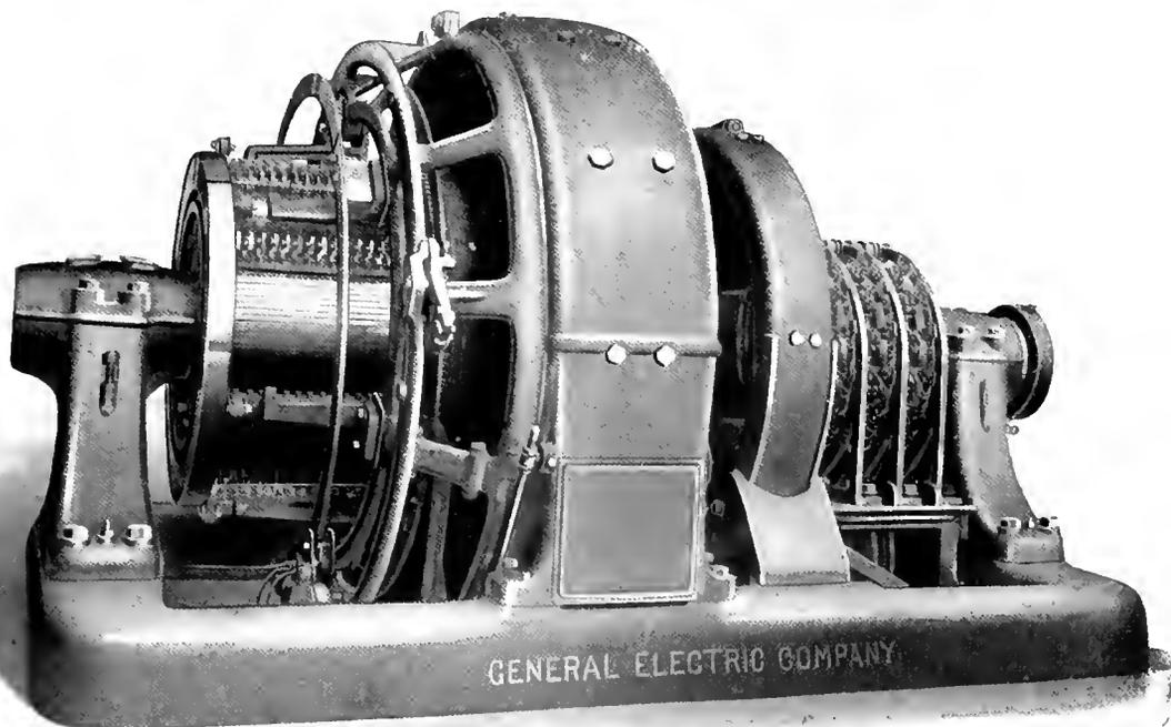
Fig. 5. 1000 Kv-a. Converter with Revolving Armature A-C Booster. The commutator cooling vanes of this machine (already shown in detail in the frontispiece on page 278) are here covered
