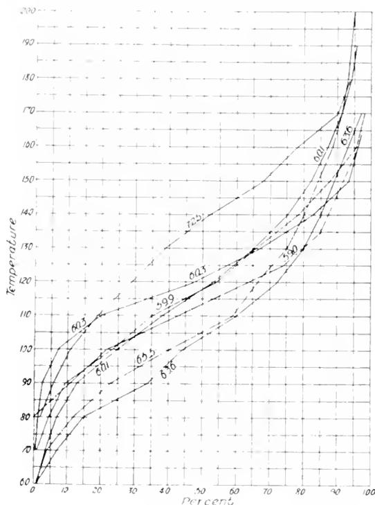
Fig. 1. Curves of Fractional Distillation of Gasolenes of Various Specific Gravities and Widely Differing Fuel Values
