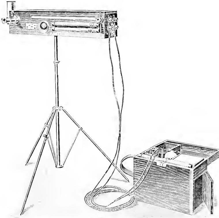
Fig. 3 a. Complete Sharp-Millar Photometer with Supply Battery
