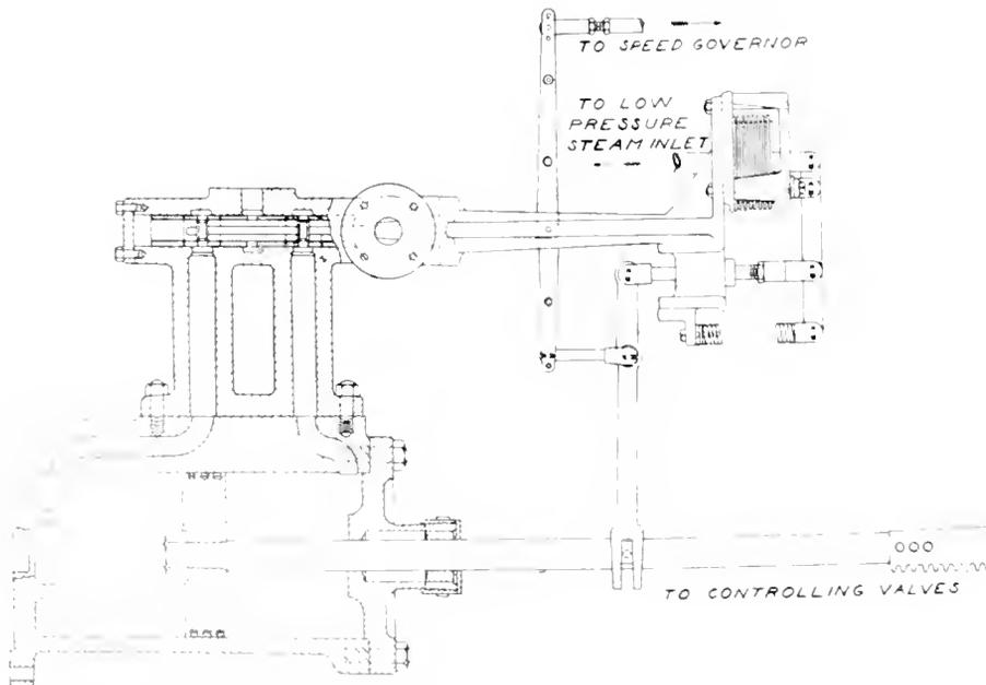
Fig. 6. Device for Automatically Opening and Closing High Pressure Valves with Variations in Supply of Low Pressure Steam
