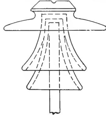
Fig. 6. Three-Part Pin Insulator
