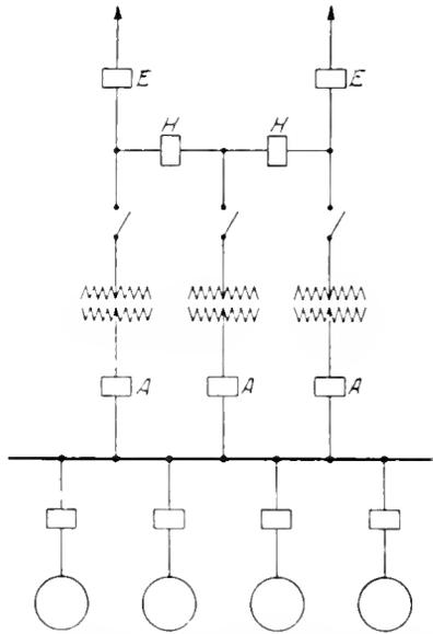
Fig. 4. Connections for three banks of transformers feeding two transmission lines. Transformers paralleled on low tension and high tension sides
