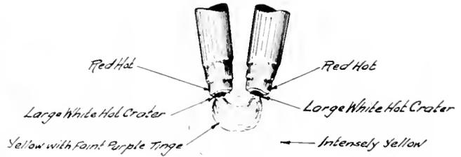
Fig. 12. Alternating Current Open Flame Arc. Converging Electrodes
