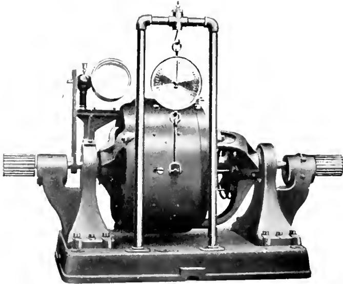
Fig. 6. Electric Dynamometer for Chassis Test
