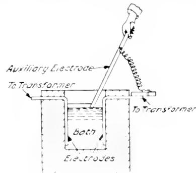
Fig. 15. Method of Starting Furnace
