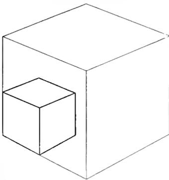
Fig. 10. Diagrammatic Representation of the Volumetric Space Required by an American Arrester (small cube) Contrasted with that Required by the Equivalent European Arrester (large cube)
