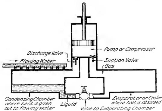
Fig. 1. Diagram of a Compression-Type Refrigerating System
