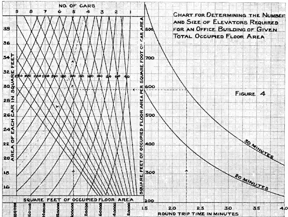
Fig. 4. Chart for Determining the Number and Size of Elevators Required for Office Buildings of Given Total Occupied Floor Area
