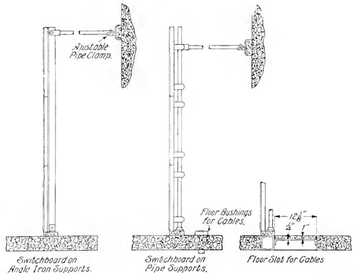
Fig. 1. Method of Mounting Standard Switchboards, Using Angle Iron or Pipe Supports and Wooden Sills
