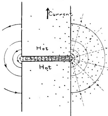
Fig. 2. Energy Flow at a Thermo-Electric Junction
