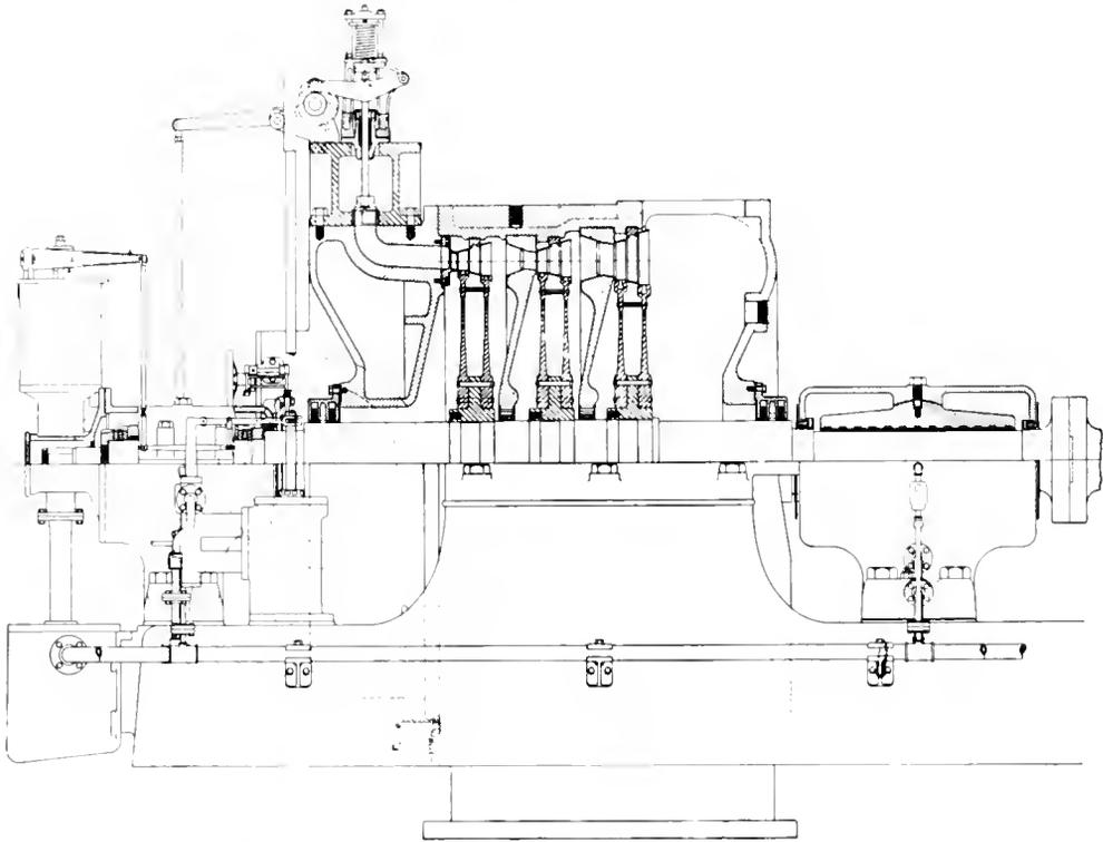
Fig. 3. Mixed Pressure Turbine Designed Primarily for Low Pressure but which will Operate with Fair Efficiency on High Pressure
