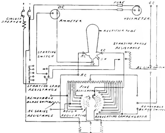
Fig. 15. Private Garage Panel With Mercury Arc Rectifier
