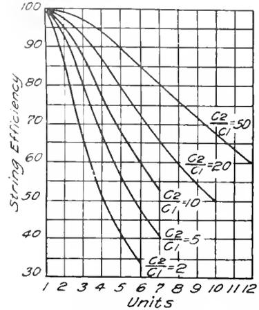
Fig. 12. String Efficiency of Various Numbers of Units for Various Values of  $\frac{C_2}{C_1}$
