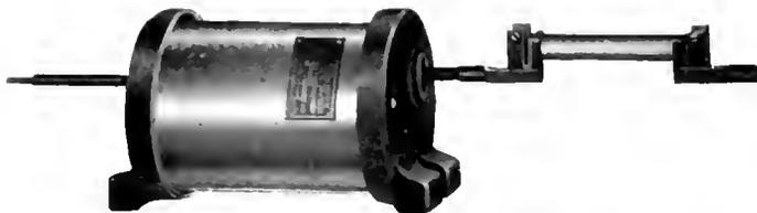
Fig. 2. The Magnetic Blowout Arrester for High Voltage D-C. Circuits. The gap setting is the minimum consistent with a reasonably large rate of current discharge. A permanent magnet is used, blowing the arc through a quenching arc-chute. The resistance is placed externally to facilitate inspection
