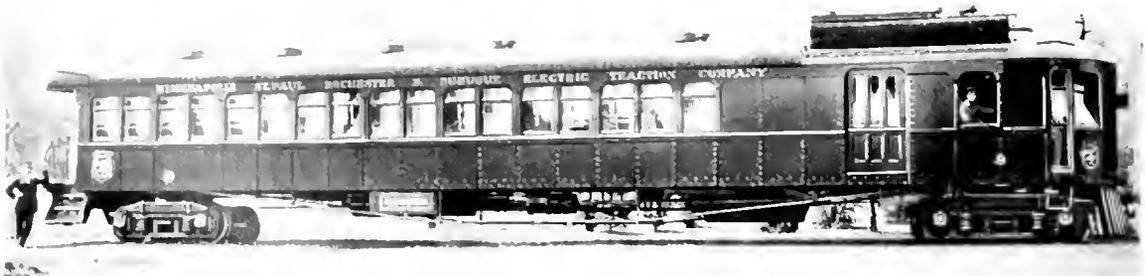
Fig. 4. Combination Passenger and Baggage Gas-Electric Motor Car Operating on the Minneapolis, St. Paul, Rochester & Dubuque Railway, commonly known as the Dan Patch Line. This car is 70 ft. long and has rear entrance
