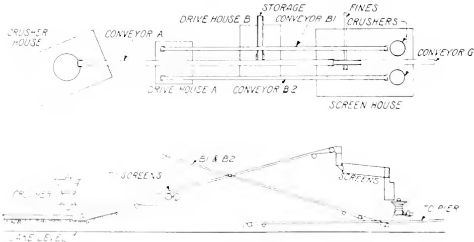
Fig. 2. Plan and Elevation Showing Relative Positions of Crushers, Screens and Conveyors Between Main Crusher House and Shore Line
