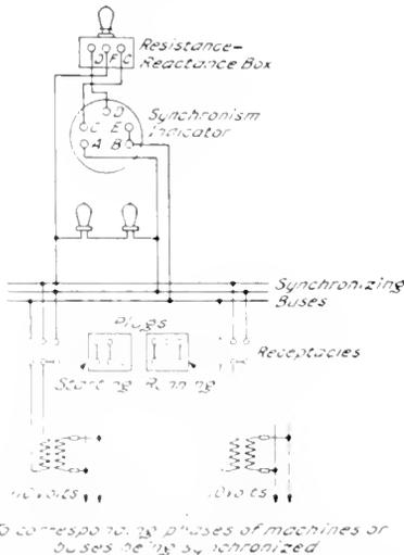
Fig. 5. Connections of Synchronism Indicator with Ungrounded Secondaries on Potential Transformers
