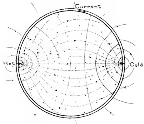
Fig. 1. Energy Flow Near a Thermo-Electric Circuit
