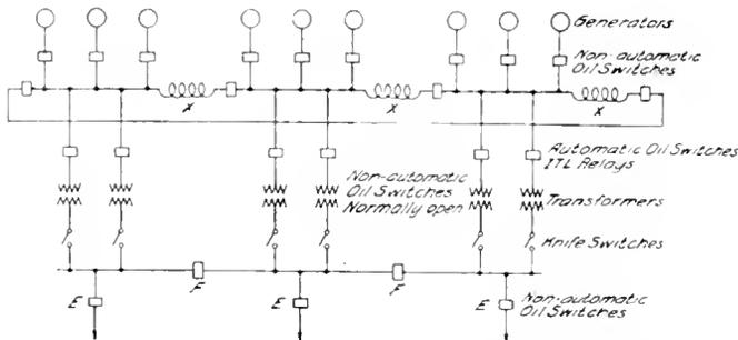
Fig. 1. An arrangement for paralleling high-tension transformers on the low tension side. The ring bus is sectionalized by bus-section switches, which permit of isolating any section without disturbing the operation of the remaining units. Current limiting reactances are also inserted to prevent excessive rushes of current at times of short circuit
