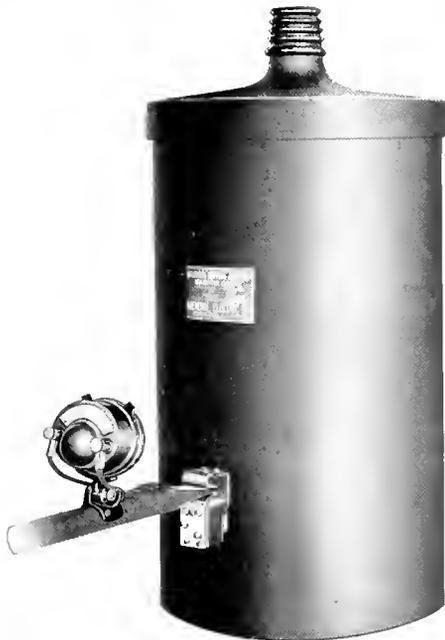
Fig. 23. Method of Using Charging Current Indicator
