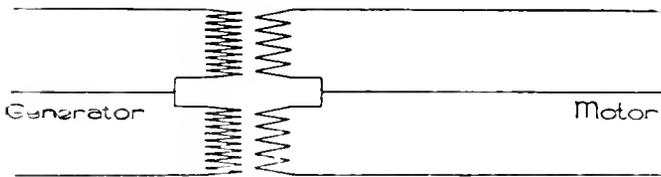
Fig. 2 Two Transformers for Three-Phase Transformation
