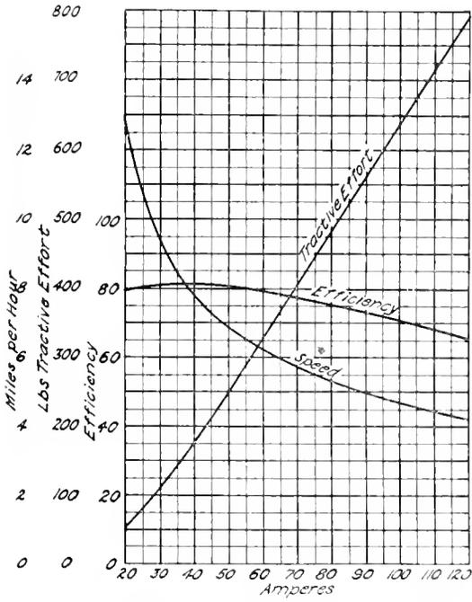
Fig. 1. Characteristic Curve of GE-1022 Motor on 85 Volts. Gear Reduction 6.21 to 1, Wheel Diameter 30 In.
