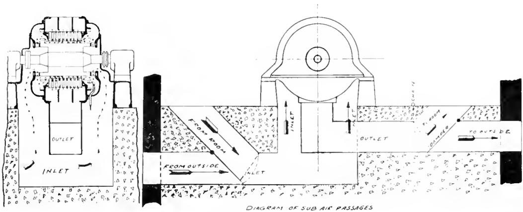
Fig. 2. Diagram of External and Internal Air Passages of a Horizontal Shaft Steam Turbine Alternator
