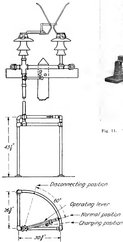
Fig. 10. Horn Gap and Operating Stand for High Voltage Arresters
