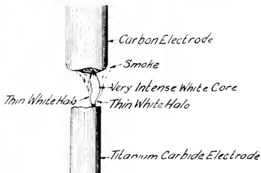
Fig. 11. Alternating Current Luminous (Titanium) Arc
