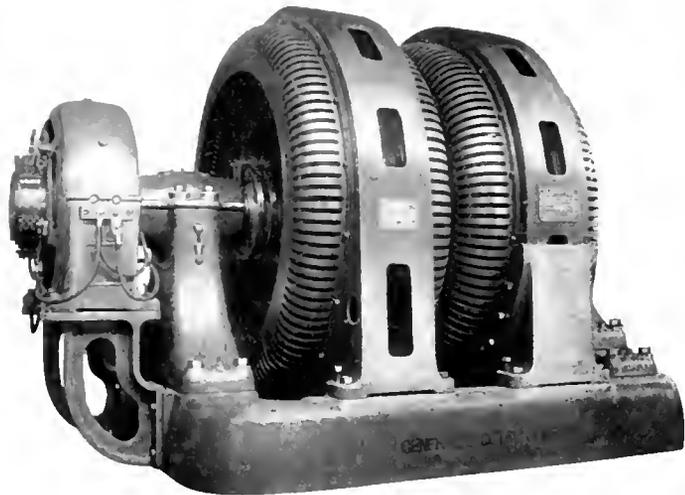
Fig. 1. 1000 Kw. Frequency Changer Set and Exciter
