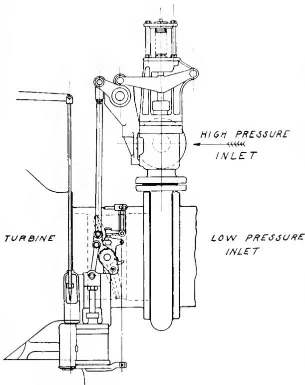
Fig. 2. Governor Operated Reducing Valve for Automatically Admitting High Pressure Steam in a Low Pressure Header
