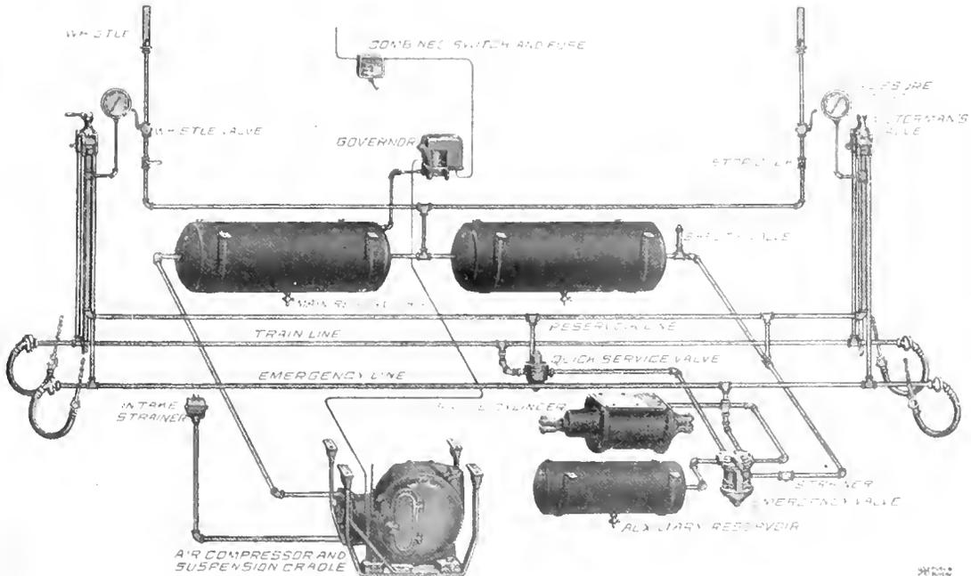
Fig. 2. Emergency Straight Air Brake Equipment for Motor Car
