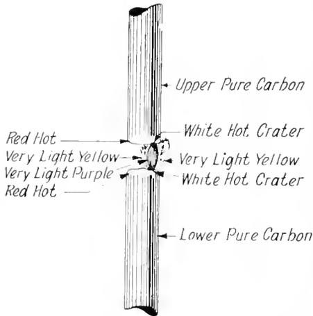
Fig. 7. Alternating Current Enclosed Arc
