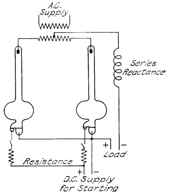
Fig. 8. Mercury Arc Lamps Connected to Act as Rectifiers
