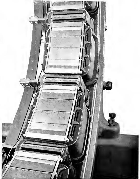
Fig. 8. Pole Face and Commutating Field Connections of Converter Shown in Fig. 6
