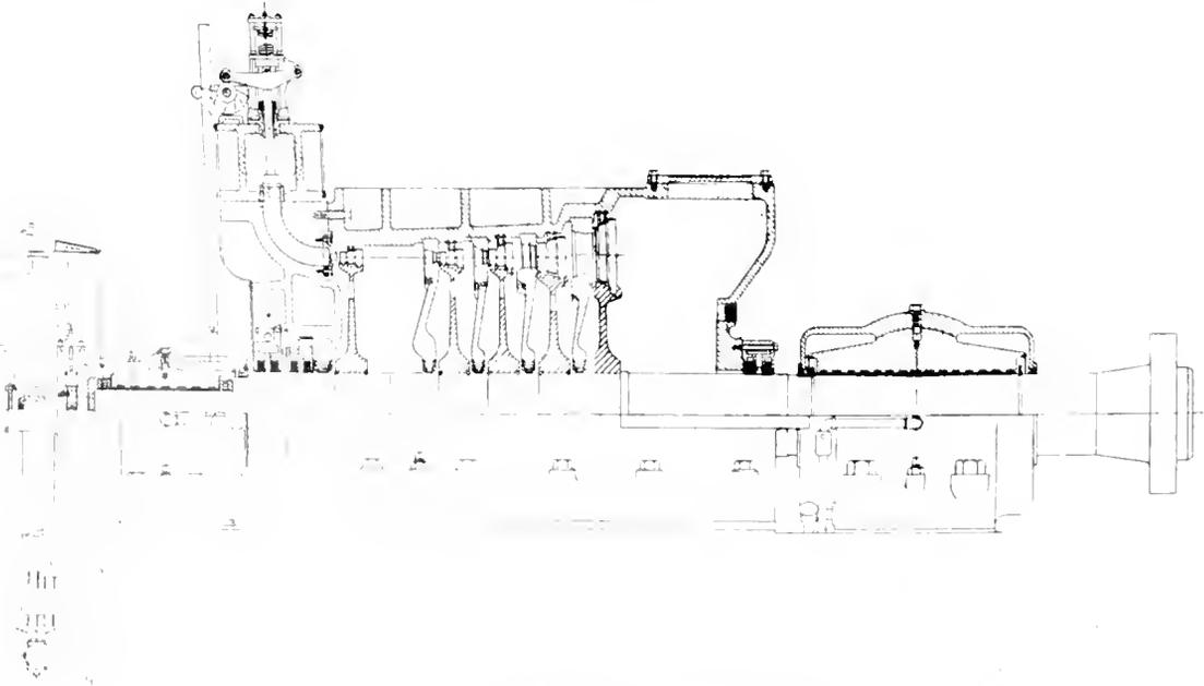
Fig. 4. Mixed Pressure Turbine — A Compromise Between High and Low Pressure and can Operate Exclusively on Either
