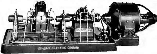
Fig. 5. 2 Kv-a. 100,000 Cycle Alternator Driven Through Single-Reduction Gearing by Direct Current Motor
