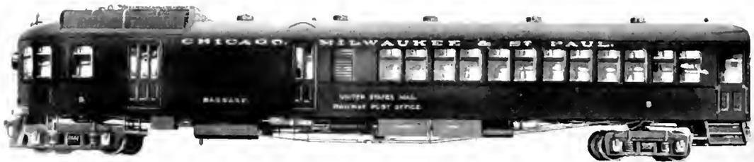
Fig. 3. Combination Passenger, Baggage and Mail Gas-Electric Motor Car Operating on the Chicago, Milwaukee & St. Paul Railroad. This car is 70 ft. in length and is provided with rear entrance
