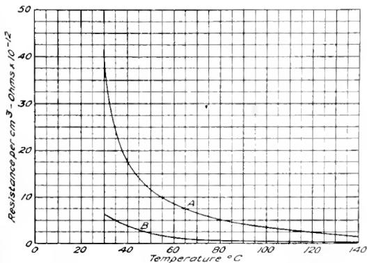
Fig. 1. Insulation Resistance of Transformer Oil
