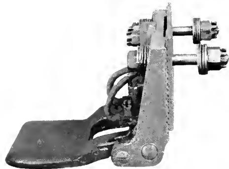
Fig. 20. Side View Under-Running 3rd Rail Collector
