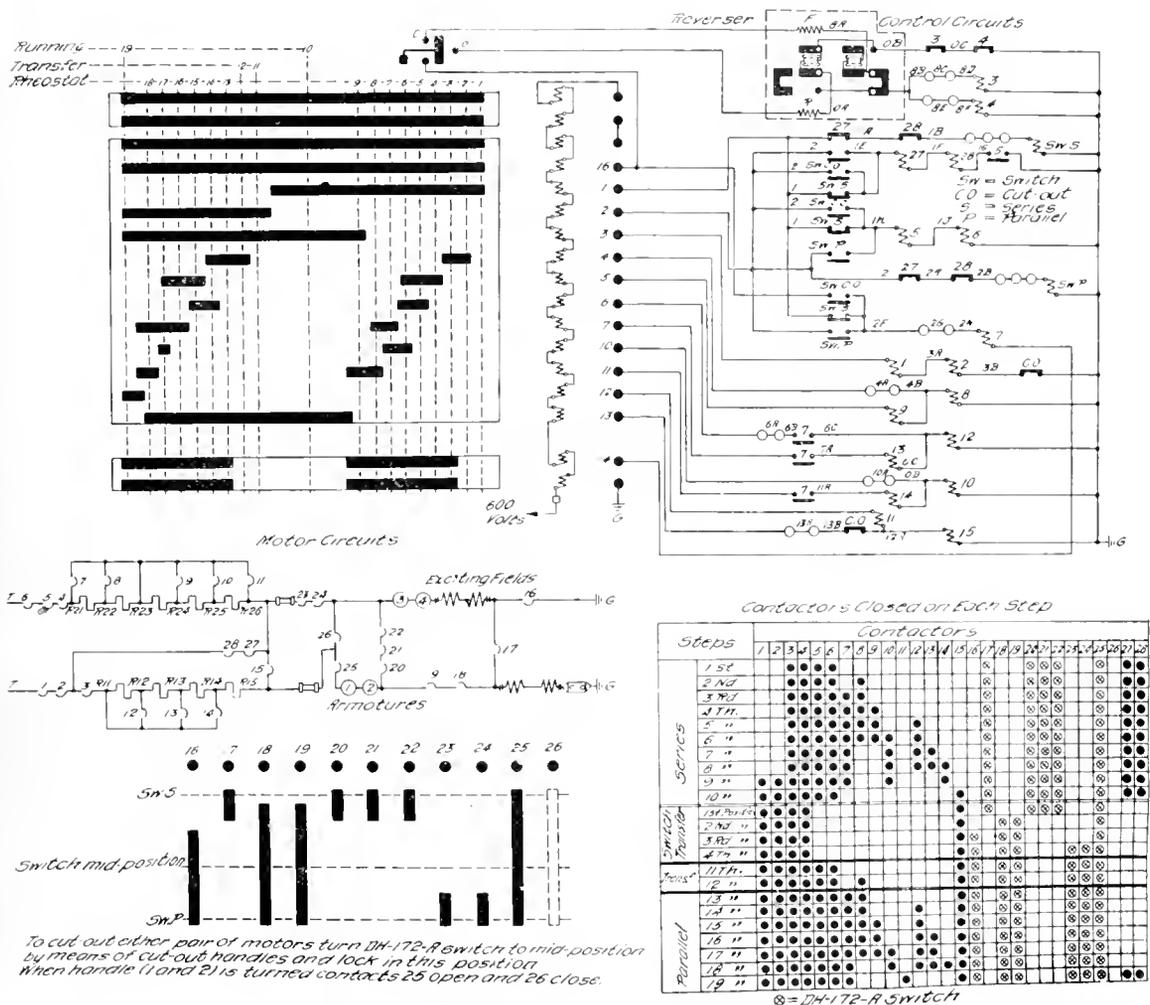
Fig. 20 Simplified Connections with C 93 Controller, 2400 Volt Trolley
