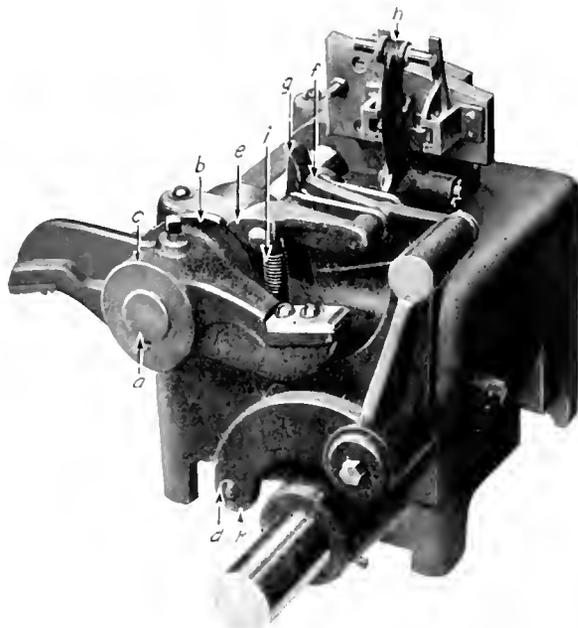
Fig. 2. Locking mechanism - at half stroke
