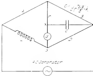
Fig 8 Connections for Anderson Bridge
