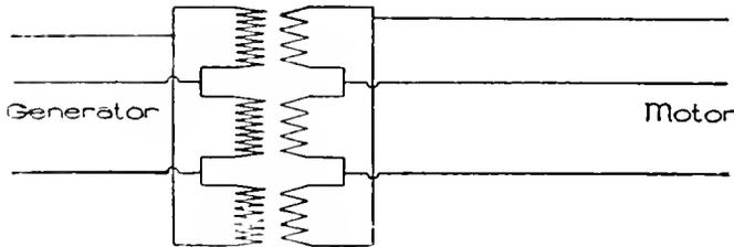
Fig. 1 Three Transformers for Three-Phase Transformation
