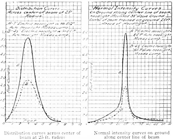
Fig. 6. Curves Showing Characteristics of Beam Projected from a 7-Inch and a 4 1/2-Inch Electric Headlight, Employing Parabolic Reflectors
