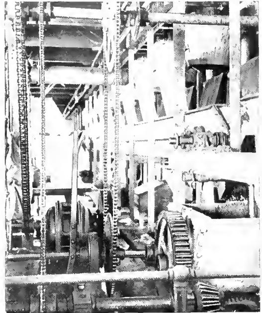
The 15 h.p., 900 r.p.m. induction motor shown above performs a variety of services in handling the sugar. Through back-gearing, a chain drive, and various bevel gears and friction sprockets, it operates a sugar conveyor, massecuite conveyor, sugar mixer, etc.
