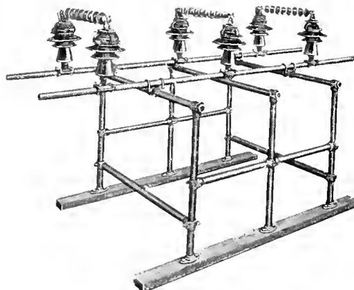
Fig. 10. High-Tension Fuse for Horizontal Mounting, 20 Amperes Capacity, for Outdoor Service on 35,000 Volts
