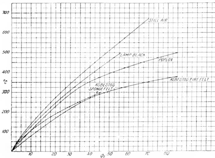
Fig. 2. Relation Between Temperature and  $\phi$ .  $\phi = \int_0^t \kappa dT$
