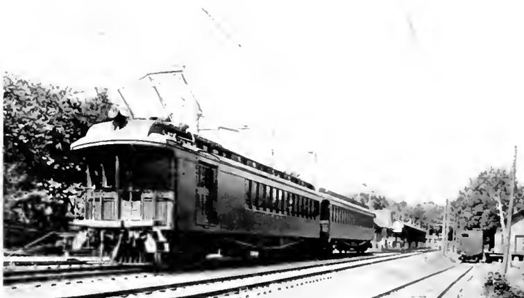
Fig. 11. View Showing Two-car Train, One Being a Motor Car Equipped with Single-Phase Motors
