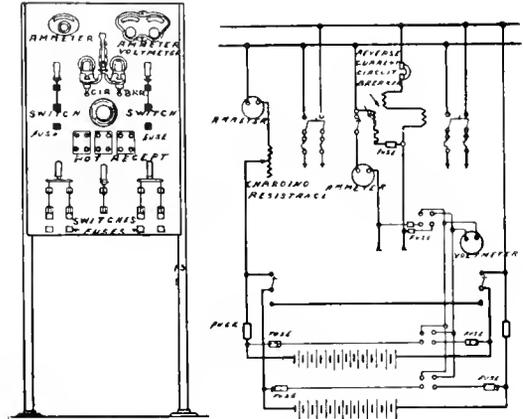
Fig. 11. Switchboard Panels for Batteries in Small Isolated Lighting Plants
