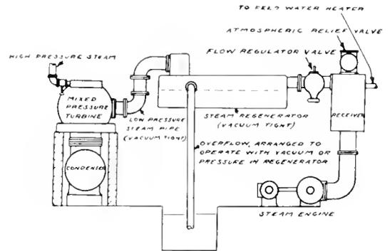
Fig. 8. Diagram Showing Flow Regulator Valve Installed Between Engine and Regenerator
