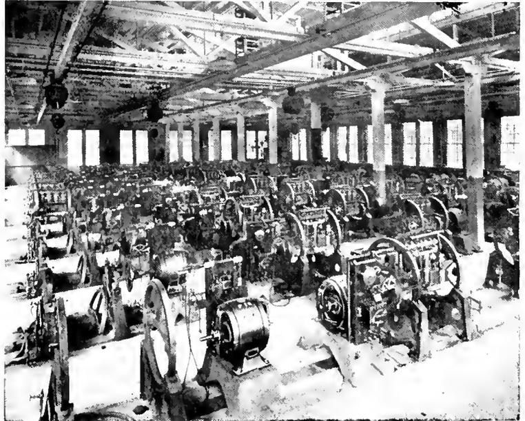
Fig. 8. Engine Testing Dynamometer, Cadillac Company, Detroit
