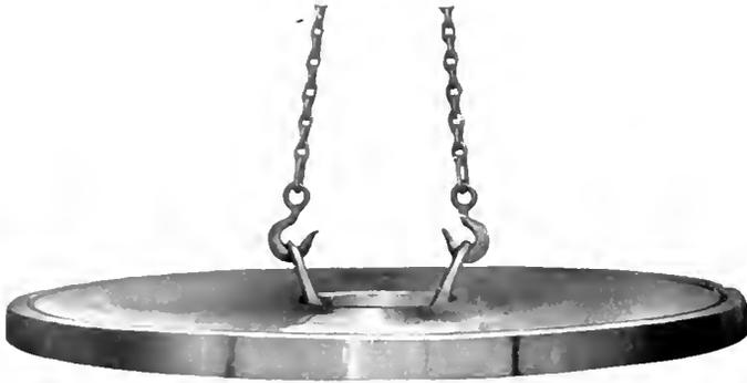
Fig. 24. Improper Use of Double Hook
