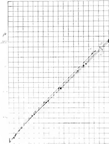
Fig. 1. Reluctivity Curves of Three Samples of 3.5 Per Cent Silicon Steel
