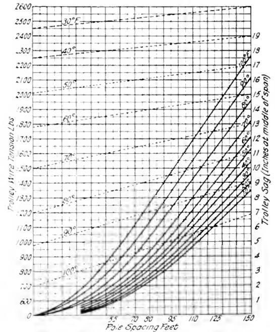
Fig. 3. Relationship Curves for a Particular Trolley Wire
