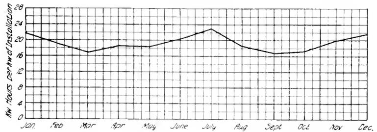
Fig 3 Current Consumption of Truck Gardeners, using Pumps for Garden and Greenhouse Water Supply. 60 Installations. Total Installation 88.6 Kw., 58 Kw. in Motors, 30.6 Kw. in Lights. 20,412 Kw-Hours used during the Year
