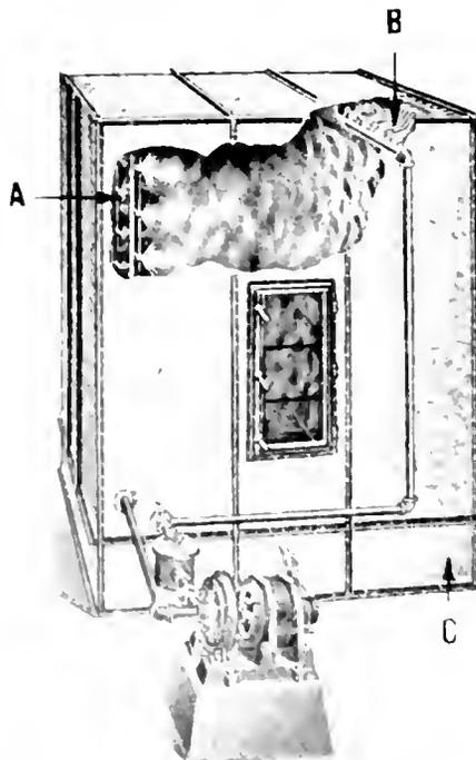
Fig. 4 External View of Circulating Pump and Humidifier With Part of Outside Casing Removed
