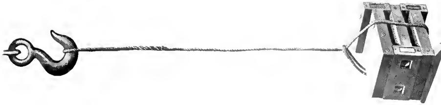
Fig. 17. Single Cable Sling
