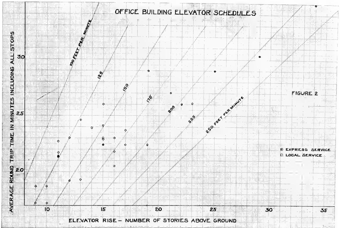
Fig. 2. Curves Showing the Average Round-Trip Time and the Average Speed, including all Stops, of Elevators in Office Buildings of Different Heights
