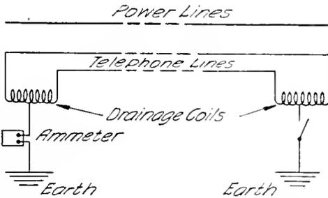
Fig. 8. The general scheme of connections of the oscillograph to the telephone circuit to obtain the oscillograms of Figs. 4, 5, 6 and 7
