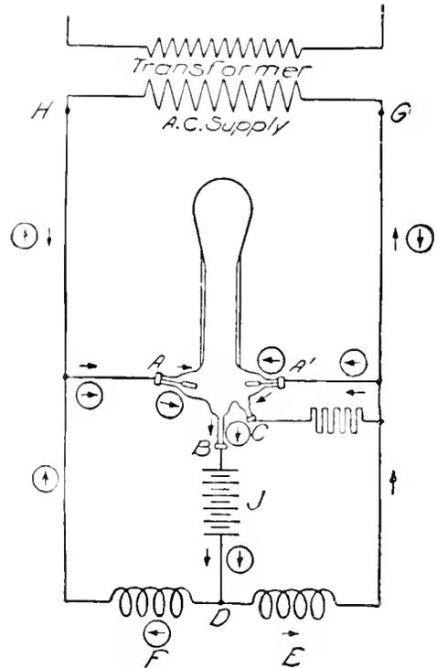
Fig. 12. Diagram of Connections for Constant Potential Rectifier
