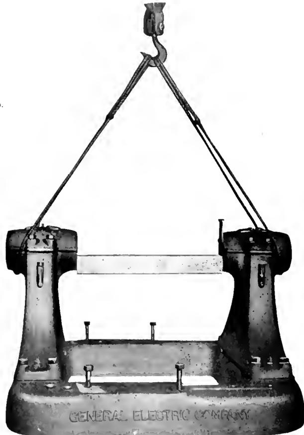
**Fig. 29. Lifting a Base with Standards**
