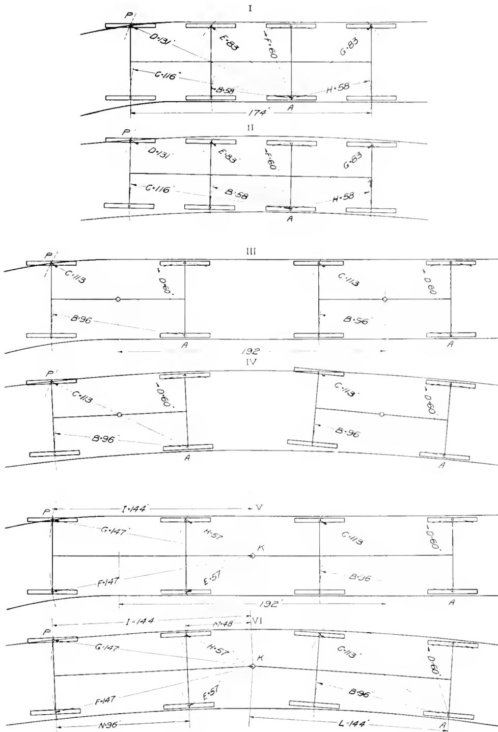
Figs. 1-6. Diagrams of Various Truck Arrangements, Showing Points of Application of the Forces Developed in Taking Curves
