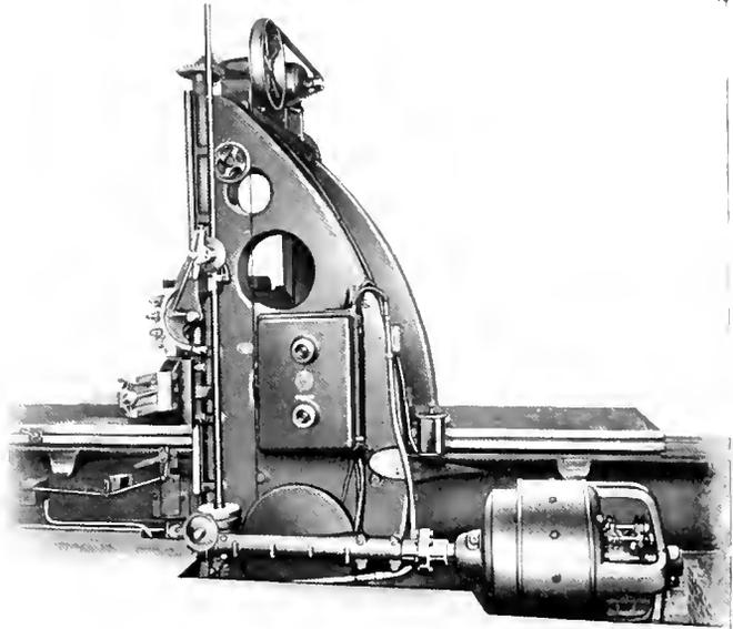
Fig. 10. Planer shown in Fig. 9 re-equipped with a 250/1000 r.p.m. Direct Connected Reversing Motor
