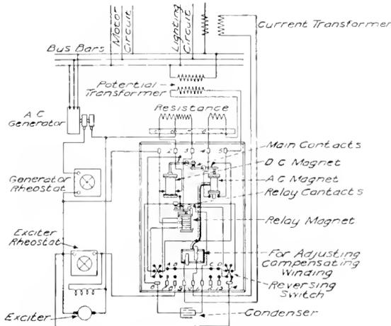
Fig. 1. Connections of Automatic Voltage Regulator for Use with Synchronous Condenser in Transmission Systems
