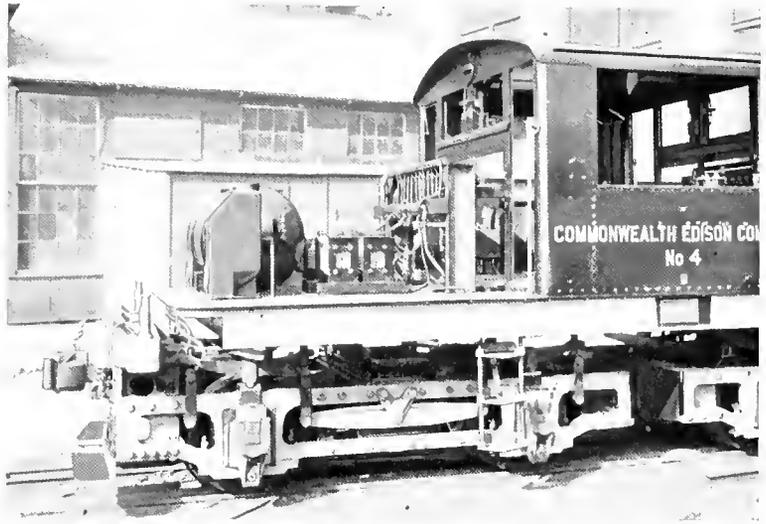
Fig. 15. 75-Ton Locomotive with End Cab Removed, Showing Auxiliary Apparatus
