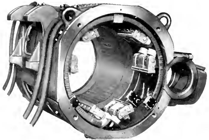
Fig. 8. Frame and Field of Single-Phase Railway Motor
