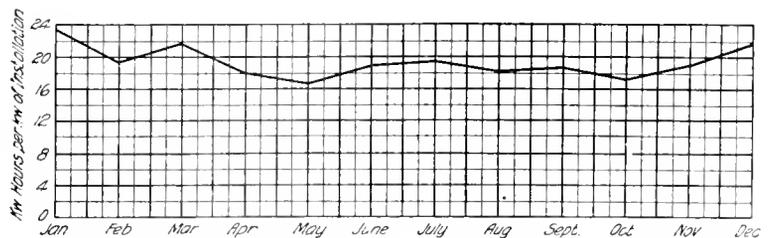
Fig. 6. Composite of Curves 2 to 6 inclusive. Total Installation 725 Kw., 525 Kw. in Motors, 227 Kw. in Lights. 175,755 Kw-Hours used during the Year
