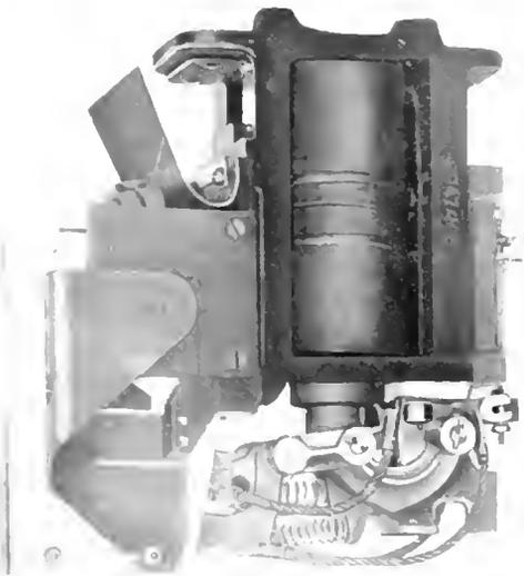
Fig. 11. Low Voltage Contactor
