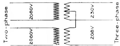
Fig. 5. Two-Phase to Three-Phase Transformation
