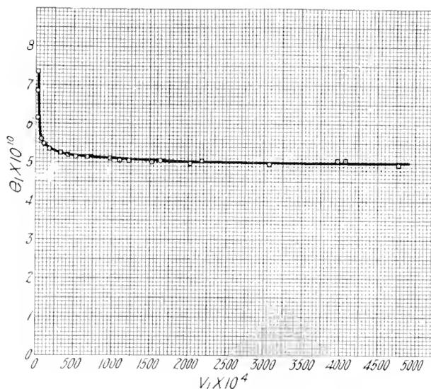
Fig. 1. Curve Showing Relation Between Charge ( $E_1$ ) and Velocity of the Drop ( $V_1$ ) Obtained by Applying the Equation (2)
