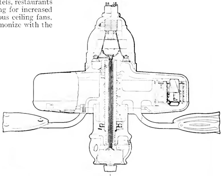
Fig. 4. Sectional View of Alternating Current Fan
