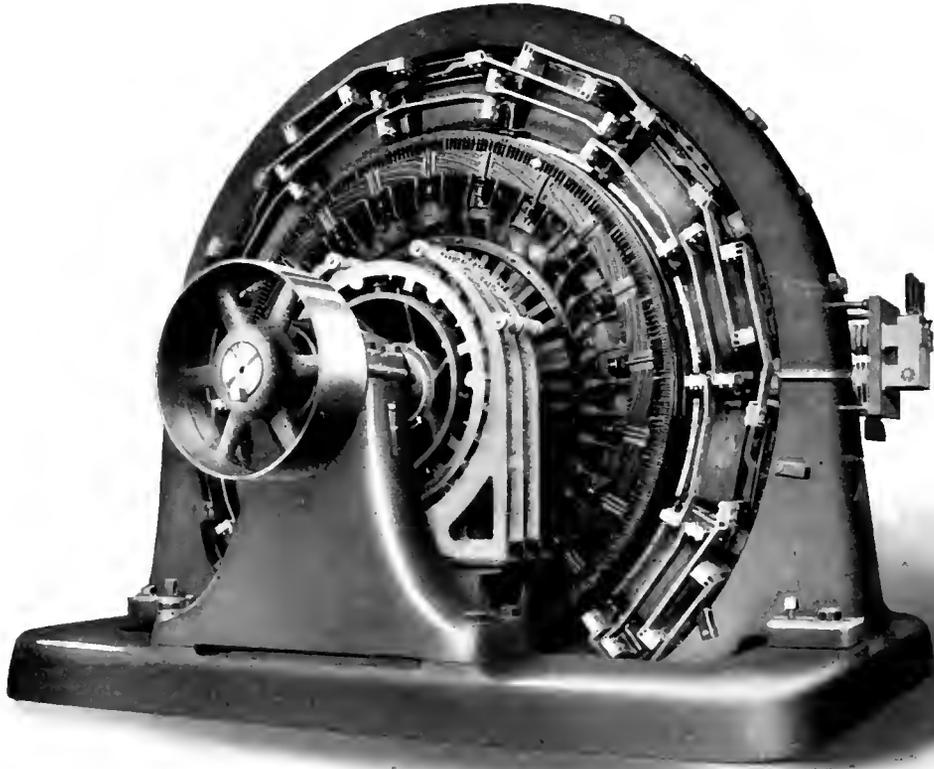
Fig. 6. 3000 Kv-a. Compound Wound Commutating Pole Railway Converter, 300 R.P.M., 600 Volts. The field connections of this machine are explained in the text. The pulley, it need hardly be explained, is on the shaft purely for testing purposes
