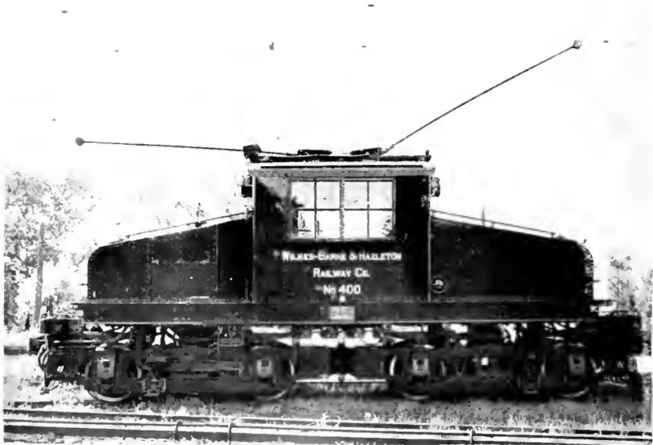
Fig. 7. A 60 Ton Articulated Truck Locomotive
