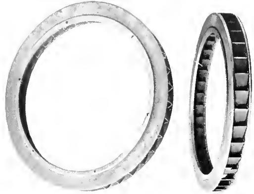
Fig. 7. Fans for Rotor of Turbine-Driven Alternator
