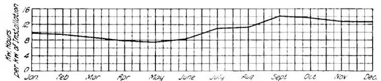
Fig. 5. Current Consumption of Farmers using Electricity for Lighting only. 41 Installations. Total Installation 73 Kilowatts 9,382 Kw-Hours used during the Year
