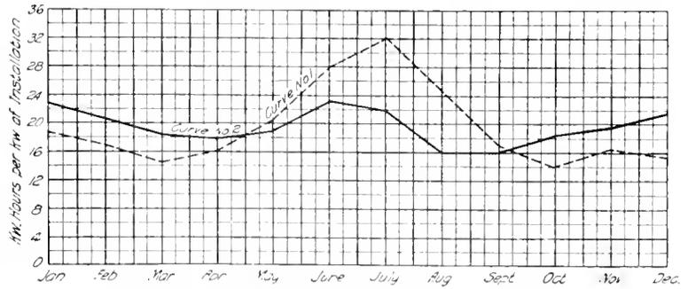
Fig. 10. Curves showing the Difference in Current Consumption of a strictly Pumping Load, as compared with a Load consisting of 62% Pumping and 38% Lighting. Curve 1, Pumping only. Curve 2, 38% Lighting, 62% Pumping
