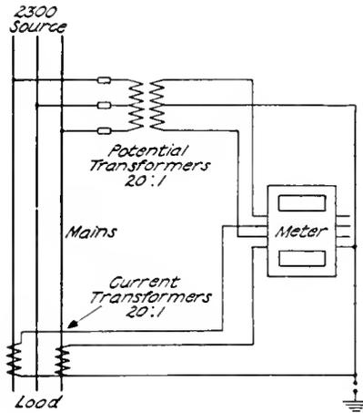
some arrangements of wiring or other local conditions, this is not sufficient and 110-volt single gap arresters are required between the two outside wires on the low-tension side of the potential transformer and ground. The gap in the common ground connection of the meter wiring is contrary to good practice. This point should be dead grounded.
