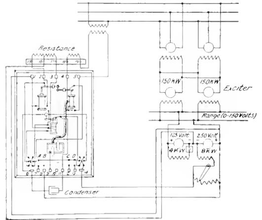
Fig. 2. Connections of Synchronous Condensers, Combination of Exciters, and Automatic Voltage Regulator, for Use on Transmission Lines Having a Heavy Charging Current. The Arrangement Provides a Range of Excitation on the Condenser from Zero to 250 Volts
