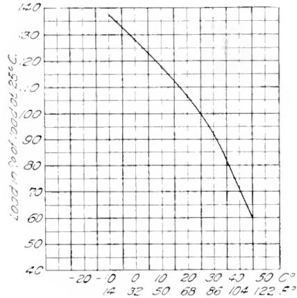
Fig. 5. Permissible Load on a Turbo-Alternator as a Function of the Temperature of the Ingoing Air
