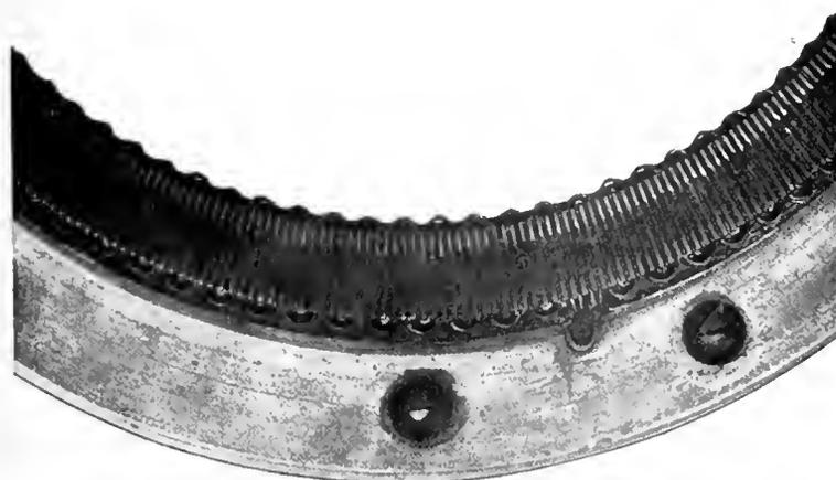
Fig. 8. Special Winding for 100,000 Cycle Alternator, with 400 Slots
