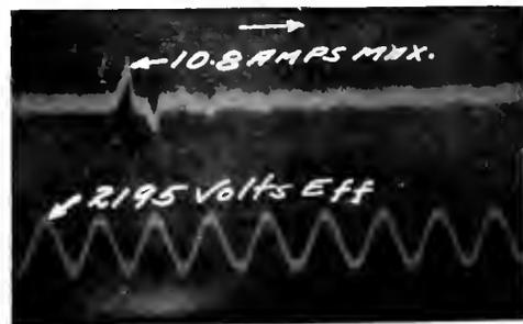
Fig. 20. Normal charging current, through an arc, of an aluminum arrester
