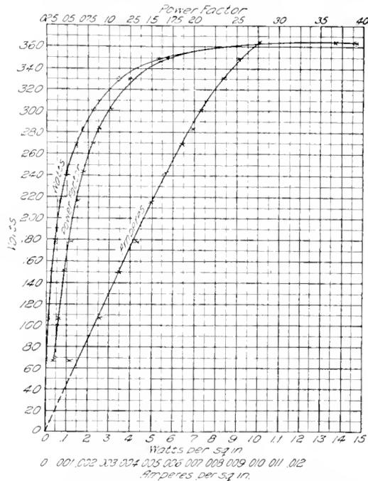
Fig. 1. The relation of the impressed voltage on an aluminum cell to each of the following factors: Watts per square inch of aluminum film; amp. per square inch of aluminum film (numbers at the bottom of the cut); and power-factor (numbers at the top of the cut)
