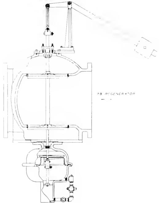
Fig. 5. Flow Regulating Valve
