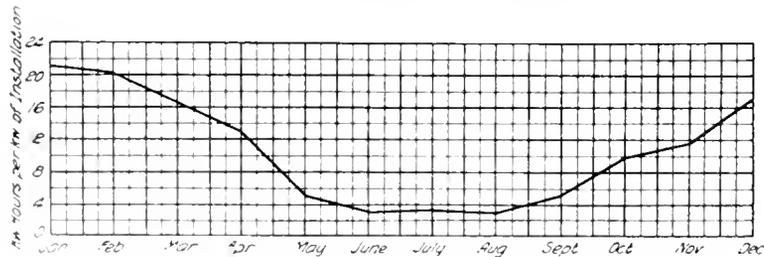
Fig. 2. Current Consumption on Dairy Farms using Feed Grinders, Huskers and Shredders, but not using Refrigerating Machines. Total Installation 302 Kw., 284 Kw. in Motors, 18 Kw. in Lights. 38,150 Kw-Hours used during the Year
