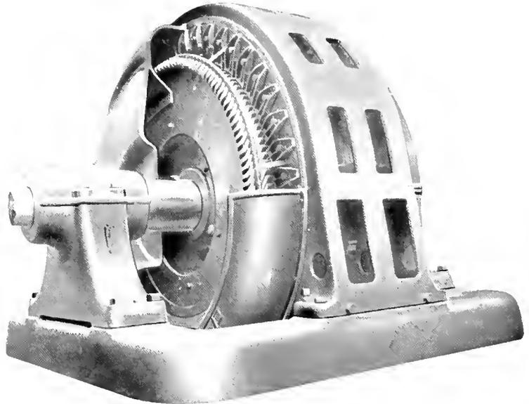
Fig. 4. A 7000 Kw., 11,000 Volt Generator, ventilated by air drawn from the pit and expelled into the room through holes in the frame
