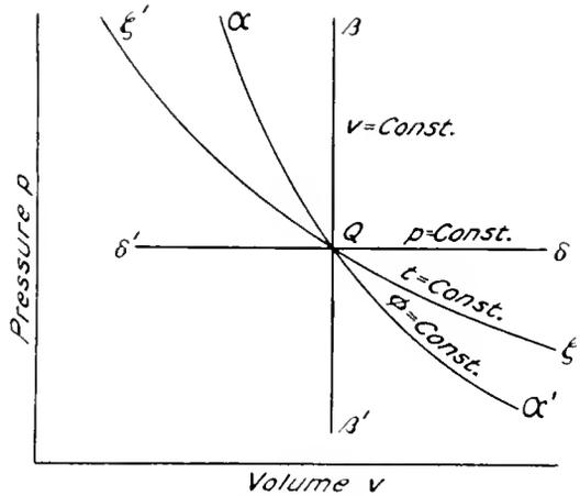
Fig. 6. Thermodynamic Changes in a Perfect Gas Represented in Terms of its Volume and Pressure
