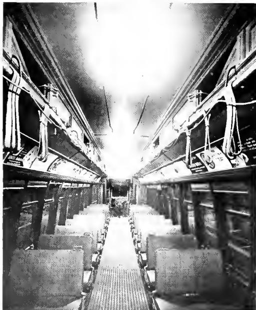
Fig. 1. Interurban Car Illuminated by Mazda Lamps
