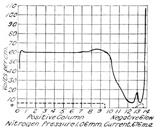
Fig. 4. Distribution of Potential Gradient in Geissler Discharge
