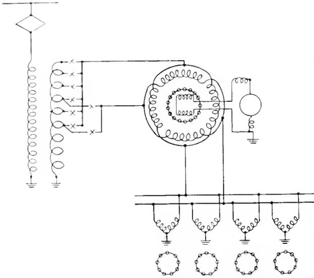
Fig. 2. Wiring Diagram of Split Phase Locomotive
