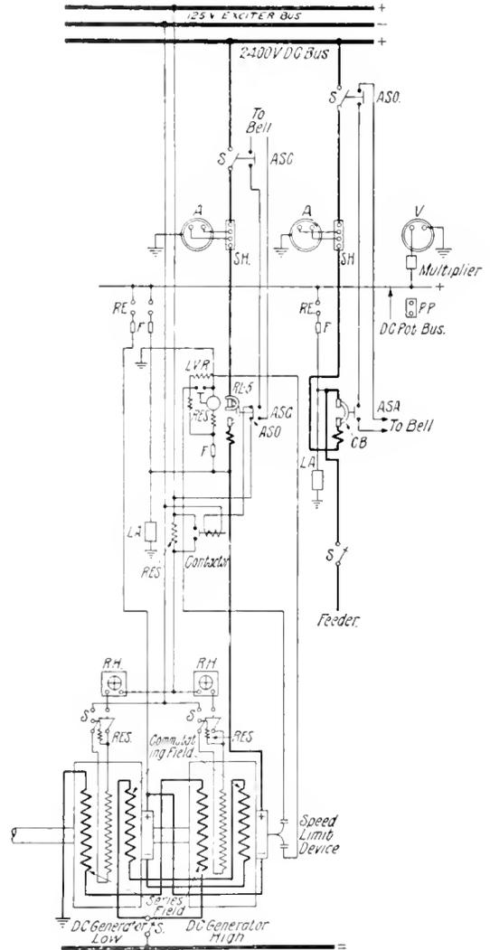
Fig. 1. Diagram of Connections, 2400 Volt D-C. Switchboard
