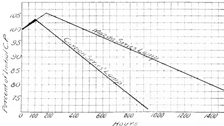
Fig. 2. Variation in Candle-power During Life of Tungsten Series and Carbon Series Lamps
