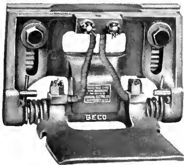
Fig. 19. Front View Under-Running 3rd Rail Collector
