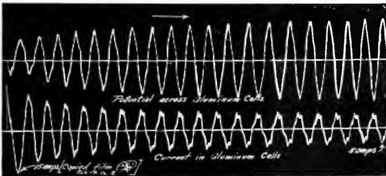
Fig. 21. The current and potential of 33 kv. arrester after the films had stood six weeks in electrolyte without charging. This oscillogram shows the valuable function of charging resistance. A fuller analysis is given in the text
