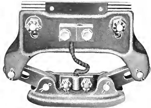
Fig. 14. Gravity 3rd Rail Collector, Front View
