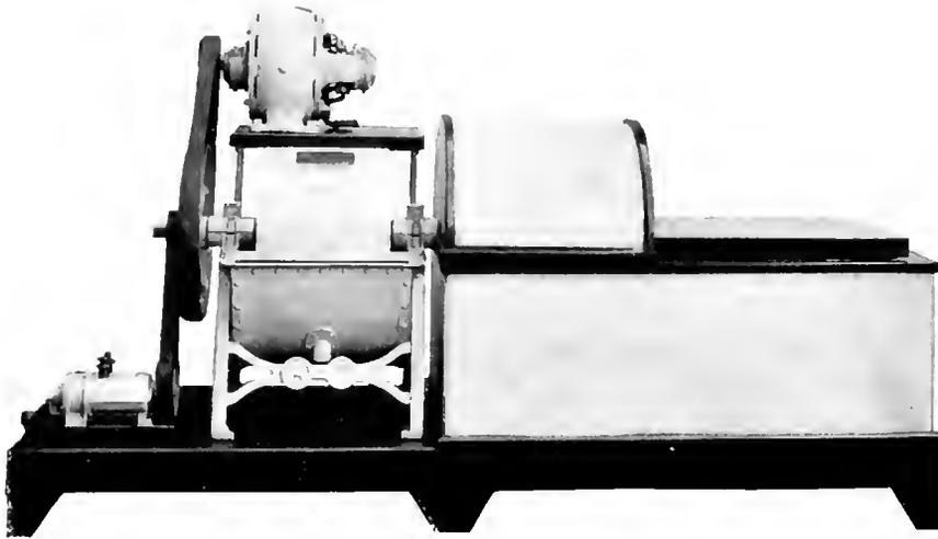
Fig. 12. Motor-Driven Compression Refrigerating Machine, Audiffren-Singrun Type
