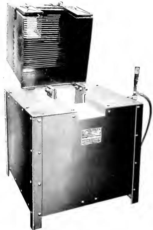
Fig. 1. Electric Hardening Furnaces
