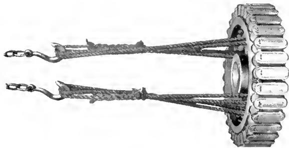
Fig. 15. Proper Way to Lift and Turn Revolving Field (First Position)
