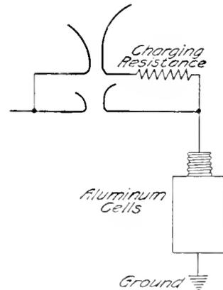
Fig. 8. The Essential Theoretical Features of an Aluminum Arrester
