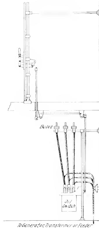
Fig. 2. Busses and Oil-Switches on Frame-work below Floor of Switchboard Room
