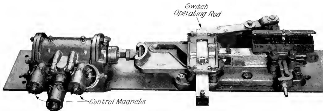
Fig. 3. Electro-Pneumatic Plate Switch and Movement
