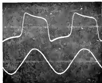
Fig. 4. 60 Cycle Arc—Flame Carbon Electrode
