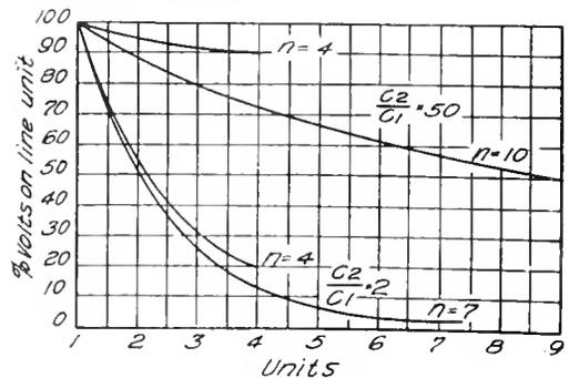
Fig. 13. Fall of Potential Across Individual Units for Values of  $\frac{C_2}{C_1} = 2$  and  $\frac{C_2}{C_1} = 50$
