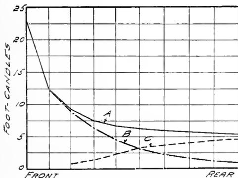
Fig. 10. A Suitable Distribution of Light Intensity Along the Center Line of Stage, from Front to Back
