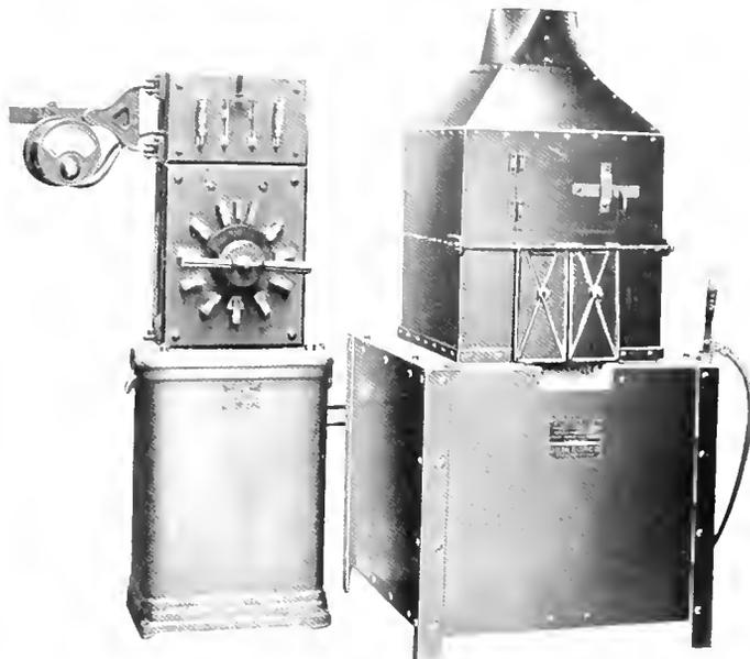
Fig. 7. Furnace for Hardening Carbon Steel
