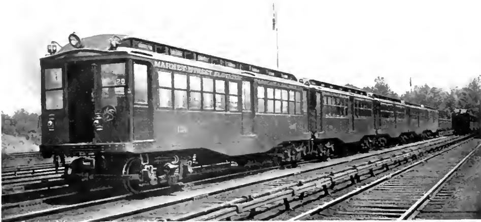
Five-Car Elevated and Subway Train, Philadelphia Rapid Transit Company. Each Motor Car Equipped with Two 125 H.P. Motors (GE-66) and Sprague G-E Type M Control
