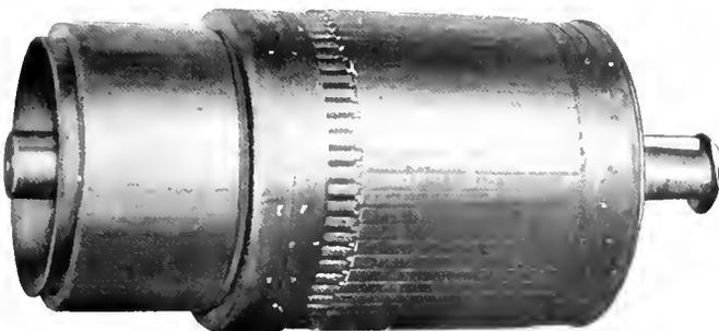
Fig. 9. Armature of Single-Phase Railway Motor
