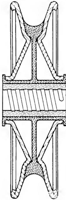
Fig. 2. Cross Section of Steel Flanged Trolley Wheel
