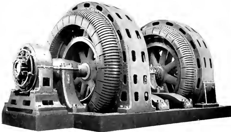
Fig. 2. 2500 Kw. Frequency Changer Set and Exciter with Sub-bases under Middle Bearings
