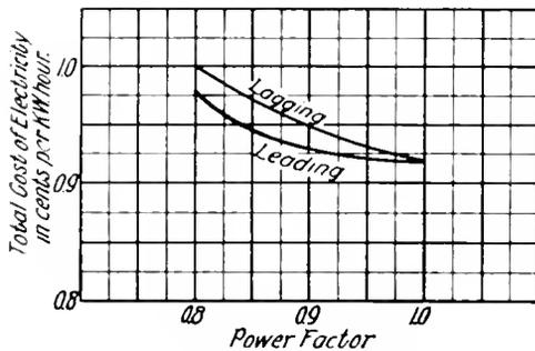
Fig. 3. Curve Showing the Relation Between Cost of Electricity and Power-Factor, Leading and Lagging
