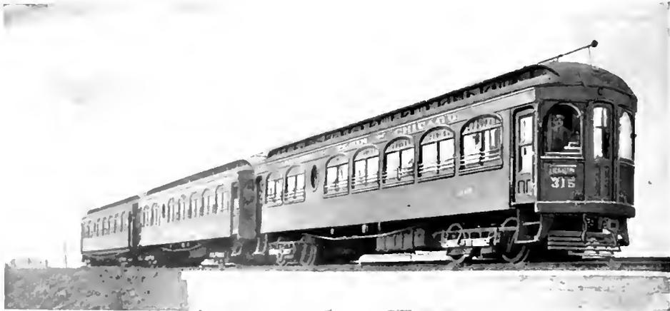
Three-Car Interurban Train, Aurora, Elgin & Chicago Railway. Each Car is Equipped with Four 125 H.P. Motors (GE-66) and Sprague G-E Type M Control
