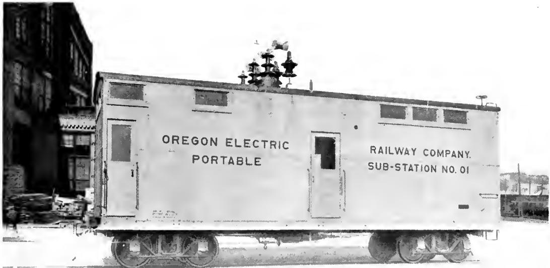
Fig. 7. Portable Substation Built for the Oregon Elec. Ry. Co., 60,000 Volt Incoming Line, 1200 Volt 500 Kw. Converter
