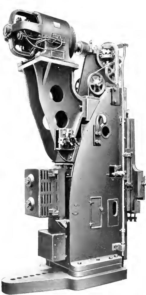
Fig. 17. 48 in. Slotter equipped with Reversing Motor Drive. Left hand side, panel cover closed
