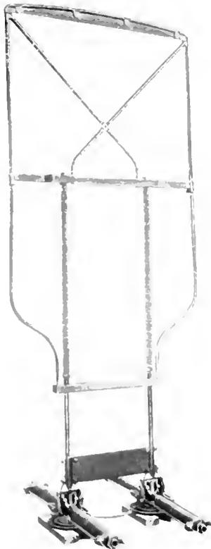
Fig. 11. Bow Trolley for Freight Yard Shifting Service
