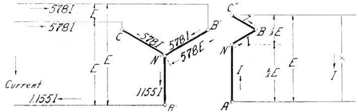
Fig. 8. Y-Connection, One Leg of Secondary Reversed, Ratio of One Phase One-Half Ratio of Other Phases
