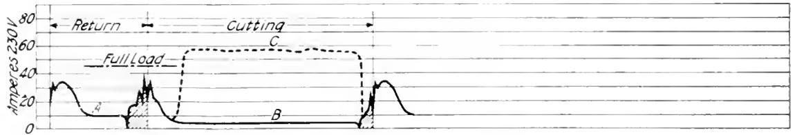
Graphic Recording Ammeter Curves (Slotters)
