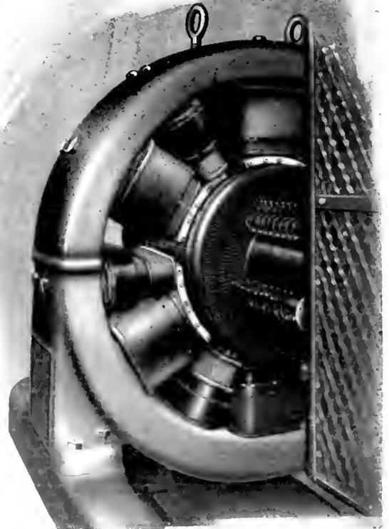
Fig. 3. 250 Kv-a 500 550 Volt, Regulating Pole Converter
