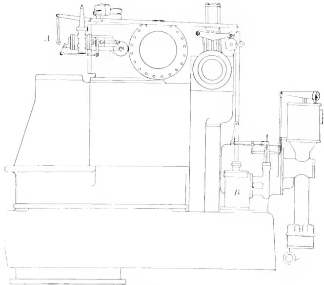
Fig. 6. A Simpler Mechanism for Controlling the Extraction of Steam from Curtis Turbines
