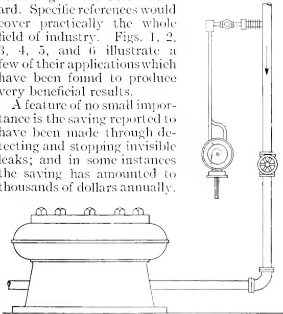
Fig. 5. Application of Steam Flow Meter to Rubber Vulcanizer
