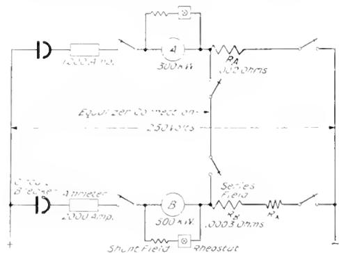
will cause each series field to carry only its own armature current. Since the machines are of the same compound, each will then automatically assume its own share of the total line load, after having once been set with the shunt field.
