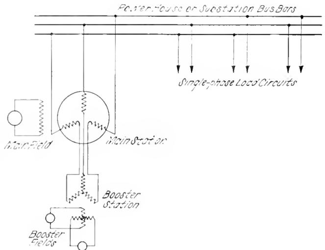
Wiring Diagram of Phase Balancer Set
