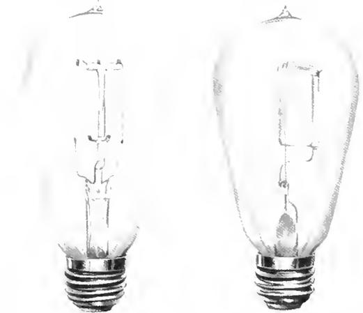
Fig. 4. 8 C-P., 45 Volt Standard Lamps Used in Tests with Rood Flicker Photometer
