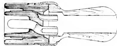
Fig. 13. Charging Plug for Vehicle Batteries
