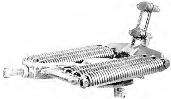
Fig. 4. Ball Bearing Trolley Base
