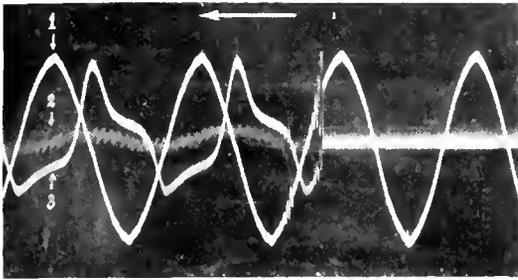
Fig. 9. Switching Transformer onto Generator by Low-Tension Switch. (1) Wave of Low Tension Voltage, (2) Wave of Capacity Current at Middle of High-Tension Winding, (3) Wave of Exciting Current
