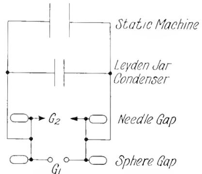
Fig. 2. Diagram of Rewired Testing Apparatus. A Sample Reading Taken with this Scheme of Connections is Given in Table II
