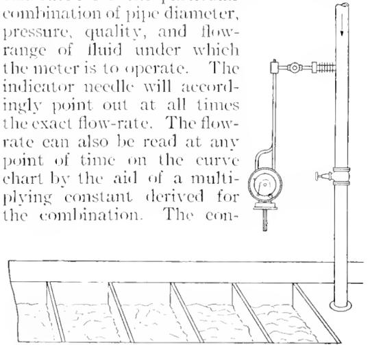
Fig. 6. Steam Flow Meter for Regulating the Process of Tanning Leather
