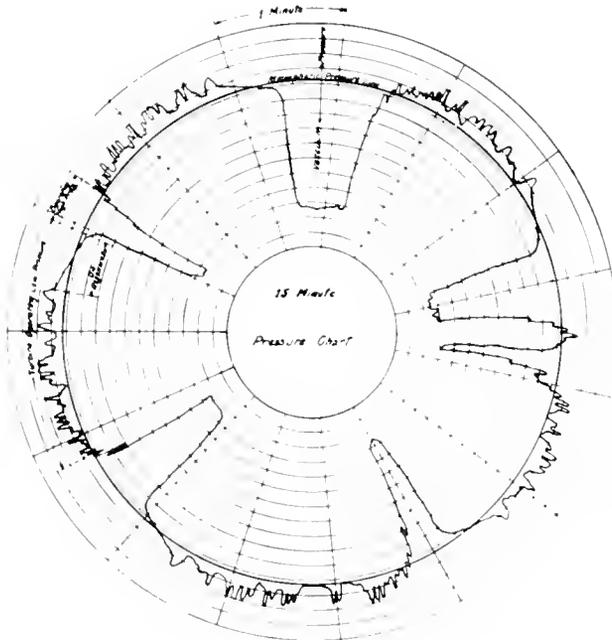
Fig. 9 Chart Showing Low Pressure Steam Supply
