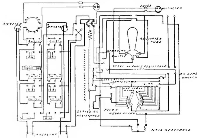
Fig. 17. Public Garage Panel with Mercury Arc Rectifier
