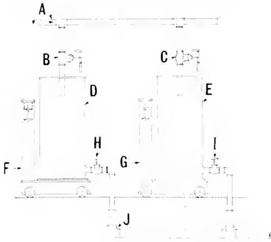
Fig. 2. Alternative Arrangement of Discharge Piping and Tanks for Weighing Condensed Steam in Water-Rate Tests of Steam Turbine Sets
