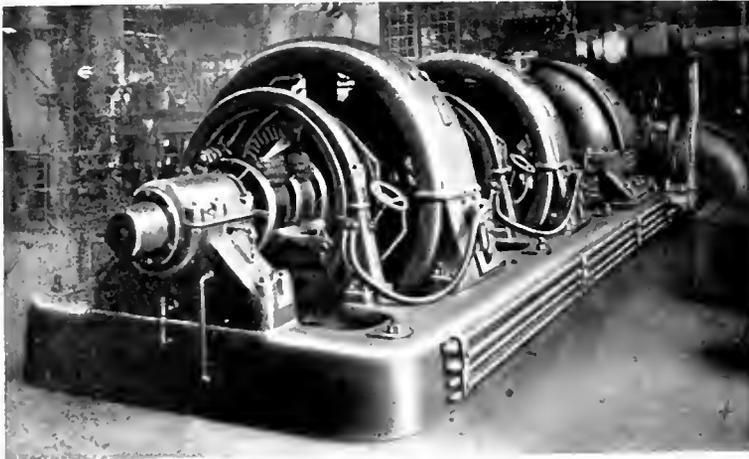
Fig. 4. Two 500 Kw., 600 Volt, 1500 R.P.M., Direct Current Generators Using Graphite Brushes and Slotted Commutators. The commutators of these machines are designed with three shrink rings, the central one dividing the length equally and preventing any tendency of the bars to buckle.
