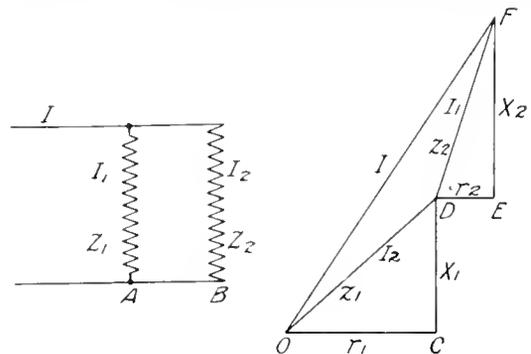
*A* and *B* respectively. Draw *OF*. If the vector *OF* is allowed to represent the total load current *I*, then *DF* will represent the current in transformer *A*, and *OD* the current in transformer *B*, both in magnitude and phase relation. It should be noted that the vector representing the impedance of one transformer gives the load current of the other transformer. W.W.L.
