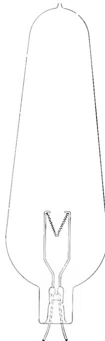
Fig. 2. High Efficiency Nitrogen-Filled Lamp for Low-Voltage Current
