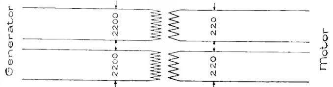
Fig. 4. Two Transformers for Two-Phase Four-Wire Transformation
