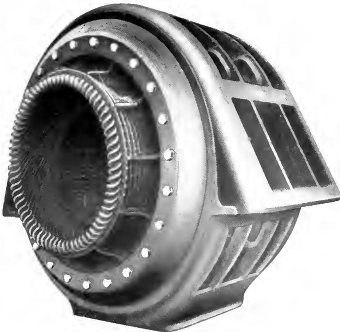
Fig. 2. Complete Stator of Turbine-Driven Alternator without End Shields or Lagging
