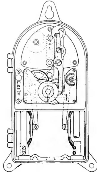
Fig. 19. Automatic Time Switch for Storage Batteries
