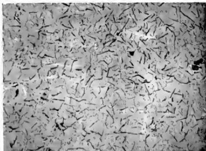
Fig. 7. Electrolytic Iron Electrode. Weld made in air.
