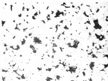
Fig. 10. Section of Weld Made with Pure Electrolytic Iron
