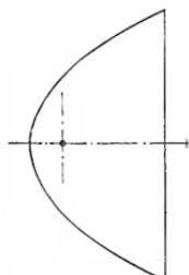
Fig. 1. Parabolic Reflector commonly used for automobile headlight service
