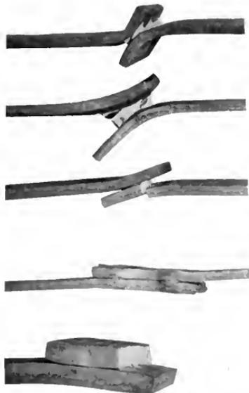
Fig. 4. Test of Samples  $\frac{1}{2}$ -inch and 1-inch Thick showing Tearing Action when a Single Row of Welded Spots is Used and the Jaws of the Testing Machine are Offset to Accommodate the Displacement. It is, therefore, obvious that, as with rivets, more than one row of spots should be used.
