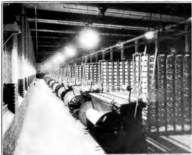
Fig. 1. Night Photograph of a Row of Warpers Well Illuminated by 75-watt Mazda C Lamps in Deep Bowl Steel Reflectors Hung Over the Beam and the Creel. Work under such can be carried on effectively, independent of daylight conditions. With good illuminations, the shop is perforce clean and safe. Employees are contented and production is kept at a maximum
