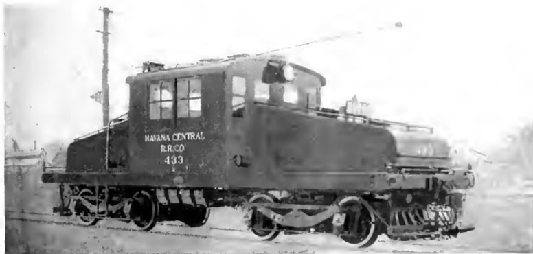
60-ton Trolley Type Electric Locomotive for Bringing in Cane Trains from the Fields
