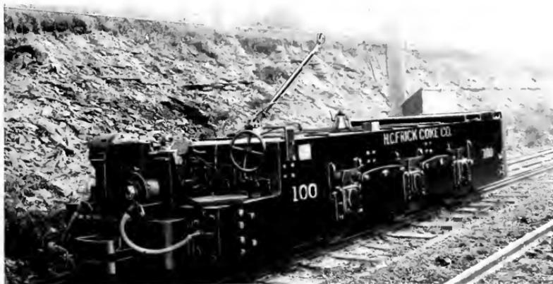
Fig. 15. 30-ton, 48-inch Gauge Mine Haulage Locomotive
