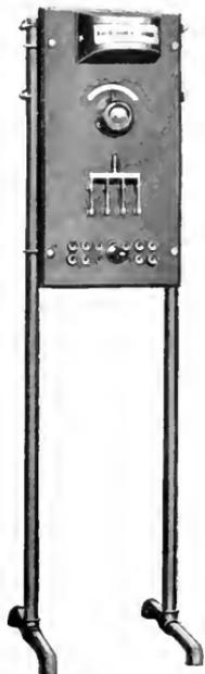
Fig. 3. Front View of Alternating-current Temperature Indicator Panel
