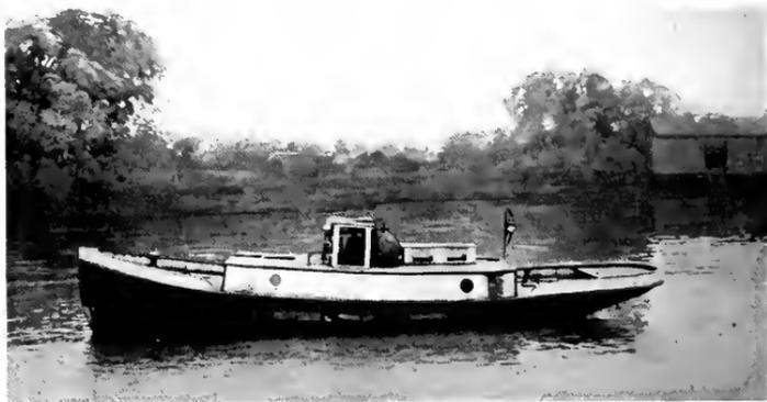
Fig. 1. Side View of Electrically Welded Boat
