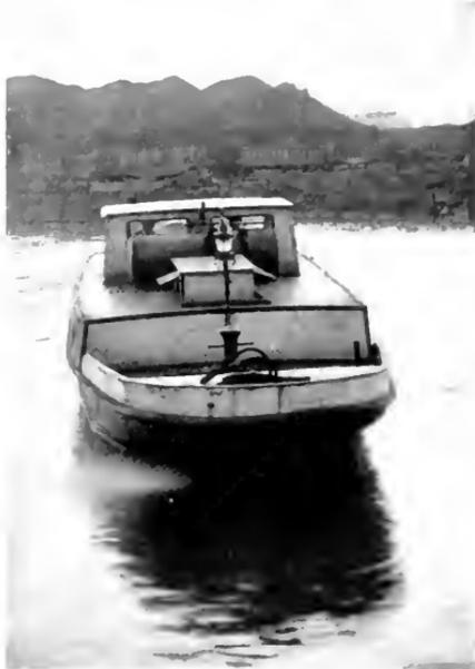
Figs. 2 and 3. Bow and Stern Views of Electrically Welded Boat
