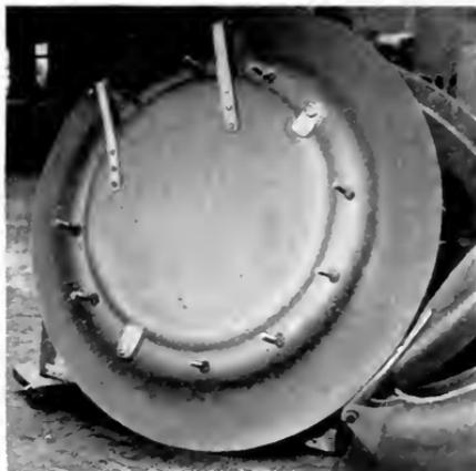
Fig. 8. Smoke Box Front with Studs Welded by Electric Bare Arc Process
