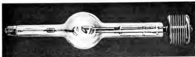
Fig. 2. Special Self-rectifying Roentgen-ray Tube
