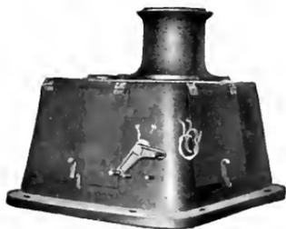
Motor-driven Winch for Placing Cane Cars on Unloading Platforms
