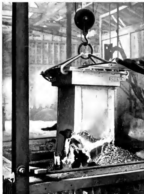
Fig. 4 Photograph taken shortly after 20-inch square carbon electrode had broken on a single-phase Ferro-silicon Furnace
