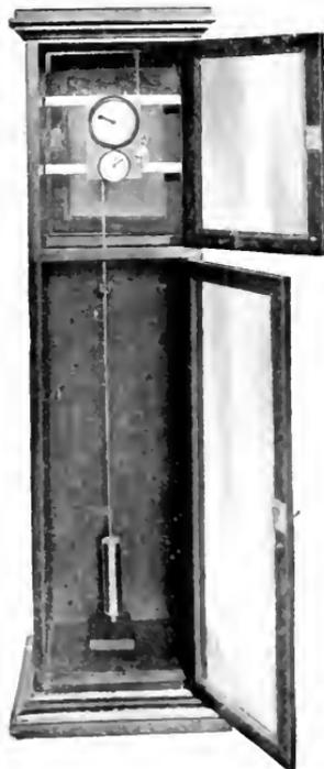
Fig. 1 The Warren Clock for Frequency Regulation
