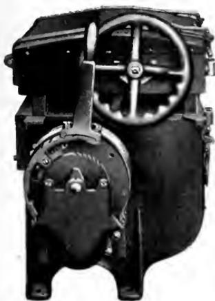
Fig. 3. End View of Controller Showing Ratchet Operating Mechanism
