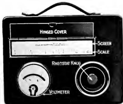
Fig. 86. Foot-candle Meter—Front View
