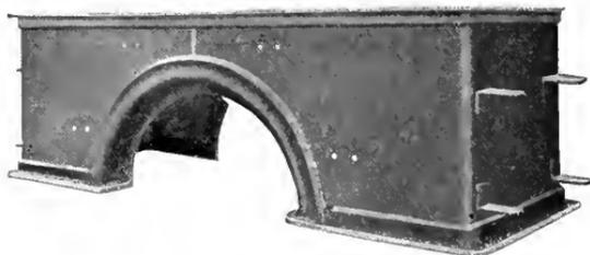
Fig. 12. Electrically Welded Turbine Exhaust Hood
