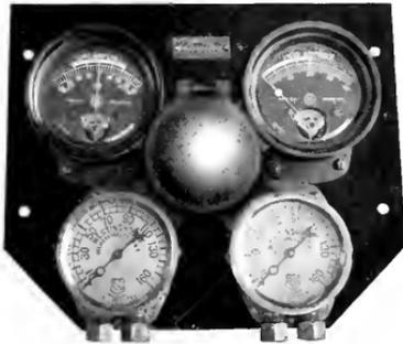
Fig. 5. Ammeters Showing Degree of Regenerative Braking
