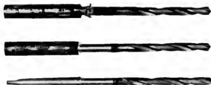
Fig. 8. High Speed Drill Electrically Butt-welded to Shank of Ordinary Machine Steel
