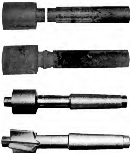
Fig. 5. Various Stages in Manufacture of Machine Tool Formed by Electrically Butt-welding High Speed Steel to Shank of Ordinary Machine Steel
