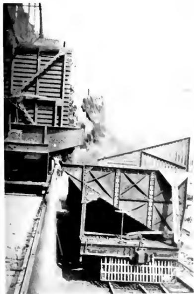
Fig. 9. This View Shows the Red Hot Coke being Discharged from an Oven into the Quenching Car
