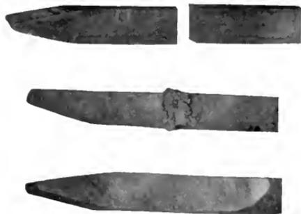
Fig. 7. Electrically Butt-welding High Speed Cutting Face to Machine Tool Shank
