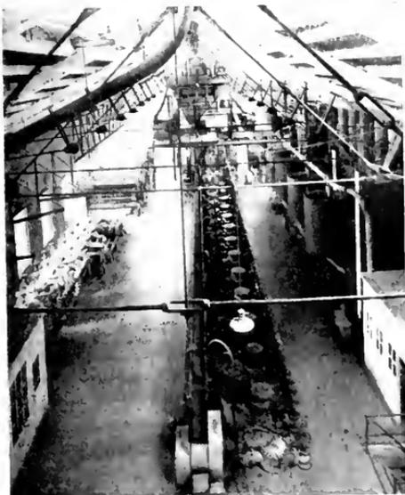
Fig. 7. Cell Floor showing Diffusion Cells and Cassette Conveyor in the Center with Heaters, Filter Presses, and Carbonation Tanks at the side. American Beet Sugar Company, Chino, Cal.
