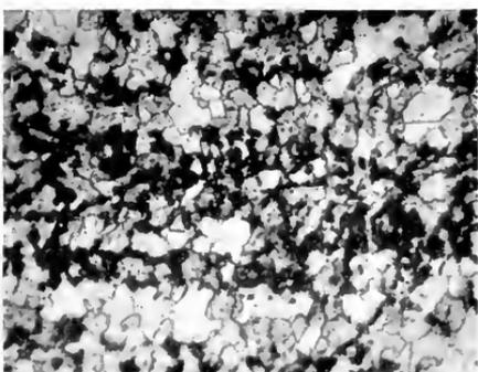
Close to weld, showing ferrite grains with normal spherulitic structure. 150 diameters.
