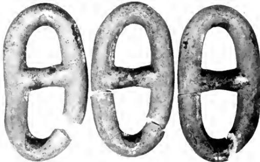
Fig. 10. Two-inch Electric Cast-steel Links Made at Schenectady and Tested at the Charleston Navy Yard
