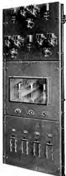
Fig. 30. Control Panel for Furnace
