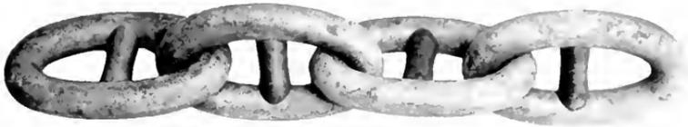
Fig. 5. The Section of Chain shown in Fig. 3 after the Studs have been Placed in Position
