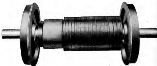
Fig. 6. Wheels and Armature of Bipolar Gearless Motor
