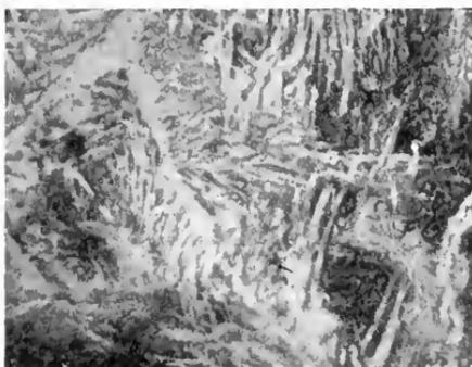
At weld, showing very large sorbitic grains with irregular band of ferrite. 150 diameters.
