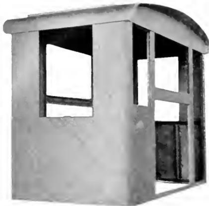
Fig. 1. Electrically Welded Locomotive Cab
