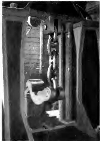
Fig. 8. 2 1/2-in. Naco Anchor-chain Links in a Standard MCB Drop Testing Machine, National Malleable Castings Co.
