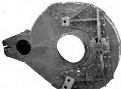
Fig. 9. Gear Housing on Which the Seams are Electrically Welded
