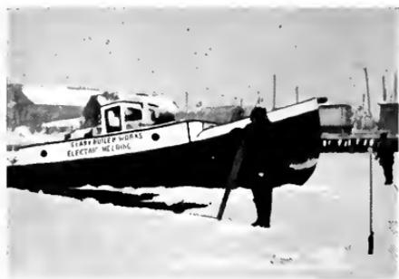
Fig. 9. Electrically Welded Boat Attempting to Break Through Twelve to Fourteen-inch Ice
