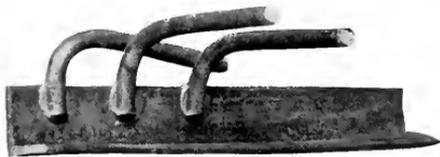
Fig. 3. Straight Rods Spot-welded to Angle Iron and then Bent by Hammer Blows, the Angle Being Supported only by the Unwelded Flange
