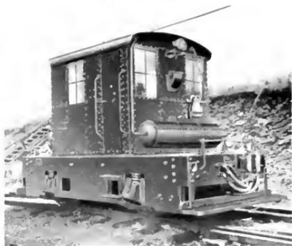
Fig. 10. A 20-ton Electrically Operated Quenching Car Locomotive
