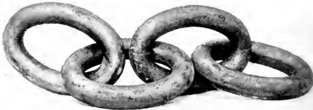
Fig. 3. First Anchor-chain Links Electric Die-cast at the Schenectady Works
