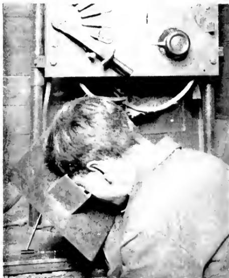
Fig. 8. Proper Distance at which to Hold the Electrode from the Work
