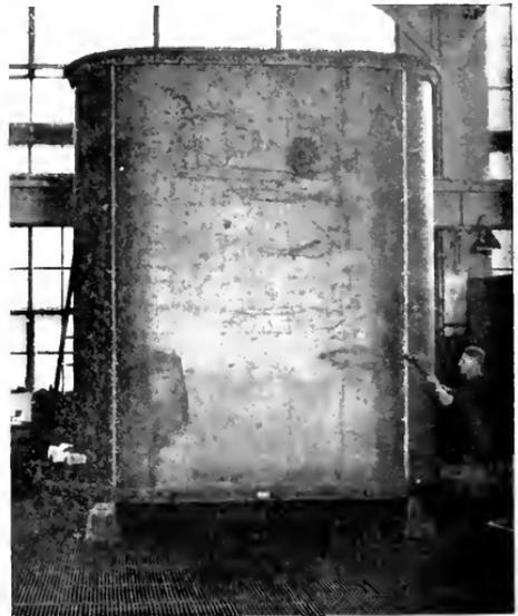
Fig. 14. Large Tank in Regular Test for Leaks. It is filled with water and allowed to stand for 48 hours. This tank with 90 ft. of welding did not develop a single leak. While filled with water the seams are given sharp blows throughout their length with a five-pound hammer
