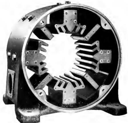
Fig. 5. Magnet Frame of RF Motor Showing Construction and Arrangement of Pole Pieces
