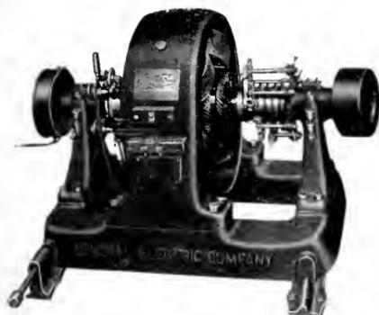
Fig. 3. 4-pole, 10-kw., 1800-r.p.m., 110-volt Shunt-wound Synchronous Converter
