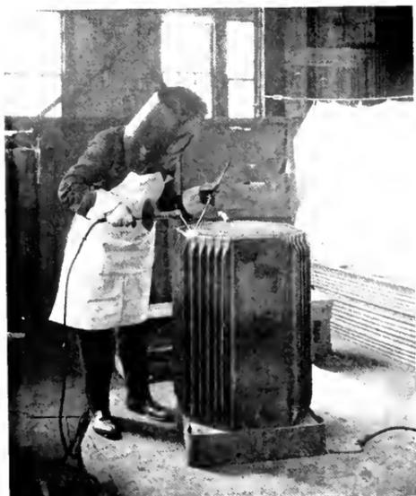
Fig. 19. Use of Carbon Electrode with Metal Filler when Welding  $\frac{1}{2}$ -in. Steel Bases to the Edges of Crushed Corrugations
