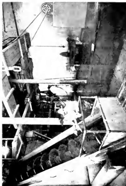
Fig. 4. Beet Screw for Elevating the Beets from the Flame to the Washes at the top. American Beet Sugar Company, Chino, Cal.
