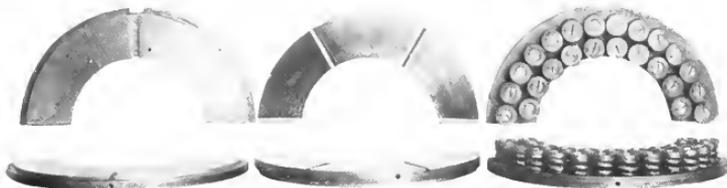
Fig. 4. Stationary Babbitted Ring, Rotating Ring and Springs of a Spring Thrust Bearing
