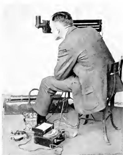
Fig. 17. Reading Illumination on a Horizontal Plane with the Sharp-Millar Photometer
