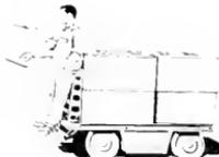
Fig. 8. An Electric Storage Battery Propelled Load-carrying Truck usually geared for about four to five miles per hour, capable of carrying about two tons. This truck is especially suited for handling miscellaneous cargo at steamship and railway terminals; also is adapted for peddling packages of 100 lb. and less in factories or assembly plants where the radius of operation
