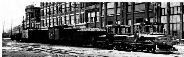
Fig. 23. Two 40-ton Storage Battery Locomotives Operating in Tandem as an 80-ton Unit
