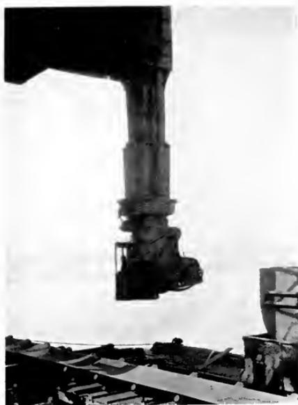
Fig. 38. Coal Trimmer at Bottom of Telescopic Chute, Showing Location of Operator's Cage
