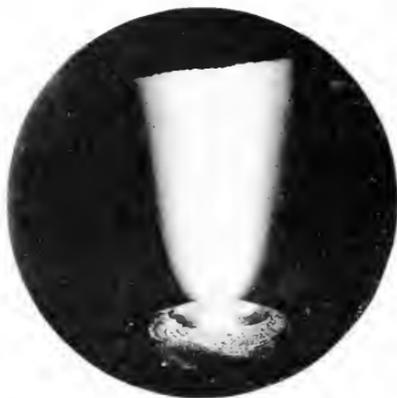
FIG. 1. Arc and Tips of the Electrodes of the Luminous Arc Lamp. The arc rises from a molten pool of oxides, spreads out, and furnishes all the light emitted from this type of lamp
