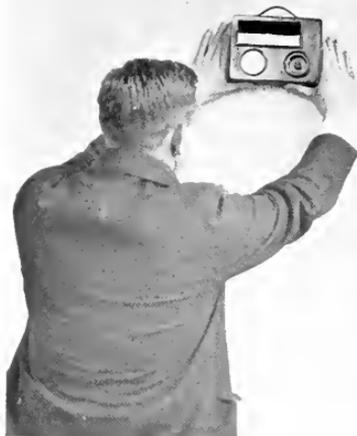
Fig. 21. Reading Illumination on a Vertical Surface with the Foot-candle Meter
