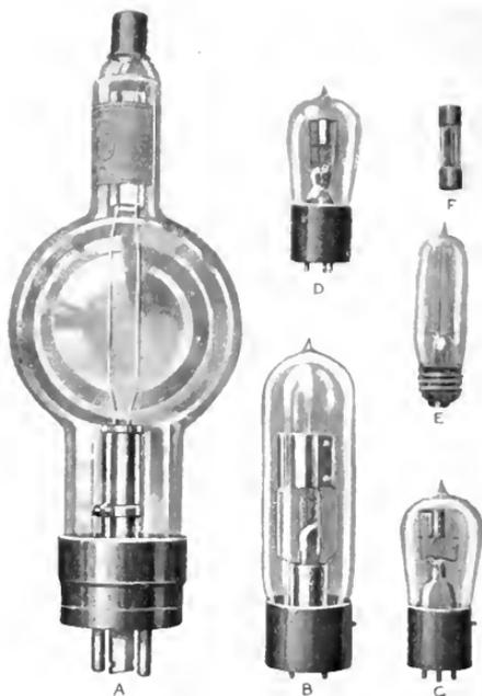
Fig. 4. Vacuum Tubes of Sizes from 5 to 250 Watts Power Output
