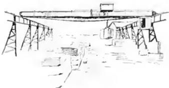
Fig. 31. The Electric Overhead Traveling Crane is especially adapted for handling all size packages at a high rate of speed and especially material weighing over 1000 lb. which men could hardly be expected to move by any other means. It is economical only where a large volume of material is to be moved every day.
