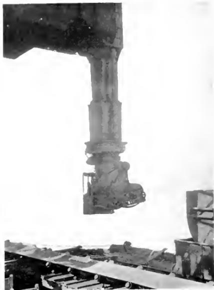
Fig. 2. Coal Trimmer at Bottom of Telescope Chute. Collector Rings (with Cover Removed) Just Above the Operator's Cab
