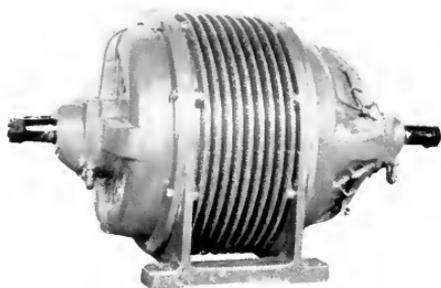
Fig. 1. Alternating-current Deck Motor Recently Installed on the Mooring Winch of a Tank Steamer
