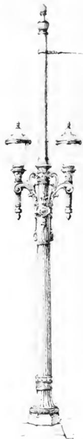
Fig. 14. A Two-unit Bracket Mounting for Use on the Trolley Poles of Important Streets
