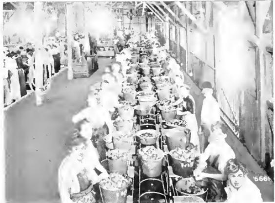
Fig. 4. Continuous Moving Conveyor in Canning Factory
