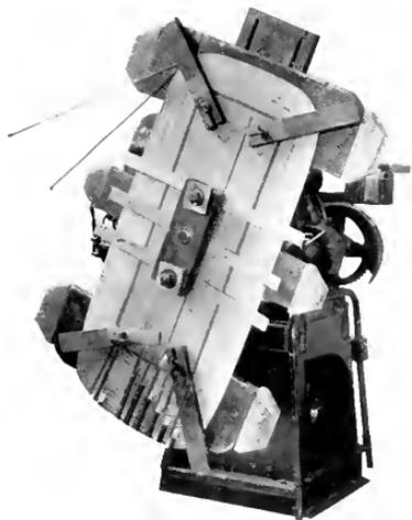
Fig. 5. The Difference in Tension Applied in Winding a Rectangular Coil is Illustrated by the Difference in Lever Arm, i.e., the Difference in the Distances from the Spindle to the Sides. It is impossible to obtain uniform tension in such a coil structure
