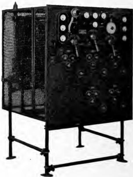
Fig. 6. Vacuum Tube Transmitter of Medium Power
