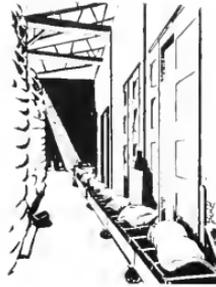
Fig. 5. Portable Power-driven Conveyor set up in sections and used for filling a warehouse with medium size packages. The conveyor can be easily transported to another section of the warehouse for similar duty. The capacity is about one ton per minute
