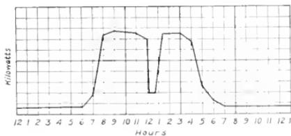
Fig. 7b. Load Curve of Marble Cutting Plant
