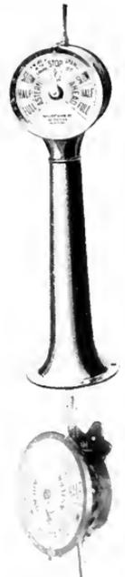
Fig. 8. Mechanical Engine Order Telegraph System
