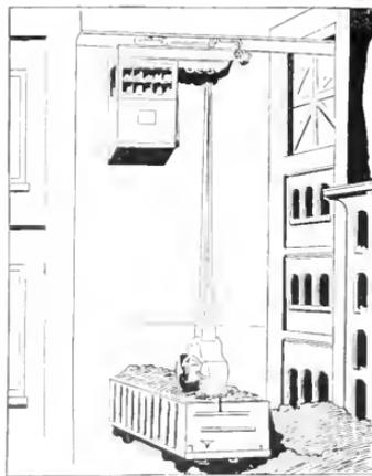
Fig. 34. An Electric Overhead Monorail Crane equipped with self-filling grab bucket suitable for carrying bulk material from railway cars or storage piles into buildings. It can manipulate curves and travel at speeds of 7 to 10 miles an hour.
