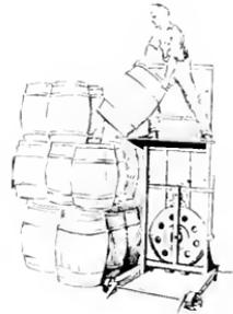
Fig. 26. A Portable Elevator enables one man to pile to any height, inside a building, heavy packages which he could not otherwise pile unassisted. As seen in Fig. 27, two men in team work can pile these heavy packages advantageously. The device will handle packages up to about 1500 lb. and will make one trip in about two minutes
