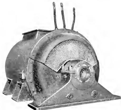
Fig. 1. Partial Assembly of Three-phase Alternating-current Generator for Electric Propulsion of Cargo Boats
