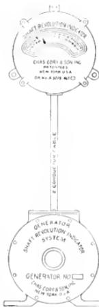
Fig. 4. Shaft Speed Indicator Outfit
