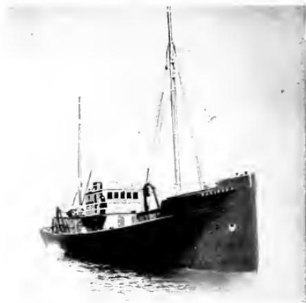
Fig. 1 The Mariner: The First Diesel Engine Electrically Propelled Vessel
