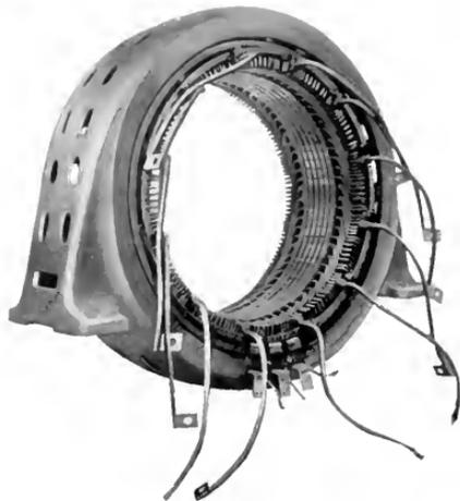
Fig. 3. Completely Wound Stator of Scherbius Regulating Machine
