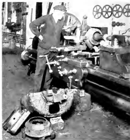
Fig. 3. Broken Cast Iron Motor Casing and Brake Housings Welded by General Electric Constant Energy Welding Machine - Case Broken in Twelve Pieces
