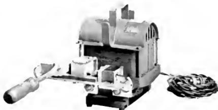
Fig. 7. Heating a Soldering Iron with the Pyrotip
