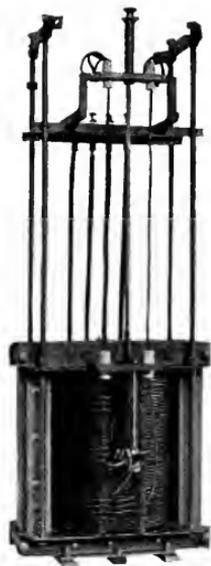
Fig. 4. Large 13,800-volt Transformer Ready for Tank, High-voltage Side, Showing 100-amp. Ratio Adjuster
