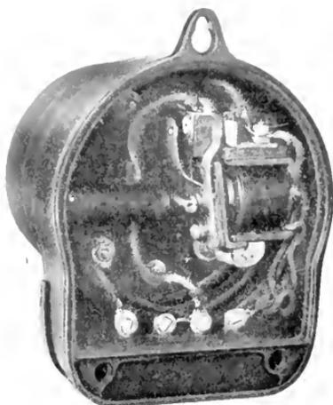
Fig. 6. Under Side of High Capacity MC-1 Relay Showing Auxiliary in Base
