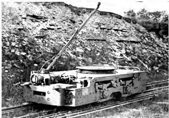
Fig. 17 New Type of Gathering Locomotive Showing Arrangement of Controller and the Use of Journal Leaf Springs
