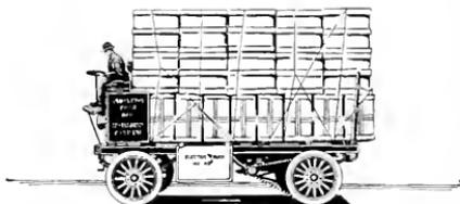
Fig. 17. The Electric Storage Battery Automobile Truck for road use is especially adapted for peddling packages of 200 lb. and less within a radius of about one mile. It has a speed of about 10 miles an hour
