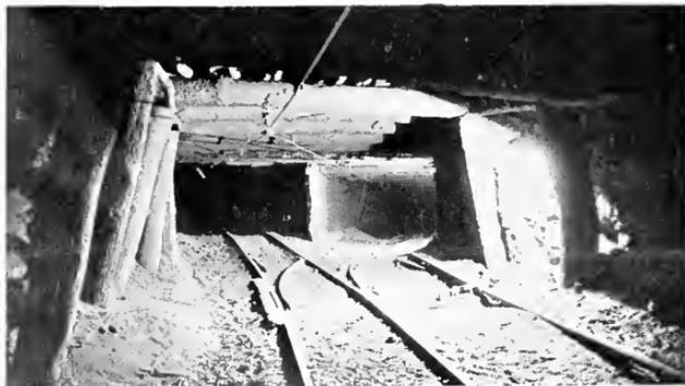
Fig. 90. The Switchpoint in a Coal Mine, with Suitable General Illumination. It is very interesting to contrast this picture with conditions as usually encountered in the mine. It is no wonder that the accident rate is relatively high considering the dangerous operating conditions and the total inadequacies of the lighting as ordinarily supplied
