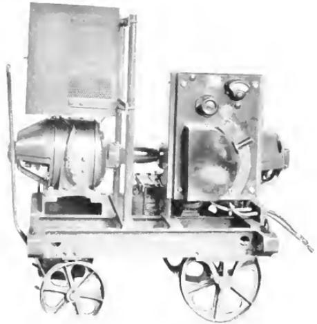
Fig. 5. Portable Single operator Constant Energy Arc Welding Machine 60 20-volts 200-ampere
