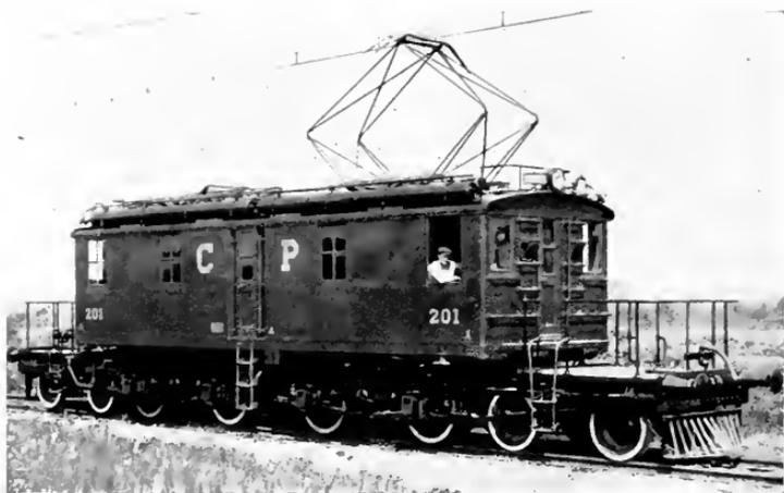
Fig. 3. One of the Four 120-ton Geared Passenger Locomotives
