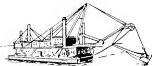
Fig. 35. A Floating Dredge which handles a dipper bucket at the end of a stiff boom is suitable for excavating submerged bulk material. It is used in mining operations and in canal digging or canal clearing.
