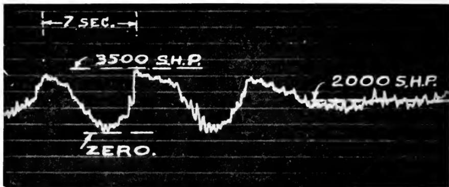
Fig. 2. Record from Torsion Spring Coupling on *Jebsen* in Ballast in a Moderately Rough Sea. Part of the smaller fluctuations resulted from an untrue collar in the instrument; otherwise the record is correct
