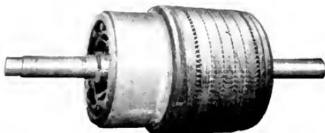
Fig. 5. Armature of 150-h.p., 720 r.p.m., 2200-volt Varying-speed Brush-shifting Motor
