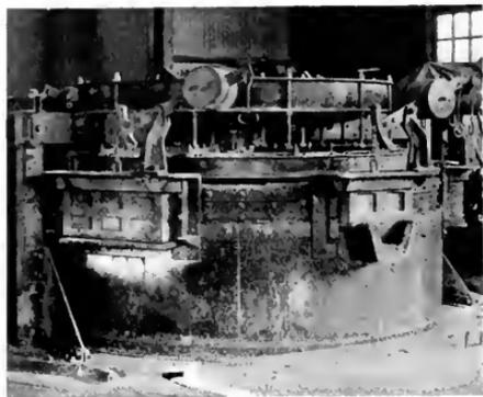
Fig. 11 Induction Type Furnace at Pittsfield Works, Which Has Recently Completed 555 Heats on One Lining
