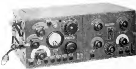
Fig. 5. Radio Set for Aircraft, Vacuum Tube Transmitter and Receiver Combined in One Unit
