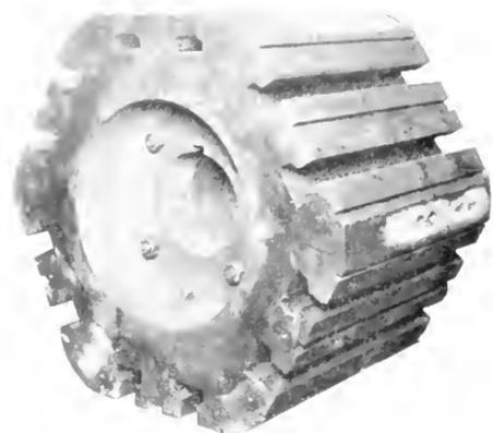
Fig. 6. Rotor Spider of a 6-pole, 3530-kv-a., 500-r.p.m. Water-wheel Driven Alternator
