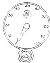
Fig. 15. Selsyn Indicator for the Operation of Bascule Bridges
