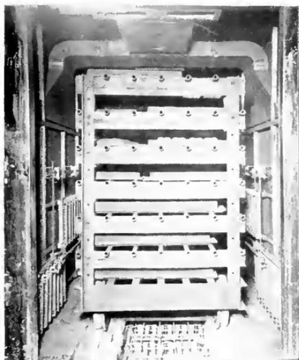
Fig. 5. Electrically Heated Core Baking Oven, Showing Loaded Truck and Electric Heaters. Oven 10 ft. long, 5 ft. wide, 7 ft. high, 72 kw. connected
