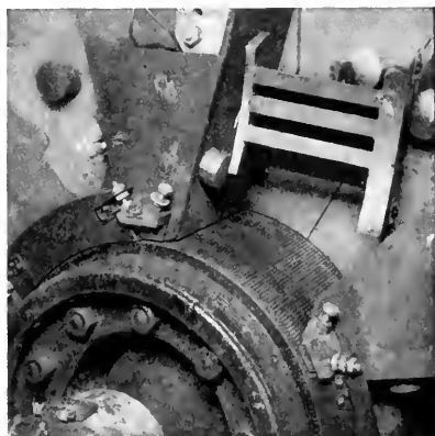
Fig. 6. Barrier Removed for Inspection After 50 Maximum Short Circuits as Shown in Fig. 5
