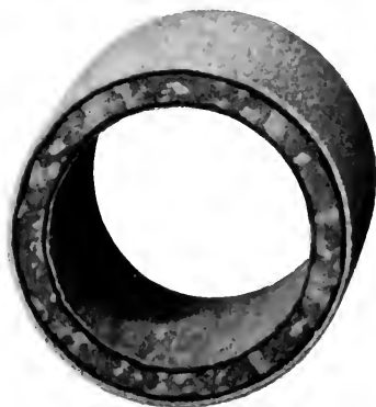
Fig. 2. Calorized Steel Showing Oxidation of Unprotected Section
