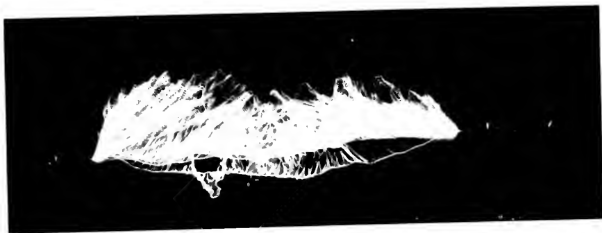
Fig. 14 Several Successive 1,200,000 volt Arcs Between Points Spaced 11 Ft. Apart
