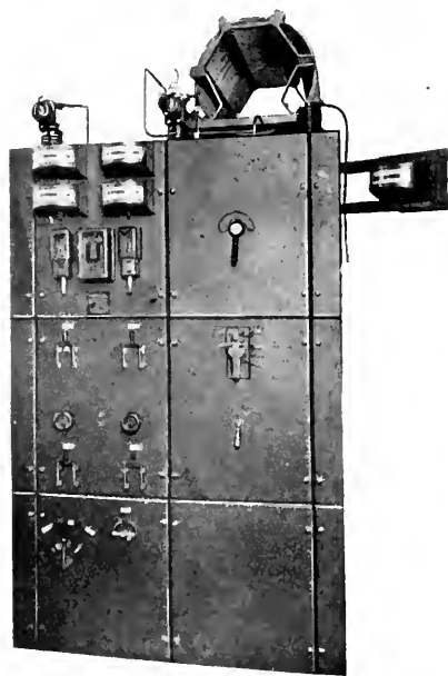
Fig. 12. 2-kw. Radio Telegraph Transmitter for Interrupted-continuous-wave and Continuous-wave Communication. Wavelength 600 to 3000 meters
