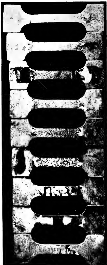
Fig. 7 Crystal Growth in Aluminum Sheet After Various Elongations Followed by Anneal for 65 hours at 550 deg C. One-third size. From Crystal Growth and Recrystallization in Metal, by Carpenter and Elam. Jour. Inst. Metals, Vol. 24, p. 104, Plate IX, 1920.
