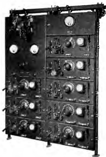
Fig. 8. Eight-circuit Battery Charging Switchboard for Constant-current or Series-resistance Charging with Automatic Cut Off and Ampere-hour Meters in Each Circuit
