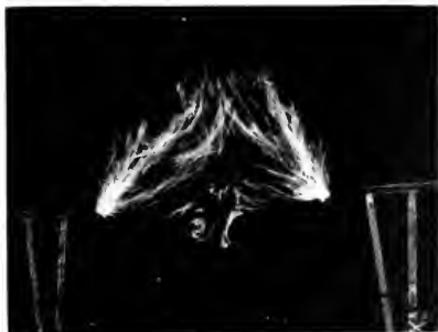
Fig. 18. Spark-over Between Needle Points at One Million Volts. Distance about nine feet
