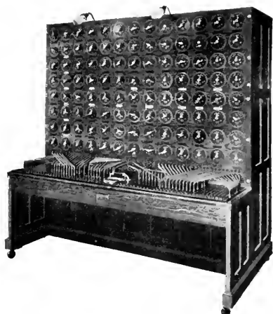
Fig. 21. Short Circuit Calculating Table
