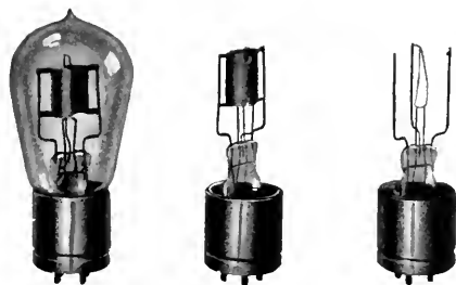
Fig. 4. Kenotron Rectifier Tube (UV-216) Complete and in Two Stages of Assembly
