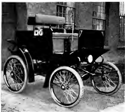
Fig. 1. Typical Four-passenger Runabout of 1898 (Columbia Electric Vehicle Company)
