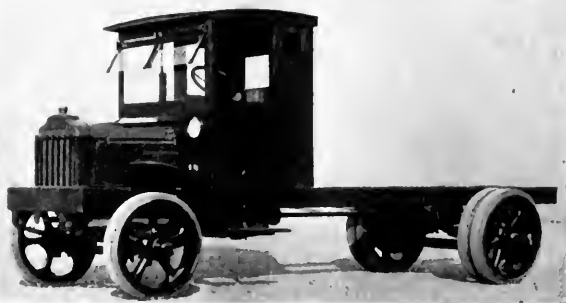
Fig. 2. A 5-ton Gasoline Truck with Front Axle and Steering Mechanism Parts Interchangeable with Those of an Electric Truck of the Same Capacity
