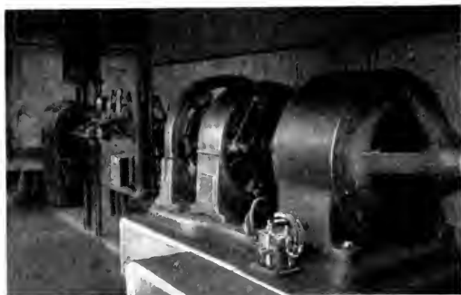
Fig. 5. Motor-generator Set and Control (225-h.p. induction motor; 150-kw., 75-volt generator) for supplying energy to five operators per shift
