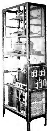
Fig. 5. Kenotron and Power Control Unit Used in the Duplex Radio Telephone Tests
