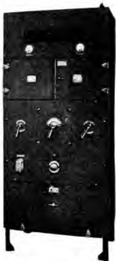
Fig. 4. 1-kw. Commercial Transmitter for Telephony. Interrupted-continuous-wave Telegraphy and Continuous-wave Telegraphy
