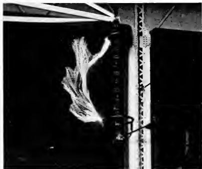
Fig. 3. Suspension Insulator String with Antenna or Shielding Ring of the Peek Type for Equalizing the Voltage
