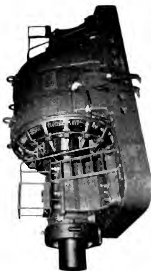
Fig. 18. 200-kw. Synchronous Converter with Automatic Control in Drifton Colliery of Lehigh Valley Coal Company
