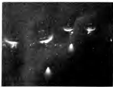
Fig. 21. Automatic Shielding by Corona (See Fig. 23)
