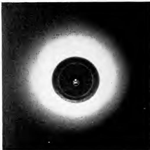
Fig. 22. 800,000-volt Corona, through Quartz Lens
