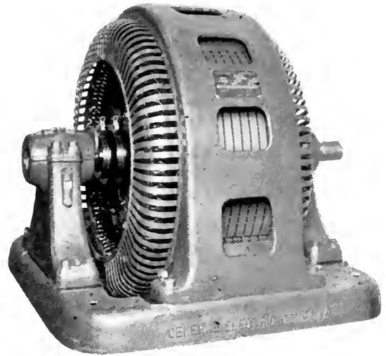
Fig. 2. Medium Capacity Synchronous Condenser, 8 poles, 1500 kv-a., 900 r.p.m., 4000-2300 volts
