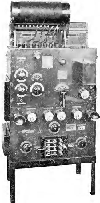
Fig. 54. Vacuum Tube Transmitter and Power Panel for use on Submarines
