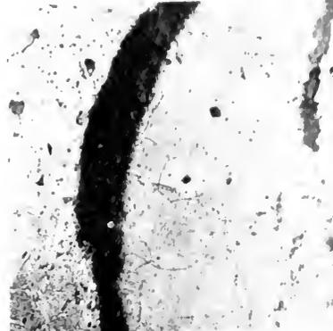
Fig. 16. Very Soft Cast Iron. No pearlitic Matrix all ferrite. Graphite plates large. Taken from large casting in dry sand. Magnified 200 dia.
