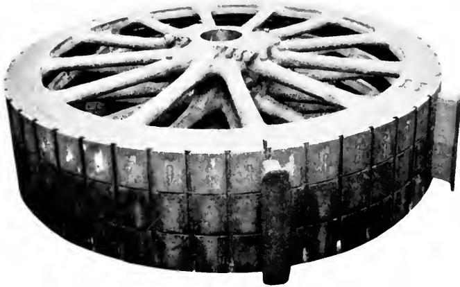
Fig. 22. Rotor Spider of 40,000-kv-a Generator for Shawinigan Engineering Company, Ltd., Canada
