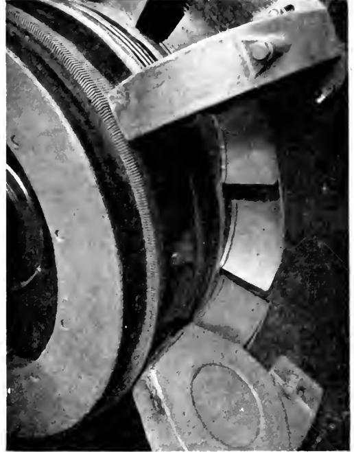
Fig. 4. Fan on Armature and Magnetic Blowout in Brush-holder for Prevention of Flash-over on 4500-kw., 1500-volt B.T.H. Synchronous Converter
