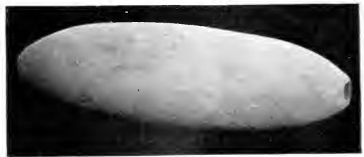
Fig. 11. Model No. 1 Fused Quartz Insulator after being taken from the furnace
