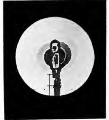
Figs. 25, 26 and 27. Eighteen-inch Searchlight Mirror Images of Spiral Filament seen from a radius of 145 ft. at points 1 deg. 30 min., 0 deg. 45 min., and 0 deg. 0 min. respectively from the axis
