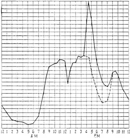
Fig. 8. Summer Load Curve showing Effect of Storm. Dotted line is for a normal day
