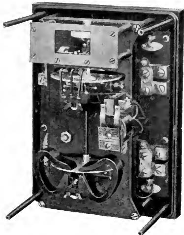
Fig. 69. Induction Polyphase Power Relay with Two Driving Elements
