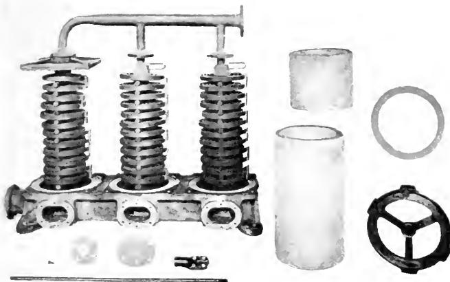
Fig. 3. Partially Dismantled Resistor of the Type shown in Figs. 1 and 2
