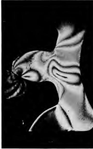
FIG. 5. COLORED IMAGE WHEN BOTH NORMAL INSIDE PRESSURE AND MAXIMUM TORQUE ARE APPLIED
