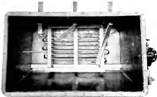
Fig. 9. Interior View of the Resistor shown in Fig. 7
