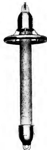
Fig. 13. First Model Fused Quartz Radio Insulator Complete with Corona Shield. Overall length 48 inches. Creepage distance 31 inches
