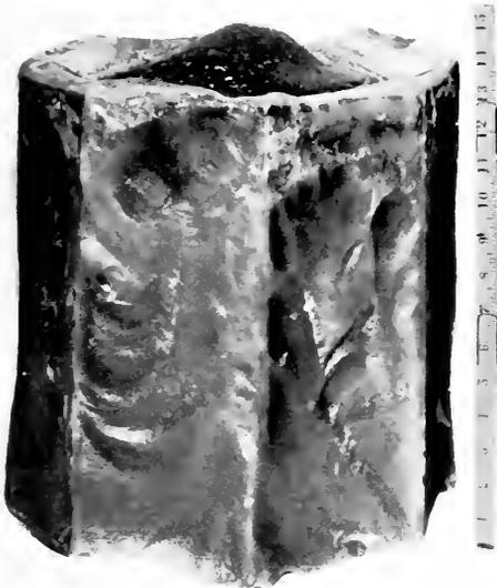
Fig. 1. Solid Ingot of Opaque Fused Quartz, Weight 115 Lb.
