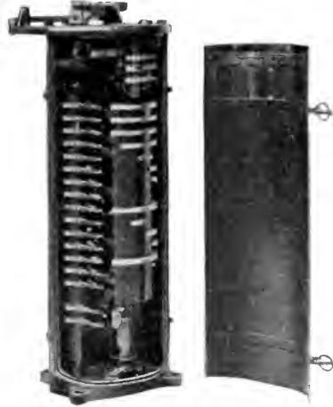
Fig. 4. Master Controller with Cover Removed
