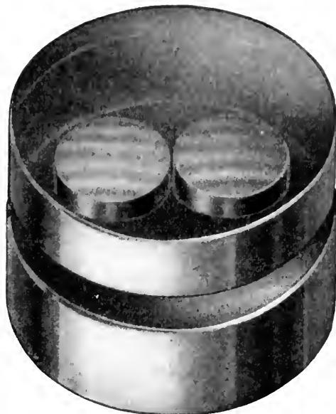
Fig. 5. Interference Bands on Two Flat Gauge Blocks That Are Being Compared for Length and Parallelism
