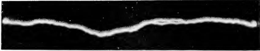
Fig. 6. A 1,500,000-volt Lightning Stroke between Points
