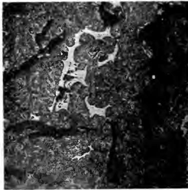
Fig. 7. Machine Cast Iron Heated Red Hot and Quenched in Ice Water. Matrix is martensite with graphite plates showing black. White spots are iron phosphide which the rapid quenching prevented from becoming phosphide eutectic. Magnified 100 dia.
