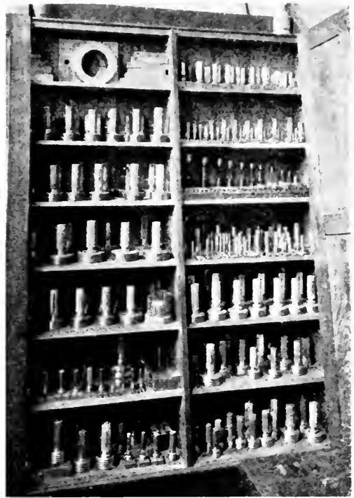
Fig. 12. Cabinet of Reference Thread Gauges
