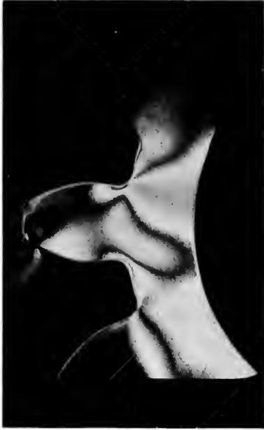
FIG. 3. COLORED IMAGE OBTAINED FOR NORMAL INSIDE PRESSURE AND REDUCED TORQUE
