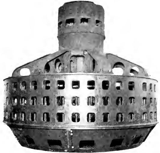
Fig. 23. 31,250-kv-a. Generator to be mounted on top of an existing 18,000-kv-a. vertical-shaft waterwheel generator
