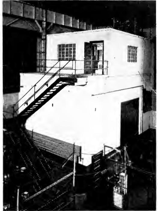
Fig. 5. Small Dark Room with Office Above. This dark room is equipped for tests up to 300 kv. to ground
