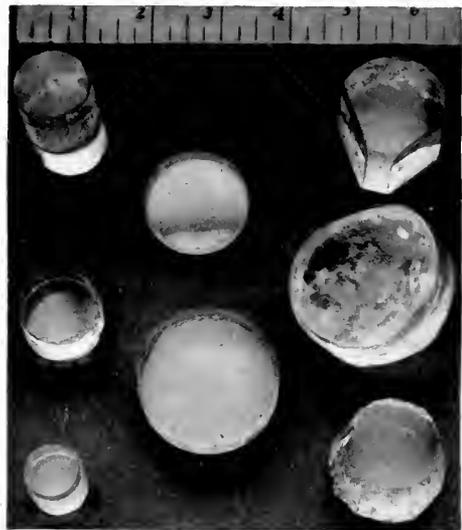
Fig. 7. Samples Clear Fused Quartz Optical Grade made in Thomson Research Laboratory, General Electric Company, River Works, Lynn
