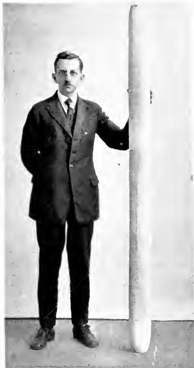
Fig. 12. Ingot of Opaque Fused Quartz weighing approximately 100 pounds. Six feet long and six inches in diameter
