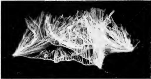
Fig. 20. 1,000,000-volt, 9-ft. Three-phase Arc showing Both Y and Delta Formations
