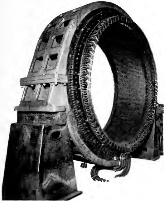
Fig. 7. Stator of the 20,000-kv-a., 257-r.p.m., 60-cycle, 11,000-volt Horizontal Generator, City of San Francisco Hetch Hetchy Development
