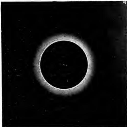
Fig. 21. 800,000-volt Corona, through Glass Lens
