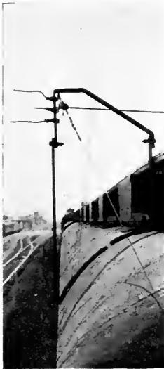
Fig. 48. Antenna Construction on Pullman train for radio reception en route
