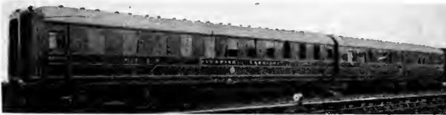
Fig. 5. Great Northern Railway, England. Two articulated cars showing the intermediate truck midway between the cars. Groups of five cars, similarly articulated, are in regular main-line service
