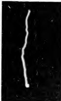
Fig. 8. Spark-over of Shielded Insulator String; single lightning stroke, 1,200,000 volts, dry
