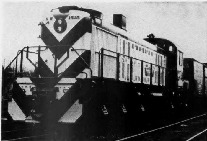
SIX-MOTOR Alco-GE road switcher for heavy-duty drag-and-transfer service
