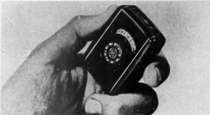
"MASCOT" exposure meter uses novel alnico magnet design for direct readings
