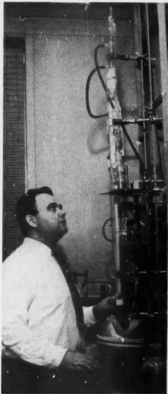
**GERMANIUM PURIFICATION** process (above) recovers 85 percent of the material lost in the original processing. The process produces material of equal purity with that commercially available and helps extend the supply of this important natural resource
