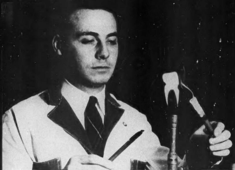
**BURNING TEST** on silicone-rubber insulation produces a white nonconducting ash. Conventional rubber burns to carbon, an electrical conductor
