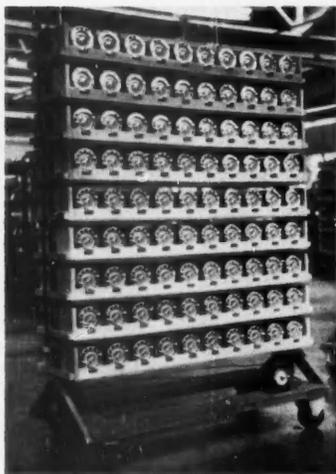
ELECTRIC TIMERS on portable test rack
