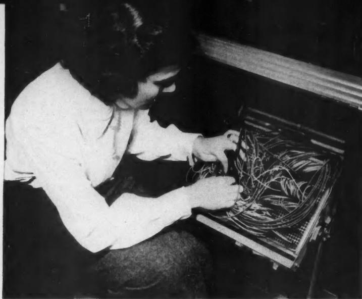
MINOR MODIFICATIONS to the wiring of the control panels can be made quickly with the panels still in the machines. Circuit plugs are easily removed or inserted
