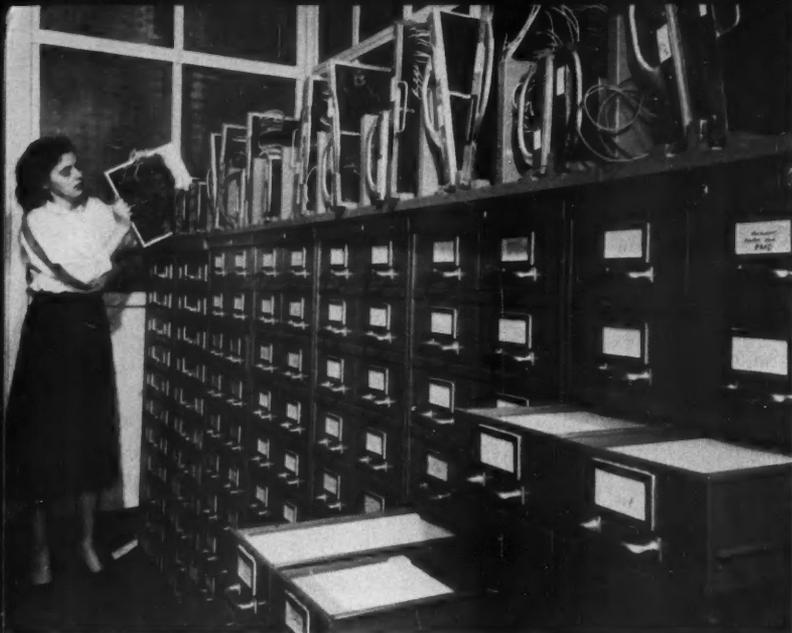
**PERMANENT CONTROL PANELS** for basic operations common to many problems are stored for future use. Cabinets contain punched cards needed for future reference
