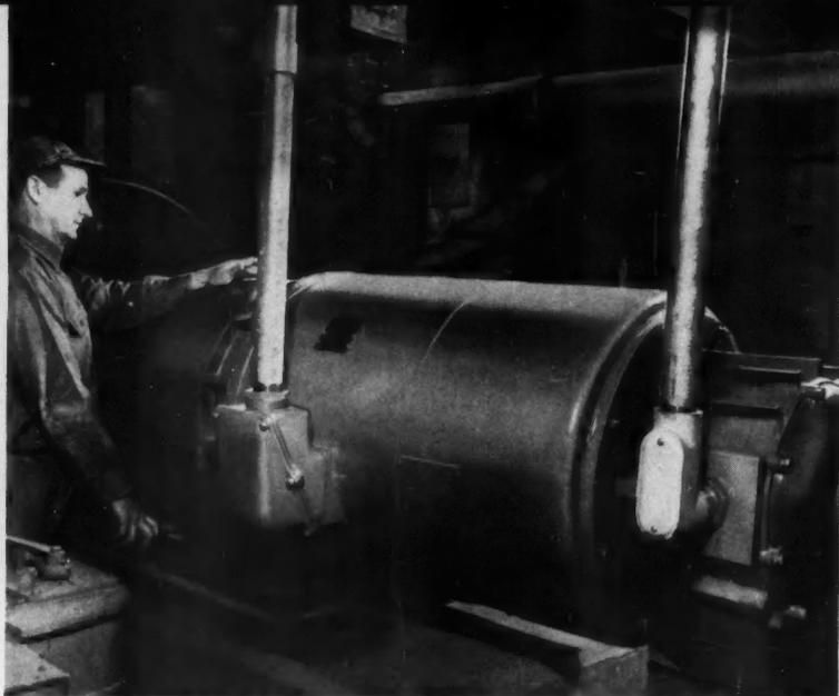
lines. Instead of another motor and speed reducer for new drive, they switched to a 75-hp G-E gear-motor (right) to gain additional power, modern equipment, savings on initial costs.
