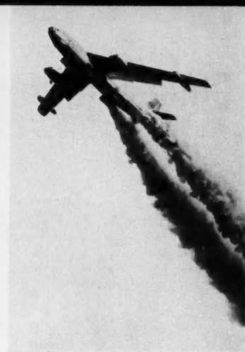
**4** Boeing B-47 Stratojet bomber seen here reaching for altitude with six jet engines and full rocket boost
