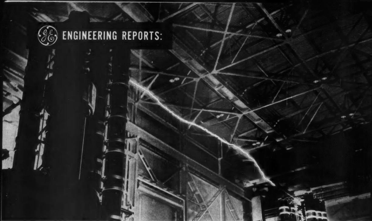
**15,000,000 VOLTS** flash 50 feet between giant lightning generators at the G-E high-voltage lab. Here, lighter, more economical equip-
