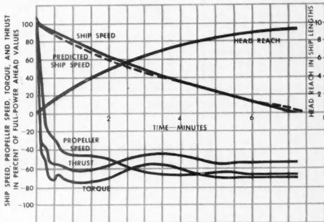
FIG. 5. SHIP-SPEED CURVES FOR A STOPPING MANEUVER ON A TANKER
