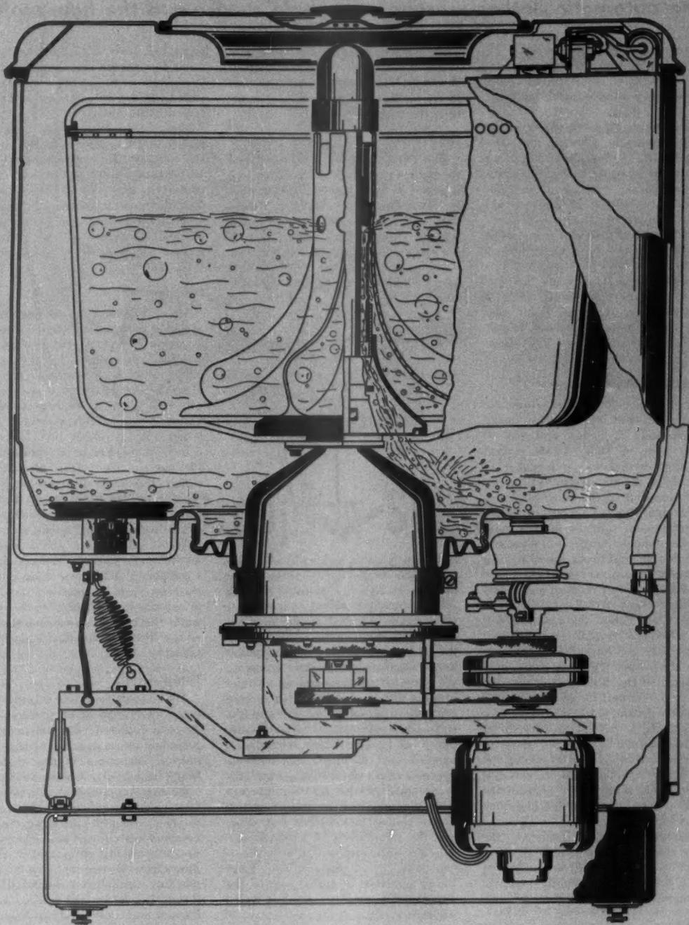
ONE BELT DRIVES THE GEAR-REDUCTION UNIT FOR AGITATING ACTION, THE OTHER DRIVES THE BASKET DIRECTLY FOR SPIN DRYING
