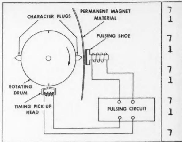
**4** Tabulating device that magnetically prints columns of figures (right), a line-at-a-time at swift speeds
