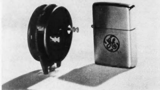
BUTTON RECTIFIER (LEFT) IS ONE OF CAREFULLY SELECTED PAIR THAT IS CONNECTED IN SERIES AND ASSEMBLED TO FORM THE G10 (RIGHT)
