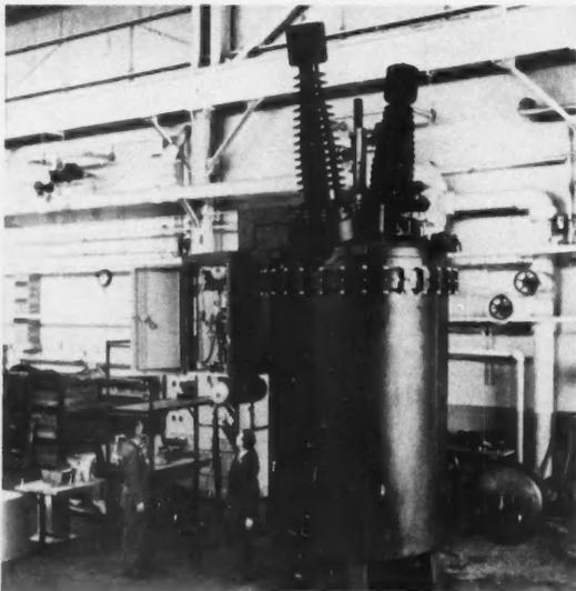
**16** In the assembly shop of the test building, apparatus is prepared for test. After the equipment is assembled on a test car, it is taken to a test cell or the high-voltage yard
