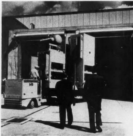
**17** Into one of the five test cells in front of the test building goes a circuit-breaker equipment on its test car. Before it was moved to the cell it went through a "dry-run"
