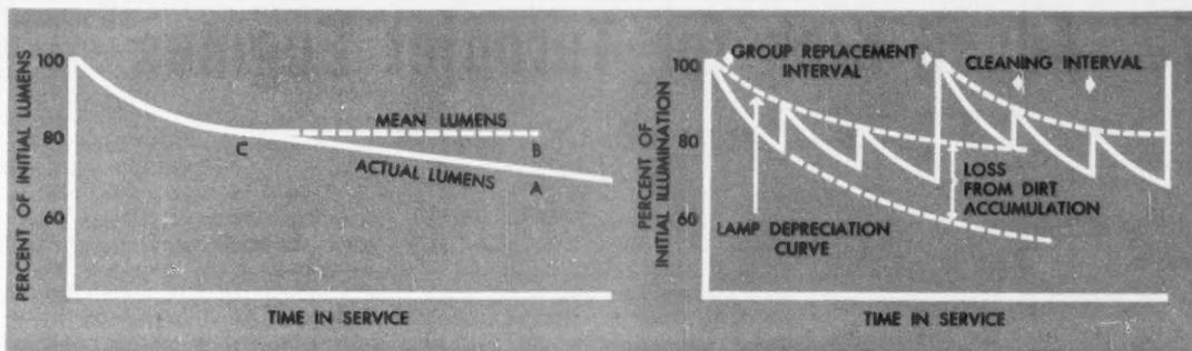
**RELATIONSHIP** between actual and mean lumens of a fluorescent lamp. Lamp remaining in service to point A supplies mean value shown at B. On the time scale, C is 41 percent of A
