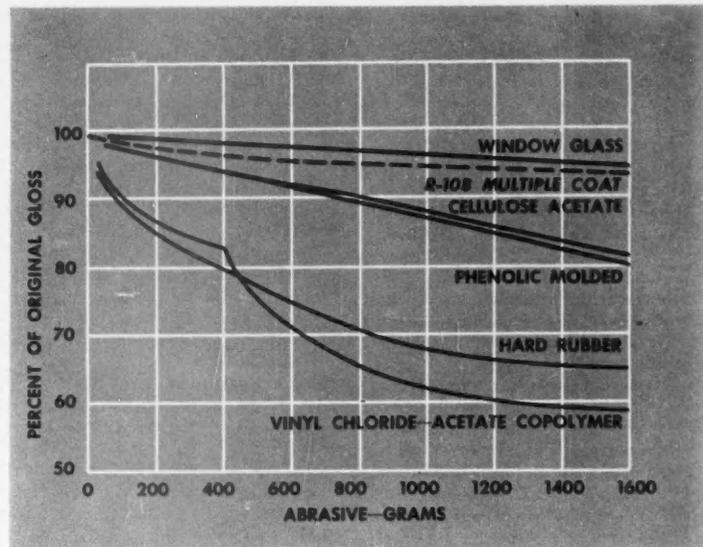
**MAR RESISTANCE** of R-108 multiple coating compared with other materials. Standard ASTM test measures resistance of glossy surfaces to abrasive action
