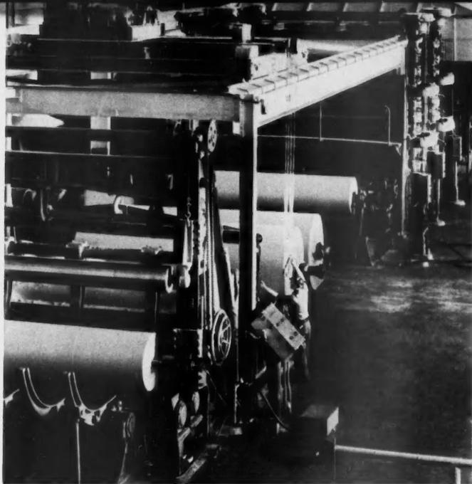
**PAPER MILLS** can rewind finished rolls of paper faster today, thanks to new drive designs indicated by G.E.'s differential analyzer. These improvements provide faster acceleration and deceleration, closer tension control, and greater system stability.
