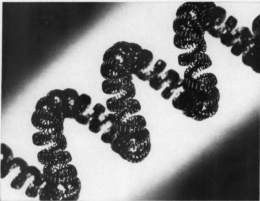
**THE TRIPLE COIL** filament developed by G.E., and shown greatly magnified above, now helps make possible another great new fluorescent lamp.
