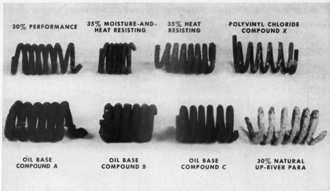
**EFFECT OF MOISTURE ABSORPTION** on rubber insulating compounds after 252 weeks of immersion in water at a temperature of 40 C. Samples originally had same diameter. Oil-base compounds had swollen considerably at the end of 137 weeks, and at the end of 252 weeks they had deteriorated to the extent that the insulation could be readily plucked from the cable
