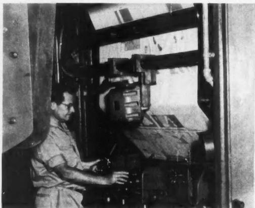
**PRINTING PRESSES** in modern plants like this depend on precision color register control developed by General Electric analytical, design and application engineers in collaboration with purchaser.
