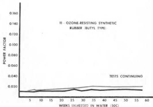
synthetic rubbers, are equal to and in many respects superior to natural rubber for use in insulation compounds. Based on General Electric tests, similarly compounded insulations of either buna-S or natural rubber show generally parallel results. Butyl rubber made possible an ozone-resisting compound having exceptional moisture-and-heat resistant properties, plus good electrical characteristics and aging ability.
