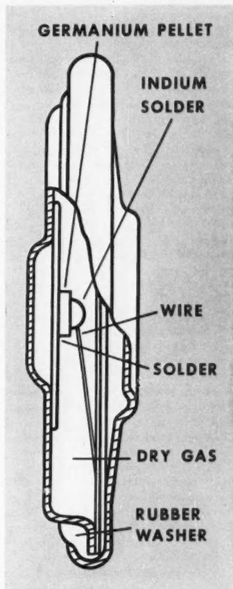
EIGHTH-INCH square pellet of spectroscopically pure germanium is mounted in the center of the button rectifier
