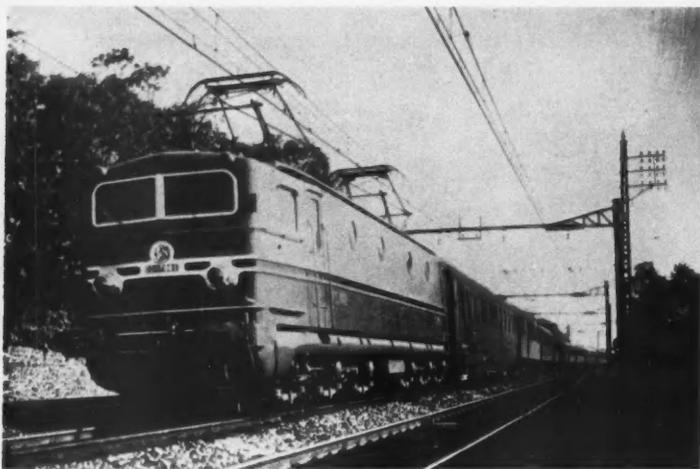
**FRANCE** The newest SNCF high-power high-speed C-C locomotive highballs under the widely used 1500-volt d-c power
