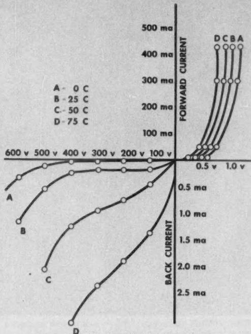
FIG. 1. TEMPERATURE CHARACTERISTICS OF THE G10 RECTIFIER
