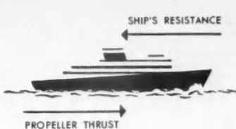
FIG. 2. FORCES ACTING ON THE SHIP
