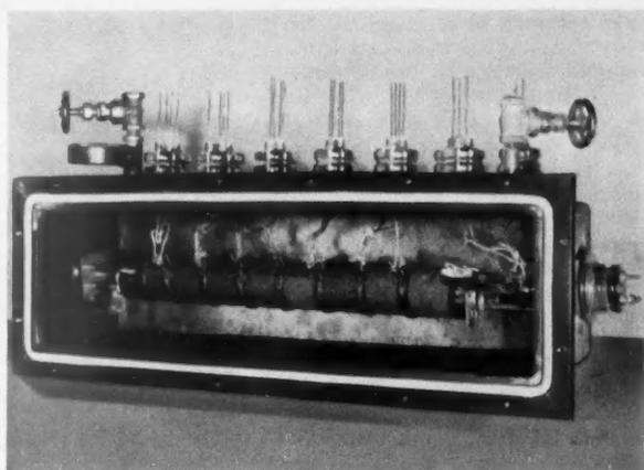
**TEMPERATURE GAIN** made by changing the base insulation material from organic (Class A in Air) to inorganic (Class B in Air) is shown by the curves. To determine the effect of excluding oxygen from Class B insulations, testing chambers (above) that used nitrogen as a gas medium were used. The "Class B in Nitrogen" curve shows that a considerable increase in allowable operating temperature is achieved if oxygen is not present
