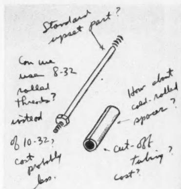
**8** Bentley suggests that possibly two parts can do the same job for less—one a cold-headed part, the other a roll-formed spacer. Next . . .
