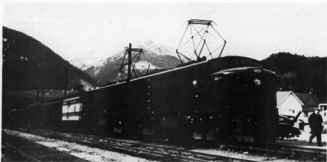
**UNITED STATES** Under 11,000-volt 25-cycle power, this new G-E demonstrator locomotive with a-c commutator motors is in service on the heavy mountain grades of the Great Northern
