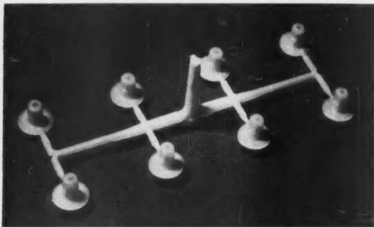
**LIFE TESTS** show this nylon pinion and worm wheel, molded in one piece with gear teeth, is equal to the previously used two-piece steel pinion and laminated worm wheel it replaced in the motor of this 10-inch oscillating household fan
