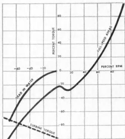
FIG. 4. TYPICAL PROPELLER AND TURBINE TORQUES
