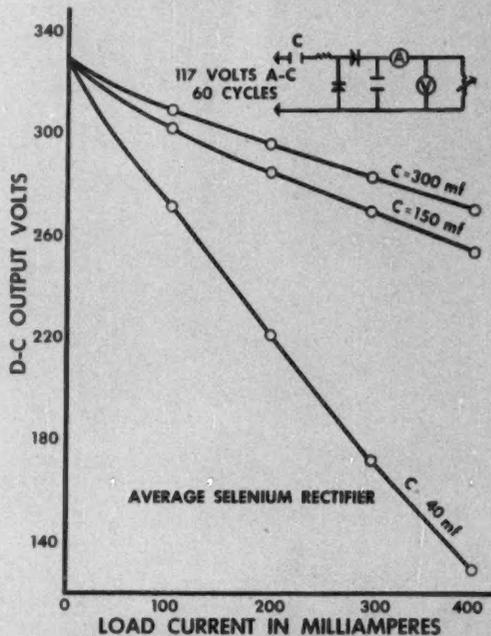
FIG. 4. STATIC CHARACTERISTICS OF A VOLTAGE DOUBLER CIRCUIT
