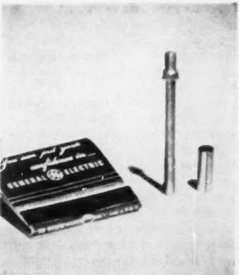
**14** Standard upset part and standard spacer are used at a cost of \$10.50 per thousand. This compares to the original \$52.50 per thousand
