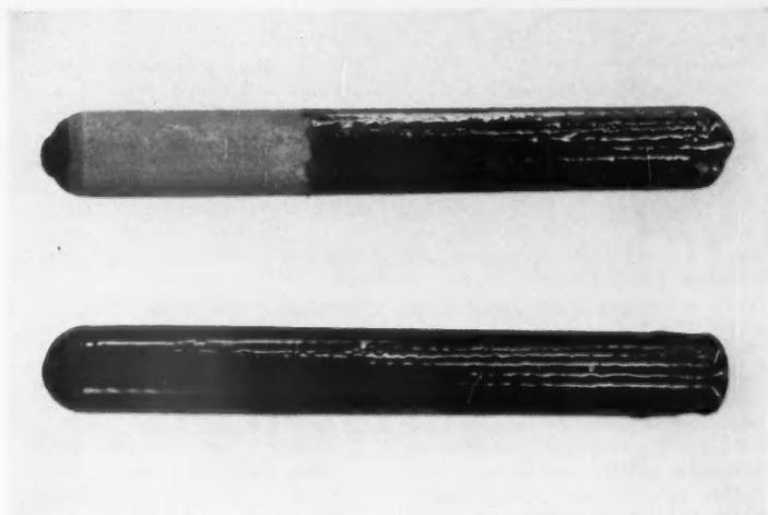
**COMPARISON** of a conventional coating (top) with an R-108 formulation after immersion in a 16 percent caustic solution at temperature of 195 F
