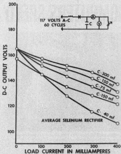
FIG. 3. REGULATION—CAPACITOR CHARACTERISTICS OF THE G10
