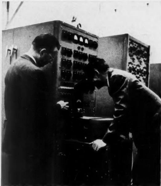
**12** In the test building, two cathode-ray oscillographs record transient phenomena—in millionths of a second—far too rapid to be picked up by magnetic oscillographs
