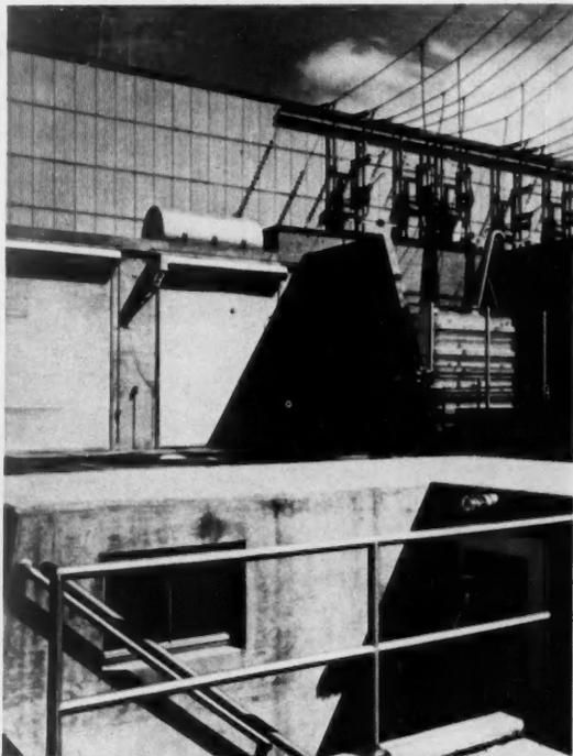
**19** For safety in emergencies, observer in bombproof shelter can instantly halt a test and de-energize all circuits
