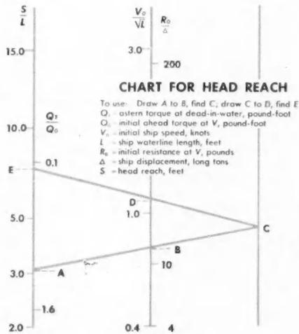
FIG. 6. CHART FOR DETERMINING HEAD REACH
