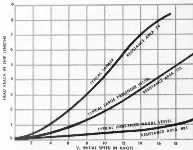
FIG. 7. HEAD REACH IN SHIP LENGTHS FOR THREE TYPES OF SHIPS
