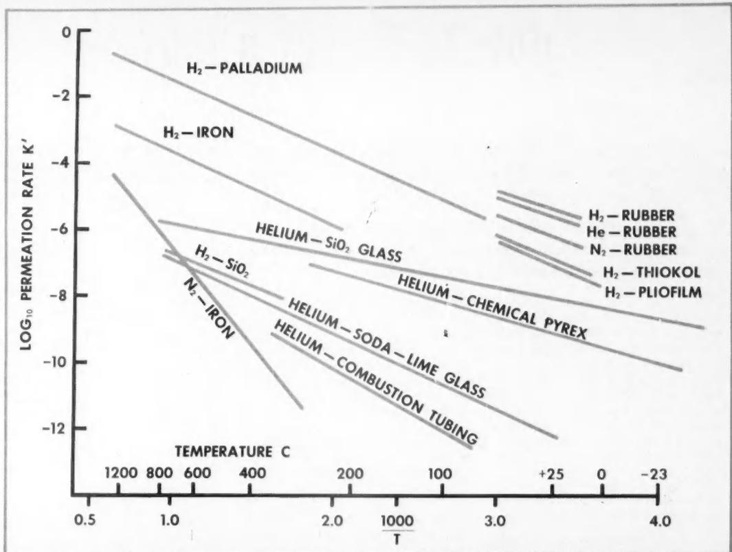
RATE OF PERMEATION of gas through solids. Units for permeation constant  $K'$  are cubic centimeter of gas (at normal temperature and pressure) per second per square centimeter of area per millimeter thickness per one atmosphere partial pressure difference
