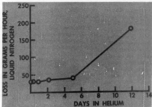
RATE OF LOSS OF LIQUID NITROGEN FROM DEWAR VACUUM FLASK
