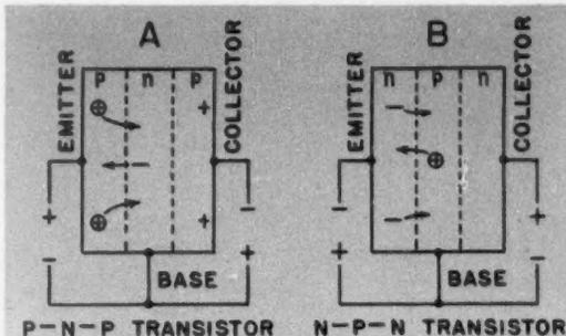
FIG. 2. TRANSISTOR COMPRISES TWO ADJACENT P-N JUNCTIONS
