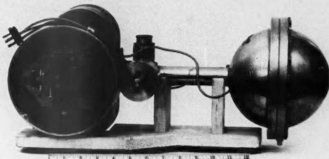
**IONIZATION CHAMBER**, of the type used for cosmic-ray study, was used by researchers for measuring low-level radiation. Spherical chamber is at right, recording camera is at left. This equipment was a forerunner of the type shown on page 20
