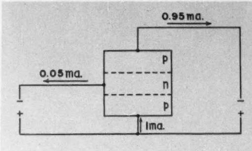
FIG. 4. JUNCTION TRANSISTOR UTILIZES SMALL BASE CURRENT
