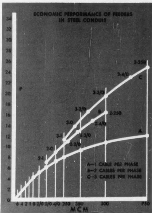
FIG. 3. COMPARISON of curve A with curves of two- and three-conductor feeders point up the advantages of multiple conductors
