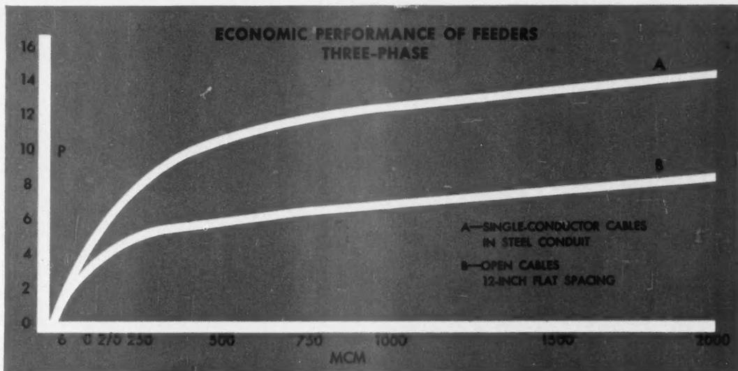
FIG. 1. SMALL INCREASE IN PERFORMANCE CAPABILITY P OF CABLE SIZES 1000 MCM AND UP DOES NOT JUSTIFY ADDITIONAL COST
