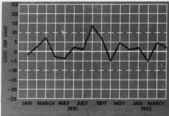
FIG. 4. COST CONTROL CHART FOR MANUFACTURED PRODUCT
