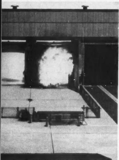
**1 FLASH** in one of five test cells results from deliberately testing a circuit breaker to destruction. Board at right indicates conditions of the test.
