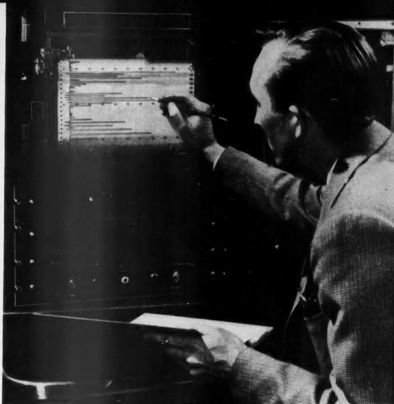
Operator observes cracking pattern of natural gas sample with G-E Mass Spectrometer.
