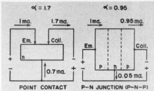
FIG. 3. COMPARISON OF TWO KINDS OF TRANSISTOR OPERATION
