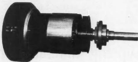
MODIFIED DESIGN SUITABLE FOR USE IN HIGH-SLIP MOTOR
