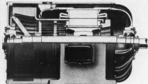
HIGH-SLIP MOTOR CALLED FOR MORE EFFICIENT VENTILATION
