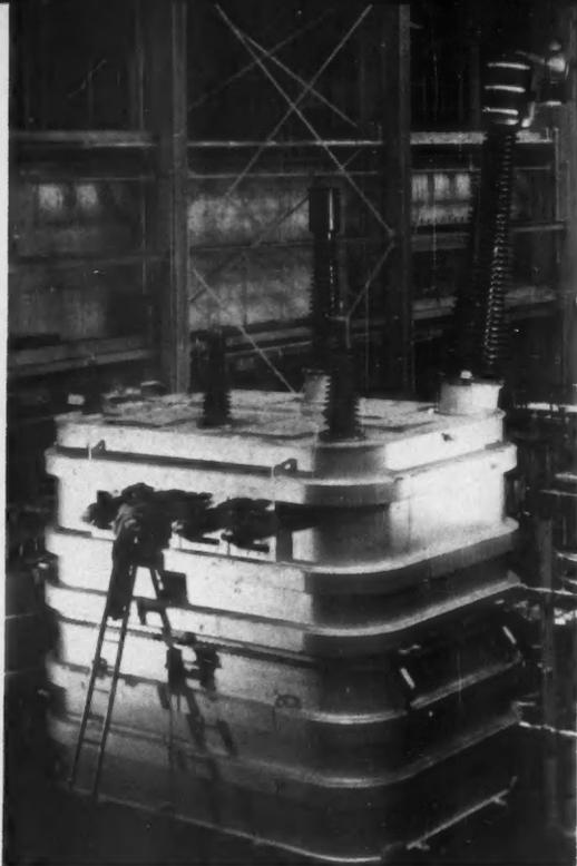
**SPECIAL TRANSFORMER WITHSTANDS 2800 TONS RADIAL FORCE**
