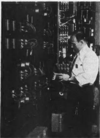
**LONG LIFE AND RELIABILITY** of G-E selenium rectifiers is proved on life test boards. Tests, still in progress, have been running continuously for over 60,000 hours.
