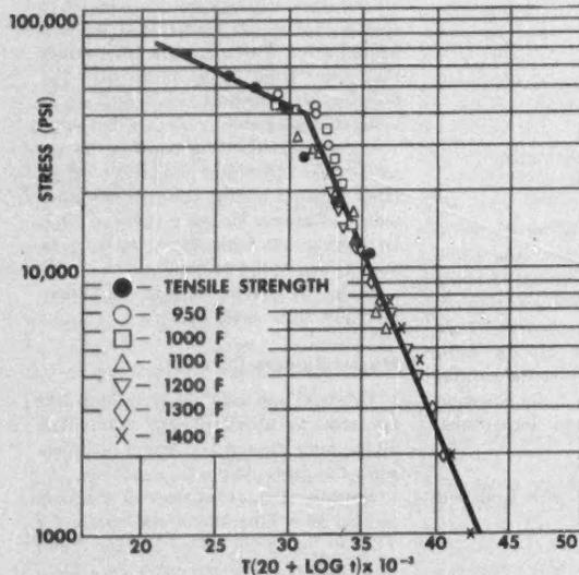
FIG. 3. MASTER RUPTURE CURVE FOR CARBON-MOLY STEEL
