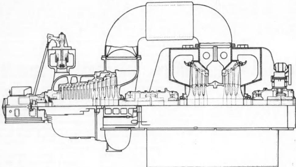
**LOW-PRESSURE UNIT** of cross-compound reheat turbine runs at 1800 rpm and carries remainder of 160,000-kw load. Advantages of this arrangement are a reduction in over-all length, the use of smaller size generators, and lower initial cost
