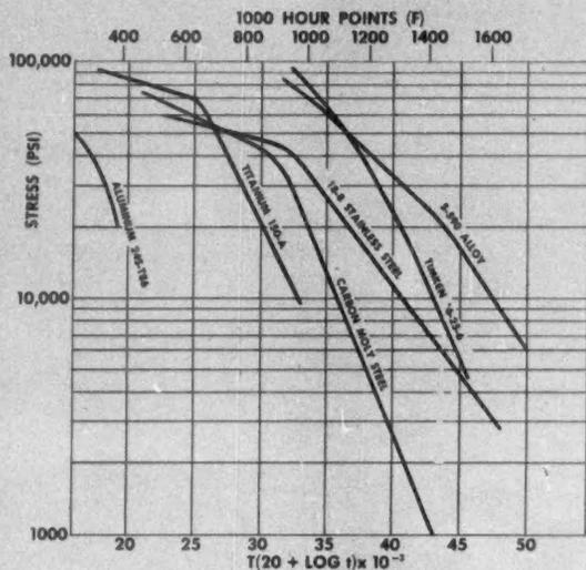
FIG. 5. MASTER RUPTURE CURVES FOR SEVERAL ALLOYS
