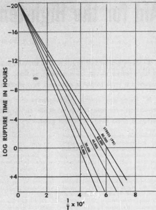
FIG. 2. VALUE OF C FOR THE S-590 ALLOY IS EXACTLY 20
