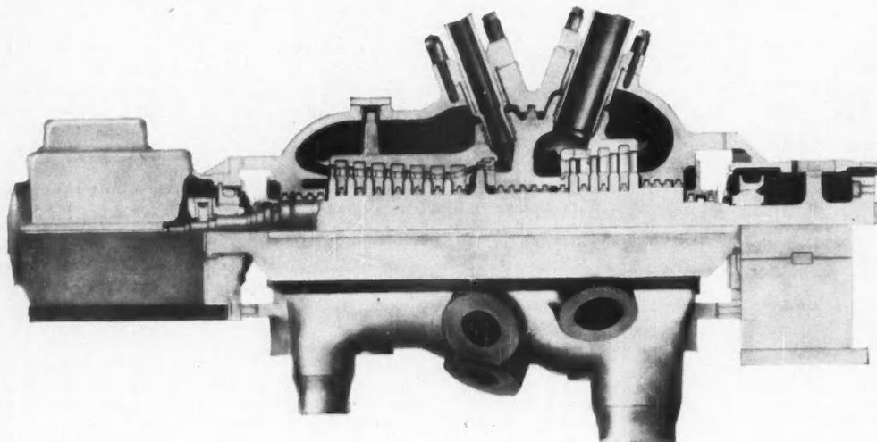
**HIGH-PRESSURE UNIT** of a 160,000-kw cross-compound reheat turbine runs at 3600 rpm and carries approximately 37 percent of the rated load. Steam to the low-pressure unit (below) is reheated in the high-pressure unit or as it crosses over
