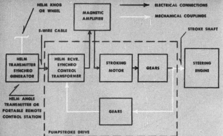
**FIVE-WIRE CABLE** that transmits helm order information is the only connection between the control station and steering engine located in the stern of the ship
