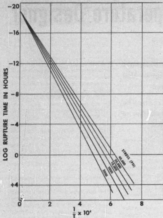
FIG. 1. TIME AXIS INTERCEPT IS C FOR CARBON-MOLY STEEL
