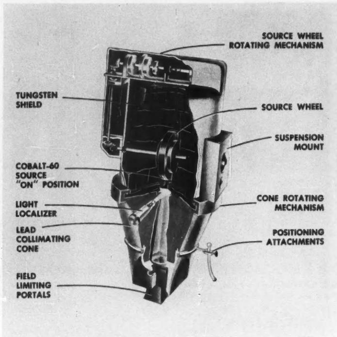
**COBALT-60 UNIT** combines good shielding for the operator with simplified control of gamma-ray beam. Treatment cones accommodate various field sizes
