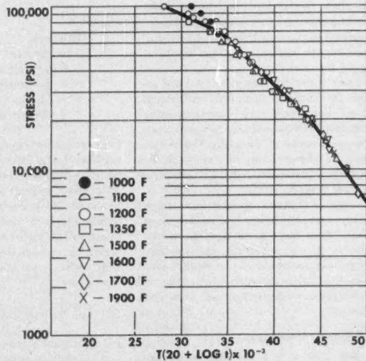
FIG. 4. MASTER RUPTURE CURVE FOR THE S-590 ALLOY
