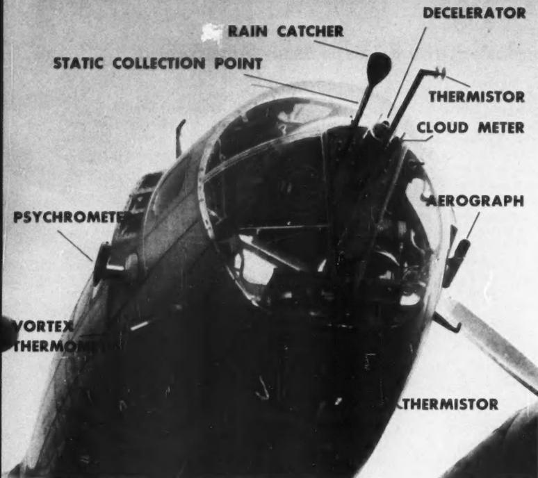
**FLIGHT INSTRUMENTS** mounted in the nose of a Project Cirrus B-17 include: static collection point to measure variations in the electrical potential of the atmosphere, a rain catcher to give average value of the precipitation in the air for approximately each 1000 feet of flight, and a decelerator to slow down the air and assist in sorting out rain, snow, dust, or cloud particles from the atmosphere as the plane passes through. A thermistor records temperatures, a
