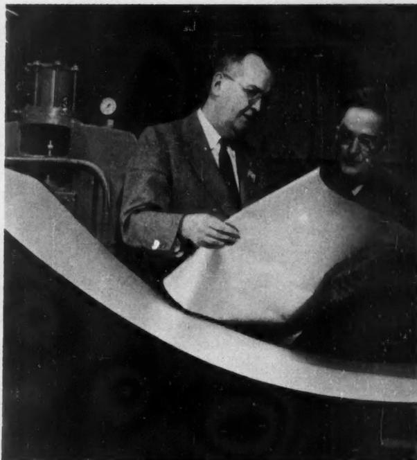
PAPER MACHINE (ABOVE) MAKES MICA MAT IN CONTINUOUS LENGTHS FOR INSULATION IN VARIOUS TYPES OF ELECTRICAL APPARATUS
