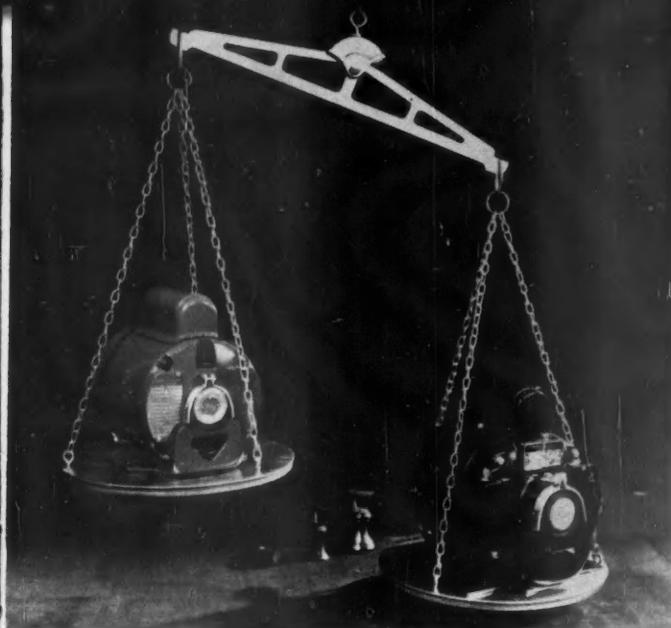
**SMALLER, LIGHTER**—Fractional-horsepower motor (left) is 51 percent less per horsepower in weight than a former model
