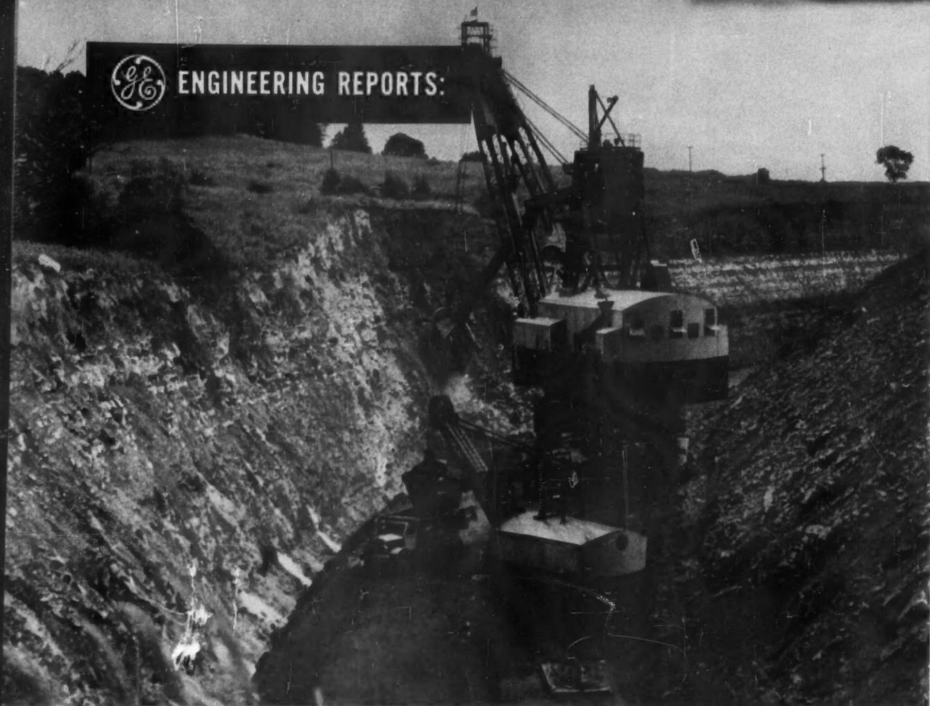
**MINING** output has been increased by amplidyne control engineered into electric shovels and mine hoists, including giant strippers like this. Instant shovel response, plus faster accel-
