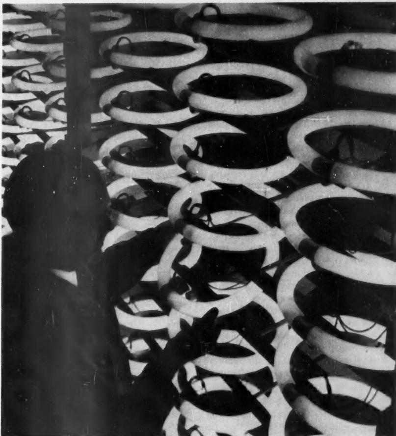
**CIRCLINE FLUORESCENT LAMPS** are now made in 8-, 12-, and 16-inch diameter sizes. For some purposes they are more effective than straight tubes
