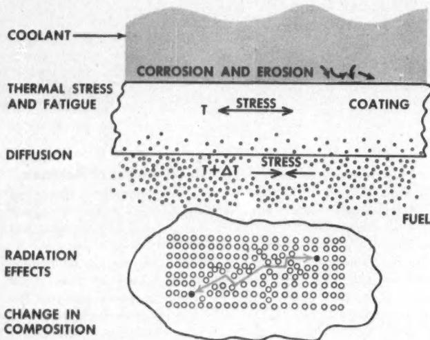
**JACKETING OF URANIUM** in a nuclear reactor is necessary to prevent corrosion by the coolant. Thermal stresses and interdiffusion are other important problems.
