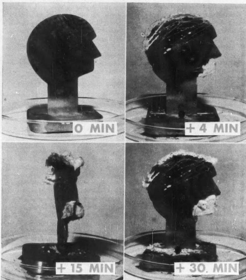
**CORROSION OF ALUMINUM** in moist air following rupture of the protective film by scratching the aluminum head under mercury. Times shown are "minutes after scratching."
