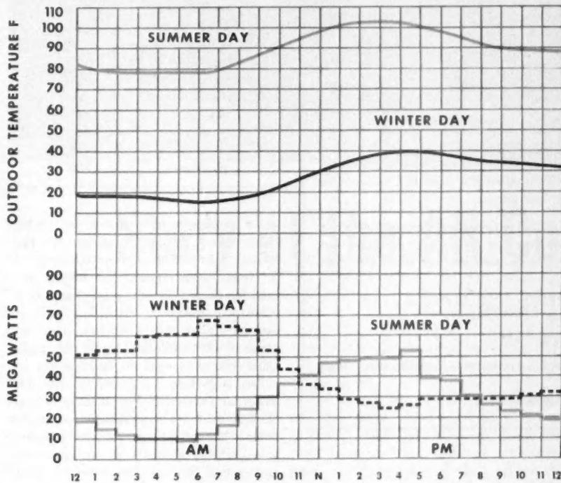
**FIG. 3. ELECTRIC LOAD CURVE** calculated for 8000 all-electric homes with heat-pump systems. In Southern locale, daytime energy consumption is greater in summer than winter.
