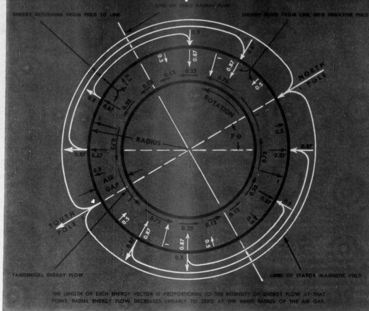
FIG. 6. FLOW OF MAGNETIC ENERGY IN NO-LOAD FIELD OF POLYPHASE (TWO-POLE) INDUCTION MOTOR.
