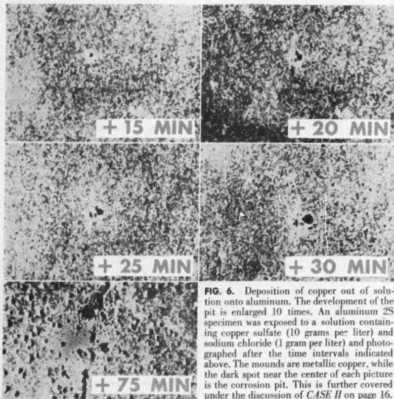
FIG. 6. Deposition of copper out of solution onto aluminum. The development of the pit is enlarged 10 times. An aluminum 2S specimen was exposed to a solution containing copper sulfate (10 grams per liter) and sodium chloride (1 gram per liter) and photographed after the time intervals indicated above. The mounds are metallic copper, while the dark spot near the center of each picture is the corrosion pit. This is further covered under the discussion of CASE II on page 16.
