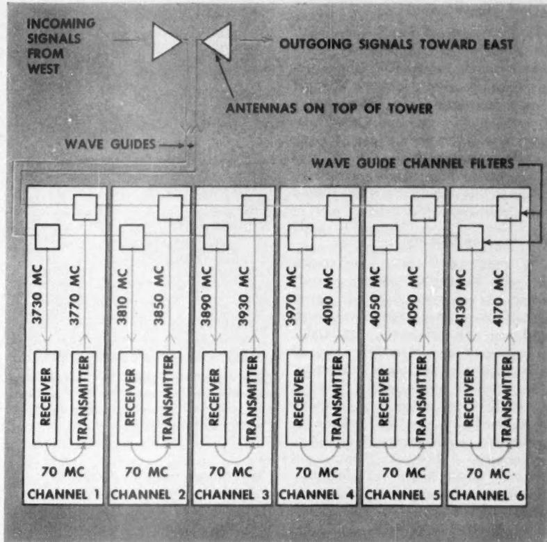
**REPEATER BAY** arrangements and frequency translations at a typical TD-2 relay station. For transmission in the opposite direction duplicate arrangements are used.
