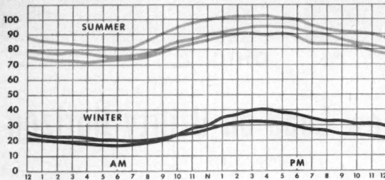
**FIG. 1. HOURLY OUTDOOR TEMPERATURES** of some of warmest summer days and coldest winter days in a southern location. Lowest temperatures usually run from six to seven am.
