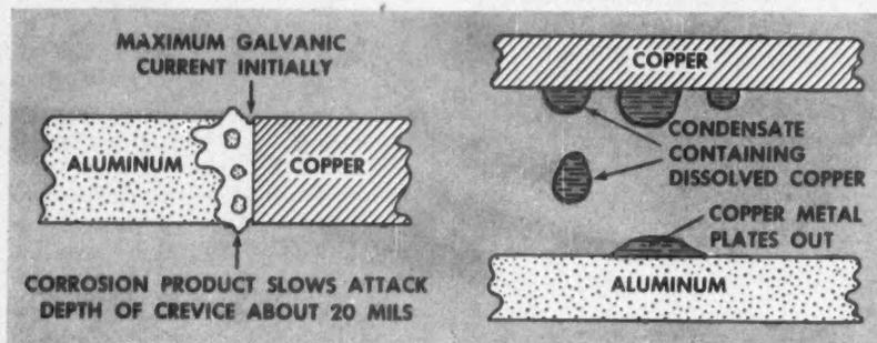
FIG. 4. Butt-welded aluminum and copper joint 30 days in salt spray.
