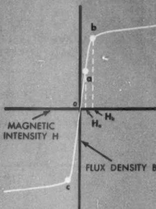
FIG. 2. B-H CHARACTERISTICS OF THE CORE MATERIAL
