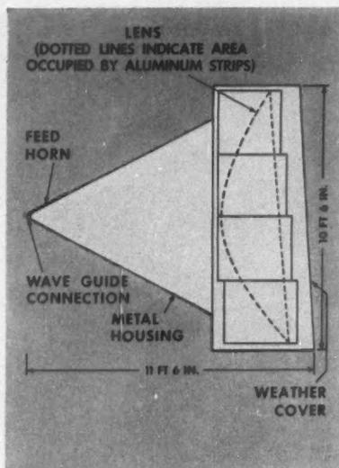
**DELAY LENS ANTENNA** has metallic lens that concentrates outgoing energy in a narrow beam and focuses incoming energy at the apex of the feed horn.
