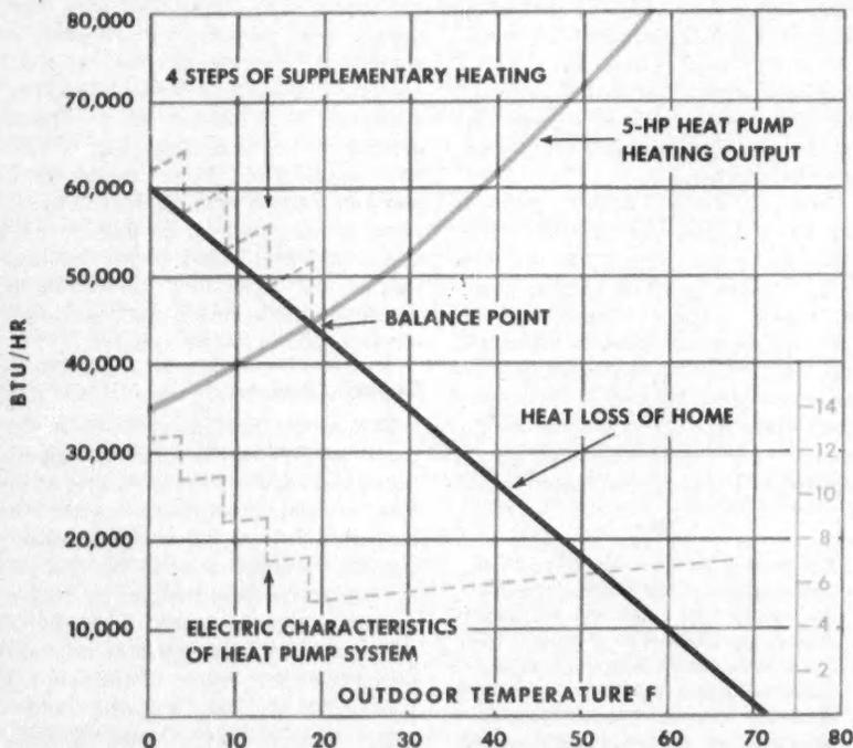
**FIG. 2. HEAT BALANCE DIAGRAM** for a heat-pump system applied to a home in Southern location. At the design temperature of zero F the home's heat loss is 60,000 Btu/hr.
