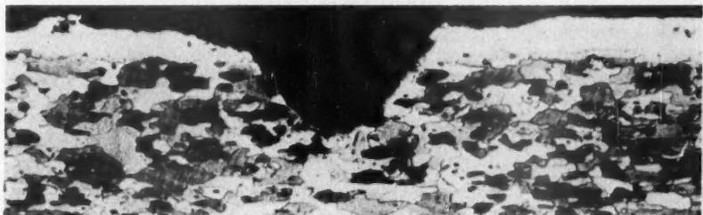
**FIG. 9.** This is the cross section of an alclad 17S-T4 (-T) sheet (0.040 inch thick) showing electrolytic protection of the core which was exposed by a deep scratch. No corrosion of the core occurred during six years' exposure to the atmosphere at New Kensington, Pa. Note sacrificial attack of coating adjacent to the scratch. (This cross section is enlarged 100 times and the sample was etched with HF-HCL-HNO<sub>3</sub>.)
