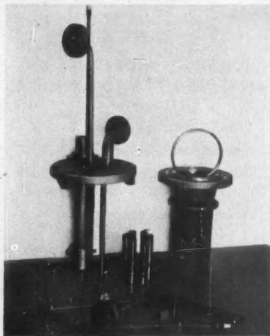
**LIQUID SODIUM** was tested in this device to determine its corrosiveness toward possible structural materials.
