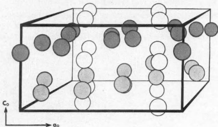
**BETA PHASE** of uranium has this complex tetragonal structure—one of the most complicated ever found for a pure metal.
