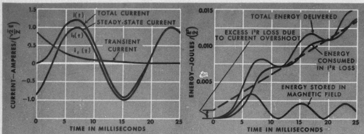
FIGS. 4 AND 5. INSTANTANEOUS CURRENT AND ENERGY COMPONENTS IN A SINGLE-PHASE RL CIRCUIT WITH 0.5 POWER FACTOR AT 60 CYCLES.
