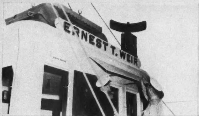
**BARREL STAVE** antenna on this electronic navigator is used for surface search on small ships; helps them navigate in all types of weather.
