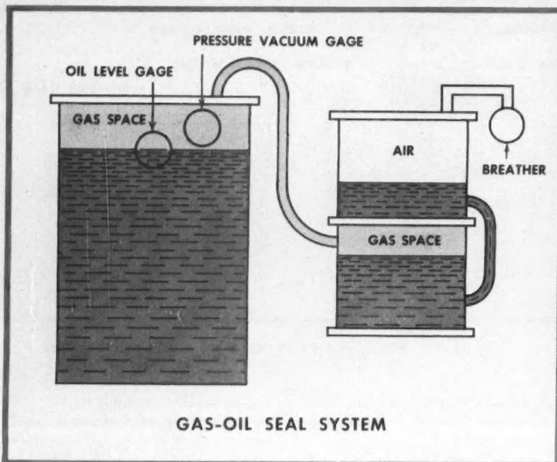
**FIG. 3. GAS-OIL SEAL** makes use of a gas space in the main tank and a variable column of oil in an auxiliary tank to seal out atmosphere and seal in gas.
