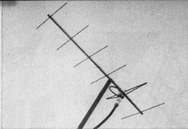
**YAGI** type UHF-TV receiving antenna for home sets. A directional unit like this has a power gain of about 10 to 1 over a single dipole, or 3.16 to 1 in signal gain.
