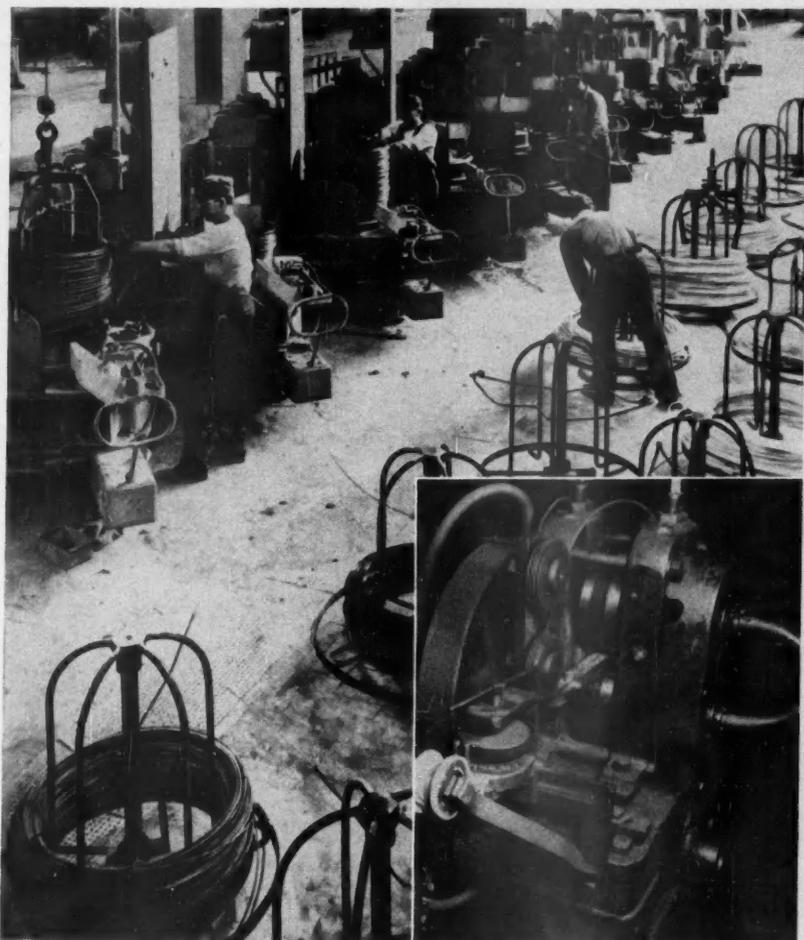
**WIRE DRAWING** with Carboloy carbide dies was first American application of tungsten-carbide. Wear resistance of dies (inset) considerably speeded production and reduced costs.
