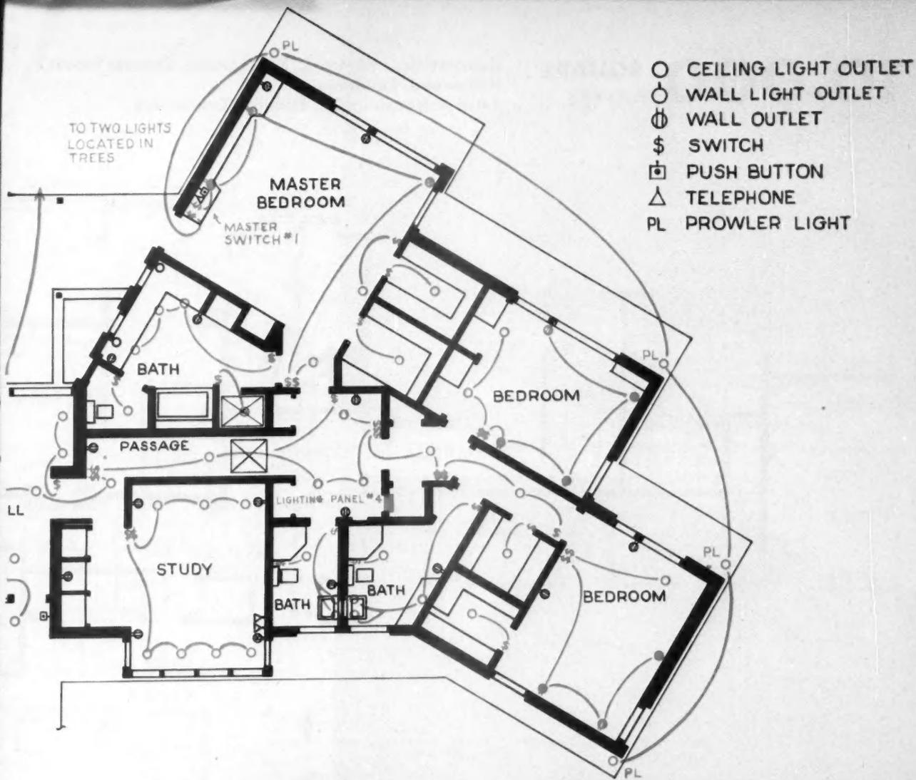
**GREEN LINES** on the floor plan show location of switches and outlet, light, or device controlled. Note location of the four lighting panels. Relays for the areas served by each panel are grouped near the panel. One master switch is in the master bedroom, the other near the main entrance. Because of space limitations, not all features of the house can be shown.
