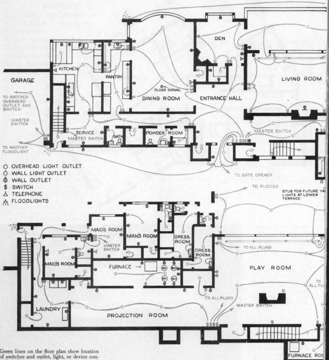
Green lines on the floor plan show location of switches and outlet, light, or device controlled. Because of space limitations, not all features of the house can be shown.
