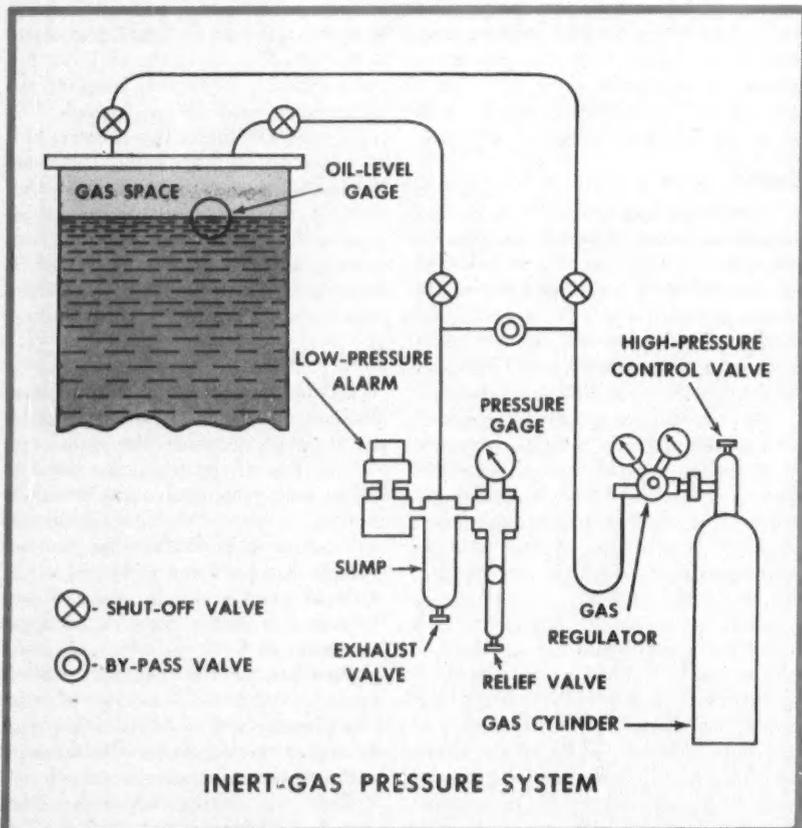
**FIG. 4. INERT-GAS PRESSURE** is most elaborate system. But gas source and control equipment maintain a positive pressure on the oil in several transformers.
