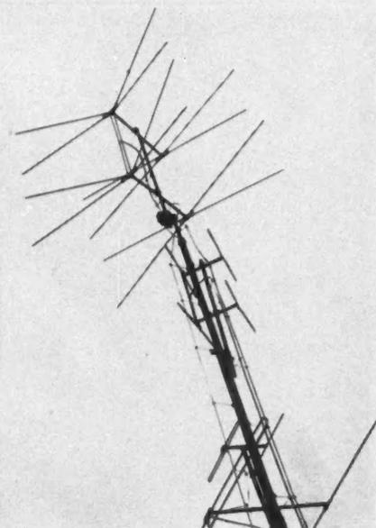
**STACKED YAGI** at the middle of the mast is a channel 8 stacked two-element beam antenna. Above it is a "Telorex" consisting of a stacked conical array. The "Hi-Lo" band antenna at the bottom consists of two two-element antennas—one covers high VHF-TV channels, the other covers low VHF channels.
