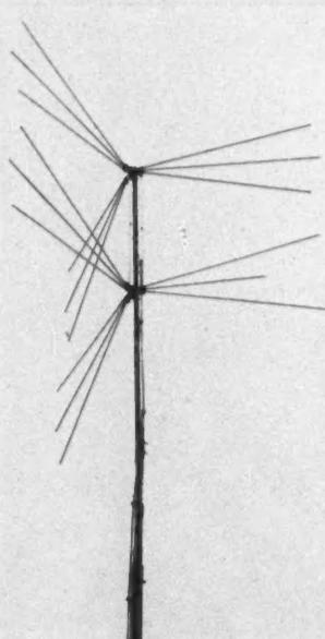
**SNYDER** is unique because a three-conductor transmission line is used along with a selector switch. TV signals may be received from any direction by using the switch to cut in any pair of elements. The antenna proper has three fan-type elements arranged at 120 degrees in a horizontal plane.
