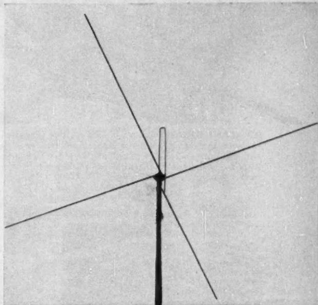
**UNIPOLE** very-high frequency (VHF) omnidirectional antenna for operation at 40 mc. This unit is used with 50- and 250-watt base-station transmitters and receivers for two-way radio communication systems such as police, fire, and taxis.
