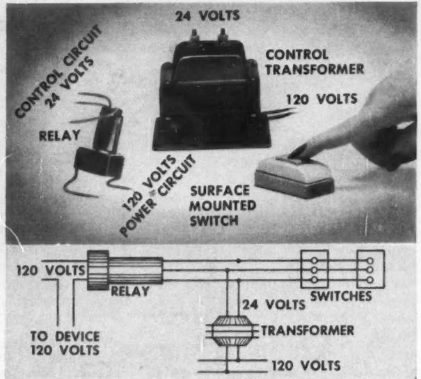
TREND IN CONTEMPORARY HOMES IS TO REMOTE-CONTROL WIRING SYSTEM BECAUSE OF VERSATILITY OF COMPONENTS (ABOVE)
