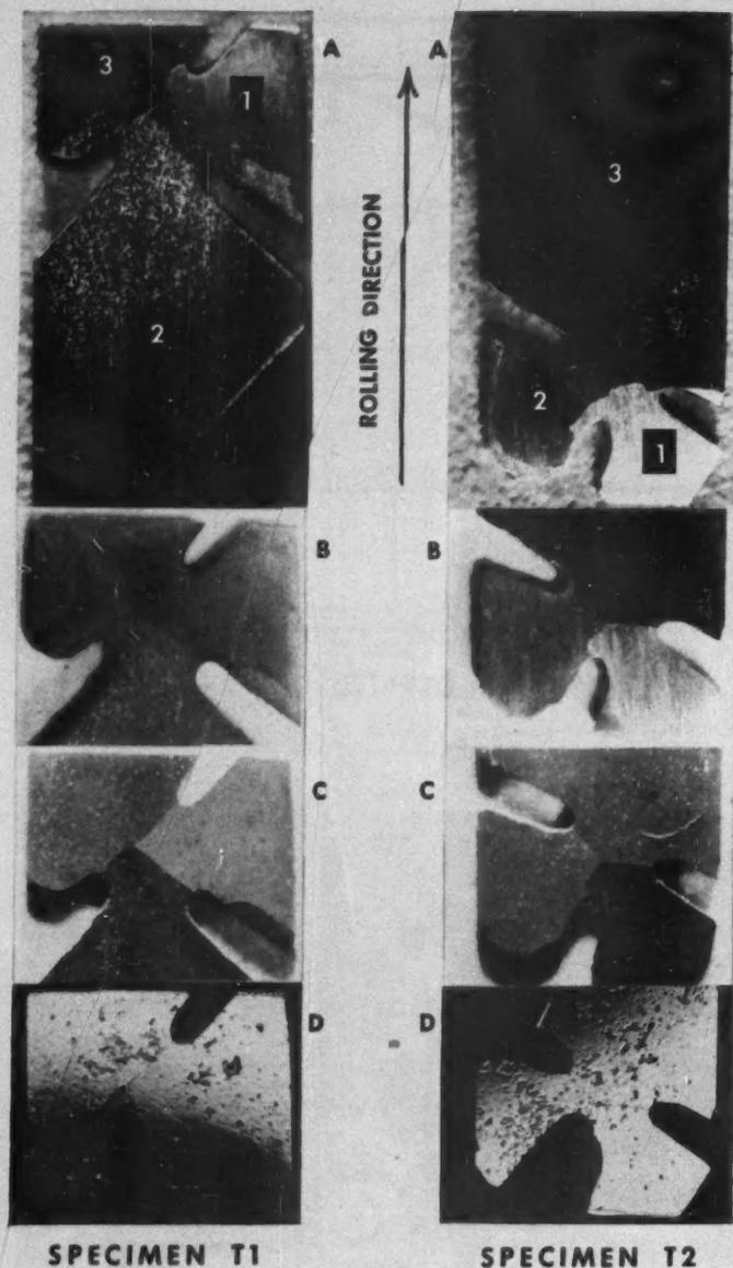
FIG. 4. GRAIN GROWTH of three-grain specimens: A, original specimens; B, after heating 12 hours at 1300 C; C, fifth anneal; D, final anneal. In specimen T1 grain three grows at expense of its neighbors. Metallurgists attribute grain growth to internal energies induced in grains by cold working of metal.
