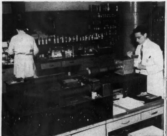
**CHEMICAL**, dye, paint and ink companies record color automatically, accurately, with the recording spectrophotometer, applied by G-E engineers to assure exact color control and matching.
