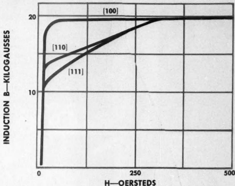
FIG. 2. MAGNETIC PROPERTIES along cube's edge are superior to other major directions. Present orientation of transformer steel has cube edge in rolling direction.
