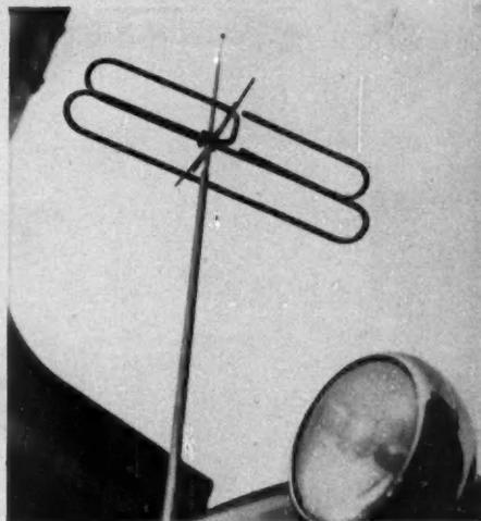
**HOT-ROD SPECIAL** is of dubious value both for radio reception and appearance; may prove to be a lethal instrument in case of a bad accident.
