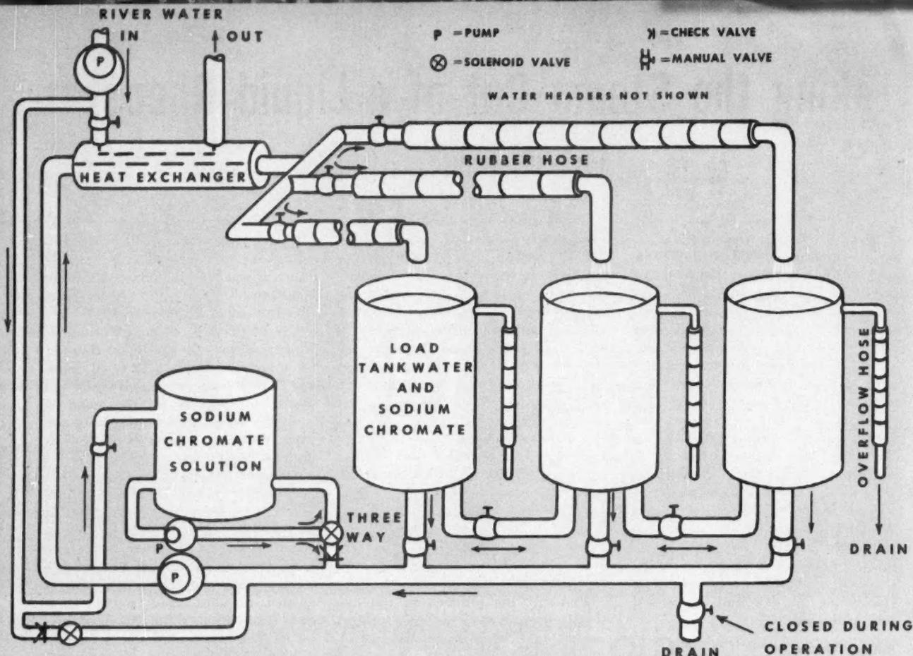
**SIMPLIFIED PIPING DIAGRAM OF WATER RHEOSTAT**
