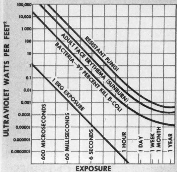
**AIR** carries bacteria, yeasts, molds, and viruses. But its circulation past germicidal lamps in air-conditioning systems effectively destroys them because repeated . . .
