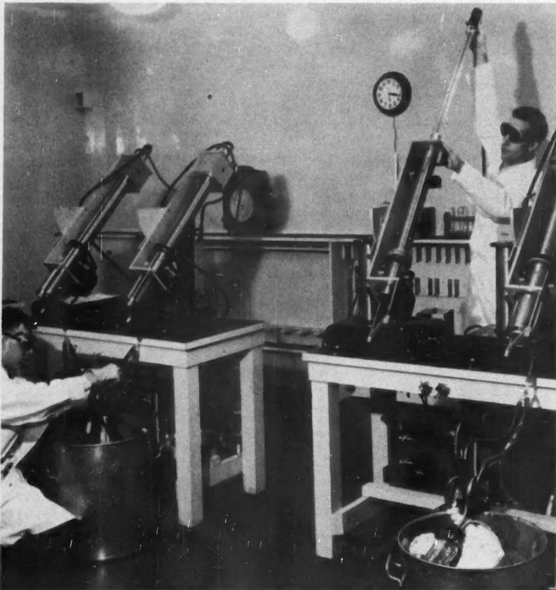
**BLOOD PLASMA** is disinfected of jaundice virus the Army way. GI medics expose thin plasma films moving along the inner surfaces of metal cylinders to intense radiation of germicidal lamps. Concentrated blood has a low ultraviolet transmission. Milk can be pasteurized the same way.
