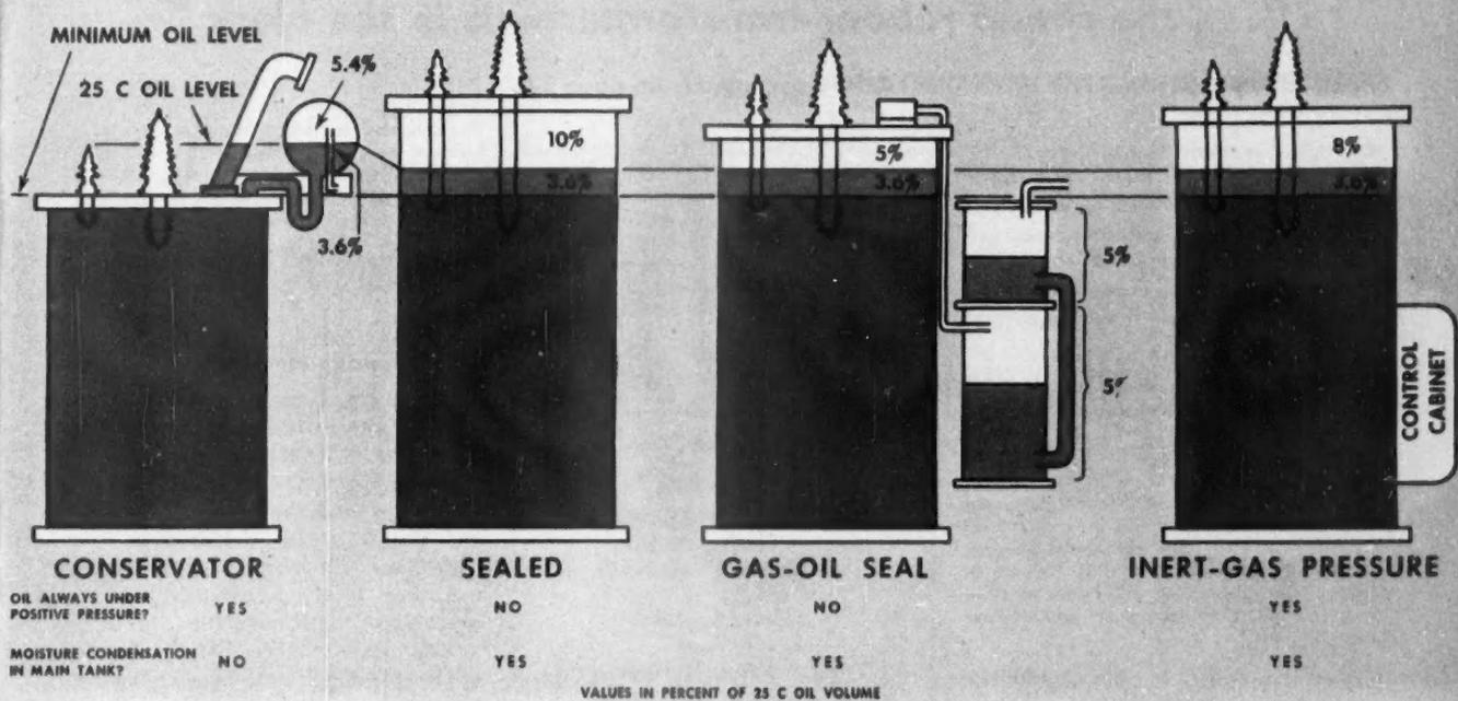
pressure is exerted in the transformer at all times. One set of control equipment and one source of gas can maintain the gas pressure for a group of transformers.
