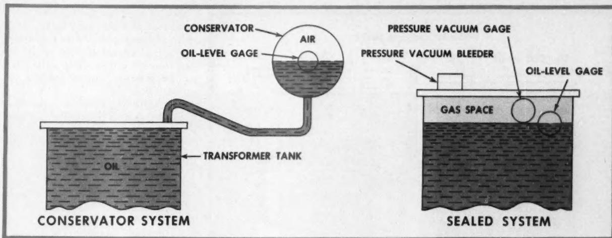
**FIG. 1. CONSERVATOR** keeps air, the trouble maker, from chemically reacting with oil in main transformer tank.
