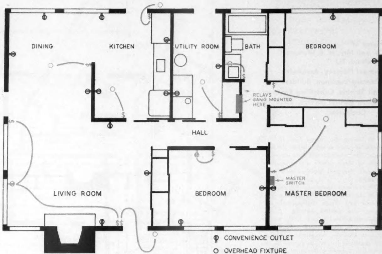
GREEN LINES SHOW LOCATION OF SWITCHES, AND OUTLETS OR LIGHTS CONTROLLED. RELAYS ARE "GANG-MOUNTED" IN HALLWAY.
