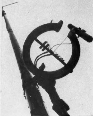
**DONUT**, or "loop-type folded dipole," with de-icing equipment undergoes temperature rise tests. Antennas like this are used for FM transmission.
