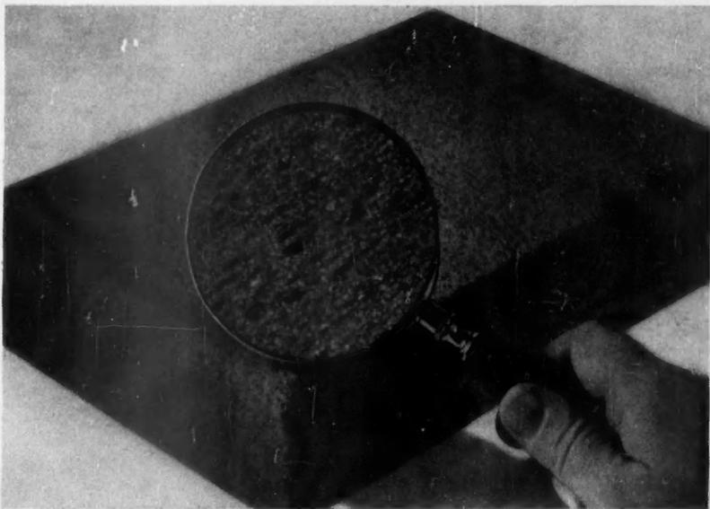
**AIR POCKETS** enclosed by solid resin films make up the expanded phenolic foam. About two-thirds of these air pockets are independent cells—the others are interconnected.
