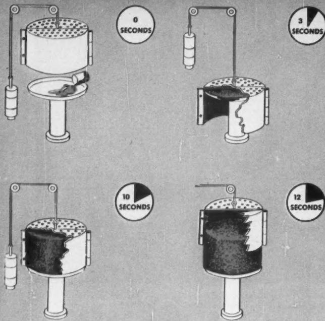
**COUNTER-BALANCED** apparatus for expanding catalyzed resin with a minimum amount of friction. Mold moves upward during expansion, does away with voids, tears, and blowholes in foam.
