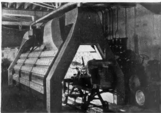
97.5 kw. infra-red oven drying finish coat on complete tractor assemblies.
