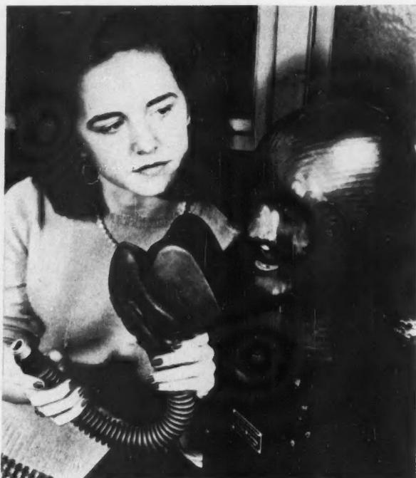
HEAD THAT BREATHES IS WIRED TO SIMULATE HUMAN SKIN TEMPERATURES; COMPLETE WITH ITS FINAL LATEX COATING (RIGHT).
