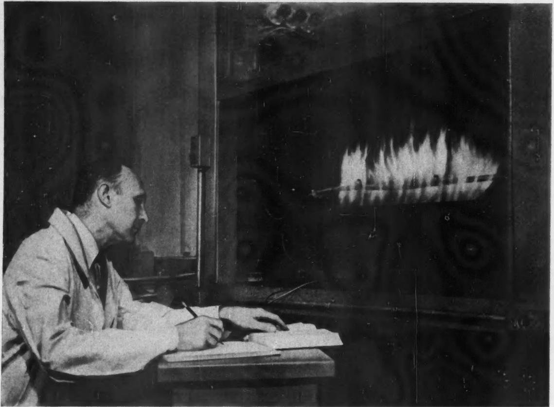
New cable withstands 1400 F flame for 24 hours in grueling laboratory test.
