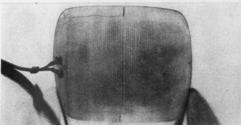
THERMOPLASTIC LENS IS ELECTRICALLY HEATED TO DEFROST AIRCREW GOGGLES.
