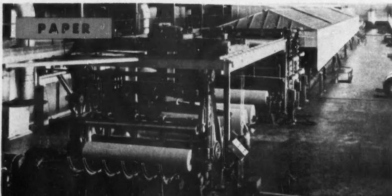
**AMPLIDYNE-ELECTRONIC**—To increase the amplidyne's ratio of amplification, a stage of electronic tubes is introduced. With this arrangement the operating speeds of paper machines have increased substantially since World War II. Tissue paper, for example, is produced at speeds 50 percent higher. Amplidyne-electronic control has made a notable contribution in the paper industry because its reliability and precision permit continuous production of high-quality paper.
