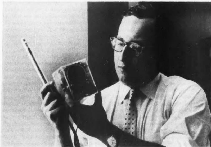
**TRANSISTORIZED RADIO RECEIVER**—a developmental project—operates from a ferrite loop antenna. Despite its small size the receiver has good quality and clarity of tone.
