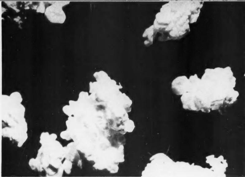
**AGGREGATES** of polytetrafluoroethylene powder (*magnified*) in silicone rubber. The fibrous elastomer is unusually tough and resistant to high-temperature lubricants.
