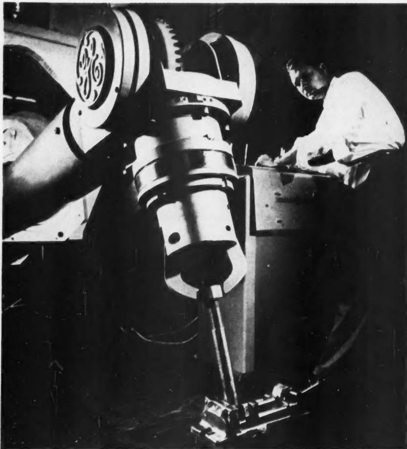
GIANT MANIPULATOR ASSEMBLES OR DISASSEMBLES MACHINERY IN RADIOACTIVE AREAS.
