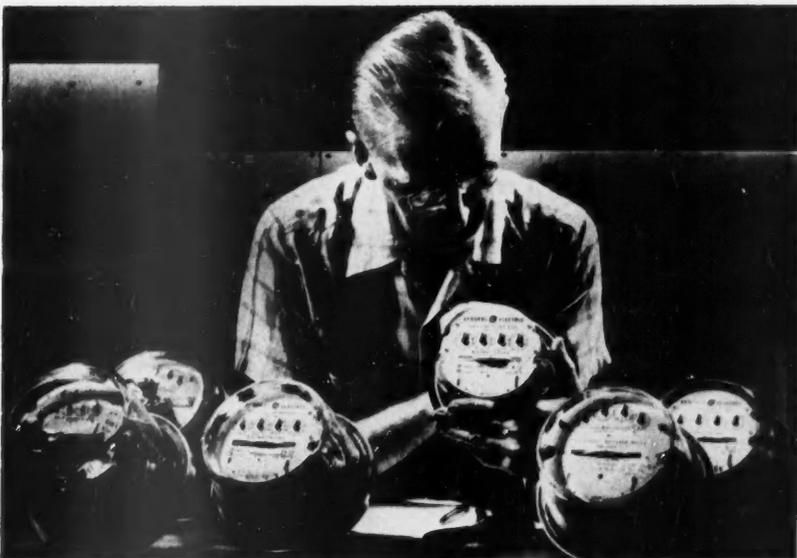
**WATTHOUR METERS** with nominal 50-amp rating are capable of continuous operation up to 200 amp. Temperature rise under this load is 20 C lower than that of former meters.
