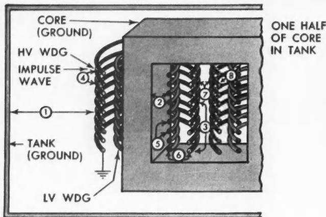
**MAXIMUM VOLTAGES THE TRANSFORMER DESIGN ENGINEER MUST KNOW . . .**
