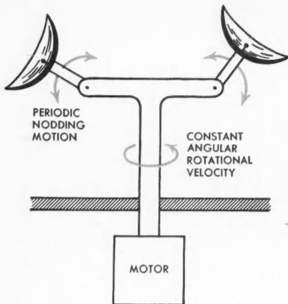
**PROBLEM: ANTENNA DRIVE SYSTEM**—Given the physical dimensions, find torques the motor must produce to drive the system.
