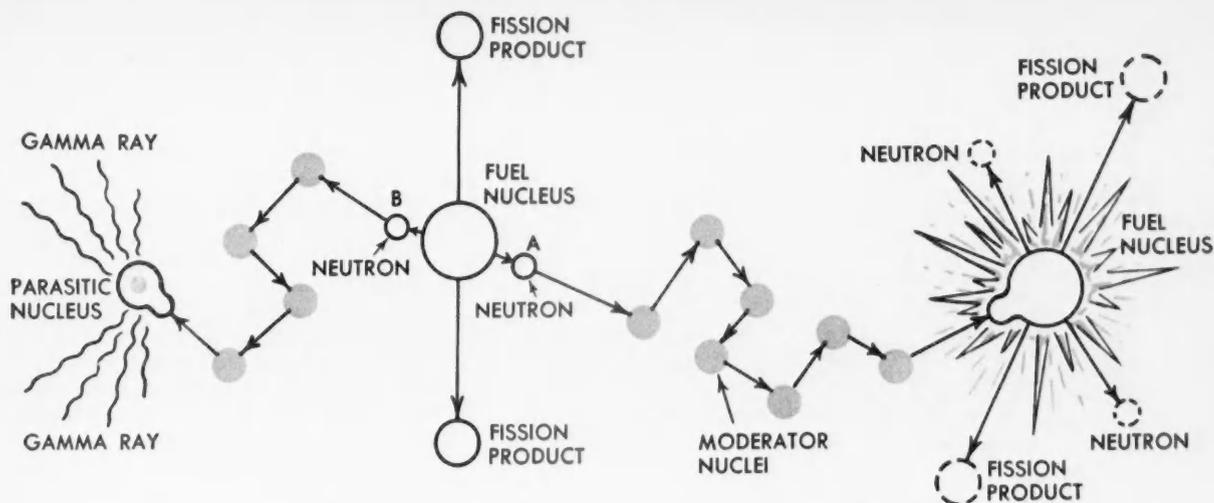
PARASITIC CAPTURE BY OTHER ELEMENTS, ELASTIC SCATTERING, AND FISSION WITH A FUEL NUCLEUS ARE BASIC NEUTRON INTERACTIONS.
