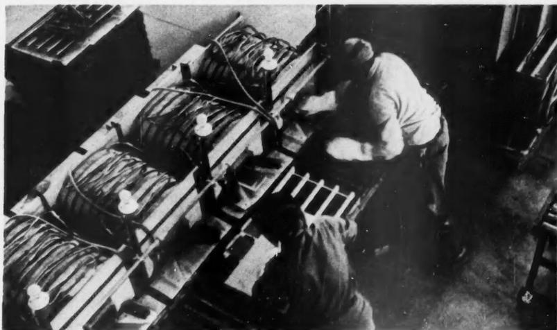
**8** ... for heat treating in a roller-hearth furnace (upper right). After heat treating, the boats are pushed into magnetizing solenoids (above) where they cool.
