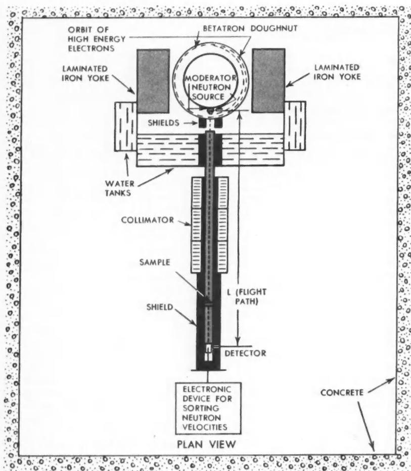
**FIG. 2. VELOCITY SELECTOR** measures time of flight of neutrons traveling fixed distance  $L$ . Betatron rated 100 Mev emits bursts of neutrons every one-sixtieth second.
