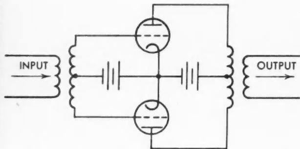
**PUSH-PULL** amplifiers using n-p-n and p-n-p transistors or electron tubes are often used for high-fidelity phonograph equipment.
