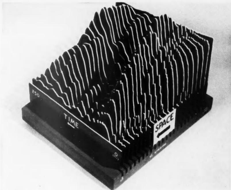
**VOLTAGE DISTRIBUTION** along length of simple helical coil in air—from conductor to ground—when the coil is impulsed by simplest type of transient voltage wave.
