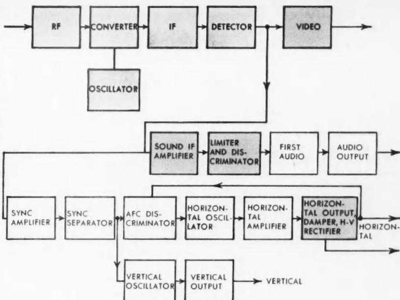
**SOME TV RECEIVER CIRCUITS** can use commercial transistors (white areas), some can use advanced laboratory transistors (yellow), while a few cannot now be transistorized (gray).
