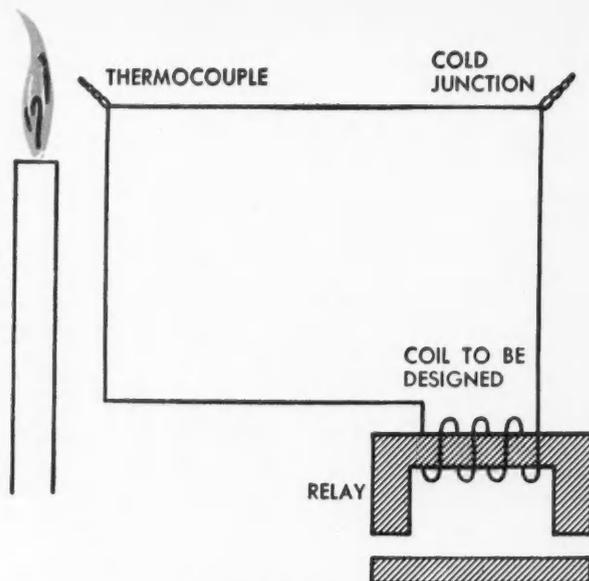
**PROBLEM: FLAME DETECTOR CIRCUIT**—Determine the number of turns the coil should have to hold the relay in a closed position.
