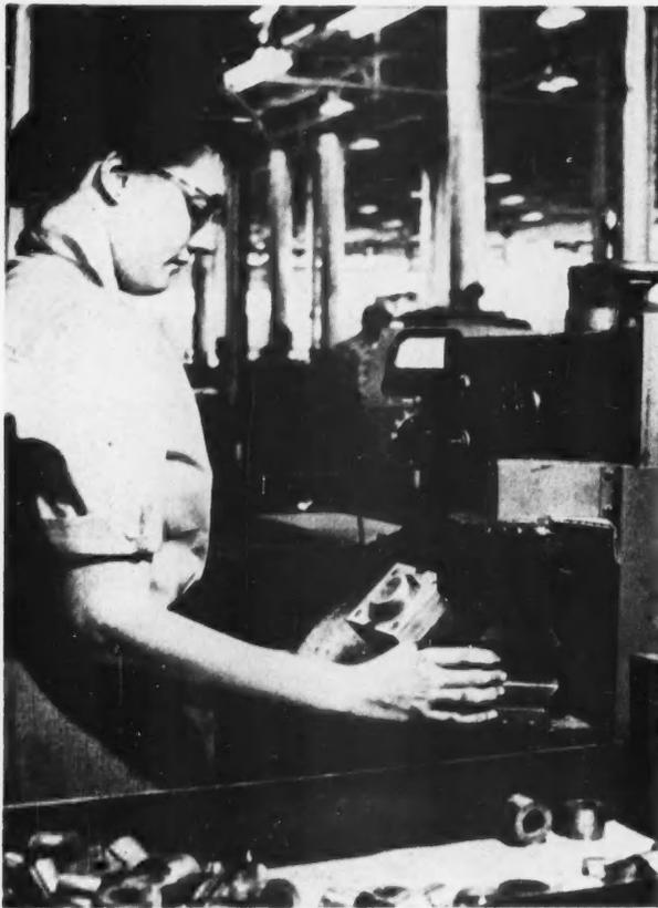
**13** . . . inspection and testing, such as for strength (*above*). Note tote box on conveyor, convenient to operator.
