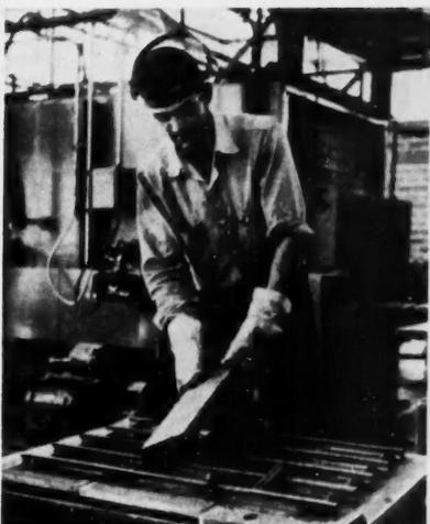
**9** After cooling, the magnets are dumped by the boatload, then conveyed to...
