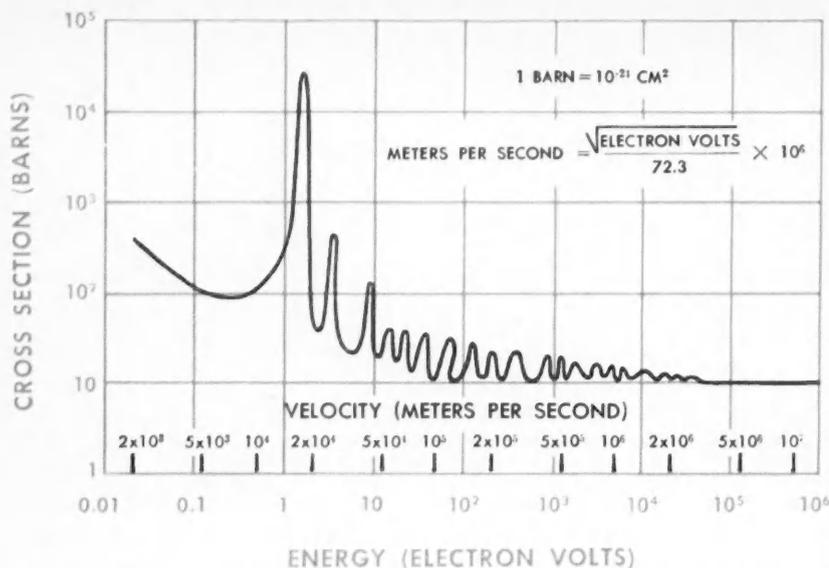
**FIG. 1. VELOCITY DEPENDENCE** of nuclear cross sections observed with velocity selector. Peaks are points of resonance where capture or scattering of neutrons is large.
