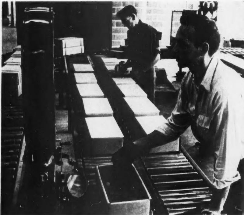
**15** . . . shipping area where magnets are counted and packed. The conveyor does triple duty: conveying, workbench, and weighing. The finished product may be used to . . .
