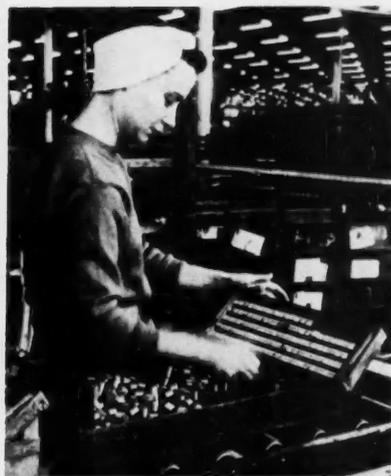
**7** After magnets are cleaned and rough ground, they are loaded into "boats"...
