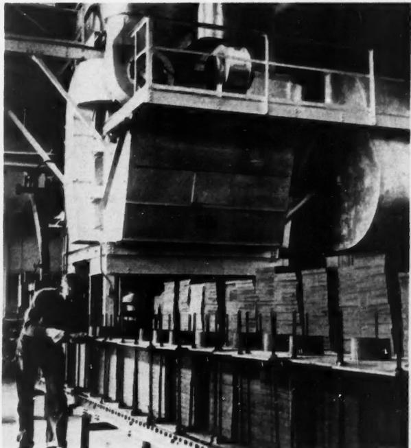
**3** . . . baked in electrically heated forced-air tower oven, then stacked 15 high on conveyors, ready for pouring.
