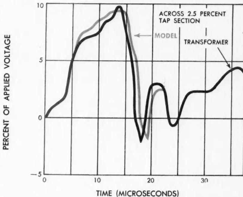
**COMPARISON** of impulse voltages in 30,000-kva transformer (138/39 kv) with those of its electromagnetic model. The model reproduces both magnitude and wave shape.
