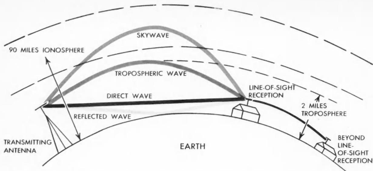
ELECTROMAGNETIC WAVES RADIATED FROM A TV TRANSMITTING ANTENNA MAY REACH THE RECEIVING ANTENNA BY SEVERAL PATHS.
