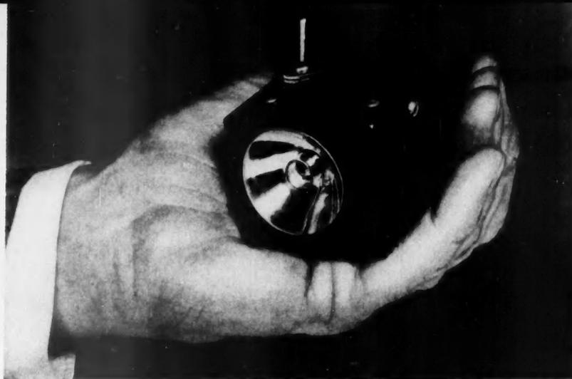
**HOME LIGHTING** can be controlled by photoconductive cell utilizing prevailing light levels at dusk and dawn. Current from highly sensitive cadmium-sulfide crystal needs no amplification.
