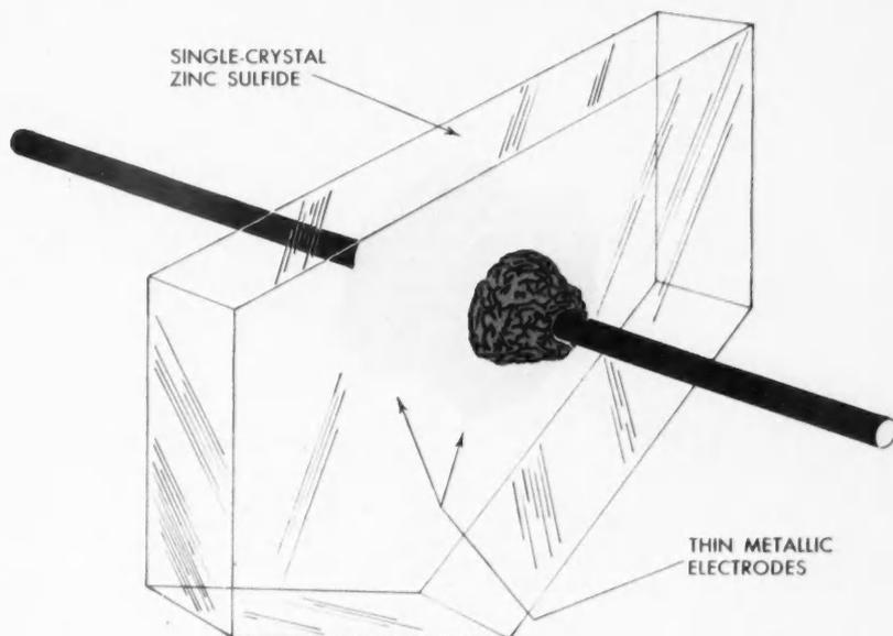
**CRYSTAL** of zinc sulfide electroluminescent cell may be grown in an evacuated quartz tube from the vapor phase at 1100 C. The thin films may be chemically deposited on glass surface.
