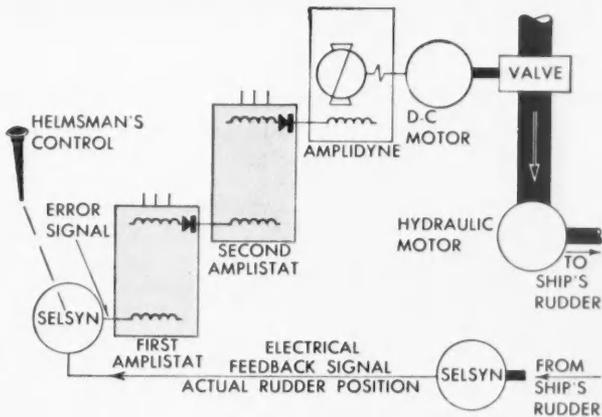
**STEERING ENGINE CONTROL** systems of destroyers like the USS *Anderson* utilize an amplistat in combination with an amplidyne. Two electrically connected selsyns compare the position of the helmsman's control lever with that of the rudder. When they
