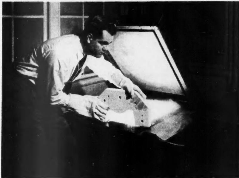
**LOW-TEMPERATURE TEST EQUIPMENT** enables the author to control the behavior of metals in such processes as sub-zero assembling, control of age-hardening, cooling during machining, and stabilization of precision parts. Mr. Gregg, Supervisor of the Metallurgical Unit, Construction Materials Laboratory, Bridgeport, joined General Electric in 1950.
