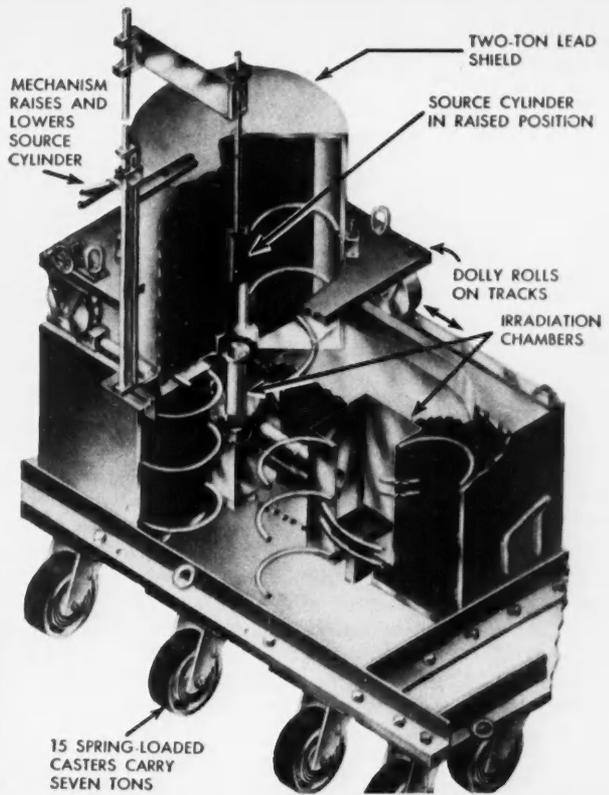
MOBILE 580-CURIE LEAD-SHIELDED COBALT GAMMA SOURCE PROVIDES ACCESS TO SAMPLE DURING IRRADIATION; AUTHOR (RIGHT).
