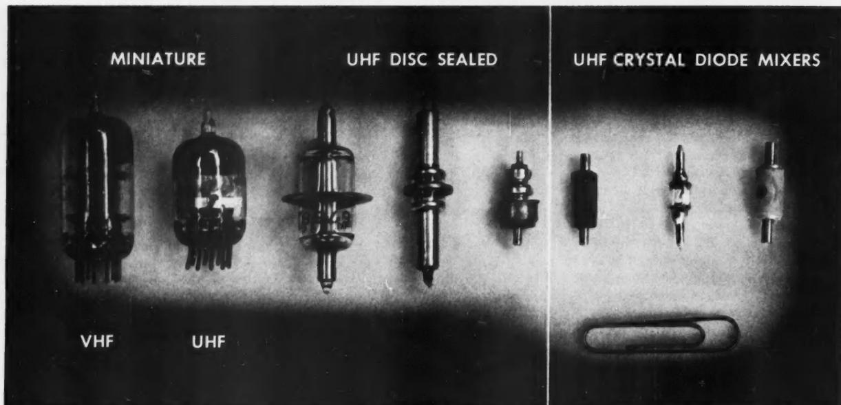
DISC-SEALED TRIODE IS MOST SUCCESSFUL TUBE THAT CAN BE USED IN UHF RECEIVER. CRYSTAL DIODE GIVES GOOD NOISE PERFORMANCE.
