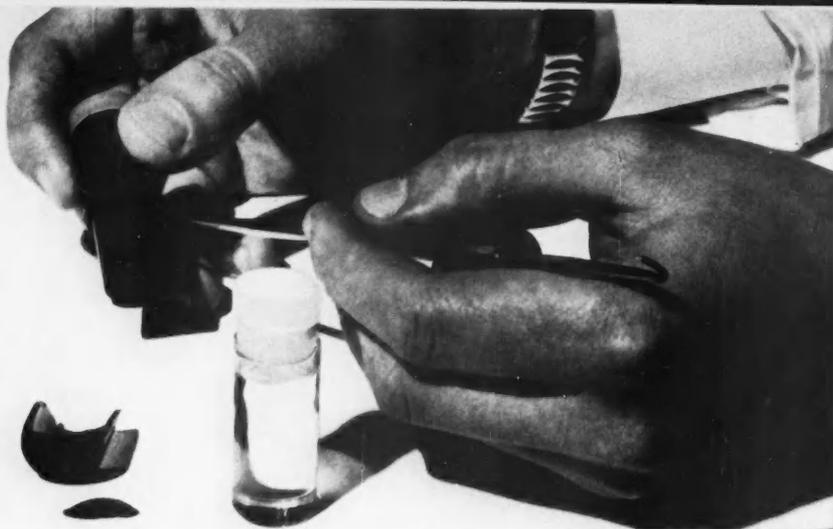
**IRRADIATION POLYMERIZATION**—A mixture of styrene and acrylonitrile in equal quantities produces a solid that often breaks its glass container.
