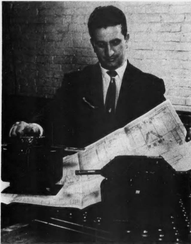
**5** Here's the completed 5000-volt instrument transformer alongside its conventionally insulated counterpart. In the former process, the unit was hand-wrapped with an asphalt-treated crepe paper—a laborious and costly process.
