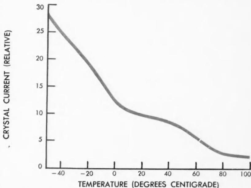
**PHOTOCURRENTS** in cadmium-selenide crystals are inversely related to the temperature. Scientists think this effect results from an increased electron mobility at lower temperatures.
