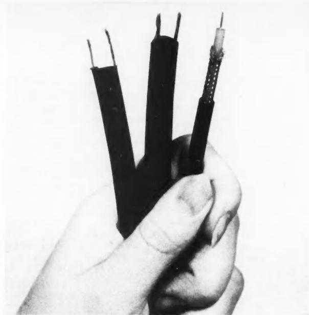
**ECONOMICAL TRANSMISSION LINE** is flat twin lead. Wet losses are less with tubular lead. Cost of shielded coaxial cable is high.
