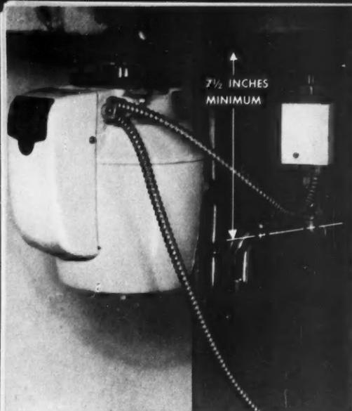
**VERY SHORT HOPPER** helps solve plumbing problems. White box is flow interlock.
