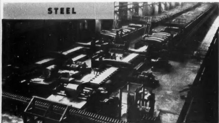
**PICKLING AND CLEANING** operation that removes scale from steel strip and prepares it for subsequent plating or galvanizing is speeded up through means of a magnetic loop control, employing an amplistat and amplidyne. The acid-resistant pick-up assures maximum
