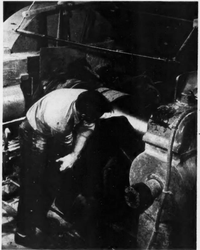
**6** Butyl rubber gum is compounded with other materials to give it desirable properties. Most of the synthetic rubbers originated in Germany, but butyl is strictly an American development.
