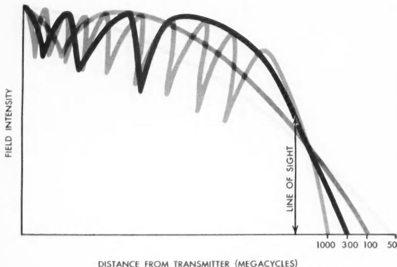
**DISTANCE** at which a signal can be received beyond the line of sight decreases with an increase in frequency. Also, field strength becomes a critical function of the distance.
