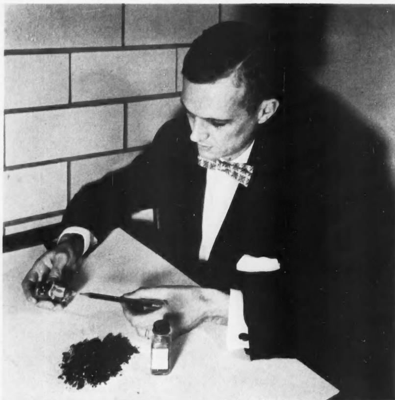
**PHOTOCONDUCTIVE CELL**, relay, and transistor make up the high-speed relaying system held by the author. In the foreground are photoconductive crystals of cadmium selenide.
