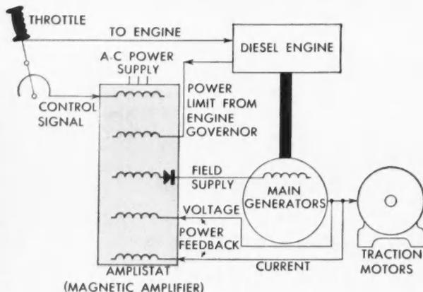
and acceleration of the traction motors in response to throttle position. The signal from the diesel engine's governor sets up a power limit and reduces wheel speed when more tractive effort is needed, thus preventing the engine from "lugging down."
