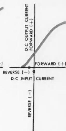
**MAGNETIC AMPLIFIER**, like the electronic amplifier but unlike the rotating amplifier, is nonreversing. A reversed input signal increases its output in the forward direction.
