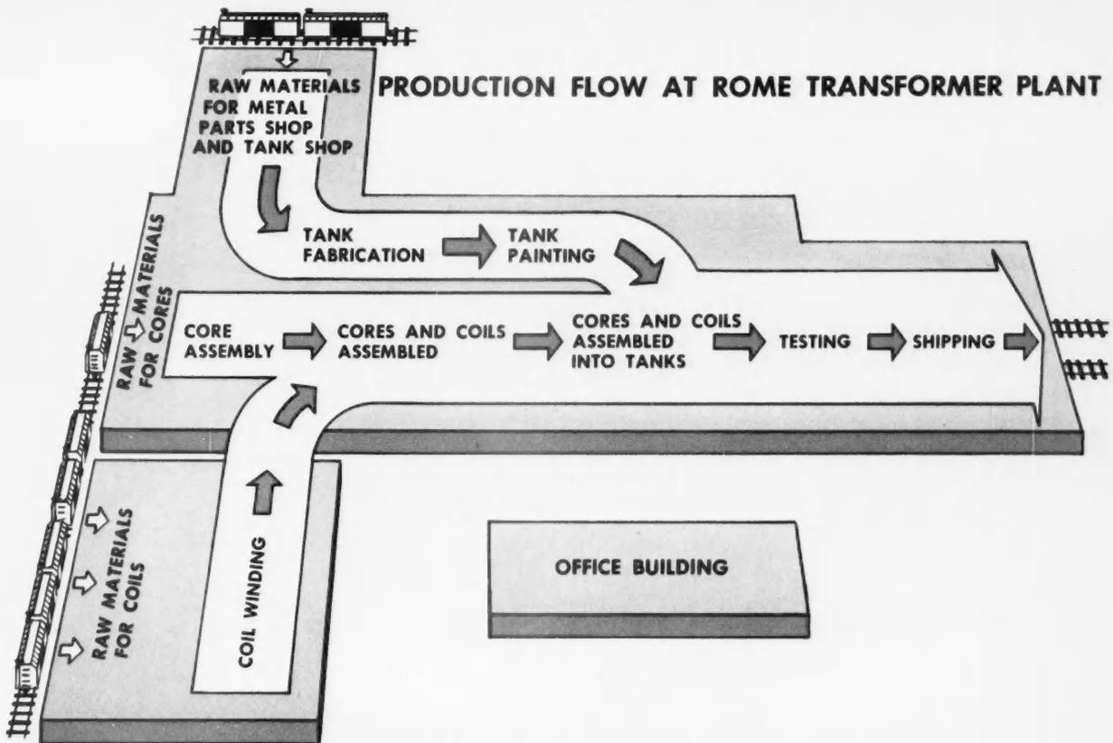
... RAW MATERIALS ARRIVE BY RAIL OR TRUCK AND ARE UNLOADED DIRECTLY AT POINT OF USE. STRAIGHT-LINE PRODUCTION SPEEDS OUTPUT.
