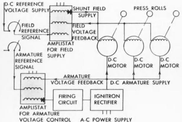
nishes the motors' shunt field supplies. This combination provides the 50 to 1 speed range needed for starting up and running modern printing presses. The amplistat-controlled ignitrons for this service are rated 150 to 300 kw.
