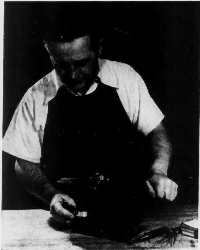
**4** Inspection of finished product follows a finishing operation and electrical testing. Butyl is the complete insulation—so elastic it won't crack under stresses caused by chemical or thermal shrinkage. (Photo sequence continued on next page.)
