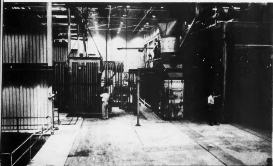
**FLOW-PAINTING** the tanks in special booths (*above*) is one of the last operations before cores and coils are installed. "Captive" cranes in paint booths make it possible to transfer the tanks to the baking oven (*left*). Tanks move through oven on conveyor.
