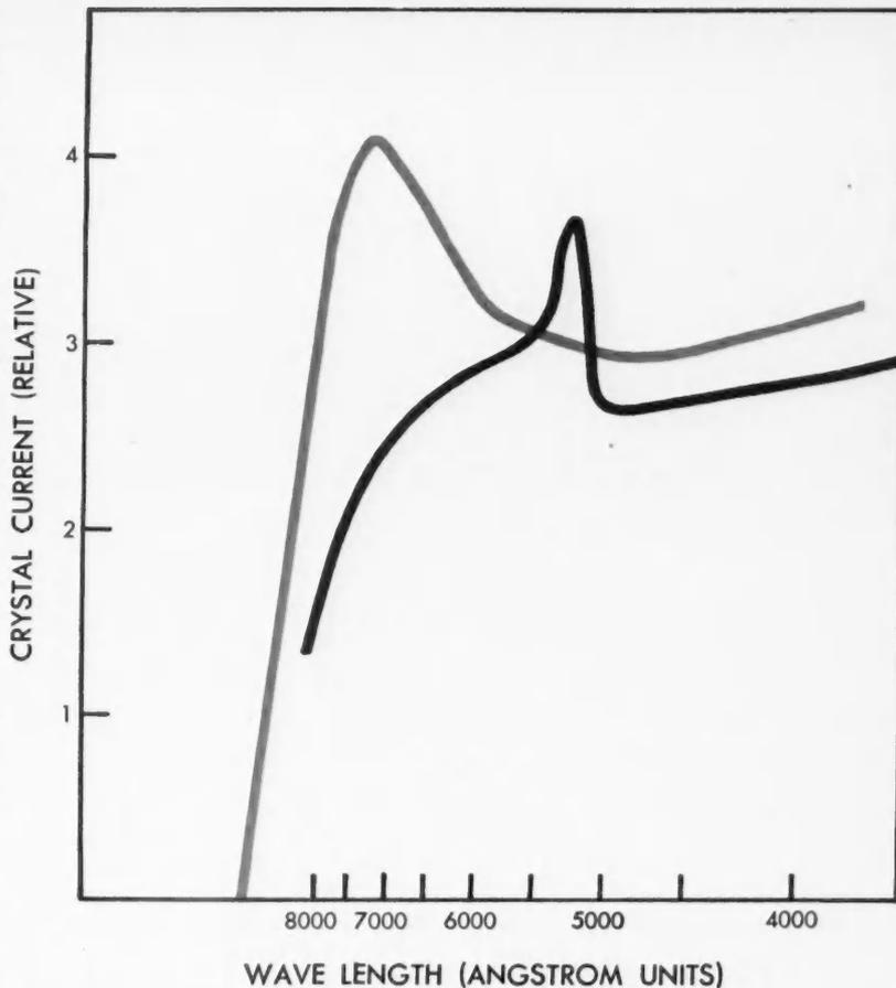
**SPECTRAL RESPONSE** of cadmium-sulfide crystals (black curve) and cadmium selenide crystals (gray curve) to visible portion of the spectrum runs from about 3800 to 7600 Å.
