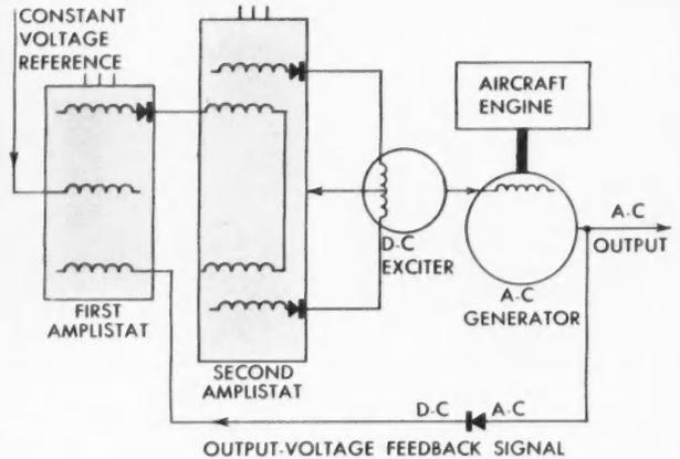
and a rectified portion of the a-c output. The amplified difference signal controls a second amplistat. And the latter, designed to supply reversing output, energizes the field of a d-c exciter that in turn excites the a-c generator.
