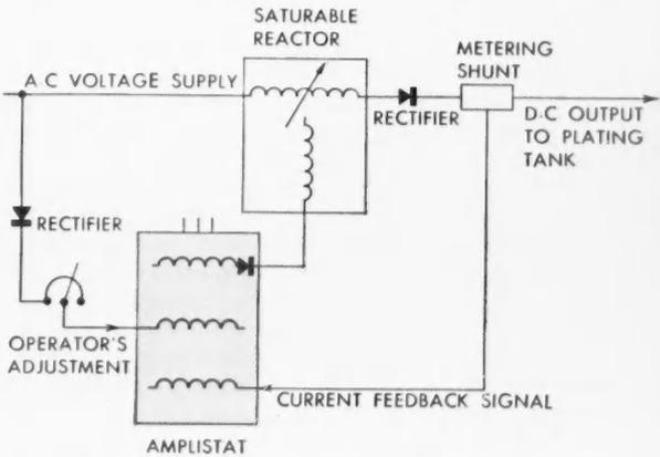
**LARGE CURRENTS** of an automatic electroplating process—in this instance the silverplating of aluminum conductors—are measured via a d-c metering shunt. The amplistat amplifies the feedback signal from the shunt (diagram), compares it with the current magnitude
