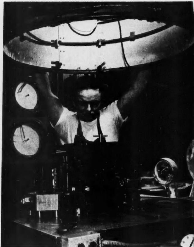
**2** Open die's mating-half is secured, a steel dome is lowered to form a high vacuum, and butyl rubber—an American-developed synthetic with superior electrical, chemical, and physical properties—is injected into the die under pressure.
