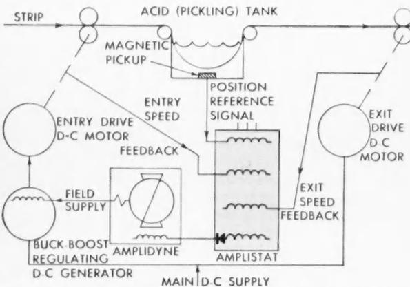
footage of steel strip in the pickling tank (diagram) without allowing the strip to drag. Output of the pickup, which depends on the proximity of the steel strip, is amplified by the amplistat and amplidyne to regulate entry speed relative to exit speed.
