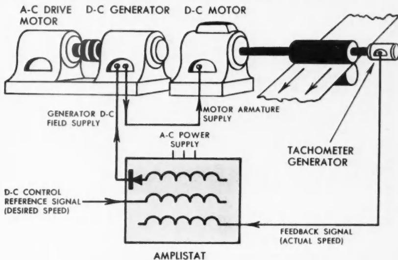
**THE MAGNETIC AMPLIFIER**, or amplistat, is an electromagnetic device. A d-c signal applied to one or more control windings varies the magnetic permeability—and thus the impedance to the flow of a-c through an output winding—to produce an amplifi-
