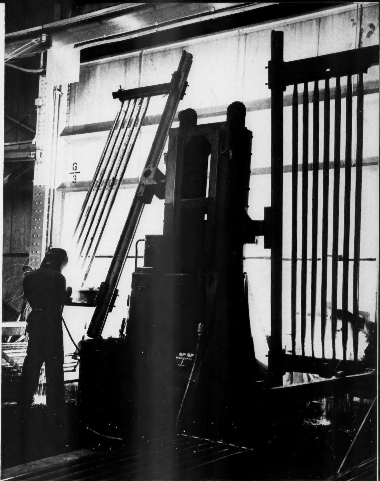
**WINDMILL** fixture holds tubes and headers in position, permits them to be turned end over end for "downhand" welding. Many such
