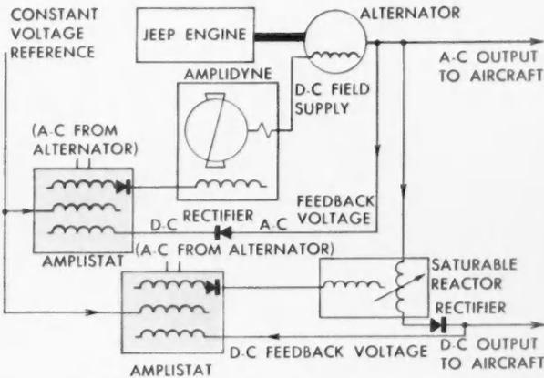
**MOBILE POWER SUPPLY** for jet aircraft—such as the Navy's McDonnell *Banshee*—employs an amplidyne-amplistat system of regulating voltage. The jeep's engine drives an alternator (diagram) that furnishes the aircraft with d-c power by means of a rectifier.
