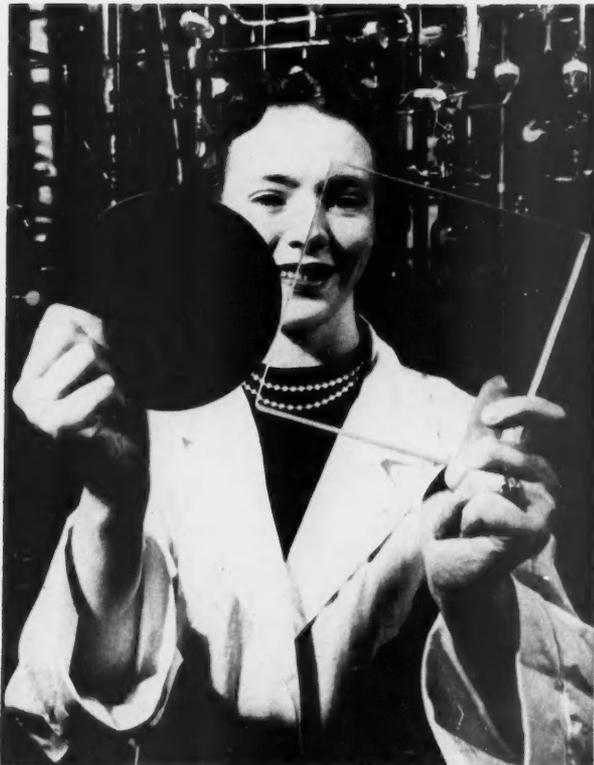
**GLASS** Most ordinary types of glasses are quite easily discolored by exposure to gamma radiation. The piece of clear glass has been stabilized against this effect.
