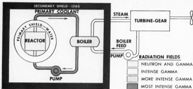
REACTOR'S PRIMARY SHIELD STOPS NEUTRONS; SECONDARY STOPS GAMMA RADIATION.
