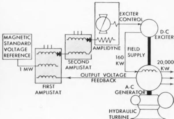
amplidyne. The deviations of output voltage from a magnetic standard reference (diagram) are detected and amplified by two stages of amplistats, an amplidyne, and a conventional d-c exciter. Note that only 1 mw controls an output of 20,000 kw.
