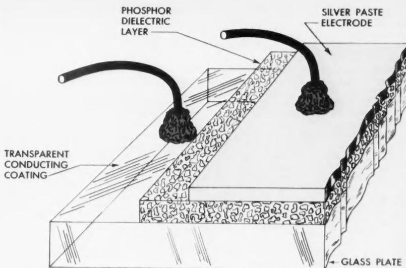
**POWDERED ZINC** sulfoselenide electroluminescent cell makes possible broad-area panels that would give a combination of high-level illumination and low surface brightness.
