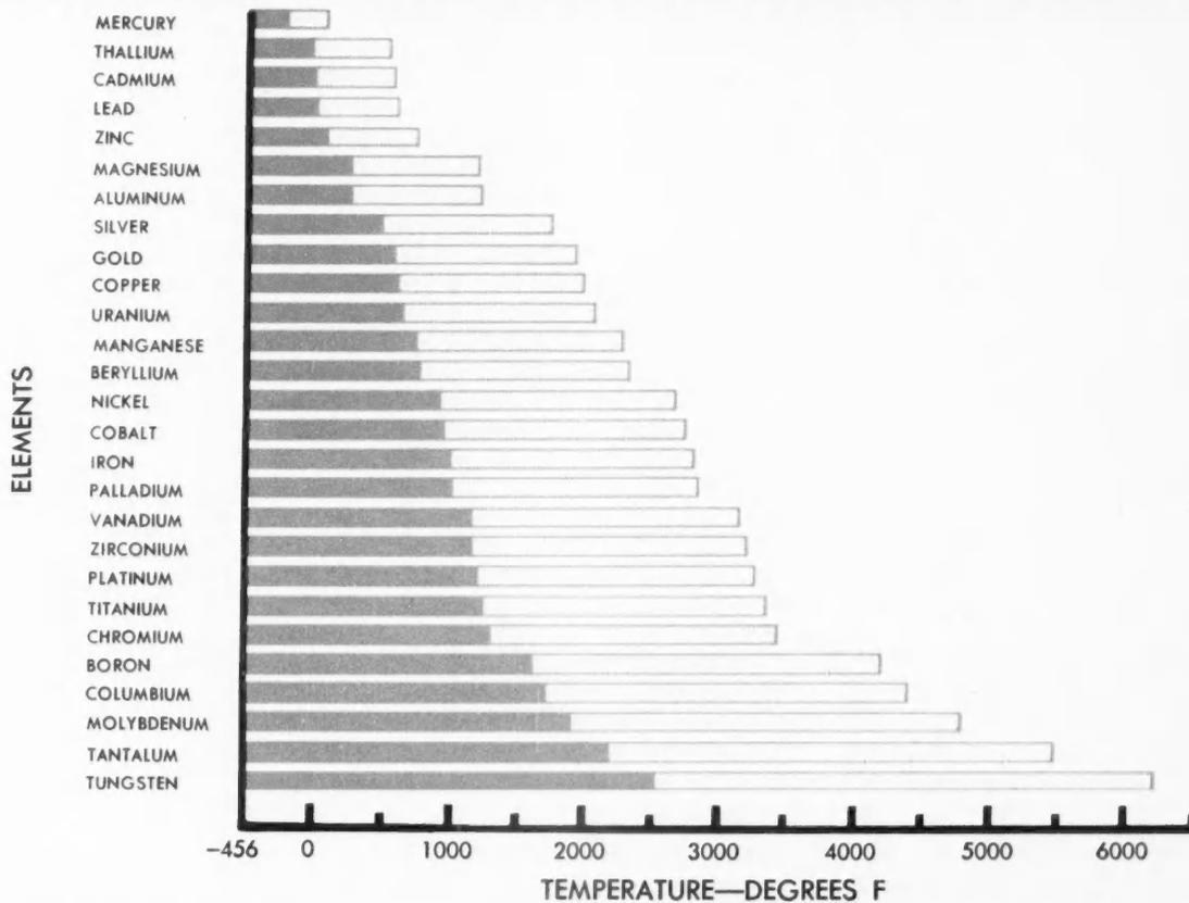
DEMARICATION LINE BETWEEN HIGH AND LOW TEMPERATURE BEHAVIOR IS ABOUT HALF THE MELTING TEMPERATURE OF A METAL.
