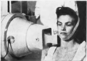
**CARBOLoy HEVIMET** is 50% heavier than lead, 40% more effective in stopping gamma rays. In this cancer therapy unit, Hevimet controls radioactive Cobalt. Other uses include weights and balances.
