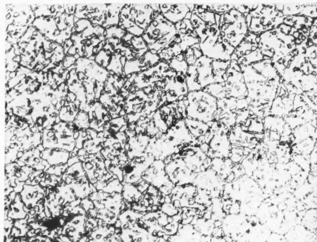
smaller. The super-alloy crystal (*above*) containing growth-preventing and strengthening particles is magnified more than 500 times.
