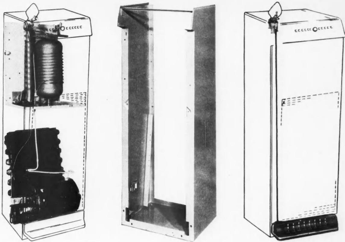
**CASE CONSTRUCTION**—One-piece side-bottom-side (center)—provides a simple chassis for mounting the removable refrigeration assembly (left). Connecting the foot pedal with the water valve are a relief spring and an operating rod.
