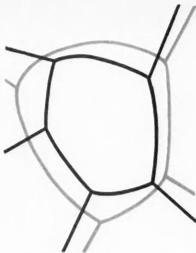
**HIGH TEMPERATURES** can weaken crystals by causing boundaries to grow (*blue lines*).
