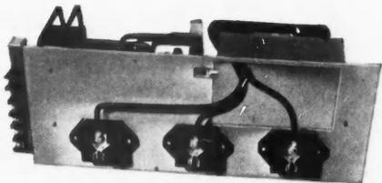
Rear view of Control unit showing three individual bus stabs of silver-plated pure copper. Re-inforced with heat-treated spring steel, they assure positive contact with vertical bus.
