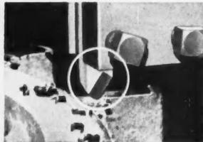
**CARBOLoy CEMENTED CARBIDES** wearproof vital parts; make tougher, longer lasting tools and dies. New heavy-duty carbide, above, increased production 30%, maintained cutting edge at red heat.
