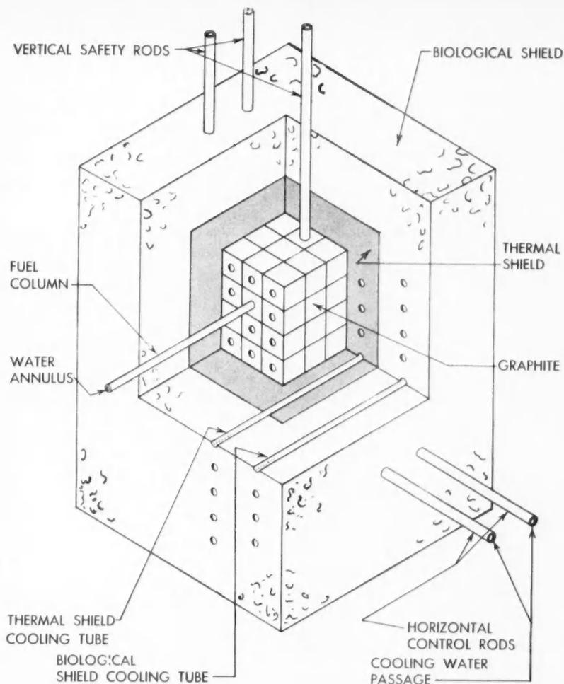
**GRAPHITE-MODERATED REACTORS** similar to this will produce commercial power in 5 to 10 years. Still a major concern of the reactor engineer is the design of facilities for . . .
