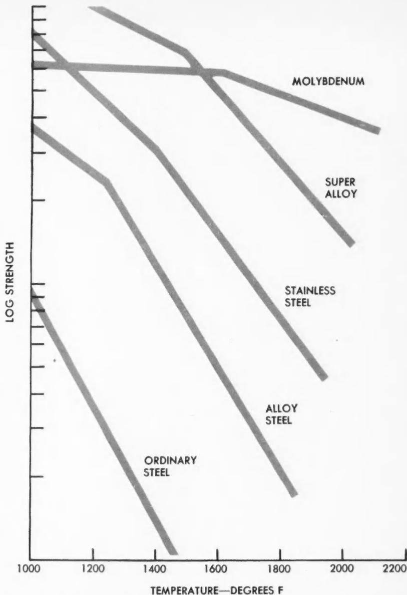
**PRIMARILY LOW-TEMPERATURE** behavior changes to primarily high-temperature behavior at the knee of the typical strength-temperature curves for various metals and alloys.
