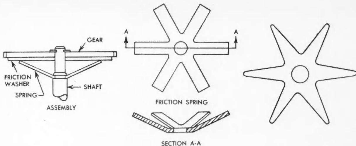
**PROBLEM:** For the time-switch clutch assembly (left), design the spring (center) so that torque variations caused by manufacturing tolerances will be minimized. Compare design with spring having tapering fingers (right), justifying conclusions by physical reasoning.
