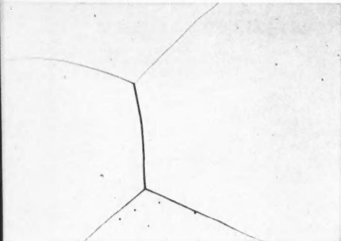
**TYPICAL METAL-CRYSTAL** structure—at about 100 magnification—appears similar in principle to table-salt crystal but is much
