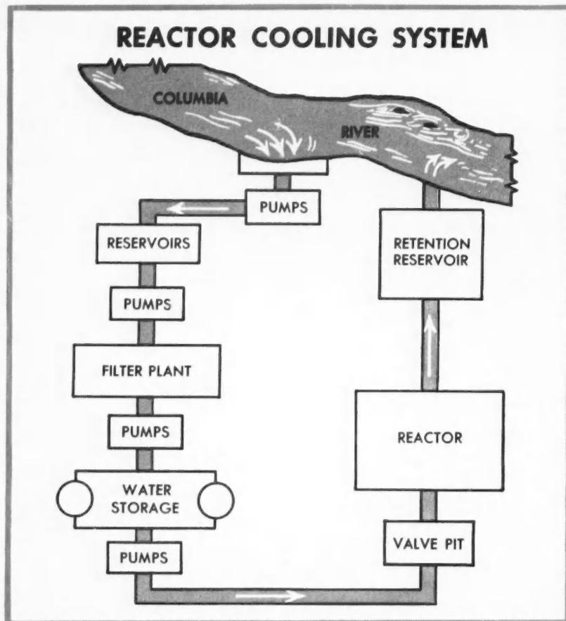
**UNIQUE PROBLEMS** involved in cooling a reactor include loss of coolant, coolant stoppage, and neutron absorption. The first two make reliability of the system extremely important.
