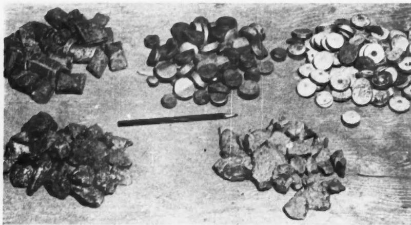
**HEAVY AGGREGATES**—steel punching and sheared bars (top) and natural aggregates of magnetite and limonite—are used in preparing high-density concrete by the prepack method.
