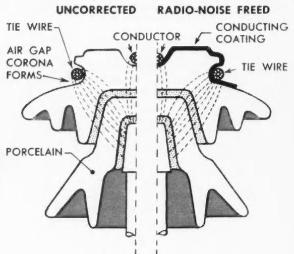
**CORONA FORMATION**, with resulting radio interference, is eliminated by applying special conducting glazes (right) to porcelain.
