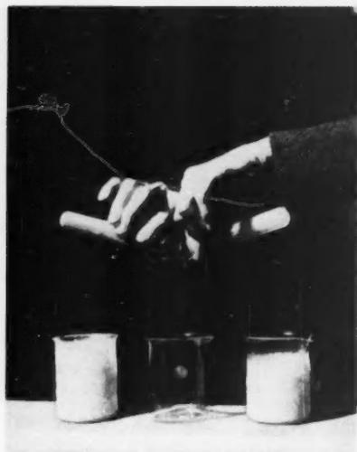
**SILICONE FLUID** pours at  $-100^{\circ}\text{F}$  (right) while standard petroleum fluid freezes over.
