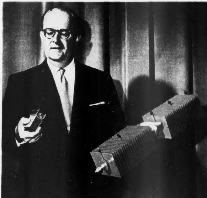
**GERMANIUM RECTIFIER CELL** rated 2000 watts (*left*) has the same capacity but is only one-fortieth the size of the selenium cell. Author McIntyre—application engineer—joined the Company's Lighting and Rectifier Department in 1947. He is now with the Illuminating Engineering Laboratory, River Works, West Lynn, Mass.
