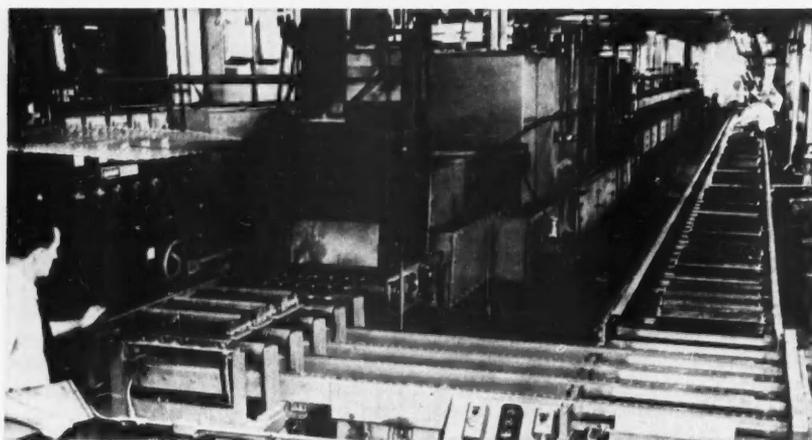
**ROLLER-HEARTH CONVEYOR FURNACE** for high-scale production, such as annealing steel cartridge cases, is equipped with return conveyor and transfer tables for automatic handling.
