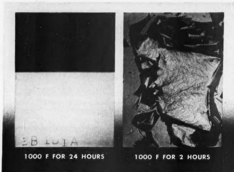
**PROTECTIVE COATING** formulated with silicone resin and applied to a steel panel (*left*) is unaffected by exposure to high temperature, while conventional coating cracks and peels.
