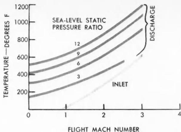
**TEMPERATURE LEVEL** throughout the compressor is increased by energy put into inlet air as flight speed increases.
