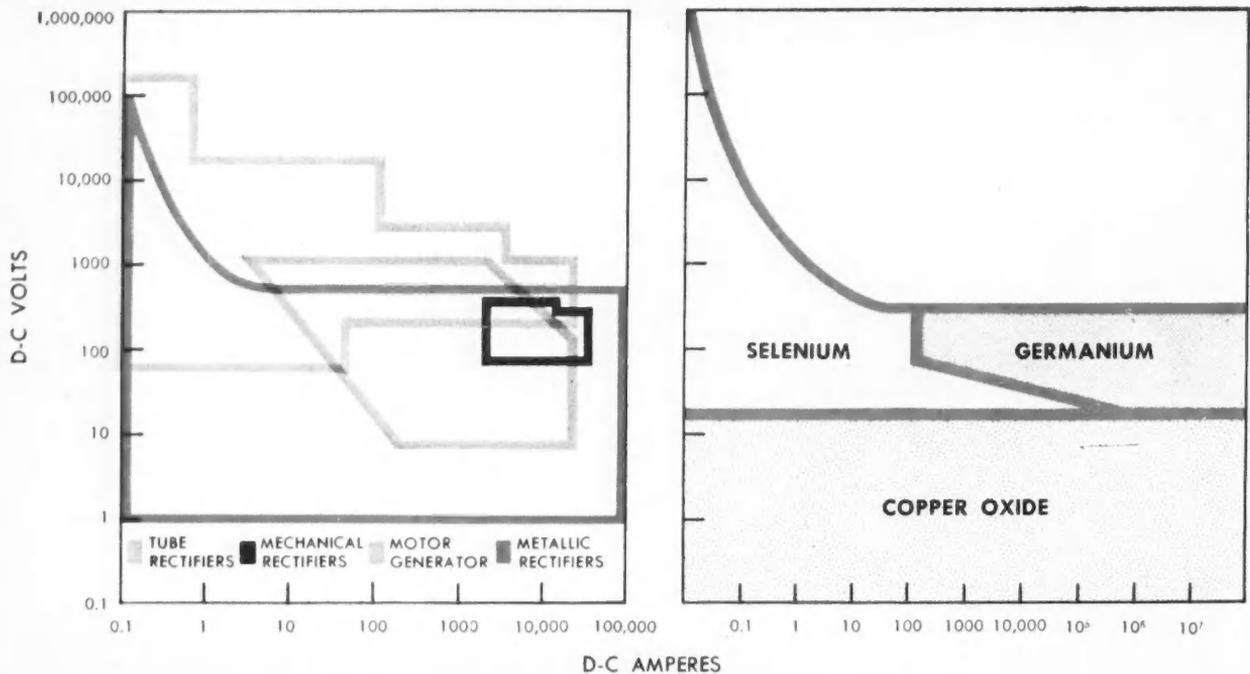
**GERMANIUM RECTIFIERS** can replace most present types of converters over a wide range of applications (above). The chart (right)
