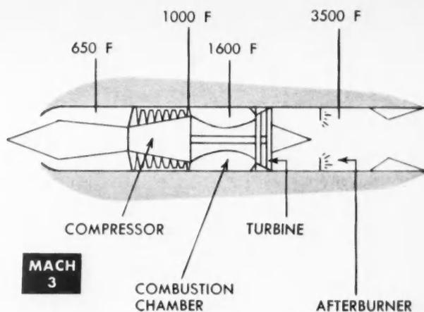
**HIGH INTERNAL JET TEMPERATURES** are almost as troublesome as high surface temperatures when aircraft travel at supersonic speeds.
