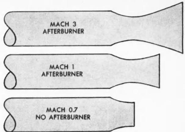
**EXHAUST NOZZLES** must be made convergent-divergent to allow for the high expansion pressure ratio attained at high flight speed.
