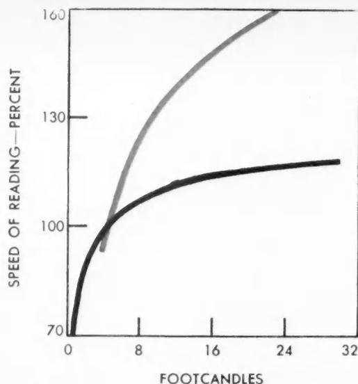
**ILLUMINATION** increases reading speed of low- (brown curve) compared with high-contrast print (black curve).
