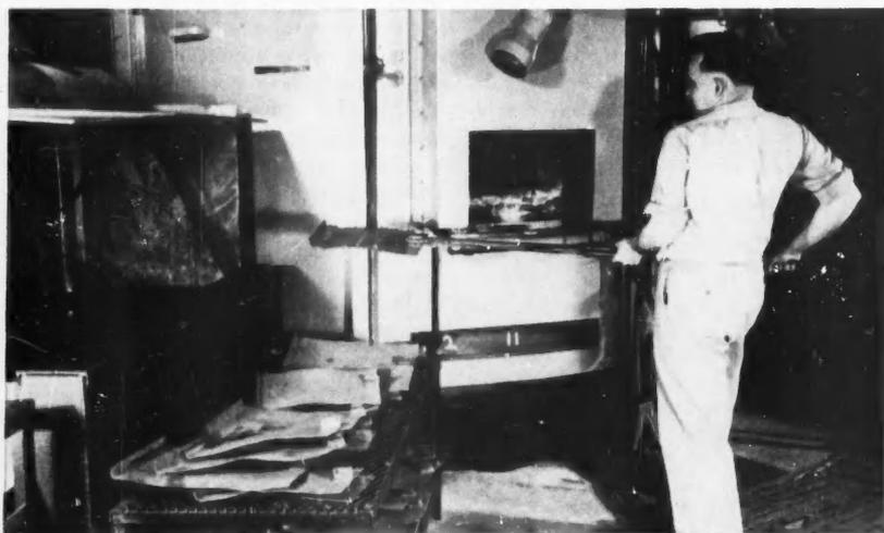
**ROTARY-HEARTH FURNACE** gives continuous heating of parts and offers such advantages as uniform hardness, freedom from scaling and decarburization, minimum labor, and low cost.
