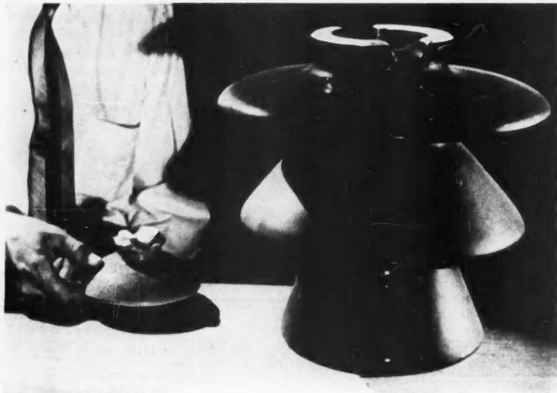
**OLD AND NEW:** Modern radio-noise-free pin-type insulator of porcelain for high-voltage transmission lines over-shadows 1906 design—still usable after 17 years of service.
