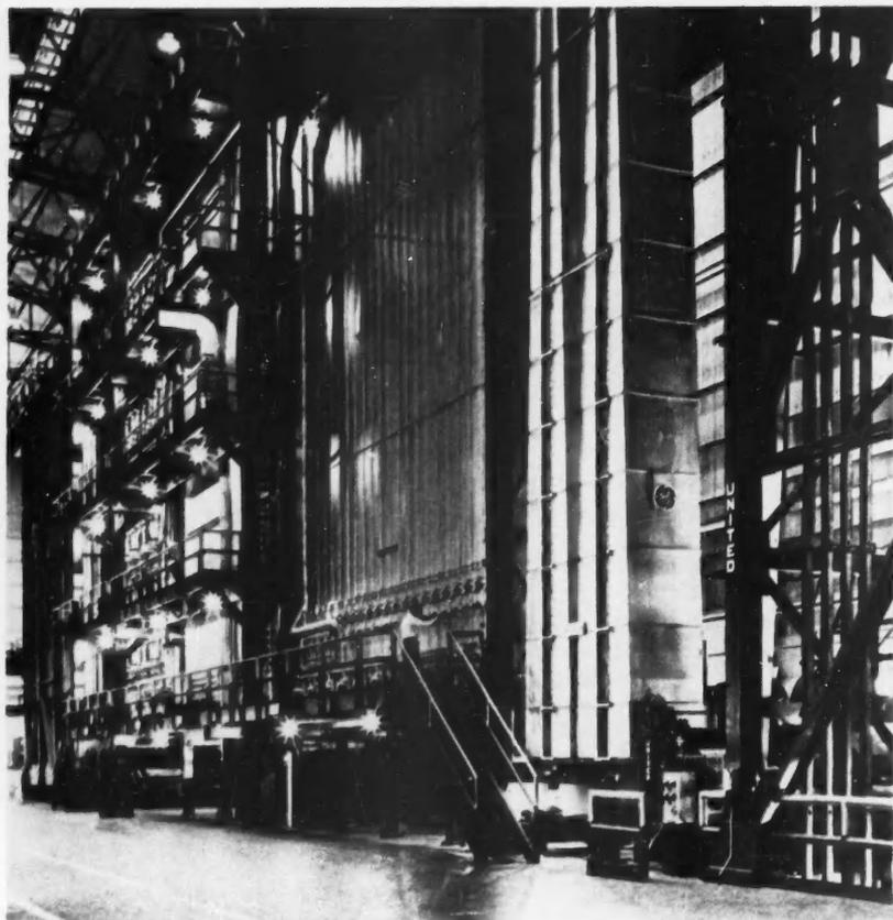
**SIZE** of protective-atmosphere furnaces seems to be unlimited, as indicated by this tower-type furnace that can bright-anneal steel tin-plate strip at the rate of 30 tons per hour.
