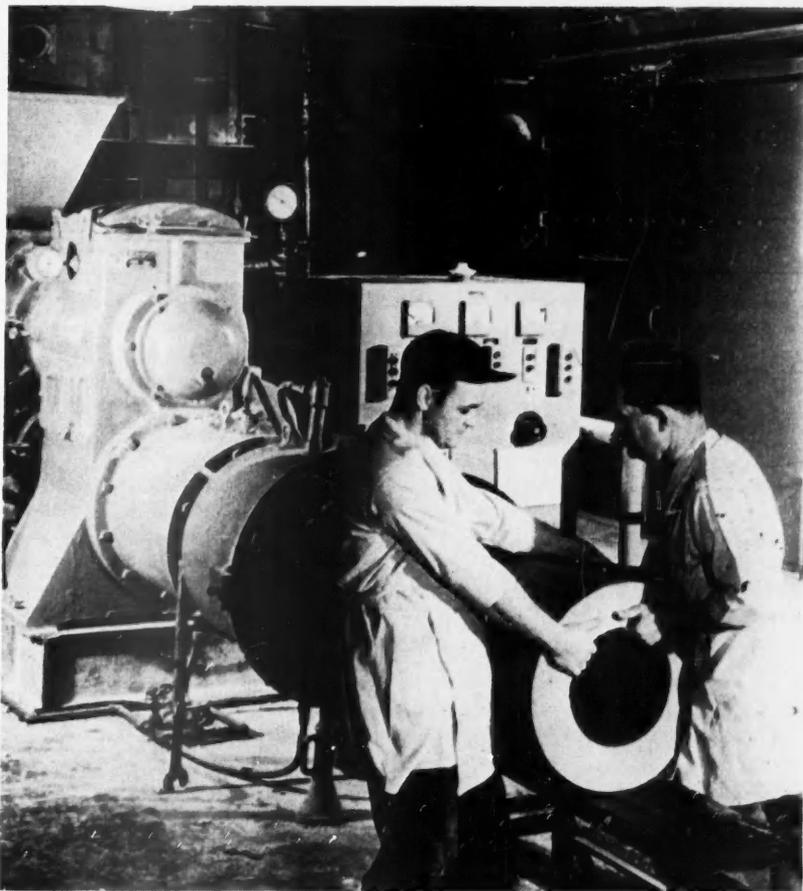
**PUG MILL** shreds clay, removes metallic contamination and air, then extrudes clay. Weighing up to 600 pounds, the pugs are later shaped into parts of apparatus bushings.
