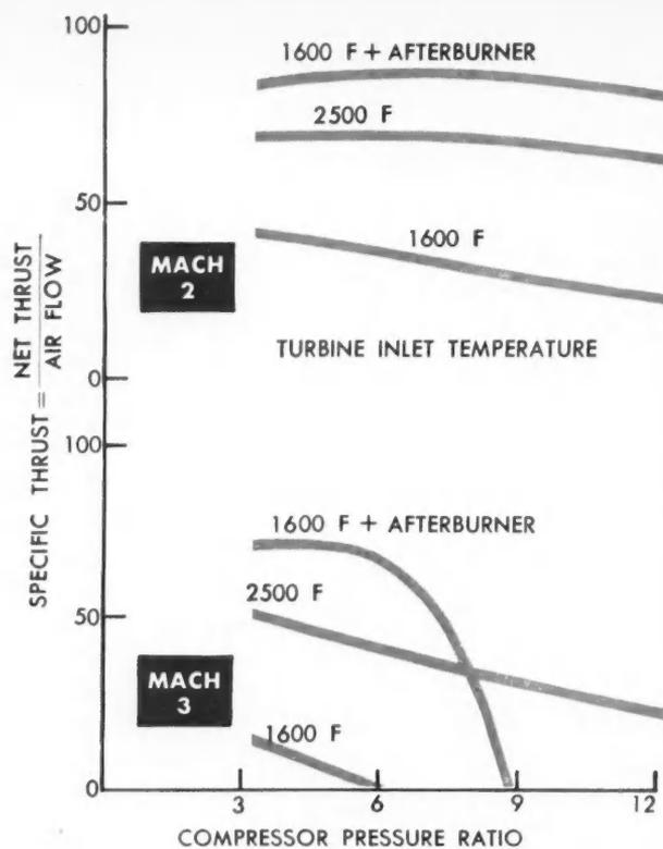
**THERMAL EFFICIENCY VS COMPRESSOR PRESSURE RATIO — SPECIFIC THRUST VS COMPRESSOR PRESSURE RATIO**—At Mach 2, Mach 2 curves undergo drastic changes when speeds reach Mach 3. At Mach 3, engines need low pressure ratio, high combustion temperatures.
