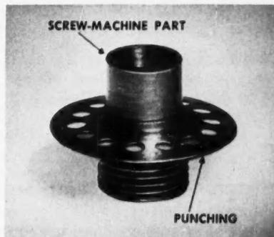
**CONTROLLED ATMOSPHERE** allows use of cheaper material in breather assembly.
