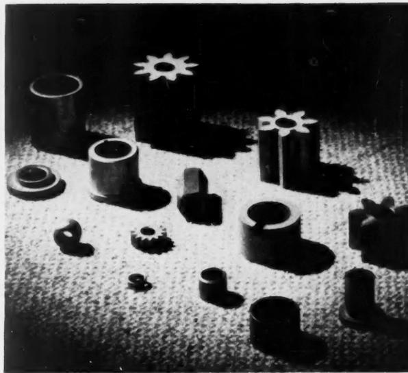
**SINTERED POWDER-METAL PARTS** usually show cost savings of 50 or 60 percent over gears cut from castings or bar stock.
