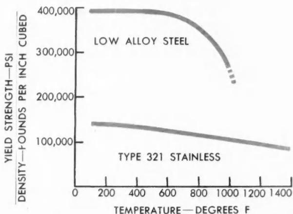
**ALL-STEEL CONSTRUCTION** either of low-alloy or stainless steel is required for high compressor discharge temperature.
