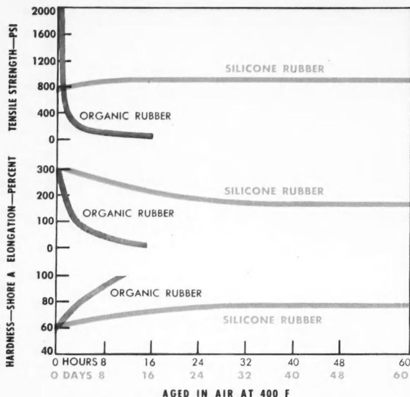
**PHYSICAL PROPERTIES** of silicone rubber remain stable at elevated temperatures. Note that the abscissa for organic rubber is in hours, silicone rubber in days.
