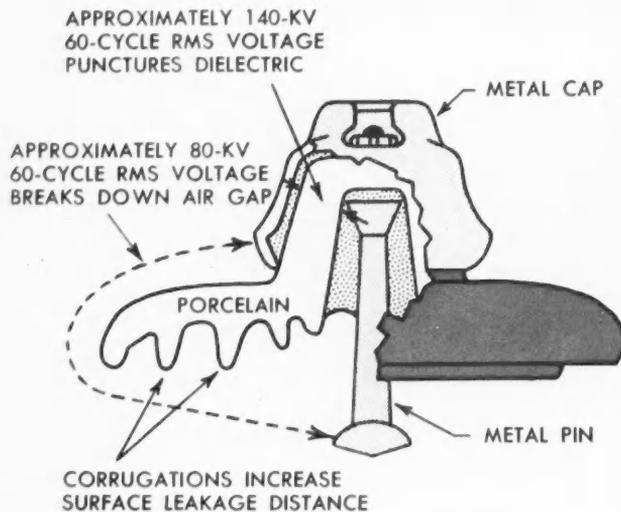
**ELECTRICAL BALANCE** between differing dielectric strengths of porcelain and air is achieved through physical design.
