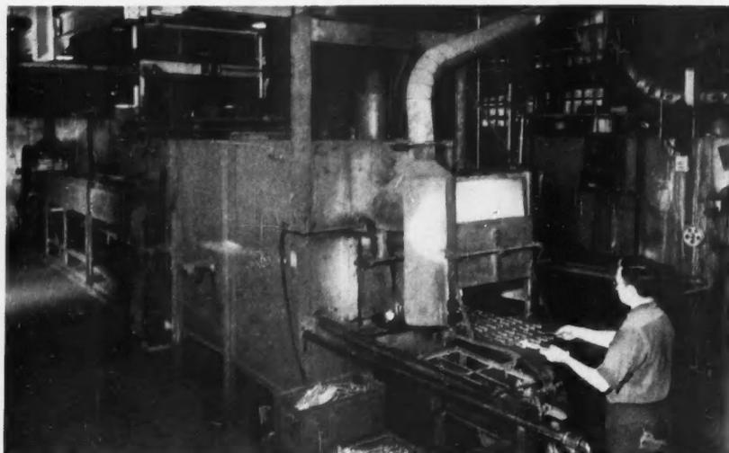
**MESH-BELT CONVEYOR FURNACE**, with heating and cooling chambers attached and protective atmosphere maintained throughout, treats bright stamped parts such as nameplates.
