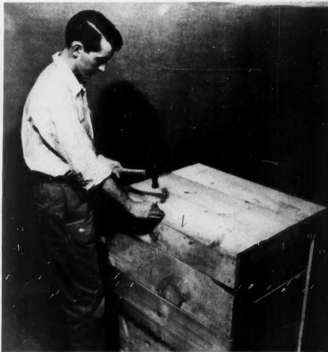
IN ANOTHER COAT OF WATERPROOF PAPER, CARTON IS FLOATED IN EXCELSIOR, AND ASSEMBLED BOX IS SECURELY NAILED FOR SHIPMENT.
