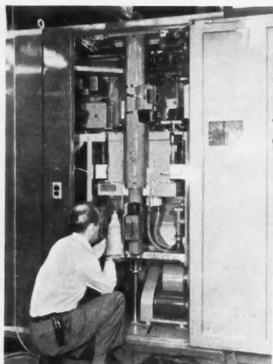
**CERAMIC-COATED TETRODE** is used with a 50-kw amplifier for high-channel VHF.
