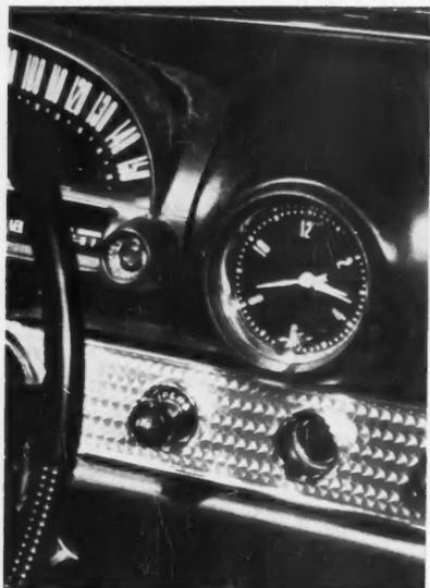
**ELECTRIC AUTOMOBILE CLOCK** has a sweep-second hand for the first time.
