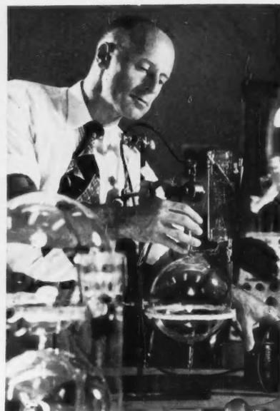
**IONIC PUMP** achieves vacuums equivalent to one billionth of normal atmospheric pressure.
