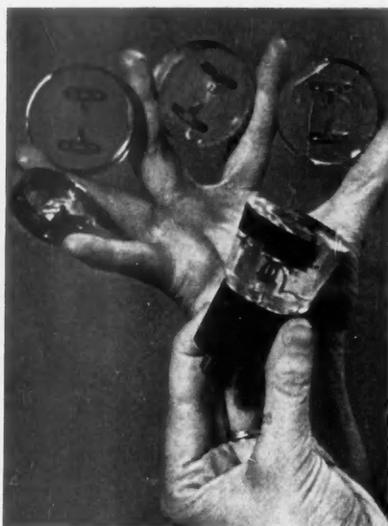
**RECEIVING TUBES** filled with clear plastics are sliced for microscopic examination.
