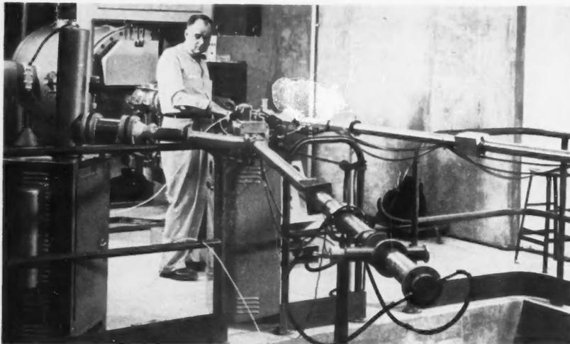
**POSITIVE-ION 2-MILLION-VOLT ACCELERATOR MAKES NEUTRONS FOR CELL-DAMAGE STUDY.**
