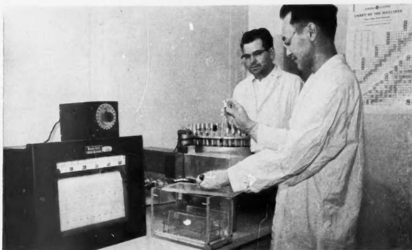
AUTOTURBIDIMETER COMPARES BIOLOGICAL DAMAGE CAUSED BY RADIOACTIVE ELEMENTS.
