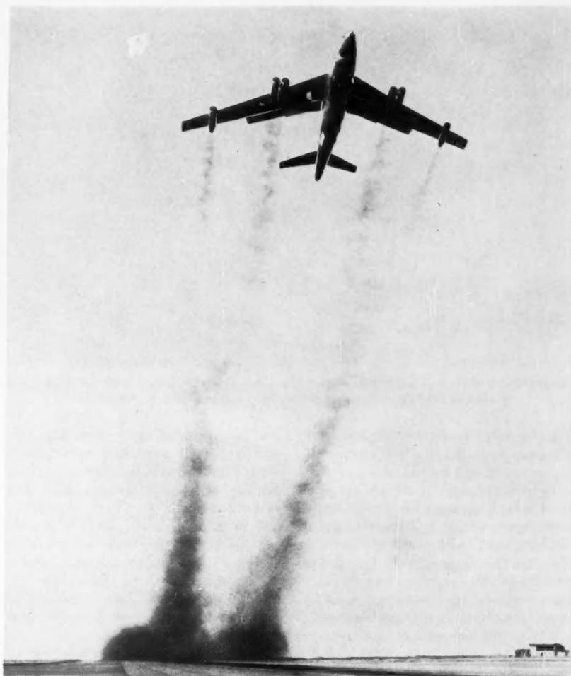
**WATER-INJECTION SYSTEMS** in the J47 jet engines of this Boeing B47 *Stratojet* provide bomber with added boost at take-off from a short runway or under a maximum load.
