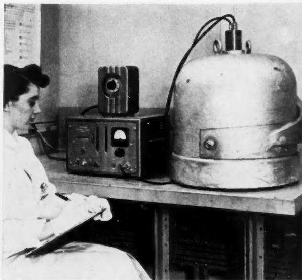
**GAMMA RADIATION** checked with scintillation counter indicates the abrasiveness of a plastics molding compound on metal-mold parts.
