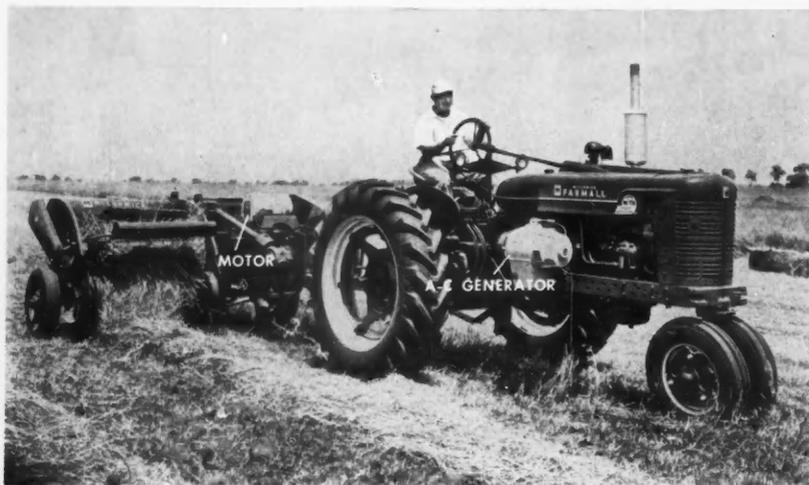
COMPACT A-C GENERATOR ADDS A SIZEABLE SOURCE OF POWER TO VERSATILE TRACTOR.
