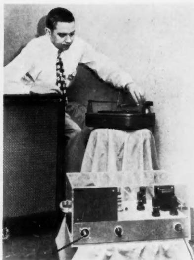
**HIGH-POWER** transistor amplifier sends 20 watts into speaker with negligible distortion.
