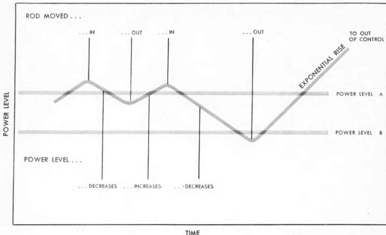
**NUCLEAR REACTORS** can be controlled by inserting rod-like neutron-absorbing materials. In this method, removal of the rod results in more neutrons and increased reactor power; insertion of the rod causes fewer neutrons and, consequently, decreased power.
