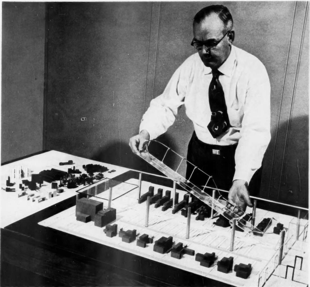
AUTHOR CARTER ATTACHES OVERHEAD PLASTIC CONVEYOR ASSEMBLY TO BUILDING STRUCTURE OF A THREE-DIMENSIONAL MODEL LAYOUT.
