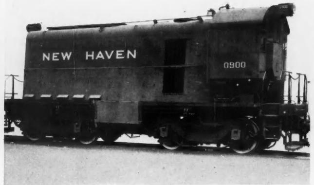
**EXTENSIVE DIESELIZATION** began in 1931 with the installation of a 600-hp switcher fitted with G-E electric equipment.
