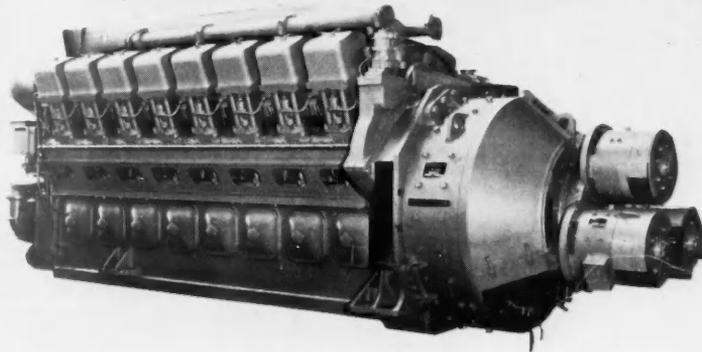
**ENGINE AND GENERATOR DESIGN** of today's 16-cylinder V-type 2250-hp diesel engine (lower) contrasts sharply with early 6-cylinder 300-hp engine, showing 30 years of progress.
