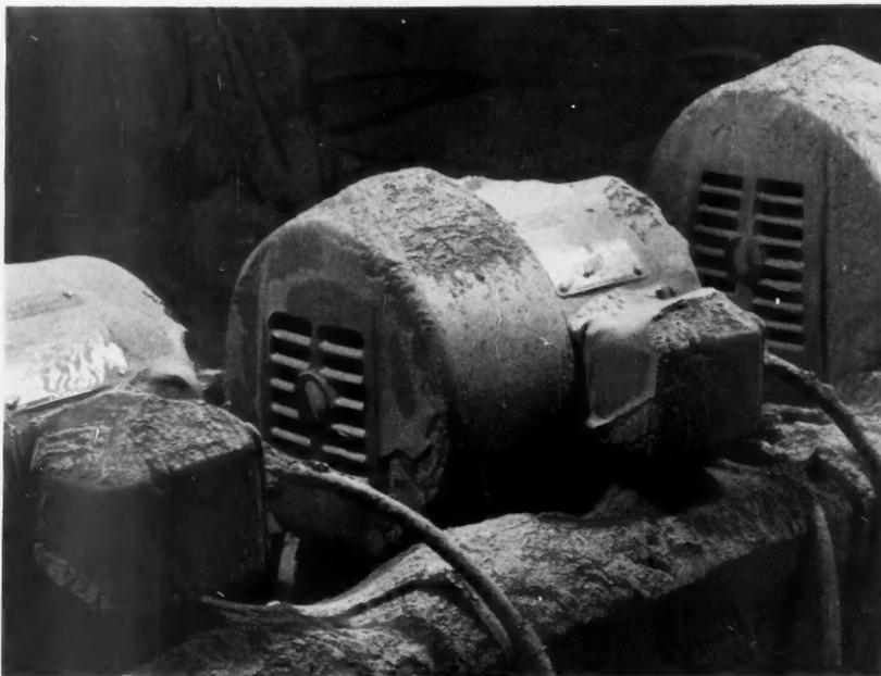
**FINE METALLIC** dust particles envelop new totally enclosed motors that are undergoing severe operating tests. Both motor frames and endshields are made of cast iron.
