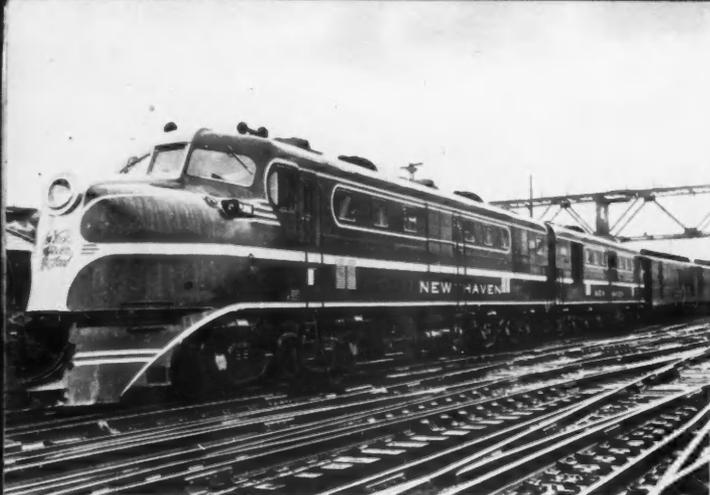
**EACH CAB** of New Haven Railroad's fleet of 4000-hp passenger diesel-electrics of the early 40's carried two 1000-hp engines.
