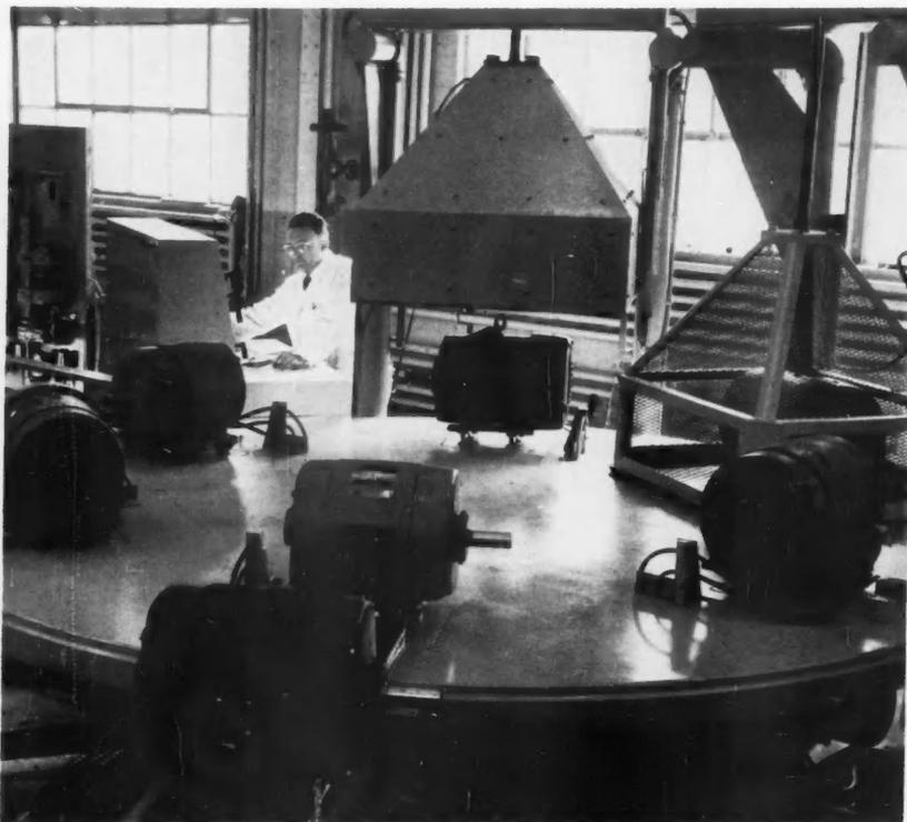
**INDUCTION MOTORS** in last phase of production receive acoustical tests for noise, mechanical tests for dynamic balance, or vibration, and several electrical tests.
