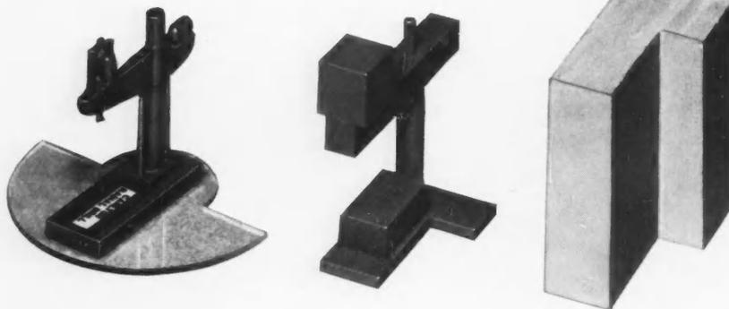
**VARYING DEGREES OF DETAIL** of a radial drill model show that a good three-dimensional model (*center*) must be recognizable yet easily fabricated and simply detailed.
