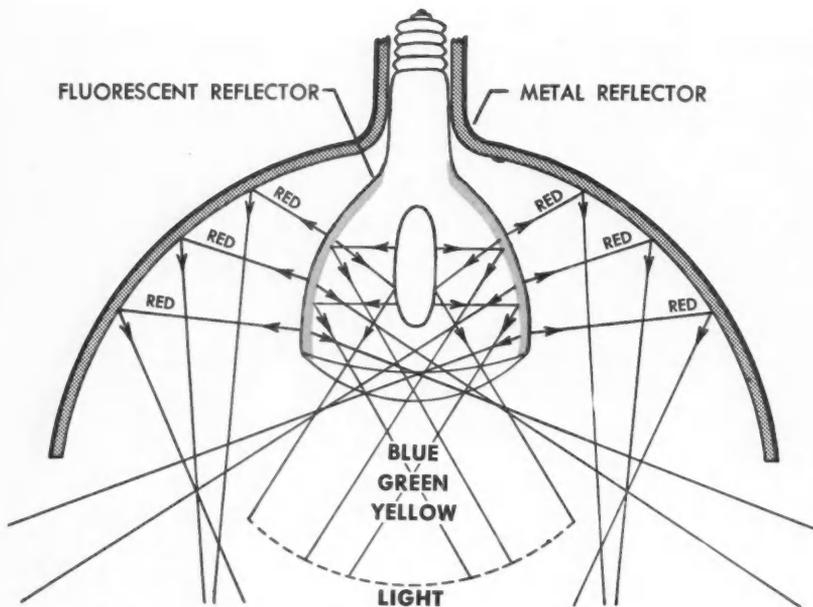
**FLUORESCENT REFLECTOR** utilizes light from both sides of phosphor coating that also reflects light from the arc, and it provides five percent more output than nonreflector lamps.
