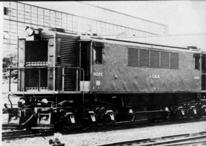
**FORERUNNER OF THE TRANSFER**, GE's 170-ton diesel-electric switcher with a 2000-hp engine was built in 1936 for Illinois Central.
