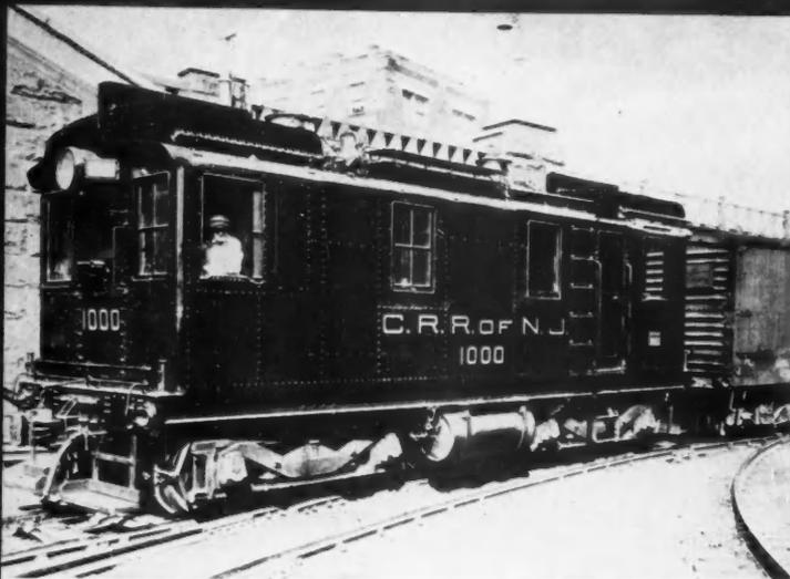
**FIRST DIESEL-ELECTRIC** to operate in the U.S.—Jersey Central's 60-ton 300-hp No. 1000—is still in service after 29 years.
