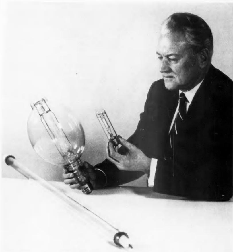
**SPHERICAL MERCURY LAMP** displayed by Dr. Buttolph finds industrial application in the 100- to 1000-watt range; tubular lamps for photochemical use range from 1000 to 5000 watts.
