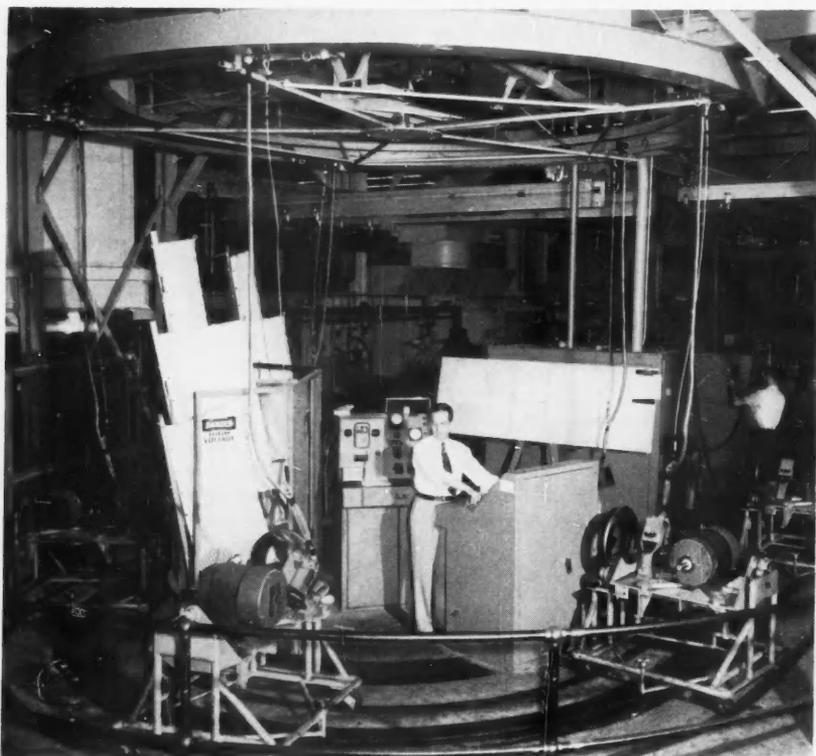
**MERRY-GO-ROUND** testing apparatus gives motors a final and different operational check at each station. The operator initiates tests from control consoles at center.
