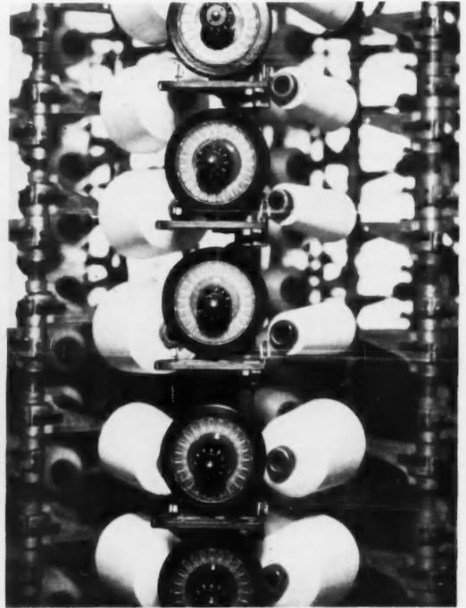
YARN-TENSION BRAKE USED ON WARPING CREELS IN TEXTILE INDUSTRY IS BUT ONE OF MANY APPLICATIONS FOR HYSTERESIS DEVICES.
