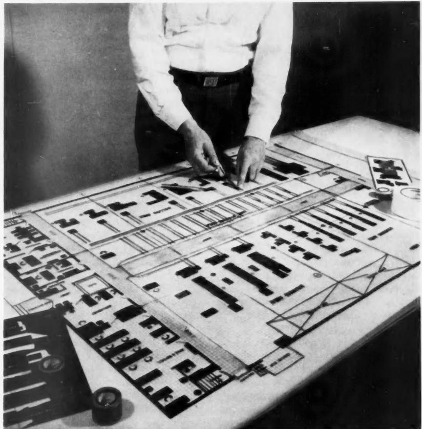
**DOUBLE-COATED SELF-ADHERING TAPE** holds the outline, or template, to the transparent floor layout. All lettering not in the template is similarly handled.
