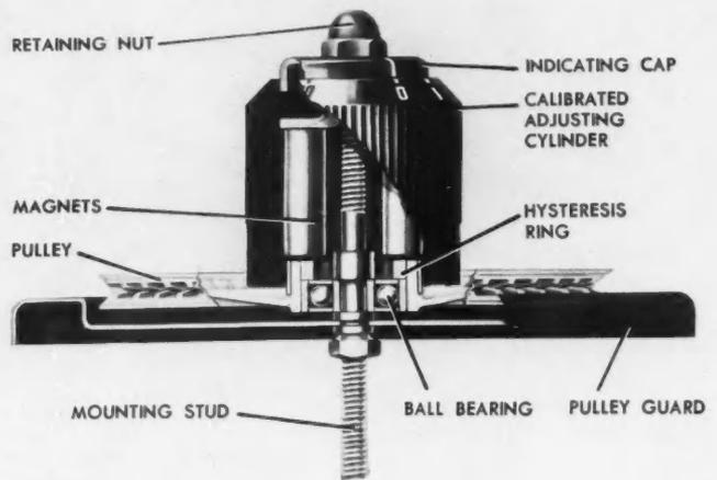
SPEED-TORQUE CURVES INDICATE EDDY-CURRENT EFFECT (LEFT); COMPONENTS OF YARN-TENSION BRAKE ARE ARRANGED AS IN CUTAWAY.
