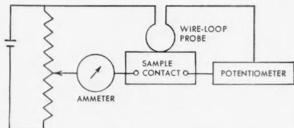
ELECTRIC CIRCUIT MEASURES CONTACT RESISTANCE OF SURFACE FILM.
