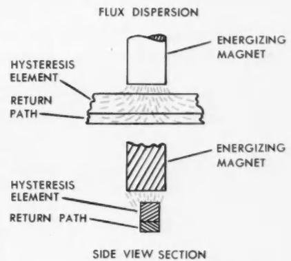
FLUX DENSITY, LENGTH OF AIR GAP, AND FLUX DISPERSION ARE FACTORS THAT DETERMINE TORQUE OF A ROTATING HYSTERESIS DEVICE.
