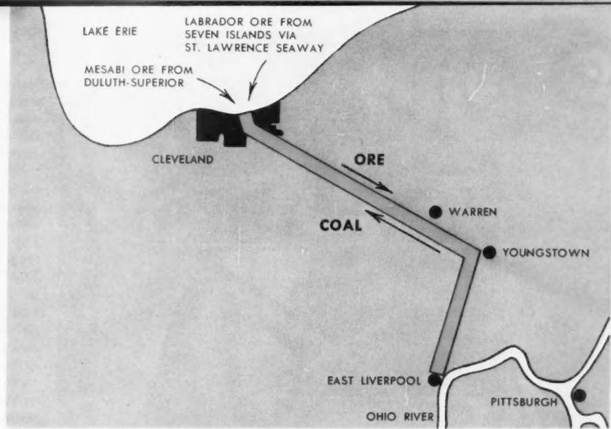
**PROPOSED 100-MILE RIVERLAKE** Belt Conveyor would carry coal from Ohio, Pennsylvania, and West Virginia fields to industries and utilities in Northeastern Ohio and to the lake terminal for shipment to other industrial areas. It would also transport ore from lake vessels to the river terminal for shipment via barges to steel plants in the three states.
