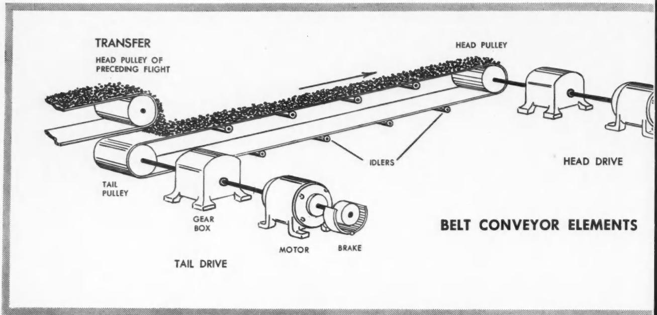
**BELT**—primary element in a belt conveyor—has rubber duck covering to protect the cotton duck, nylon, or steel-cable core from abrasion and weather. Idlers, pulleys, power drives, and supporting structure form the supplementary parts. Combined with others, one belt becomes a flight in a long-distance conveyor like the Riverlake proposal.
