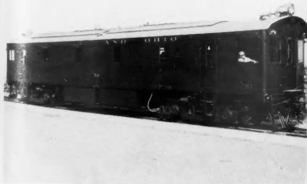
**DIESEL-ELECTRICS** having a G-E box cab invaded the passenger field in the mid-30's with 12 times the power of the early "oil-electric."
