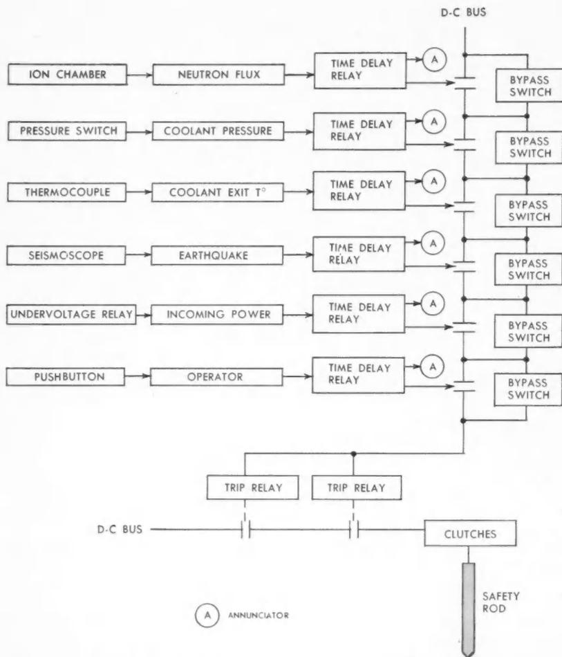
**A CONTROL-ROD CIRCUIT** consists of a number of sentinels that monitor certain conditions and properties, reporting to a series circuit that controls a set of trip relays.
