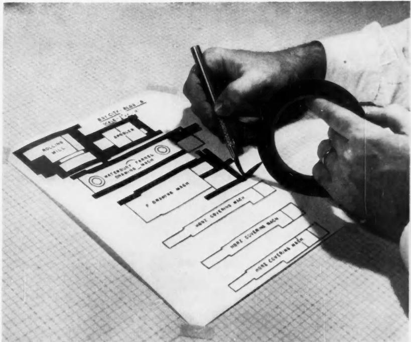
**ONE-FOURTH-INCH BLACK TAPE** or opaquing ink fills in the outside areas of complicated outlines so that the template can be easily cut out when reproduced.
