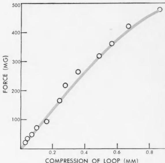
CURVE SHOWS CALIBRATION OF PLATINUM WIRE-LOOP PROBE.
