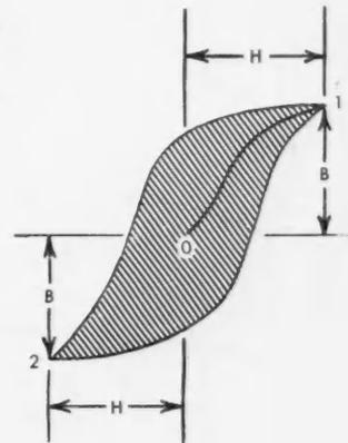
**PRINCIPLE UNDERLYING** a hysteresis torque device is continuous tracing and retracing of the magnetic material's hysteresis loop. Repulsive force is independent of speed.
