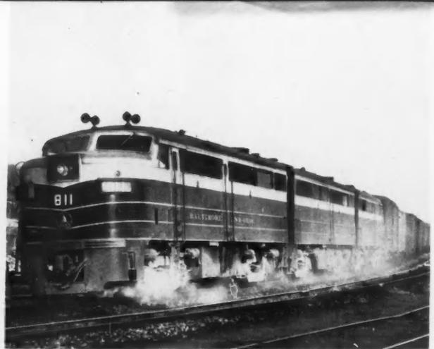
**THREE-UNIT 4800-HP DIESEL ELECTRIC**, using G-E electric equipment, typifies today's freight and passenger locomotives.
