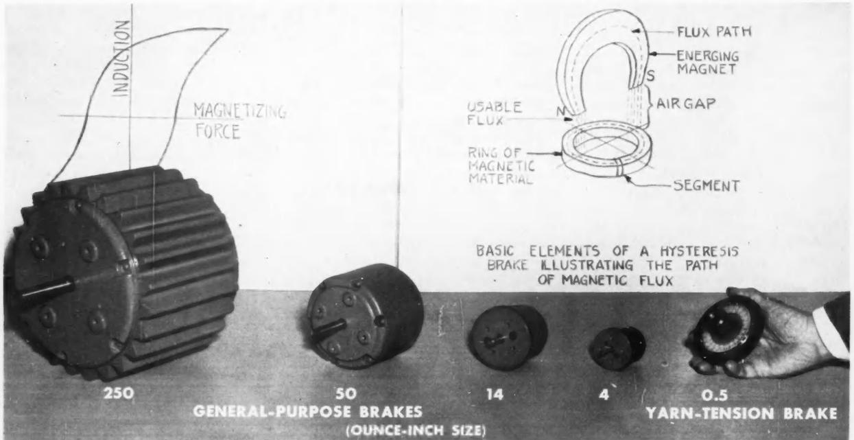
FOR GREATER VERSATILITY, TORQUE RANGES OF FOUR GENERAL-PURPOSE HYSTERESIS BRAKES OVERLAP BY A SUBSTANTIAL MARGIN.
