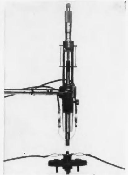
PRESSURE OF THE WIRE-LOOP PROBE ON A CONTACT BUTTON IS INCREASED IN CONTROLLED INCREMENTS WITH A MICROMETER HEAD (RIGHT).
