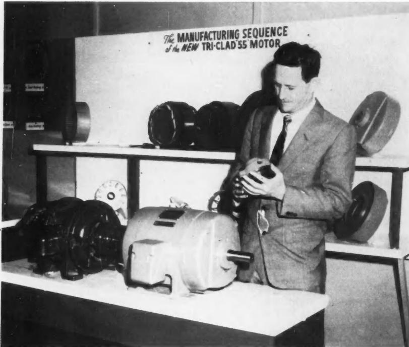
**IMPROVED BEARING HOUSING** examined by author lessens normal lubrication maintenance of new 10-hp induction motor (right). Motor at left illustrates former appearance.
