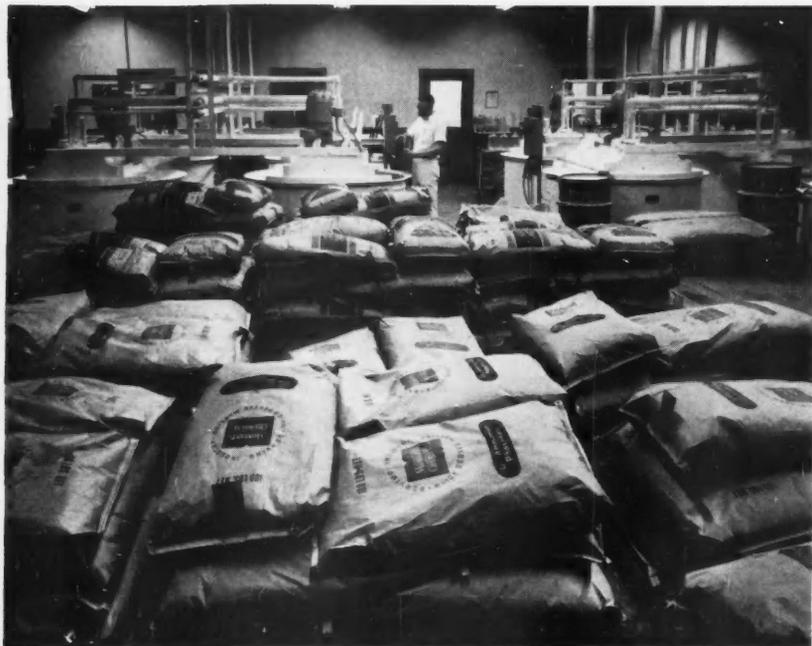
**CALCIUM CHLORIDE** and di ammonium phosphate, two common chemicals used as lamp phosphors, are treated in large glass-lined tanks for solution and purification.
