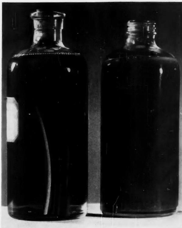
PLASTICS REMAINS FLEXIBLE IN OIL; RUBBER DISINTEGRATES.
