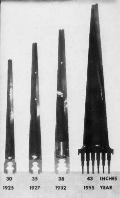
**LAST-STAGE BUCKETS** of the 3600-rpm series vibrate in 10 to 20 resonant patterns.
