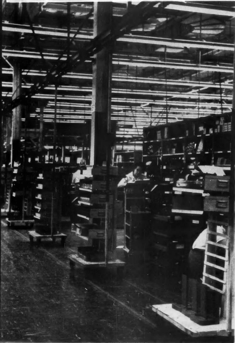
**3** Three conveyor systems carry parts from stockrooms to various product-assembly areas throughout the plant. The trucks are disengaged easily from the conveyor at the appropriate work station. No traffic problems and a clean plant layout are two results.
