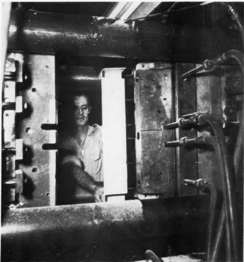
**INTRICATE** injection steel molding equipment is used for making plastics parts for air-conditioning units that eventually find their way into many homes, offices, schools, and stores.
