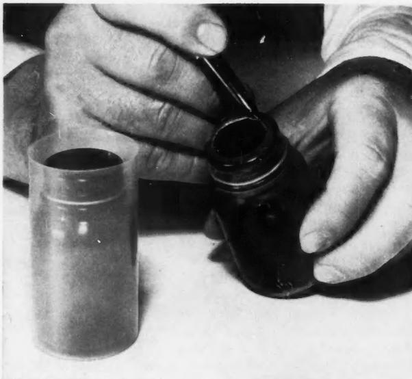
**ENCAPSULATION** of ink bottle illustrates unique means of insulating a conductor. Film heated to 150 C shrinks to fit all contours.
