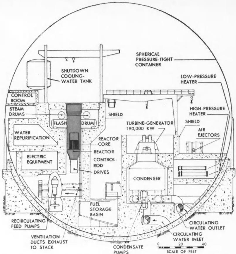
CROSS SECTION OF NEW PLANT'S SPHERE SHOWS PRELIMINARY ARRANGEMENT OF EQUIPMENT.
