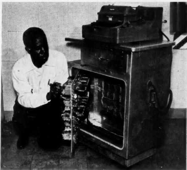
**RELAY-STORAGE** and control unit directs digitized information from converter to tape-perforating typewriter—a vital function.
