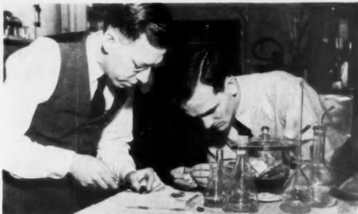
**1939** G-E physicists K. H. Kingdon and H. C. Pollock prepare small samples of natural uranium for processing by electromagnetic separations method.
