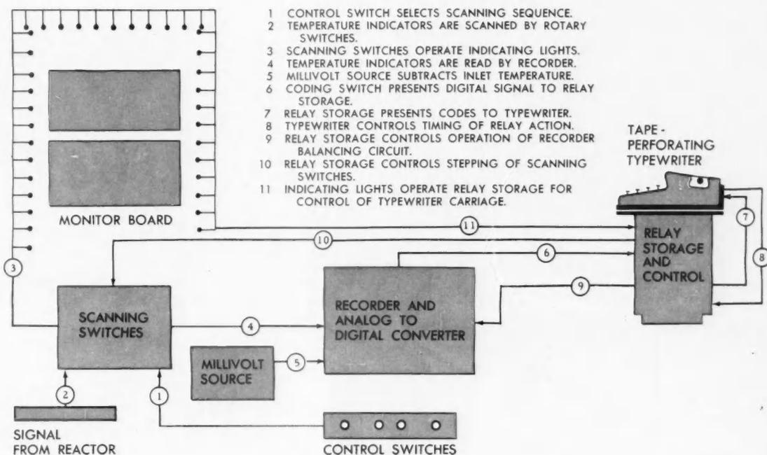
AUTOMATIC TEMPERATURE RECORDER ELIMINATES THE EXPENSIVE DRUDGERY OF MANUAL DATA PROCESSING AT THE HANFORD OPERATION.
