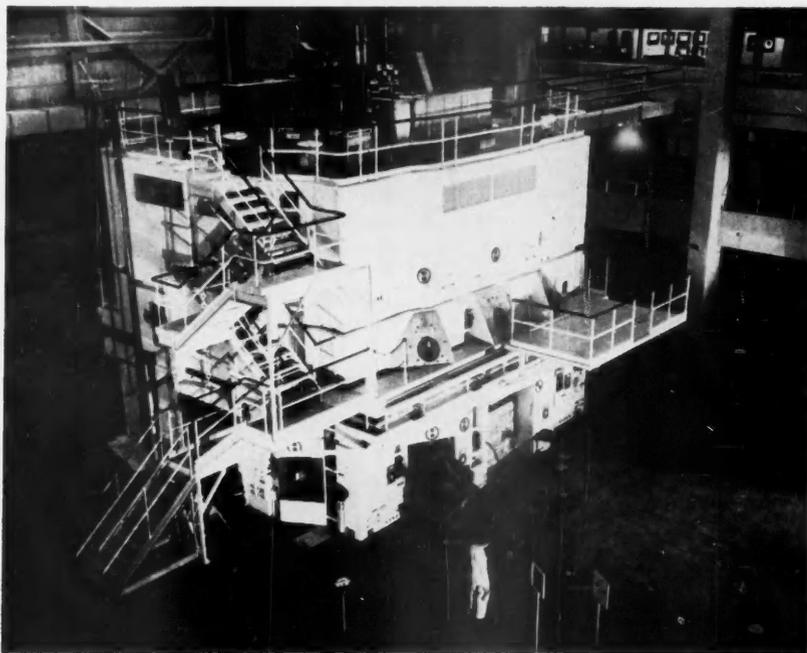
**MTR** Materials Testing Reactor, being made available to industry for irradiation service, has a universal coffin used to remove radioactive plugs and test specimens.
