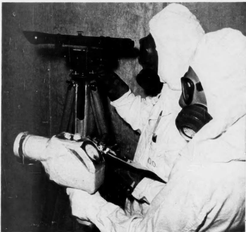
TELESCOPES PERMIT THE VIEWING OF CONTAMINATED EQUIPMENT REQUIRING MAINTENANCE.
