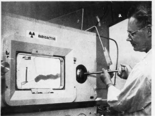
**FLEXIBLE BOOT** of a through-wall tool prevents contaminants from being carried to the outside as the arm is pulled through the wall.
