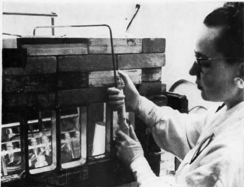
**PIPETTE** measures hot sample as operator applies suction in a controlled manner with a hypodermic syringe, the air column in the tube controlling the amount of sample.
