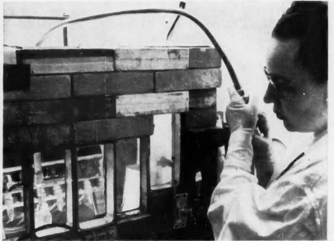
**TONGS**—here a two-cable control between handle and working ends—are the fundamental tool to grip, lift, and move radioactive items.
