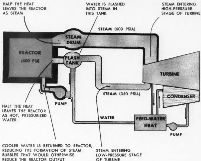
DUAL-CYCLE REACTOR ADDS TO THE BEST FEATURES OF THE BOILING-WATER REACTOR.
