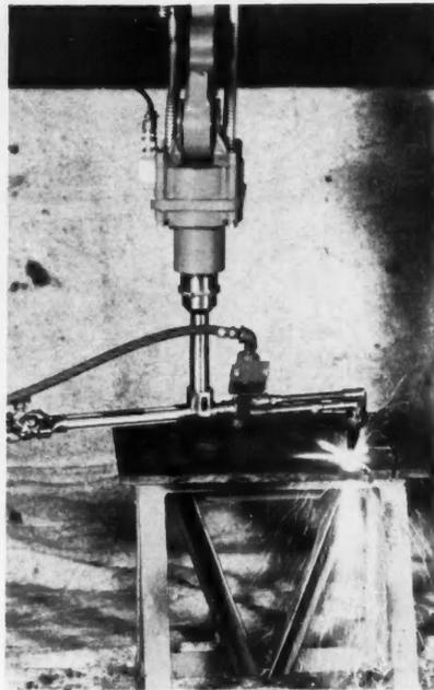
**MANIPULATOR** directs an oxyacetylene torch for remotely cutting steel plate.
